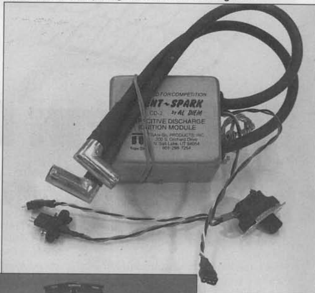
Tran-Sil electronic spark ignition module for twin ignition.
