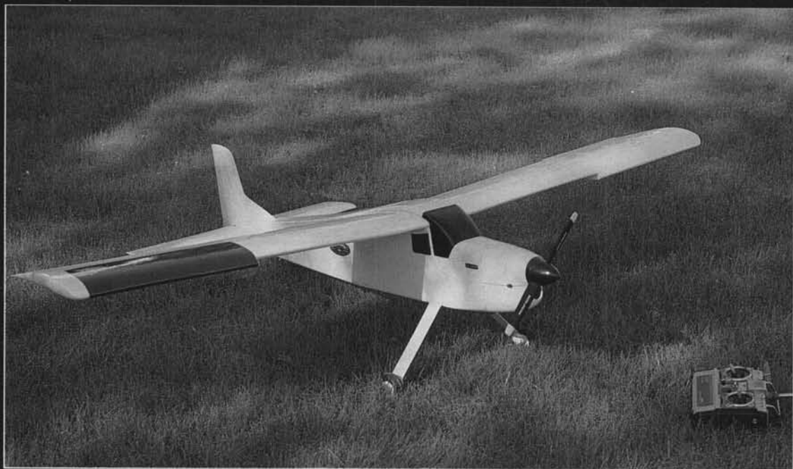
The Osprey is all set to fly. It is an easily flown sport model, with interchangeable wheeled landing gear or floats.
