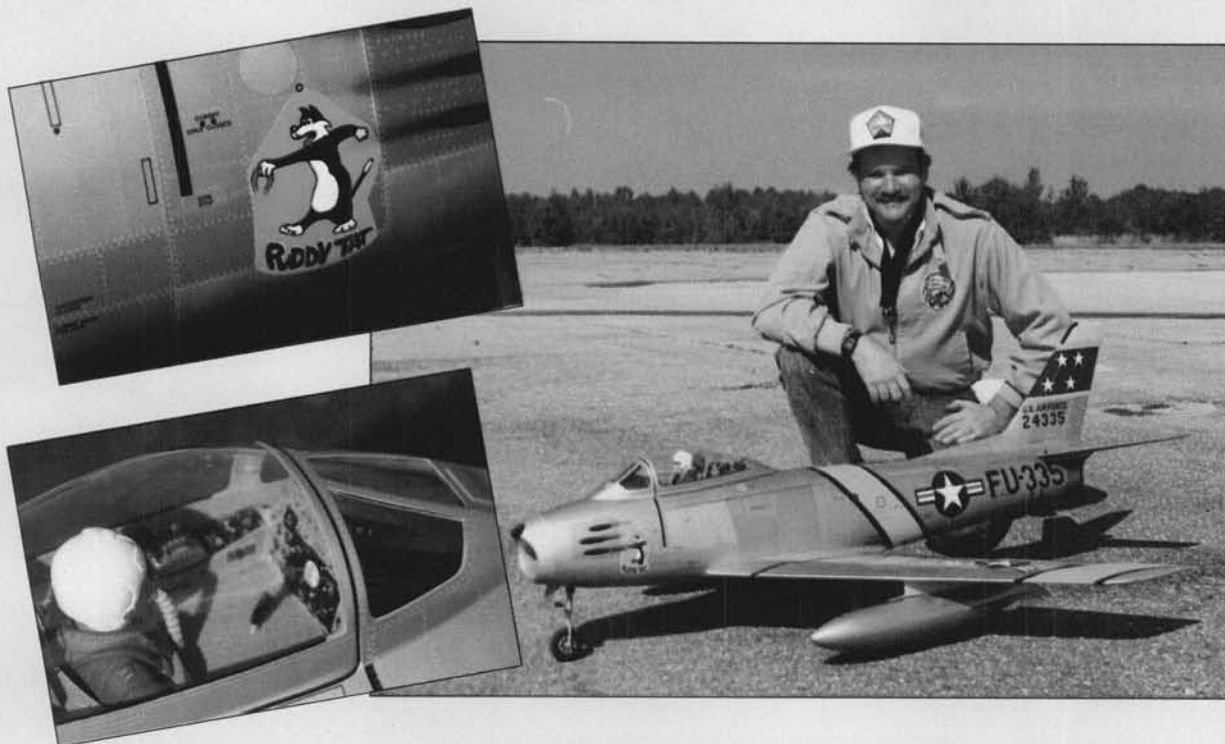
Terry Nitsch deservedly took top honors at De Land, Florida, with his F-86 Sabre, a magnificent piece of workmanship. With a KBV .82 and fan combo, it's no slouch in performance, either. (Insert top) The rivets (all 30,000 of 'em!) and the "Puddy Tat" art on Terry's F-86 are dry transfers that were professionally custom made just for this particular model. Must have cost him a small fortune. (Insert bottom) Cockpit details of Terry's F-86 Sabre.
