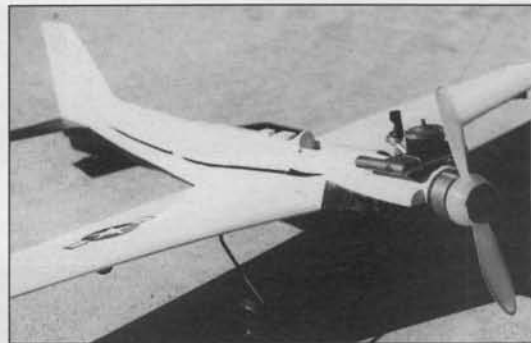
This ancient Ready-To-Fly plastic U-Control model was made by A.C. Gilbert Co.; has a Gilbert .07 engine with twin exhausts. Does any reader know how old it is?
