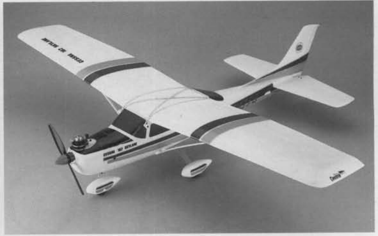
CESSNA SKYLANE 36" Wingspan 31" Length Cox .049 Engine Powered
