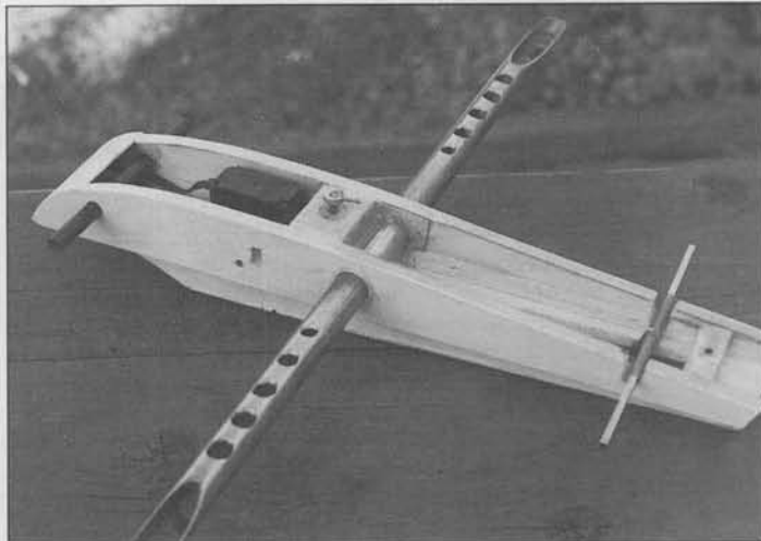
Wing center section incorporates slip-off wing mount and wing-joining rods. Note slip-out nut.
