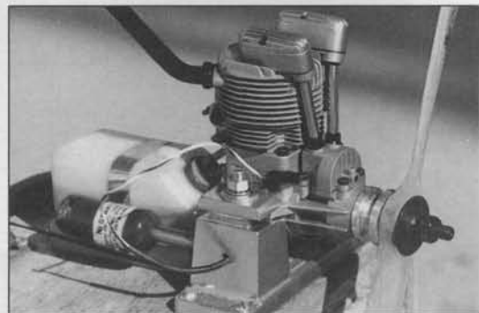
The SAFE Start engine test stand easily holds almost any size engine. It has a remote locking socket for attachment of a glow plug starter. See text for more information.
