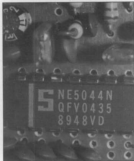
(Left) Here we see the uniform neatness of assembly that comes with automatic high volume production. The Signetics NE5044 chip is used by several manufacturers around the world with great reliability. (Right) The output gear of a NES 507 servo is in Stu's fingers and shows the spoke that protrudes downward. The spoke fits into a matching yoke that drives the delicate feedback pot inside the servo. This "spoke 'n yoke" is indirect drive that lessens measured up-link performance, but makes servos last much longer in a vibrating environment.
