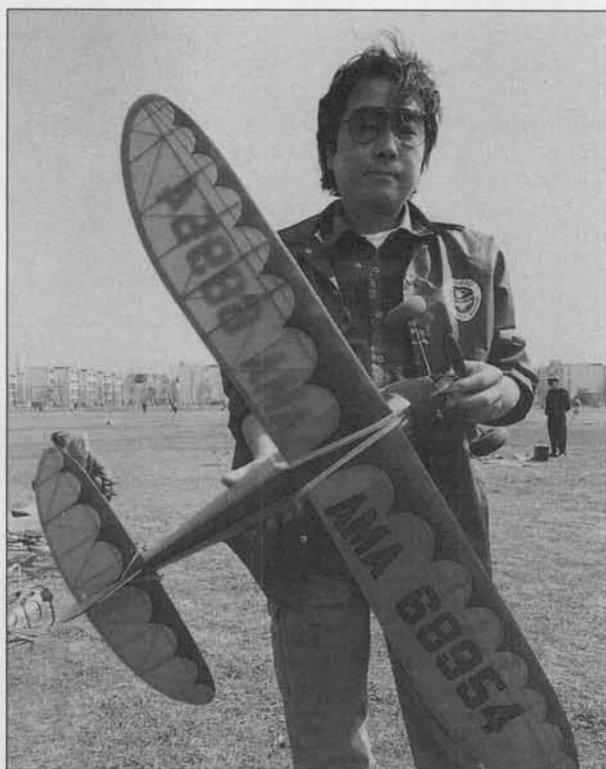
Yoshindo Harada of Japan, with his "old timer" which is powered by an Italian compressed-air motor. Eighty strokes of the air pump yields 40- to 50-second flight durations.
