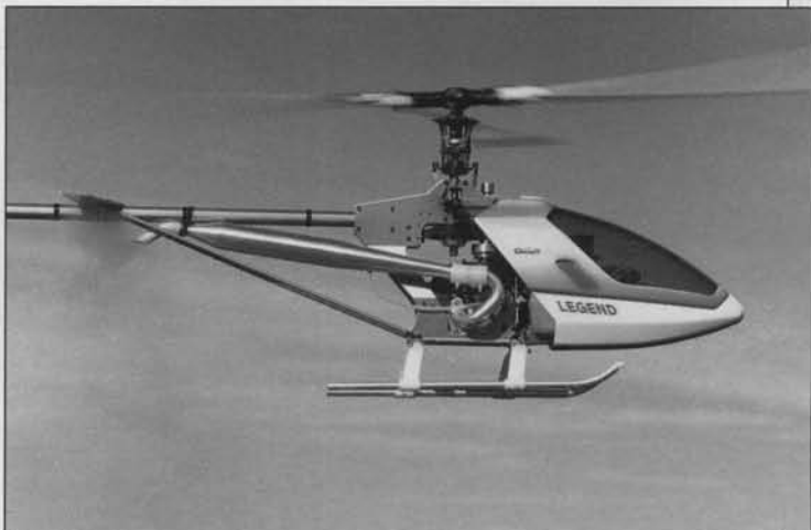
Jim O'Brien's Legend with a long Hatori tuned pipe. It sounds very good, and has lots of power, too. The header is from Century Super Tuned Pipes. Royce Brademan did the paint job.
