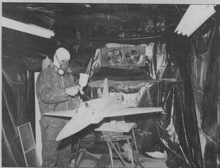
The author in his homemade spray booth as described in the text, suited up for two-way protection, and applying a coat of primer to the model. Protective glasses left off to set camera for photo. Note spark-proof exhaust fans, fluorescent lighting, and gravity-feed type spray gun.
