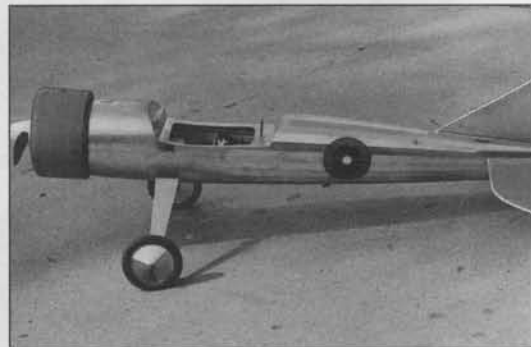
The Recon wing is retained by a single bolt, which detaches easily for transportation of the model.
