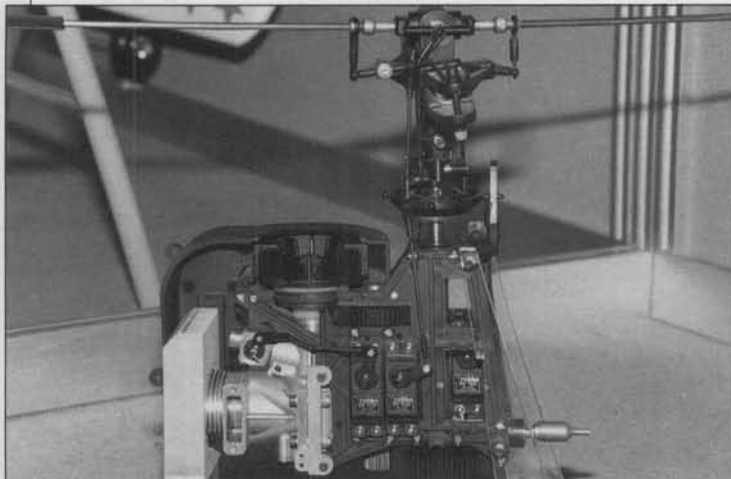
The Robbe/Schluter Prokopter mechanics. It is made from molded glass-filled nylon. Very light weight and strong. Similar to Heim mechanics, it has counterclockwise rotation main rotor, and needs CCPM mixing. This unit is for the pod-and-boom Prokopter, but it is ideal for Robbe's scale fiberglass fuselages.
