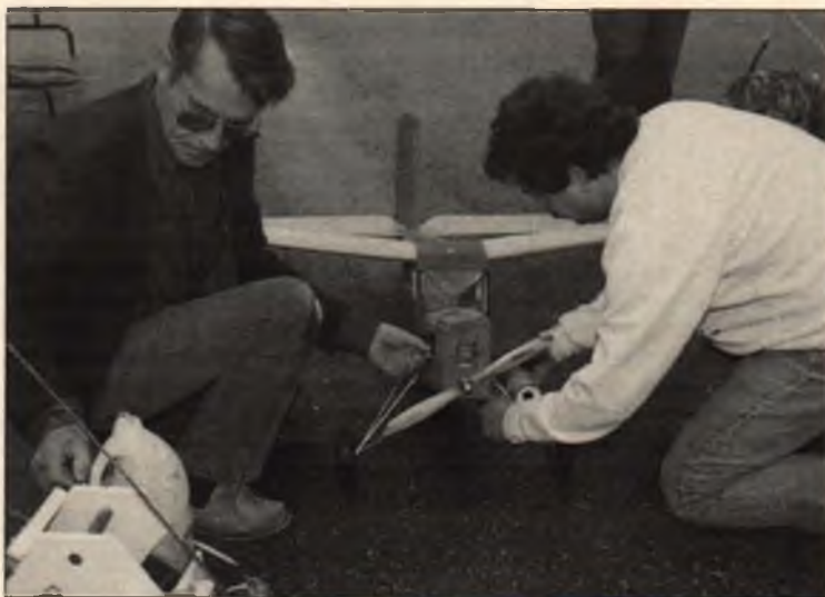
Charlie Strange (left) and Monte Salot strap the video unit to the landing gear of Charlie's big 1930s-vintage Miss Philadelphia. Stable, slow-flying Old Timers are a perfect platform for an airborne camera.
