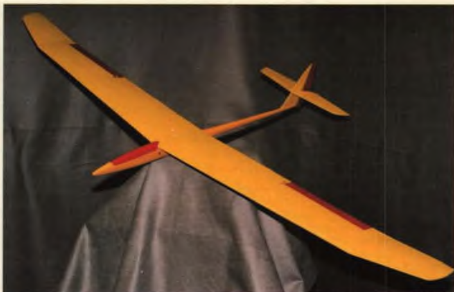
Northeast Sailplane Products' new Culpepper Models "Dove" 2-meter competition sailplane features an exceptionally clean, lightweight fiberglass fuselage and a high aspect ratio, fully sheeted foam core wing. Controls are ailerons, rudder and elevator; flaps are optional but highly recommended. The S07037 airfoil plus the 23-ounce flying weight equals great thermal performance.
