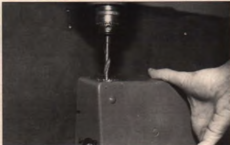
Installation of the MicroPeaker is simplicity in itself. The only modification needed to the Astro Flight charger is to drill a 5/16-inch hole in the plastic case for the MicroPeaker's wires.
