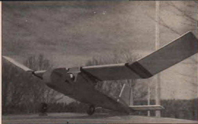
Two views of an earlier version of the Pushcart. For safety's sake, the designer recommends fitting the engine with a left-hand prop so you can retain the use of the stock Cox spring starter. Fuselage is a simple sheet balsa box and will accommodate standard-size radio gear with ease.
