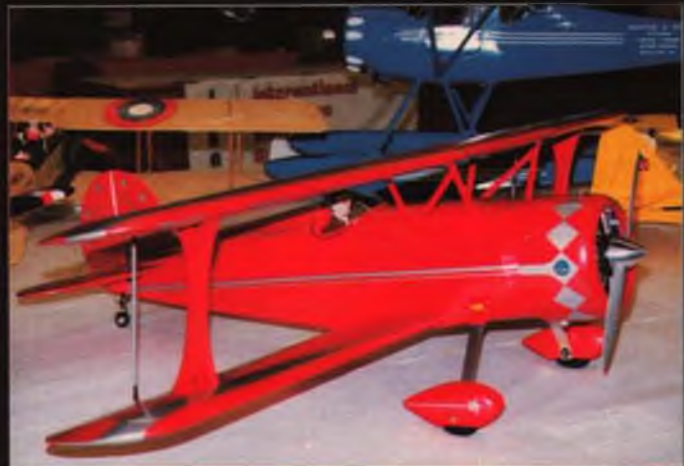
Walt Wyrick's latest project is this 70-inch span Great Lakes biplane, powered by an O.S. 108.
