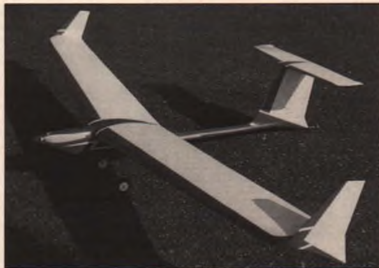
The graceful and exceptionally clean Maxi-Fli took 1st place in the Cargo event at the recent Astro Flight Electric Championships for designer/pilot Chuck Hollinger. The geared Astro 05 cobalt, running on seven cells, had no trouble at all getting the Maxi-Fli's 14.3 pounds off the ground for the prescribed flight task. At that weight, the wing loading is over 2 pounds per square foot!
