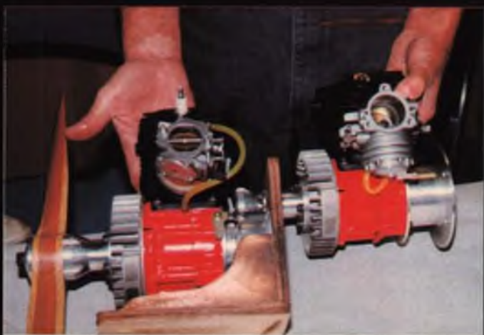
John Eaton, who runs J&K Products out of Long Beach, California, offers a big Stihl engine for Unlimited racing with either a Tillotson gas carburetor (left) or a Mikuni alcohol carburetor (right). The alcohol carb is $135 plus postage and handling.
