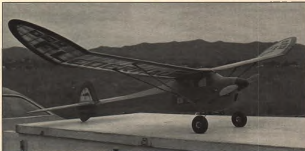
Photo No. 1. Back in the late '70s, SCAMPS member Jim Adams came up with this strut-braced cabin design for the Old Ruler event. Dubbed "Der Fledermaus" (German for "bat"), the airplane flew well with an inverted Anderson Spitfire for power.
