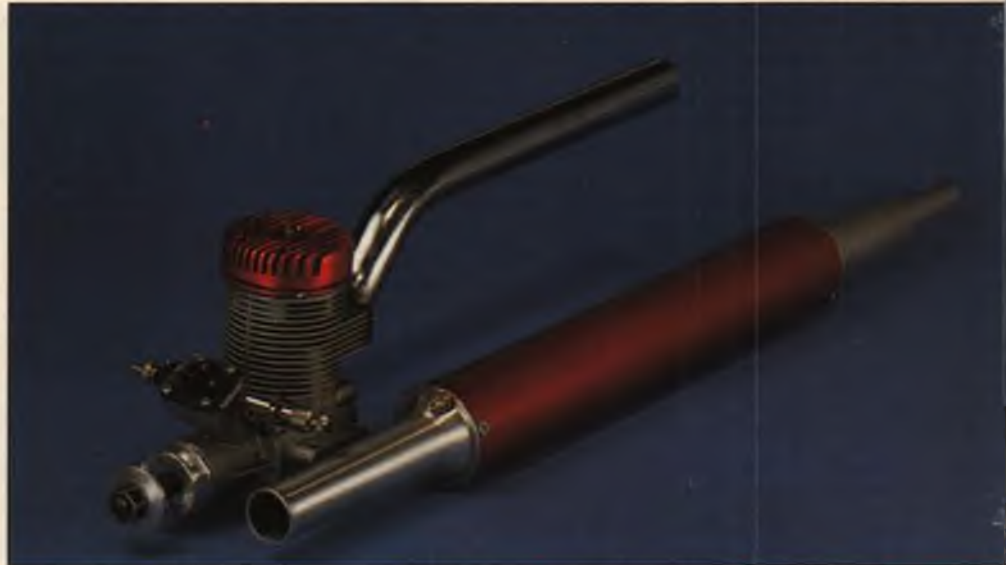
■ LEFT: The beautifully built Webra .61 Long Stroke with Dynamix carb is unquestionably the equal of any of the 10cc two-strokes currently being used in F3A Precision Aerobatics competition. Rear exhaust configuration is almost de rigueur for today's pattern aircraft. ■ RIGHT: The .61 Long Stroke and the unusual tuned pipe designed specifically for it—see diagram also.
