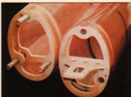
The Python's demounted fuselage halves show off the beautiful workmanship. The formers are made of fiberglass and end grain balsa laminate. The "tongue" on the aft section (right) carries the rudder servo.
