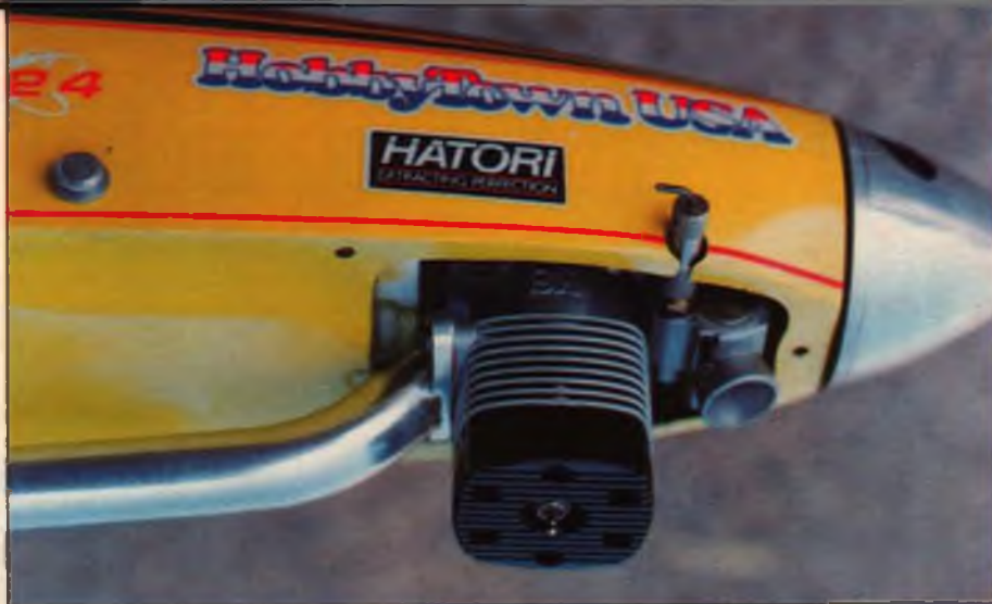
Removing the cowl reveals the inverted YS .61 AR, one of the most powerful of the current crop of two-stroke 10cc pattern engines. Engine is mated to a Hatori header and tuned pipe. Designer Quique Somenzini uses a YS 1.20 four-stroke in his model, which would eliminate the nose weight our columnist needed with the much lighter .61.
