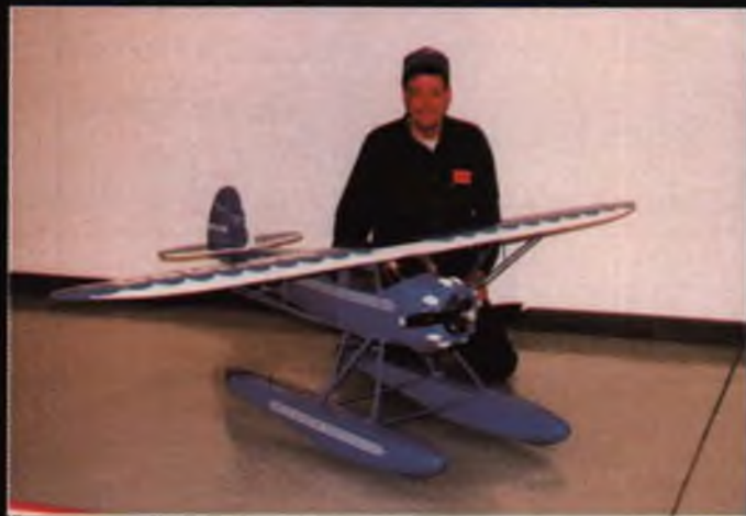
Cliff Sand drove from Eagle Point, Oregon to show his Monocoupe on floats. Built from an Ikon Northwest kit, the ship weighs 22 pounds and is powered by a Super Tigre 3000.
