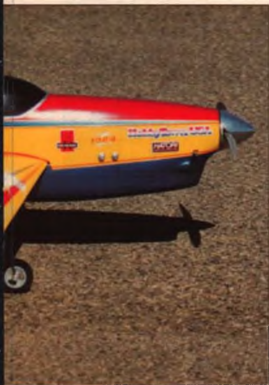
Author's model was finished with Coverite 21st Century paint on the fuselage, 21st Century film on the wing and tail. The eye-catching design was done in bright colors, which makes for good visibility in any attitude.
