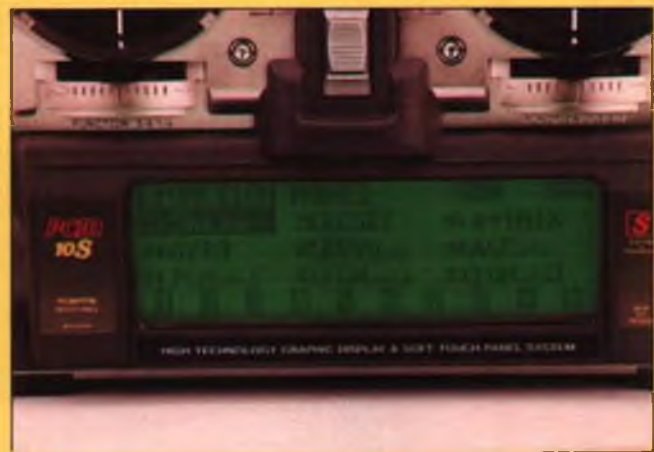
The PCM-10S transmitter has a very easy-to-read liquid crystal display screen. The radio is programmed by pressing directly on the screen. The PCM-10S displays nine function names at a time; the old PCM-10 displayed only one function name at a time. Photo courtesy Horizon Hobby Distributors.
