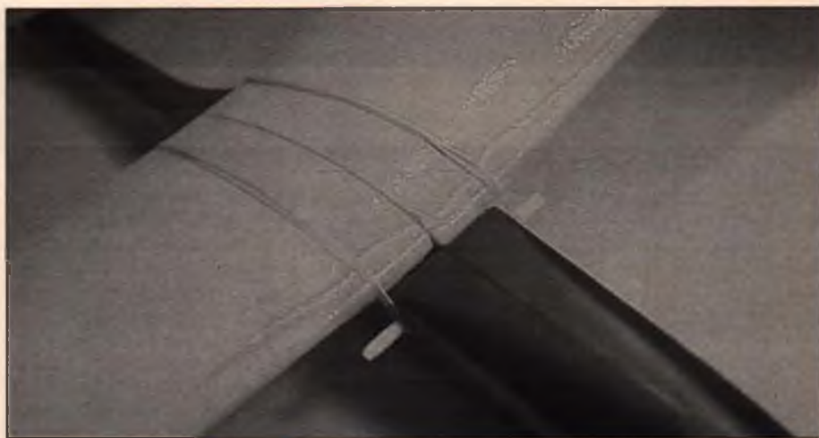
■ ABOVE: The slight difference in wing root chord lengths is more of an eyesore than anything else. This was the only flaw our author noted in the kit. Has no effect whatsoever on the flight characteristics, nor is this mismatch visible at a distance.
