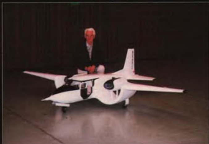
Oregon modeler Ed Hess tackles some difficult projects—his latest is a Custer Wing CCW-5. It weighs 48 pounds, wingspan is 10 feet 6 inches, power is two Saito 300 twins mounted as pushers.
