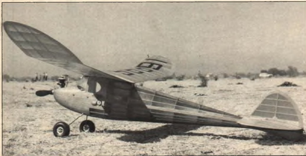
Photo No. 2. The graceful "Swift," sort of reminiscent of the So-Long in profile, was master designer/builder Bob Oslan's Old Ruler entry. Covered in silk and dope, of course, and powered by a Forster .29.
