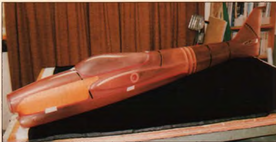
Henry Piorun's new Python fuselage is 79 inches long. To make his own personal model easier to transport, Henry engineered a clever joiner system that allows a two-piece fuselage, split just behind the wing trailing edge. Careful use of carbon fiber and Kevlar makes for a very strong and light unit.
