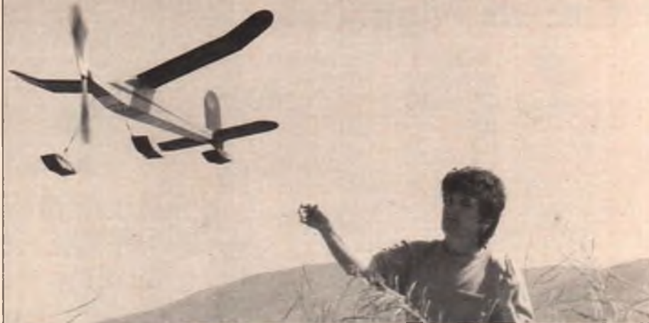
Sandy Peck launches the prototype Peck kit on a trimming flight. The model gets its name from the fact that only a few seconds are needed to convert from wheels to floats or vice versa. The Peck kit is an authentic replica of Tad Dietrich's 1938 cabin rubber model and is legal for SAM O.T. rubber events. Peck-Polymers photo.
