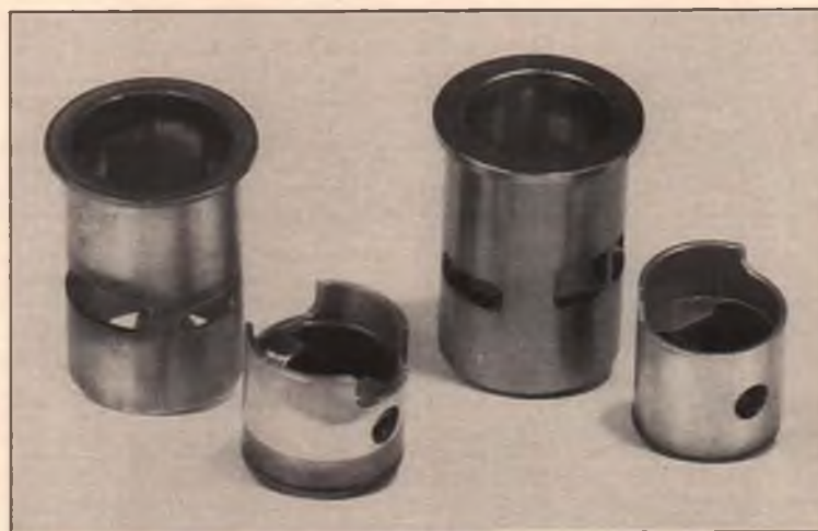
The Webra Speed .61 liner and piston (left) as compared with that of the smaller bore Long Stroke. Note the difference in the thickness of the liners, and that the Long Stroke's liner has a bar in the exhaust port to retain the Dykes ring.
