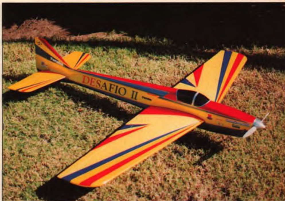
Author's model was finished with Coverite 21st Century paint on the fuselage, 21st Century film on the wing and tail. The eye-catching design was done in bright colors, which makes for good visibility in any attitude.
