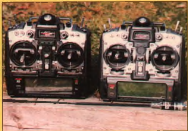
A comparison of the old JR PCM-10 (left) and the new PCM-10S. Most of the differences are internal rather than external. In the foreground is the optional JR base loaded whip antenna, which is about 18 inches long. James has been using one of these and reports no reduction in range over the standard antenna.
