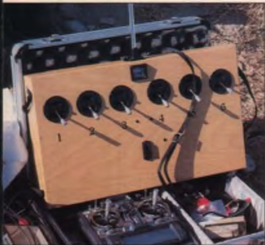
The Dornier uses a separate radio system to control the six engines; each engine can be controlled independently by the flight engineer by means of this special transmitter devised by John Wisniewski. John was the pilot for the flight. Bill Reed was the flight engineer.
