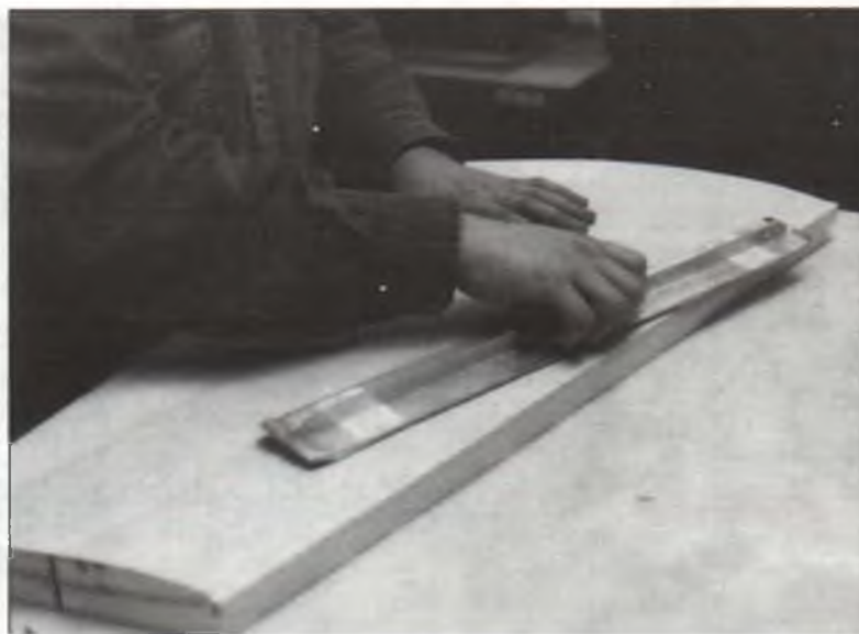
After removing the excess material with a Rabbit plane, the leading and trailing edges are finished with a long sanding block.
