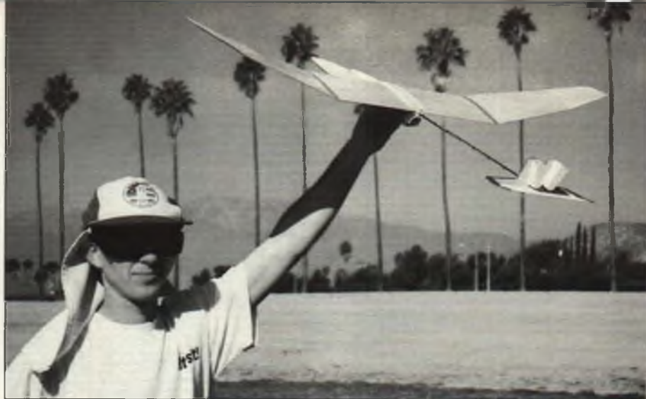
Mark McReynolds is mainly a model rocketry buff, but couldn't resist bringing his RC boost glider to the Dash for Cash. Model uses a C engine tube and nose cone for a fuselage, has a 215 square inch hollow balsa wing, weighs only 6.5 ounces with two Kyosho KS10 servos and a 27 MHz band Hitec two-channel receiver. Model was prone to tip stalling if slowed too much and wasn't as maneuverable as most, but was interesting nevertheless.
