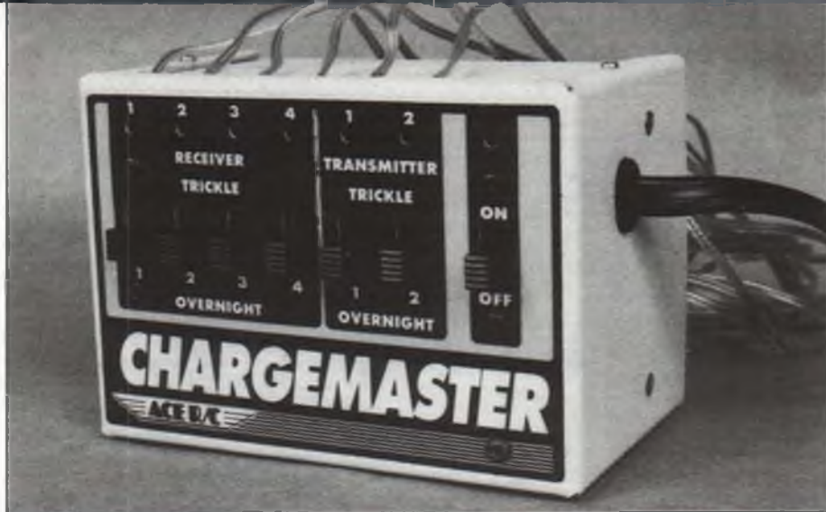
Chargemaster is a multiple-output AC charger with four receiver outputs selectable at 25, 50, 90 or 120 mA, and two transmitter outputs selectable at 50 or 90 mA. Current selection is made by installing resistor values as specified by a chart furnished. Manual changeover to a pre-selected trickle rate is done with individual channel switches.
