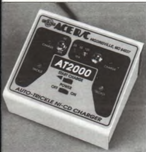
The AT2000 is a versatile multi-system AC charger with dual outputs for one to ten cells. One output provides 50 mA, the other is switchable to 25, 50 or 120 mA. After a 16-hour charge period, the rate automatically reduces to a 10 mA trickle.
