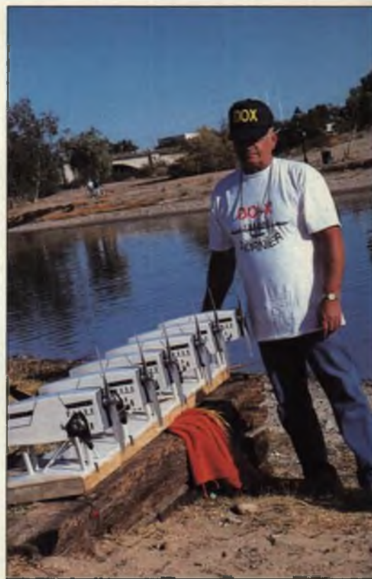
A clever design feature of the model Dornier is the engine module—a strong, removable section of the wing that supports all six engines along with their fuel systems, mufflers, servos and throttle radio. It's a completely self-contained unit that simply bolts to the wing, no other hookups required.
