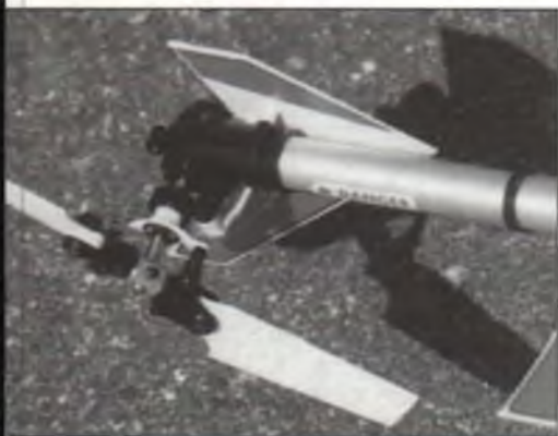
The Concept 10 uses a belt drive tail rotor. The sliding ring tail rotor control is similar to that on the Concept 60 and X-Cell. High tail rotor speed gives quick yaw response.
