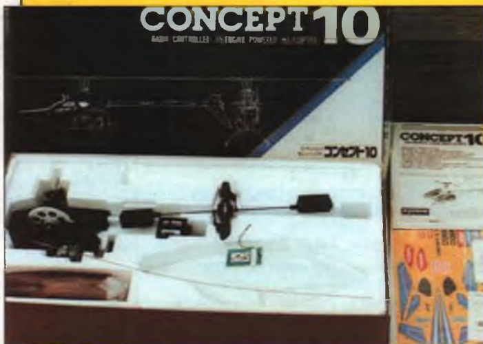
This is how the Concept 10 arrives—about 80 percent pre-assembled by the factory. Even with careful building and setting up, it took James only seven hours to complete.
