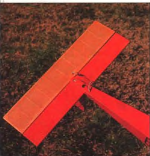
Empennage assembly is held on with two 6-32 nylon bolts, can be quickly removed for safe transport.
