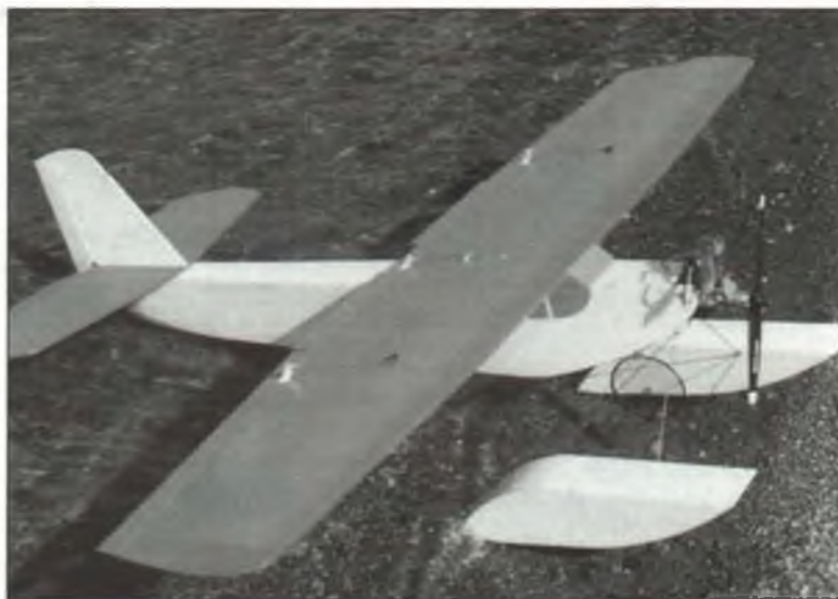
Francis simplified his later fixed-gear float design by just mounting the wheel (outlined here for clarity) on the inboard side of the float.
