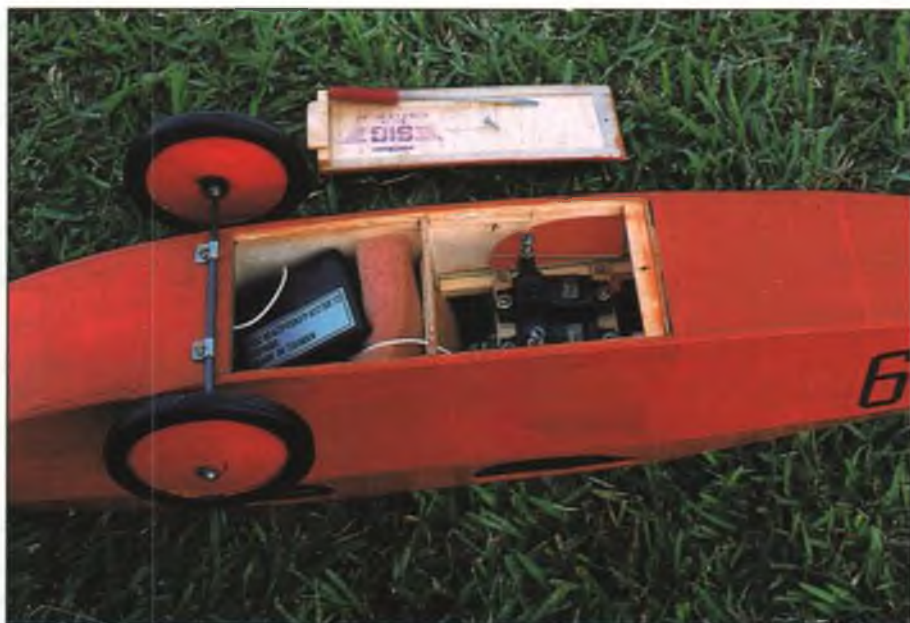
Access to the radio is through a hatch on the bottom of the fuselage. Straight-axle landing gear is secured with straps cut from an aluminum beverage can.
