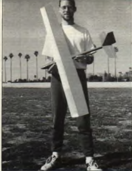
K&A Models produces a kit for the "Thermal Buster" HLG, displayed here by K&A's Ken Williams. Model features an Eppler 205 airfoil with conventional balsa D-tube wing structure. It has a wing area of 354 inches over a full 59 inch wingspan with a flying weight of 12 to 14 ounces. For info, call K&A at (310) 804-0006.
