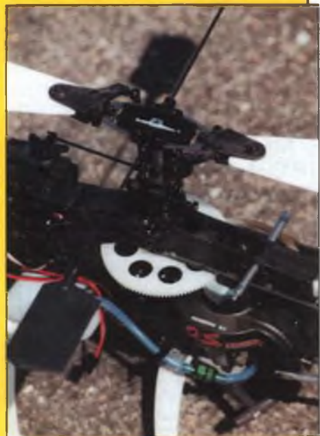
The hingeless main rotor head is the same as on the electric-powered EP Concept. The thin steel flexbeam gives soft flapping and thus a docile hover, but is still stiff enough for aerobatics.
