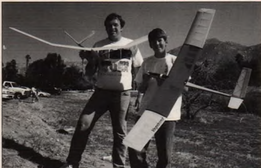
Larry Jolly is returning his focus to his kit line and has just introduced the new Vagabond HLG. Conventional balsa D-tube structure with conventional balsa fuselage and V-tail stabs make it attractive to the foamophobic masses. The performance, handling and stability of the design are truly first rate. Larry's son Emmett has become quite the competitor in RCHLG with his Vagabond.
