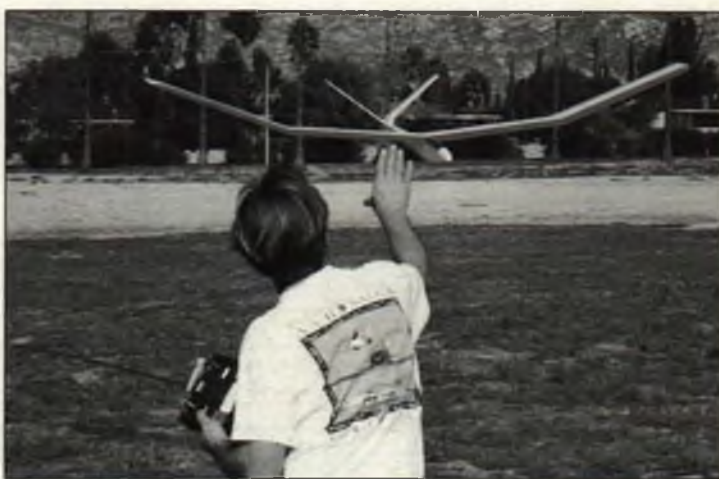
Mark McReynolds is mainly a model rocketry buff, but couldn't resist bringing his RC boost glider to the Dash for Cash. Model uses a C engine tube and nose cone for a fuselage, has a 215 square inch hollow balsa wing, weighs only 6.5 ounces with two Kyosho KS10 servos and a 27 MHz band Hitec two-channel receiver. Model was prone to tip stalling if slowed too much and wasn't as maneuverable as most, but was interesting nevertheless.
