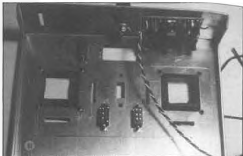
RF Module installed in case. Also note dual rate switches installed.
