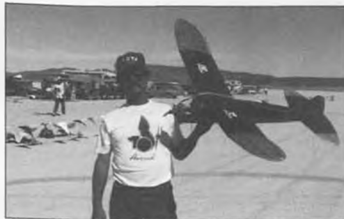
2. Tom Empey's Torp 29 powered Brooklyn Dodger features unique pull-pull cable controls made of dental floss (unwaxed) for the ultimate in light weight. Seems to work OK so far, although one line came off a servo at the SAM Champs and he could only make right-hand turns.
