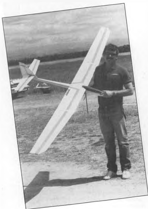
Keith's Cumic wings slide onto joiners built into removable root fairing or center section, which bolts down. Tape cleans up the airflow and holds wing snug to the fuselage.
