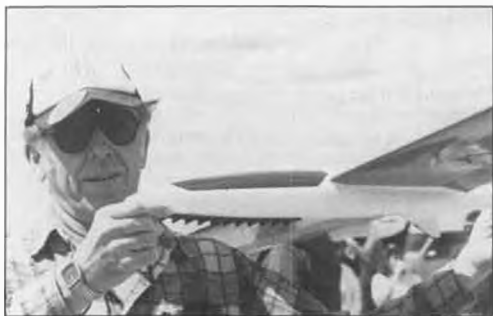
Mack the Knife has nothing on Art McNamee's soarer, sporting rubber "shark's teeth" and fish-flap skid behind two hook. No roll-out, no flip-overs (see text).
