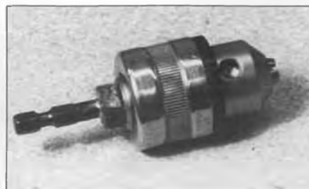
Here's a modification that will let your rechargeable screwdriver do double-duty as a drill. Some brazing or silver soldering is required. See text.
