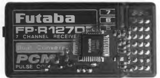
The heart of the new R124DP/R127DP PCM receivers is Futaba's custom microprocessor circuitry.
