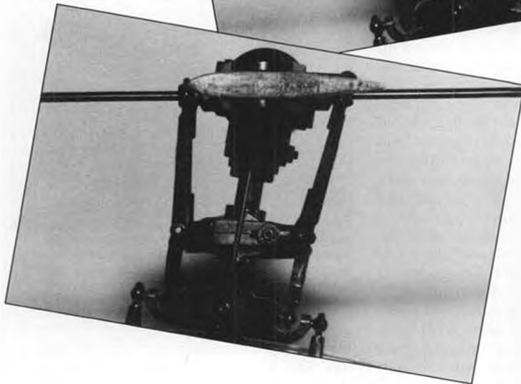
This sequence of photos demonstrates the Concept 30's 90% Bell-Hiller mixing ratio. Tilting the flybar 10 degrees relative to the rotor shaft will change the main rotor blade pitch by 9 degrees. The flybar may tilt relative to the shaft because of an outside gust or the pilot's cyclic input. Note that the swashplate is level in all three photos.
