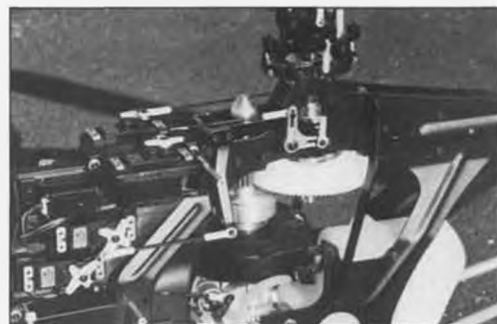
Side frames are black anodized 2mm thick aluminum and have ridges stamped into them for added strength. The Excalibur rates an "A" for crashworthiness; see text.
