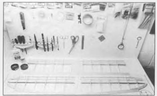
The three wing panels are constructed separately, flat on the building board over the plan sheet, and assembled later.
