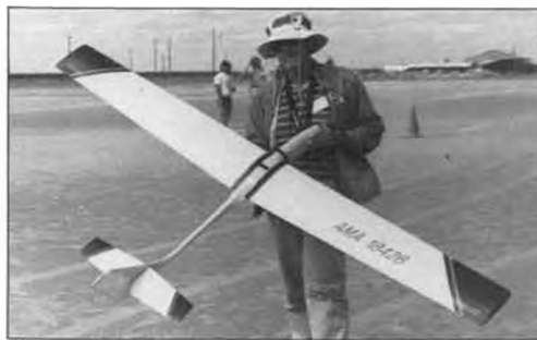
Myles Moran really modified his Pantera. Looks like a Larry Jolly Cheetah now, with S3021 airfoil, flaps, ailerons, and more (see text).
