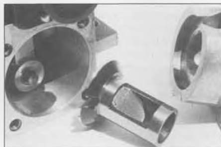
The drum intake valve (center) features an angled insert pressed into the bore that, in theory at least, deflects the incoming fuel mixture toward the cylinder bypass ports.
