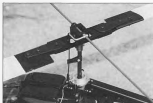
The Hiller control system as used on the GMP Rebel. This design uses a flybar, and only one control rod is needed from the washplate to the flybar. Cyclic control inputs will rotate the flybar to change the angle of the Hiller paddles. Refer also to Figure 3.
