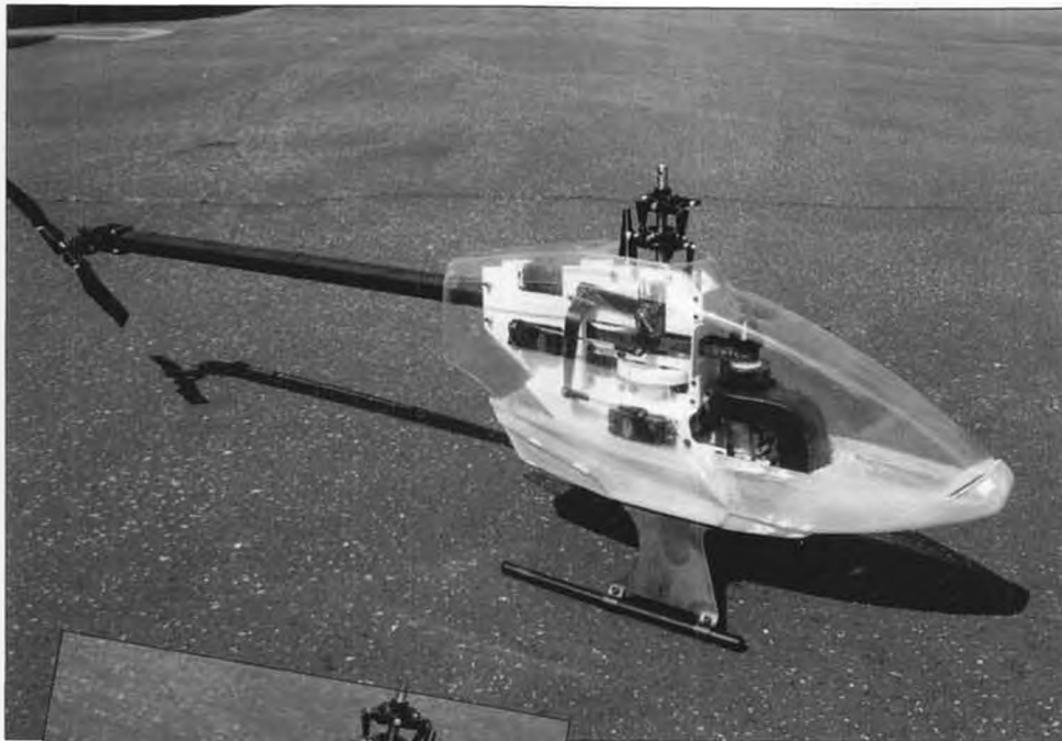
(Above) GMP's new 30-size "Viper" should be available by the end of summer. It uses a unique fiberglass pan for the lower fuselage, clear canopy on top. Will retail for about $400. (Left) A close-up of the Viper's innards reveals a forward-facing engine, belt drive transmission, belt drive tail rotor, and straight linkages from the servos to the controls. Rotor head will be an all-metal piece similar to the GMP Elite, but smaller.
