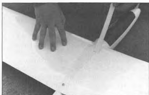
Keith's Cumic wings slide onto joiners built into removable root fairing or center section, which bolts down. Tape cleans up the airflow and holds wing snug to the fuselage.
