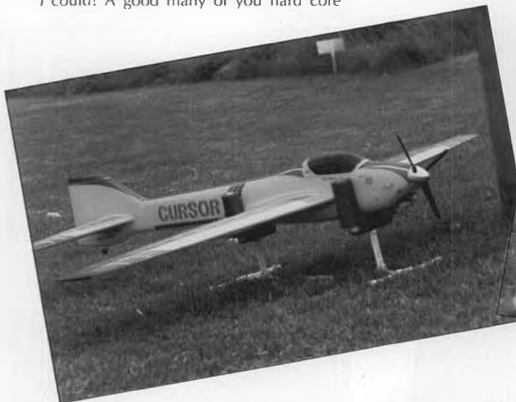
(Left) Rick Allison's prototype of the "Cursor," now being kitted by RC City. It's state-of-the-art throughout, a low mid-wing design with a thin airfoil and fairly sharp leading edge, and a large stab set on the thrust line. A very efficient and mean looking ship, especially with that four-blade prop! (Right) "Bogie" is the brainchild of Roy Speights. Note the placement of the wing and stab in relation to the thrust line. Photo by Buck Boynton.
