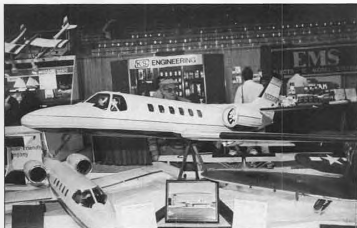
Big Cessna Citation II is the combined effort of Jerry Keller and Dave Escobar. Uses two O.S. .91/Dynamax fans, spans 114 inches and weighs in at 32 pounds. We'd guess it to be a very fast and smooth flying model.
