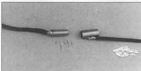
(Above) Mitch Poling's homemade power connectors are ultra simple, being made from hobby shop brass tubing, but they outperformed all of the commercial connectors Mitch tested except the Sermos. Small and light, too. (Below) This month's column tells how to polarize Deans connectors to prevent accidental backwards hookup.
