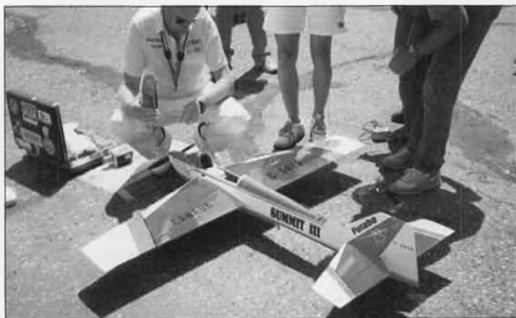
Top Canadian flier, Ivan Kristenson, flew his "Summit III" at the '89 Nats. This view clearly shows the long tail moment and very large tail surfaces that typify modern turnaround designs. Don Passey photo.
