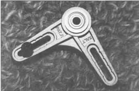
Just one example of the Excalibur kit's high quality is the roll control bellcrank, a metal casting that pivots on ball bearings. Position of the steel ball for the link can be adjusted to five different positions.
