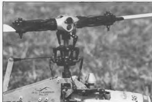
The modified GMP Prohead on the author's Cobra is a good example of the Bell control system. Note that no flybar is used; cyclic controls go from the washplate directly to the rotor blades. See Figure 2 also.
