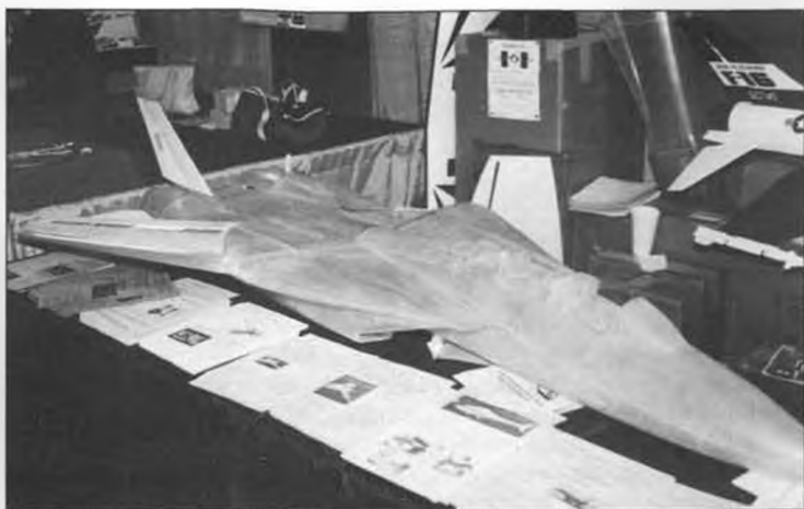
Yellow Aircraft's big F-14 Tomcat takes up darn near the whole table. Glass and foam construction, 83 inches long, 88 inches in span, 26 pounds, two O.S. .91/Dynamax fans. Do the wings swing in flight? We're afraid to ask!
