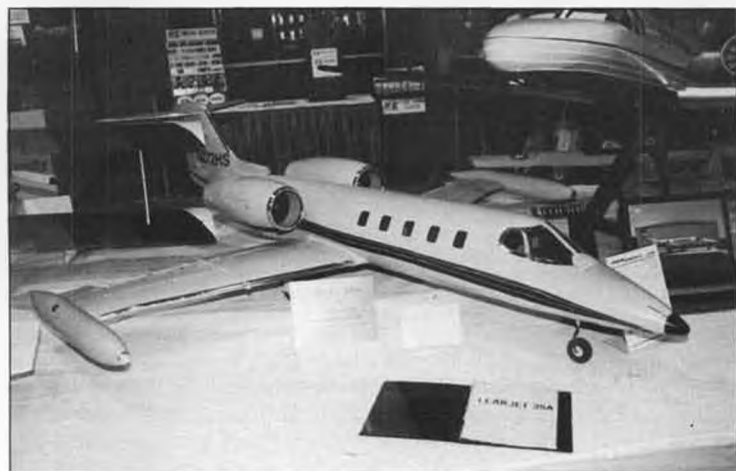
Charlie Lines used Mark Frankel plans to produce this attractive 1/6-scale Learjet 35A complete with flaps, retracts and spoilers. Power is two Rossi .65/Dynamax fan setups.
