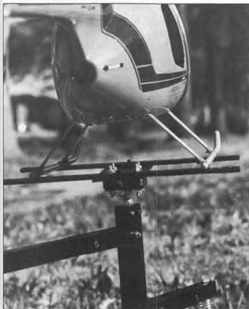
Here you can see that the supporting plate is mounted on four rubber dampers to allow the model to tilt. This is very important, otherwise, in order to move sideways, the rotor head will tilt too much and cause excessive stress on the hub.
