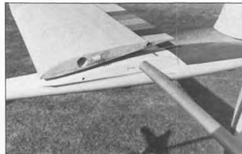
Jerry's Chameleon SE features easy-connect servo connectors built into fuselage and wing root. Note big diameter wing joiner tube, first seen in pattern ships.
