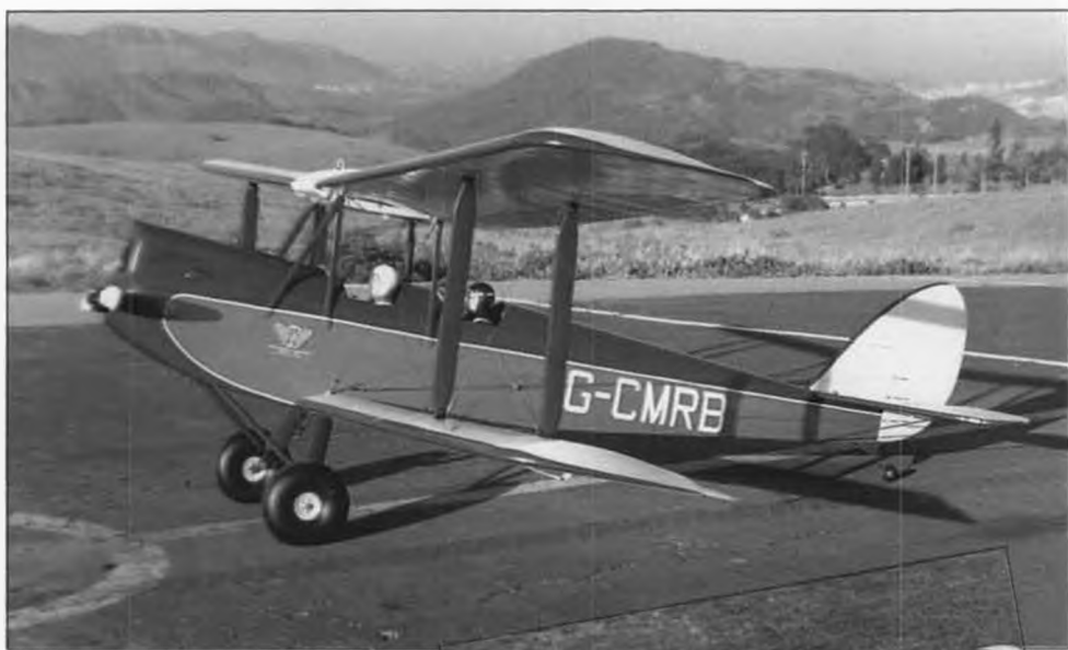
(Above) Fine example of a 1/4-scale Gipsy Moth built from the editor's plans (No.6771) by C.M. Reinisch, Thousand Oaks, California. Dry weight with O.S. 120 Surpass four-stroke is an ideal 16-1/2 pounds. Finish is Imron paint. Flies scale speed at one-third throttle, does honest loops and hammerhead stalls. Total flight trim amounted to three clicks of right rudder. (Right) Reinisch incorporated scale folding wings on his Moth. Note jury strut installed for folding, to keep wings in alignment. One-third scale plans now also available (No.2892).
