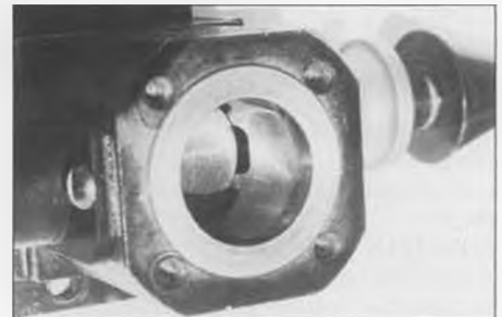
The glow plug gasket is the only gasket in the entire engine. Each MATAS engine is first run at the factory, which is why the combustion chamber area of the head is slightly darkened. Stu's engine has not been run since it left the factory.
