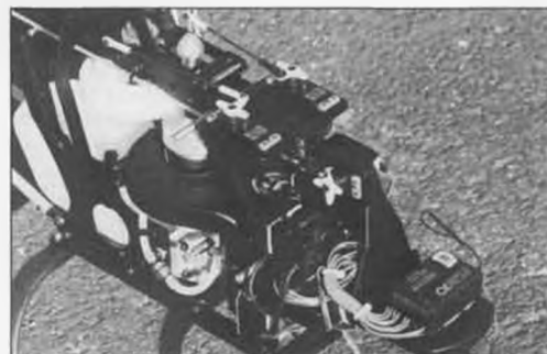
Servo tray is molded plastic, which really speeds up assembly. Note that our author has tied the servo wires together very neatly—he was not expecting to crash!
