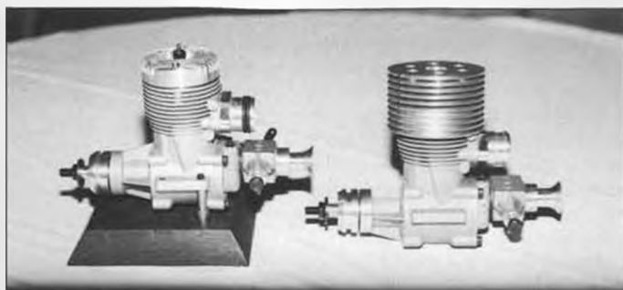
K&B's new .82 size ducted fan engine is offered with your choice of a regular head for tractor fans or a heat-sink head for pushers. Shaft extensions are included with both.
