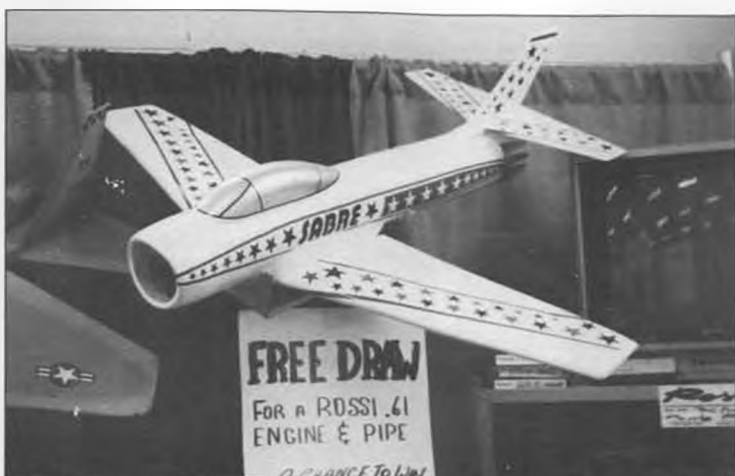
The ARF Sabre from Bob Parkinson is made of molded vinyl plastic. Bob claims it can be built in about eight hours.
