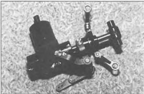
Beautiful workmanship is evident in this close-up of the tail rotor gearbox. Most model helicopters have the pitch control bellcrank fixed to the gearbox. The Excalibur's pitch control bellcrank sits on an arm that can pivot, which gives better kinematics for smooth pitch change action.
