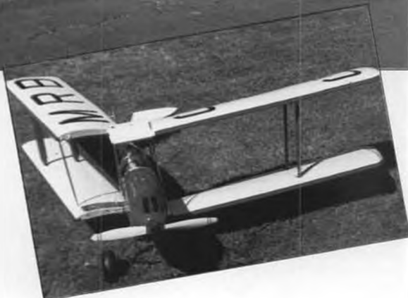
(Above) Fine example of a 1/4-scale Gipsy Moth built from the editor's plans (No.6771) by C.M. Reinisch, Thousand Oaks, California. Dry weight with O.S. 120 Surpass four-stroke is an ideal 16-1/2 pounds. Finish is Imron paint. Flies scale speed at one-third throttle, does honest loops and hammerhead stalls. Total flight trim amounted to three clicks of right rudder. (Right) Reinisch incorporated scale folding wings on his Moth. Note jury strut installed for folding, to keep wings in alignment. One-third scale plans now also available (No.2892).
