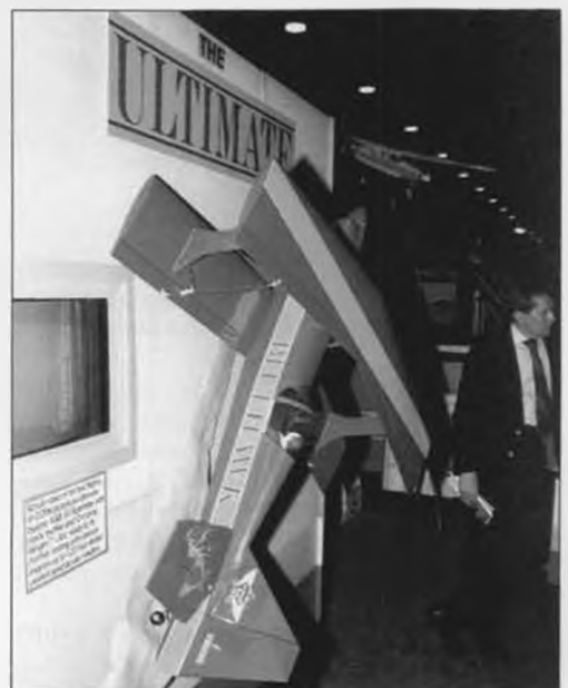
The new Ultimate 10-300 from Carl Goldberg Models, designed by Dave Patrick. Span 54 inches, area 980 sq.in., weight 7.5 - 8.5 lbs., power; .60 two-cycle. .90 - 1.20 four-cycle.
