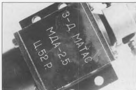
Engraving on the bottom of the crankcase gives the name, the displacement and the price: 52 Rubles, a very expensive engine by world standards!
