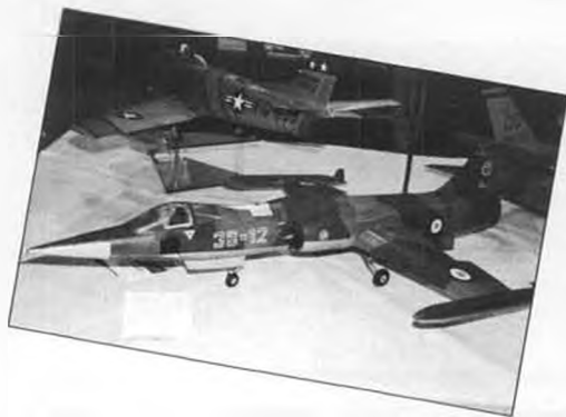
Pat DeFillippis and Aldo Guerrier teamed up on this impressive F-104 Starfighter, built from a Master Fly kit. Features a Rossi .81/Byrojet fan combo and operating slats and flaps.
