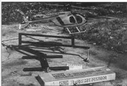
Century Import's 3-Dimension R/C Helicopter training stand can do away with a great deal of the grief (and expense) of learning to fly R/C helicopters. It allows the model to rise, yaw, and translate, and simulates free flight quite well.
