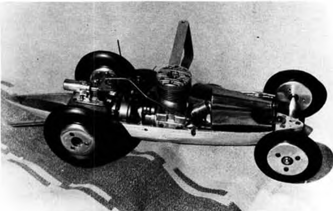
The author's 1234 car with big Dooling aboard. Note shut off switch lever sticking up. This is tripped with stick as car goes by.
