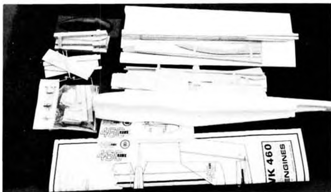
The Hawk 460 by World Engines features a combination of foam, plywood, and balsa construction. Span is 52 inches. For 19 to 40 engines
