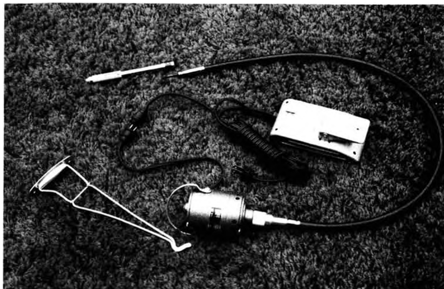
Pfingst flexible cable power tool being marketed by Brave Products. Drives 1/8 inch bits at speeds up to 14,000 rpm. High torque, 1/15 HP motor, foot controlled rheostat.
