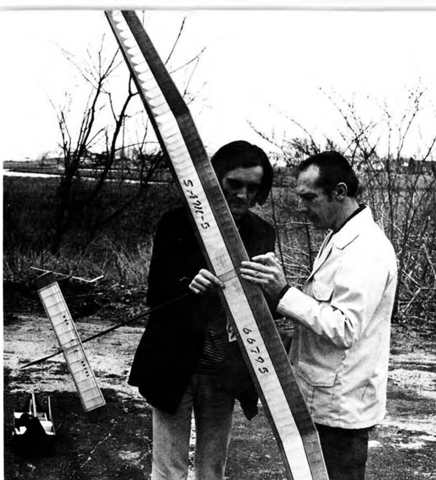
Author-designer Ron Evans (left) and Bob Lipori preparing SAM for a test flight. Glued on thread turbulators were used here but were not as effective as outrigger type shown on plans.
