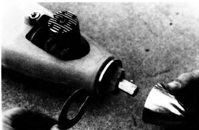
Use of 1/32 inch ply spacer assists in proper location of engine firewall. Ensures spinner clearance without excessive gap.
