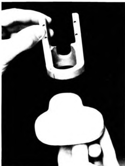
Fitting motor mount to ply firewall. Note the traced outline and location mark. CB mount.
