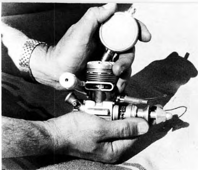
Timing a Dooling with a special fitting and a dial gauge. The timing light is hooked to the exhaust.
