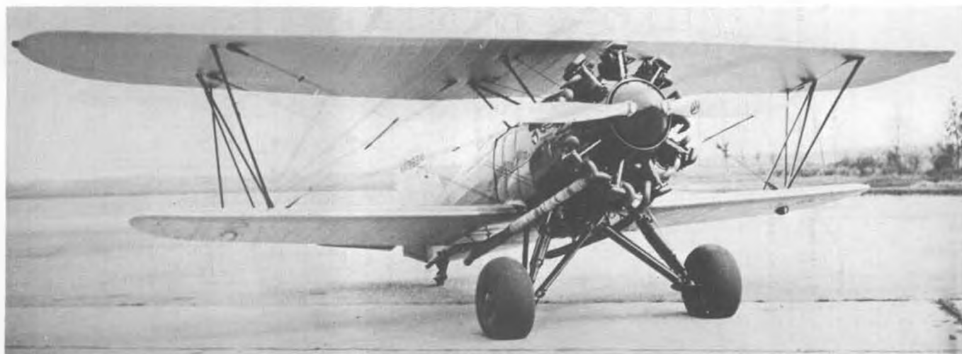
Originally known as the Hawk IA, Al Williams' Curtiss was basically an F6C-4 with a P-6 landing gear, fuselage saddle-bag gas tanks, and a Bliss modified Bristol Jupiter, 550 hp engine. Thrilled the spectators at the 1931 National Air Races in Cleveland.
