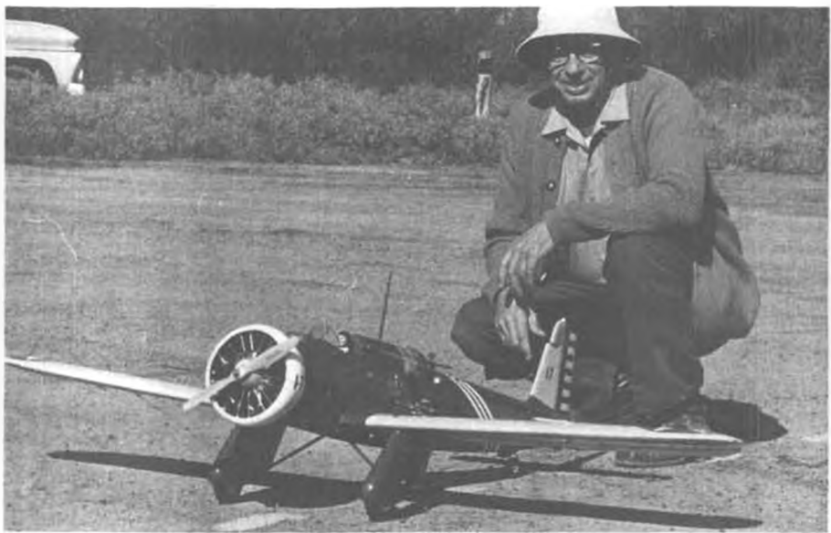
Charlie Smith and his dual purpose 'Shrike.' Note lead-out wires, and guide plate near left wing tip. Flying prop just about clears ring cowl. Radio gear remains aboard for U/C flights.
