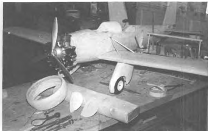
Remaining cylinders are attached to shaped balsa cowl. Engine is almost completely hidden. Balsa skin throughout.
