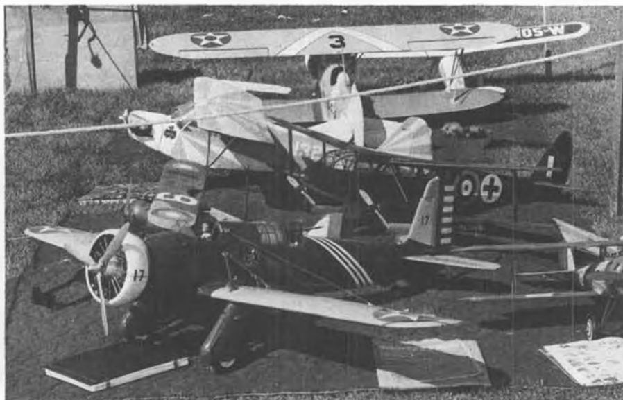
The 'Shrike' with some select company. Note Noel Hess' Boeing F4B-4 in background. Prototype Shrike was Army Air Corps' first all metal plane. Model has 66 inch wingspan.
