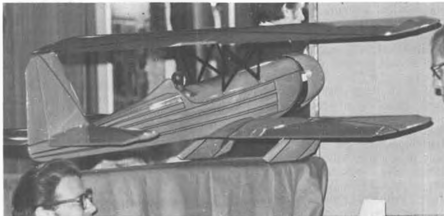
Elmer Good (lower left) is almost ready to release plastic, glass, and foam Big John kit after 2 years in the works. Weighs respectable 9-1/2 lbs ready to fly. Stringers molded into fuselage.
