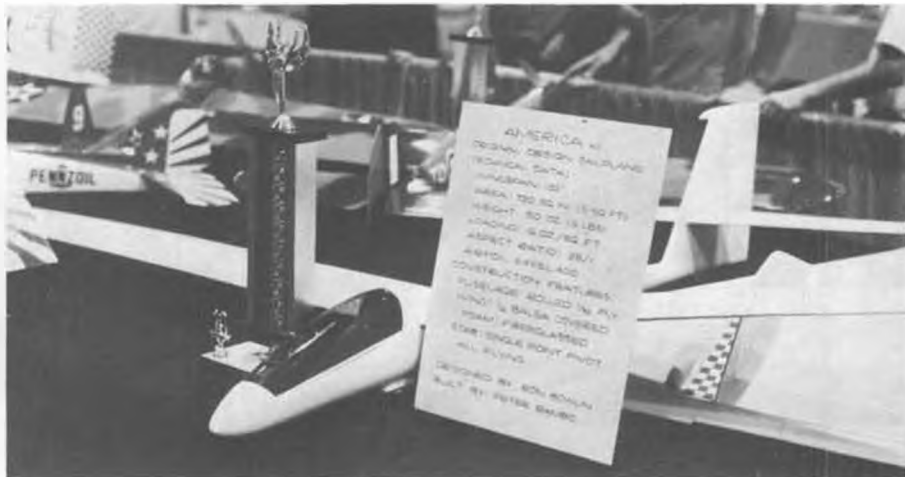
MAC Show prize winning sailplane design, "America", by Ron Bowlin and built by Peter Rambo. Features rolled 1/32 plywood fuselage and 1/16 balsa skinned foam wings. Span is 132 inches.
