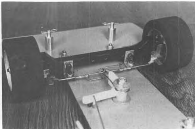
Associated-HRE steering override. Output spring wires can be bent to give soft center, slop, some spring rate or preload change. Fig. 3
