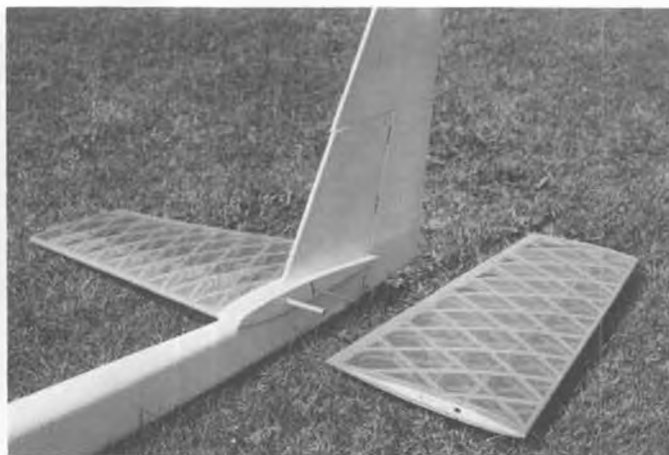
Plug-in flying stab on 'Leo' spans 36 inches, features light and strong geodetic construction. Note aerodynamic balanced rudder.
