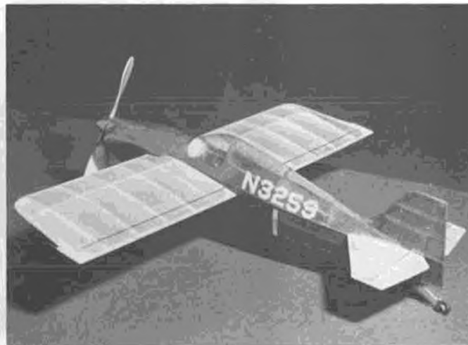
Only deviations from scale are a slight increase in stab area and an 1/8th inch of dihedral added to the otherwise flat wing.
