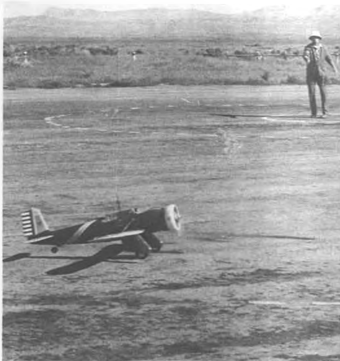
Charlie starts a takeoff. Note the right main and tail wheels are off the ground. Rudder and ailerons trimmed right for U/C.
