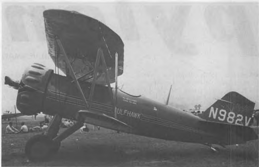
As restored by Frank Tallman, the Gulfhawk had P & W Wasp and other parts from an SNJ. Note one grooved, one diamond treaded tire.
