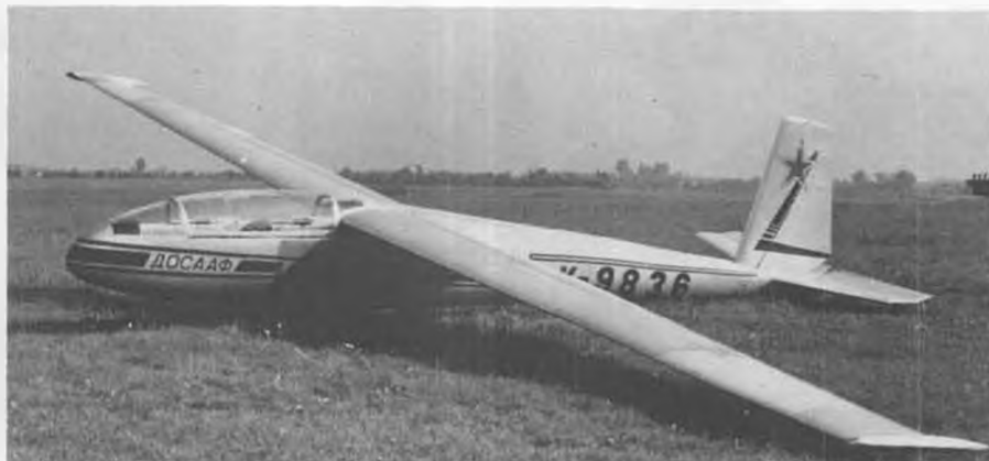
Stabilizer has just enough dihedral to clear the ground when the ship is heeled over. Good thinking! Semi-retracted wheel should simplify modeling problems. Note tip "tanks."
