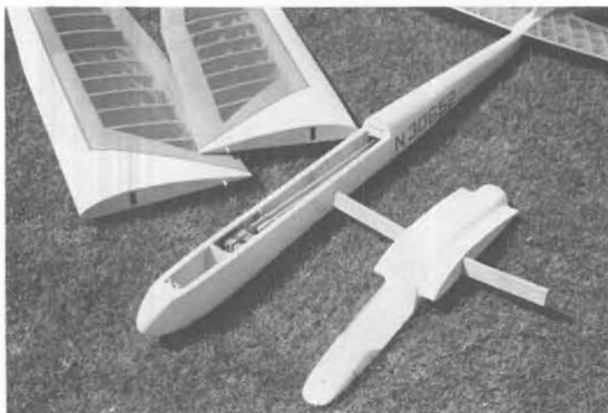
Huge maple tongue is imbedded in removable fuselage top section. Pushrod dowels are spliced. Radio area like Grand Central Station!
