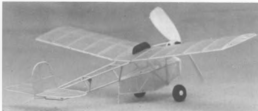
The condenser paper covered indoor model almost disappears into the background. High thrust line allows generous size propeller.
