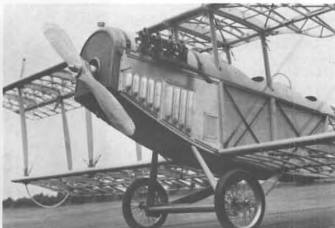
Best thing to do with this job is cover it with clear mylar to keep out the dust then build another one to fly. Note routed spars!
