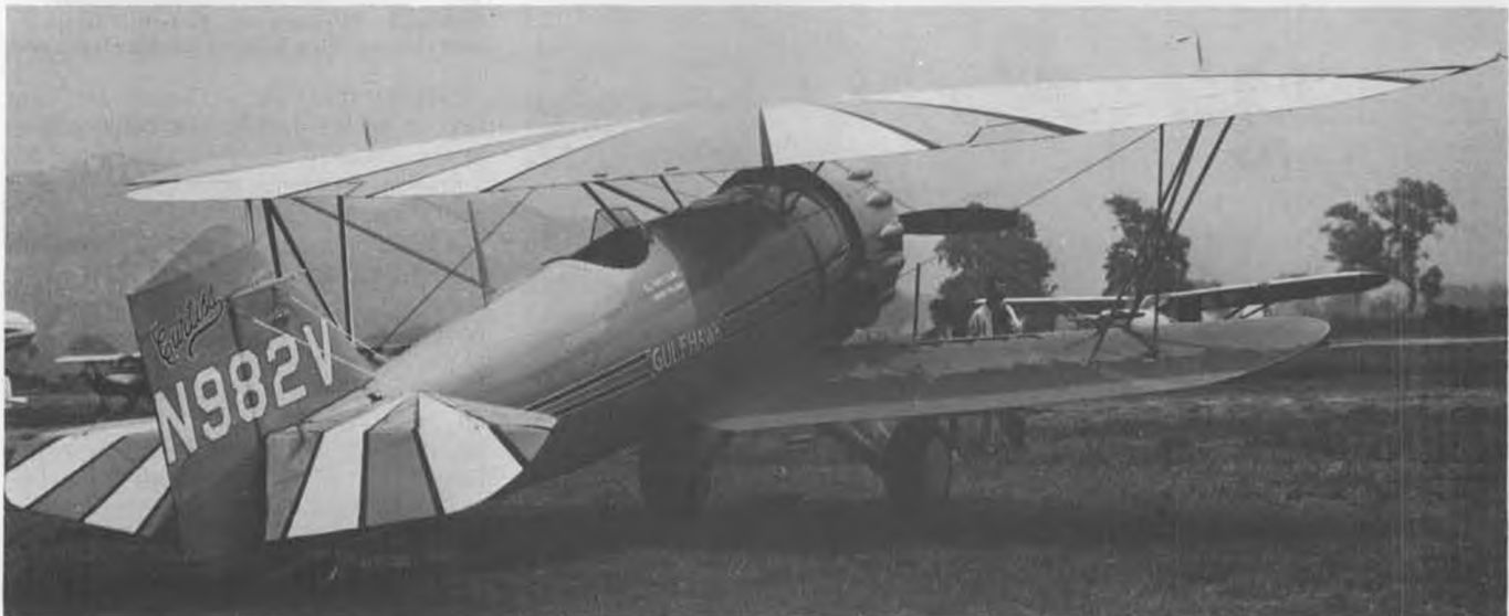
Big cowl and barrel fuselage limited ground visibility. Large tail surfaces great for stunts, but small ailerons made rolling maneuvers a bit mushy.
