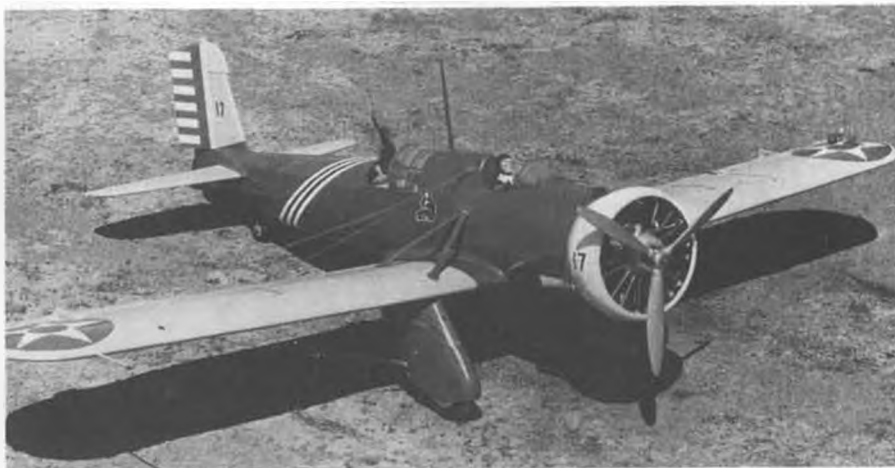
All rigging is permanently attached to the wing, unbolts at fuselage when broken down for transporting. Right trim is put in by radio before ukie flights. Roberts control for U/C.
