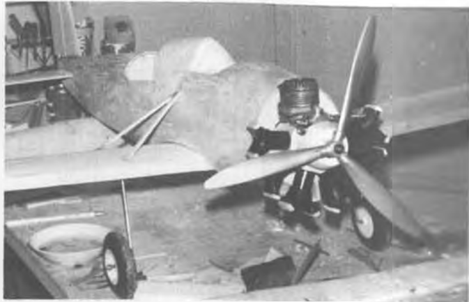
Dummy engine is entirely built up from scratch (Sorry about that, Williams Bros! At least he used your wheels). Webra 60 R/C engine.
