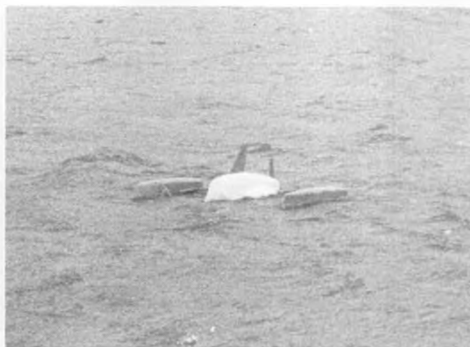
hulls yaw to port, decelerate, bury, and trip over starboard outrigger. Finally, "Stable II" is attained. No damage, no water inside. See text.
