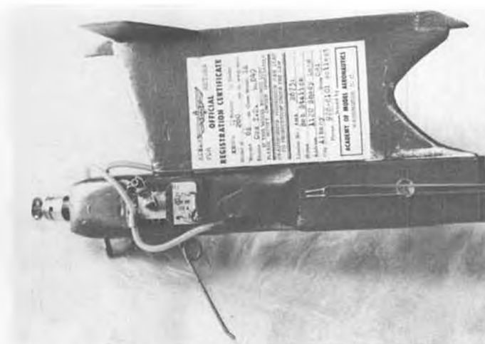
"Other" side of Fast Rod, showing timer installation and wing mount.
