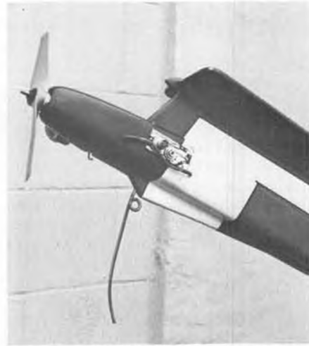
Engine side of Hal Woods' cowed version. Final version has shorter fore and aft moments.
