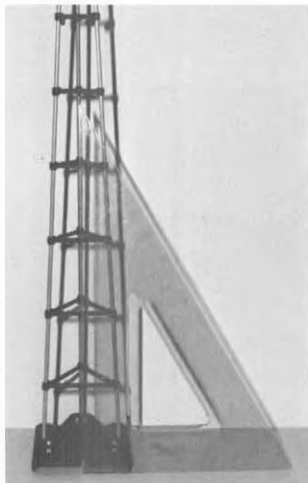
No, it's not an oil derrick! Proper alignment is important for free running tail rotor drive shaft.
