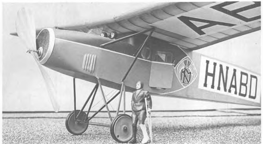
Close-up of Fokker reveals double-truck wheels, also "laminated" Peck-Polymers propeller. Radiator is brass filter screen, struts are hollow 3-ply Strathmore paper. Pilot is former skier!
