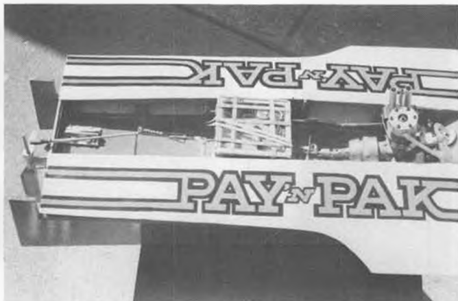
Radio box installation. Location is far forward for good C.G. Belly pan allows engine to be lowered, giving room for moving radio ahead.
