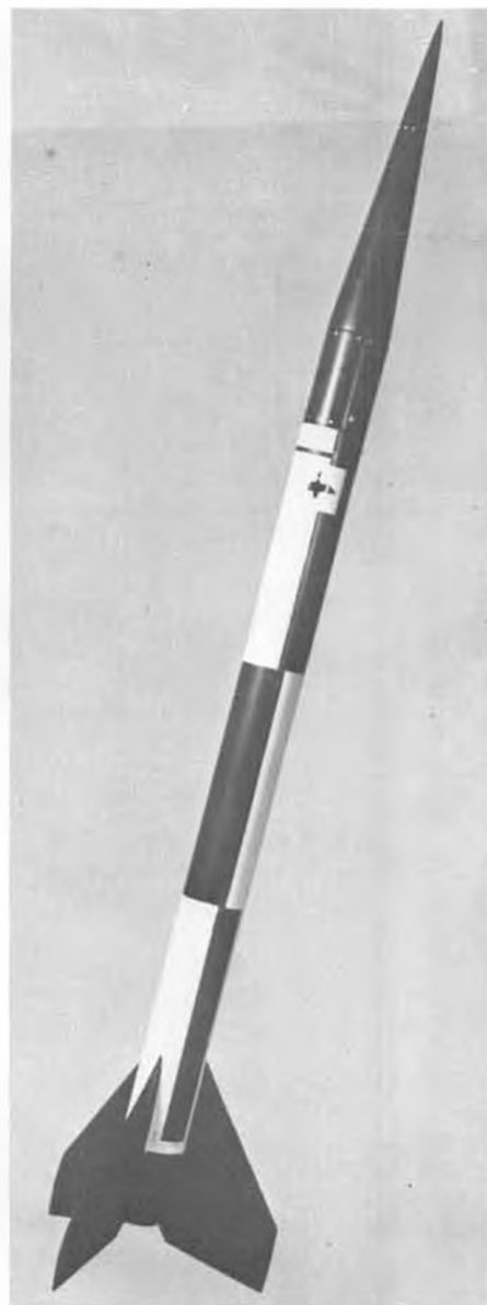
FSI scale Black Brant II kit, in Canadian color pattern. Flies with F100 Loadlifter engines, as used in model of Goddard's rocket for NASA.
