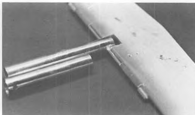
Stabilator hinge is silver soldered to end of inner boom tube. Everything on the plane can be replaced or scavenged, handy in combat!
