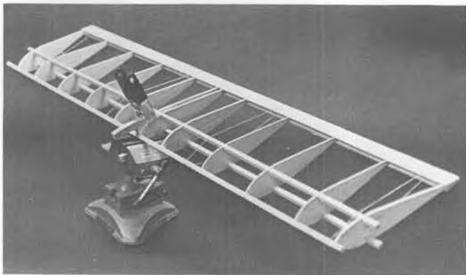
With airframe mounted in a vise, both hands are free to twist any stubborn worps out of it. Rubber bands hold LE while glue sets up.
