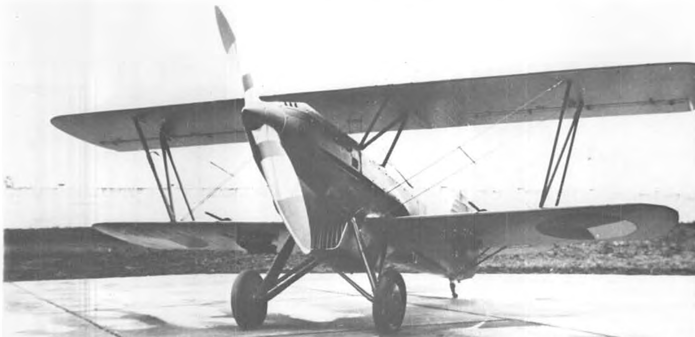
A Series I B-534, very similar to the Series II in the drawings, with two guns in the fuselage and two in the wings. Note huge wood prop made of twelve laminations.
