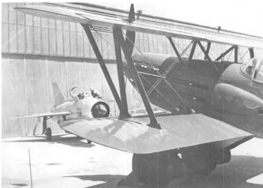
Powered by a 750 hp Hisso, the Avia B-534 was fast and tough. It fought well into WW II, and even tried to tackle some USAAF B-24's! Blister on fuselage covers machine gun breeches.
