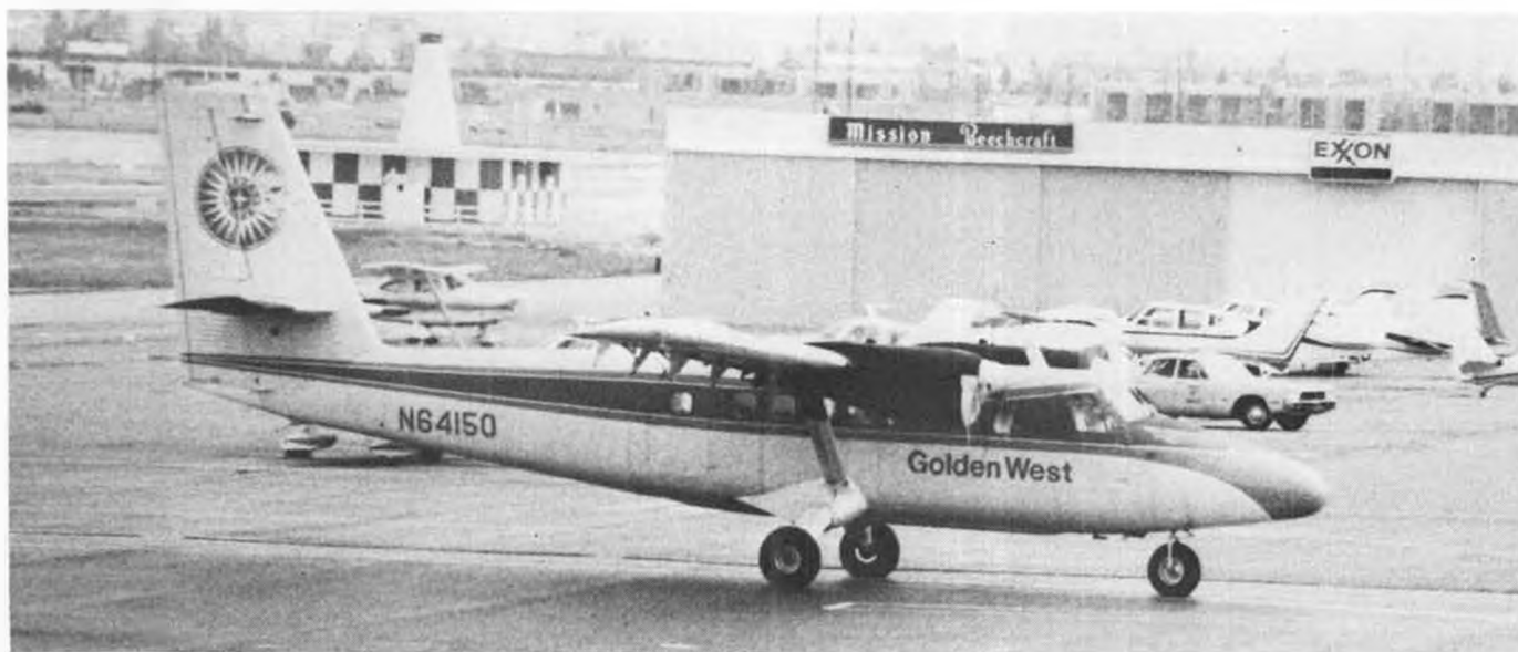
Generous fin and rudder area, ample dihedral, and fixed landing gear, make the Twin Otter an ideal subject for sport or museum scale. Original model flew well on two OS .30's, keeping it within the .61 limit still maintained on scale in the FAI rules.
