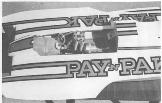
Installation of K&B .40 engine and Sullivan 8 oz. fuel tank. Most of the running hardware is as recommended by Dumas.
