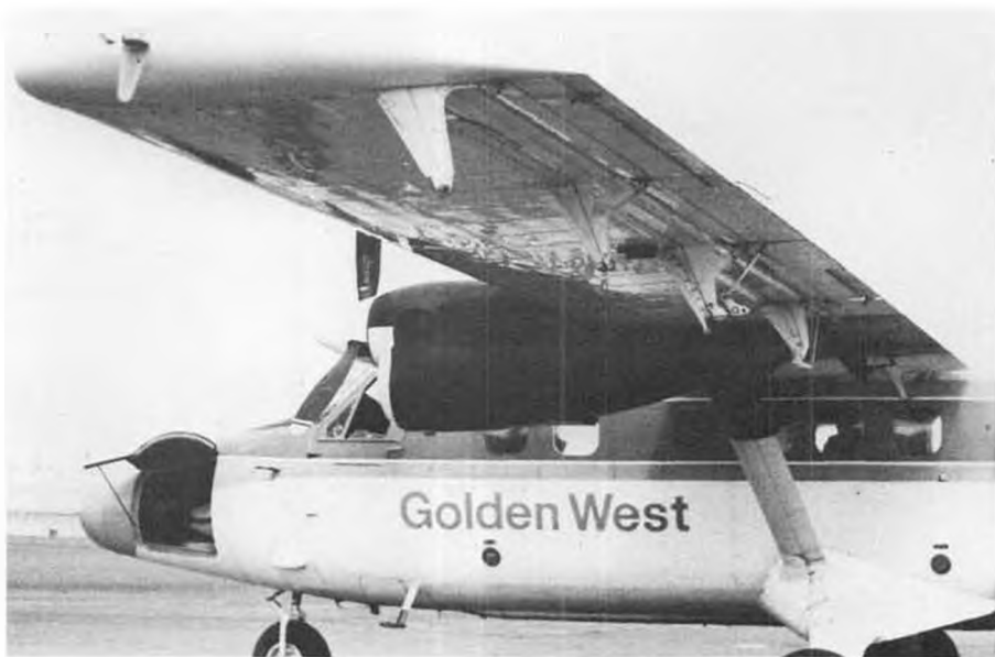
Complicated hinging mechanism provides for a Fowler flap effect on the ailerons, even as they are being used for baggage . . . or ballast, in a model!
