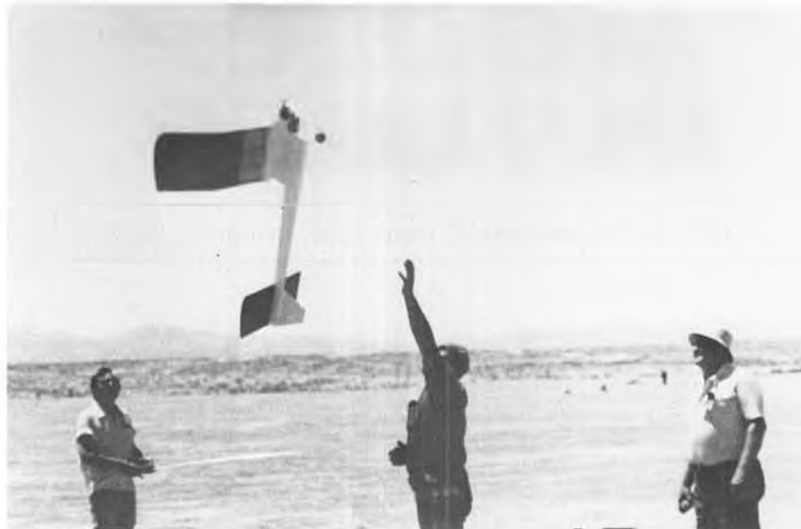
The moment of truth! Sal Taibi launches our K&B .40 powered 900 Starduster on its first flight. That's right, we're holding our Signature Series Kraft transmitter. The completely hidden R/C system consists of rudder tab and trimmable stab platform. Engine's on Tatone timer, no throttle control. See text for more info. Woody Petersen watches, and if we remember correctly, we handed our Nikon to Tim Anderson, from North Carolina, to shoot photo at '76 NFFC, Taft, Ca.
