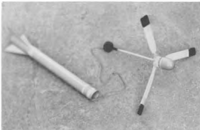
Kopter kit, showing the ejectable rotor unit. Rotor spins free on a shaft between nose cone and end plug. No wadding needed. See text.
