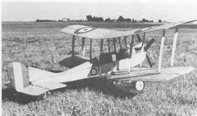
BE-2c powered by Mills 1.3 diesel, built by Dee Mathews, Greensburg, Kansas. Drawings from "Fighter Aircraft of 1914-1918 War."
