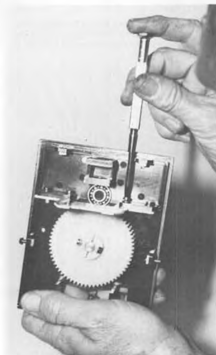
Assembly of the main transmission is very systematic. The main considerations are free movement and proper alignment.
