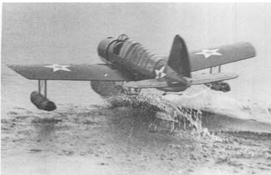
Main float is just about to come out of its plowing attitude as ship gains speed. Note that although right rudder has been applied, the left float is still out of the water. Lotsa action!
