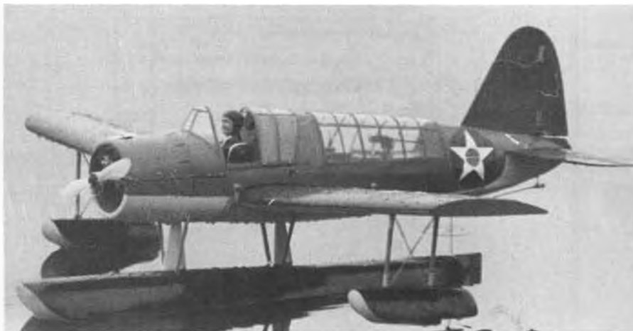
The author's model of the "Kingfisher" is extremely easy to fly and very stable in the air. Out-board floats will "knock off" if necessary. Note rubber bands holding main float in position.
