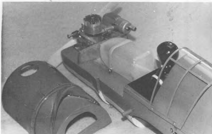
Pilot has excellent view of fuel tank with cowl/hatch removed! Excellent accessibility for work on engine, throttle, tank, etc.
