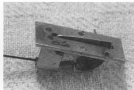
Switch in locked position.
