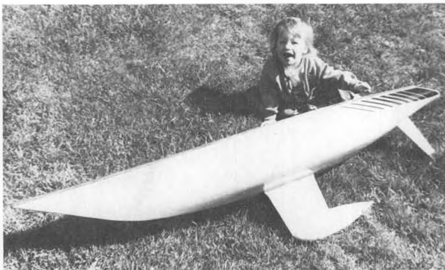
Tracey Carr, the author's 2-year old daughter, points out the nifty striping job on Pop's big yellow creation that borrowed her name. Hull is pine planking over frames, glass cloth inside.
