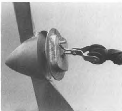
Bobbin and rubber tensioner latch show up well in this close-in photo. Wind without prop.
