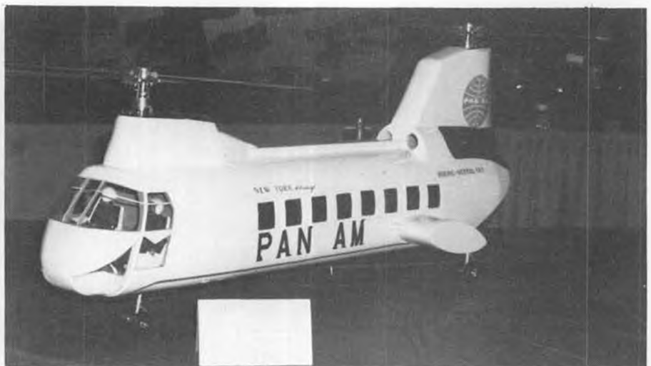
Twin rotor Boeing Vertol 101, built by Horst Nietzel, Cypress, California. Ship is 6 feet long, weighs 13 pounds, and is powered by a single .60 engine. Building time was 700 hours.
