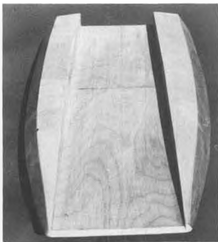
Bottom view of the tunnel hull. Boat rides on inner corners of sponsons, which must be kept sharp for directional control.
