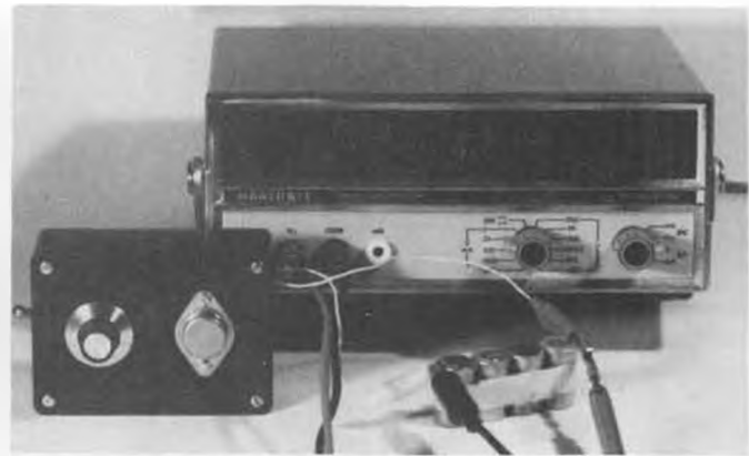
Testing battery voltage under load. See text for instructions on how to build the variable loader.
