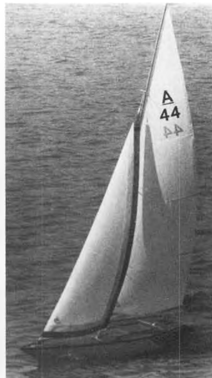
The author's "A" Class "TRACER", weighs 39.8 lbs, carries 1600 sq. in. of sail.
