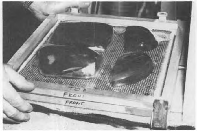
Finished "Baby Ranger" windows about ready to come out of the vacuum molder.
