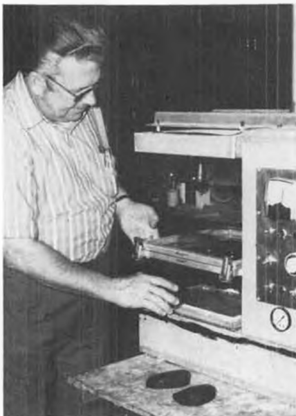
Charlie removing molding plugs from tray. Windows are still in the frame.
