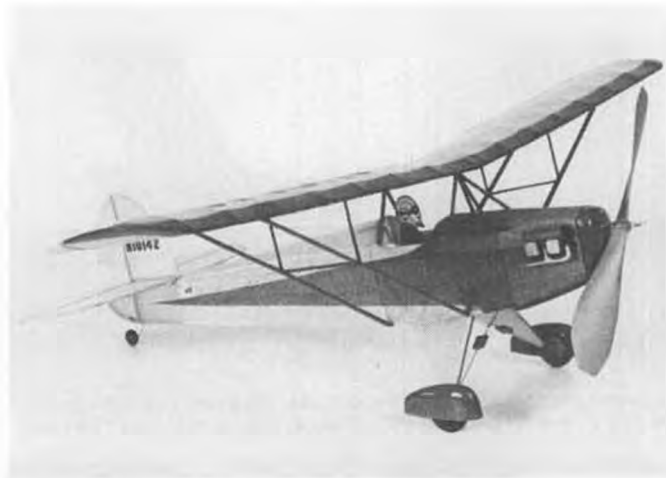
Walnut Scale "Baby Ace" by Peck-Polymers spans 17-1/2 inches, for rubber or CO 2 power. First of a series.
