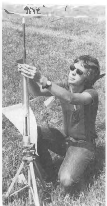
Mike Micci connects altitude entry to his advanced piston launcher, which is enclosed in clear tube and mounted on tripod.
