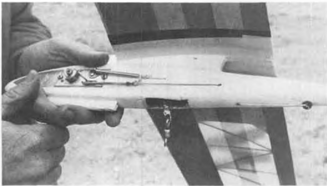
business end of Don Zink's "Wishbone". Twanger system uses a plunger to actuate rudder for zoom launch.
