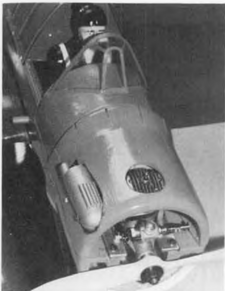
Though cowed, there is still plenty of room for cooling air to circulate around engine.
