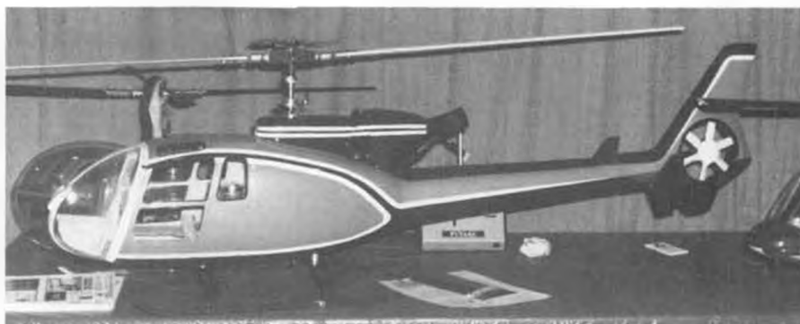
The new "Gazelle" helicopter to be available soon from American R/C Helicopters. Note "Fenestron" tail rotor.
