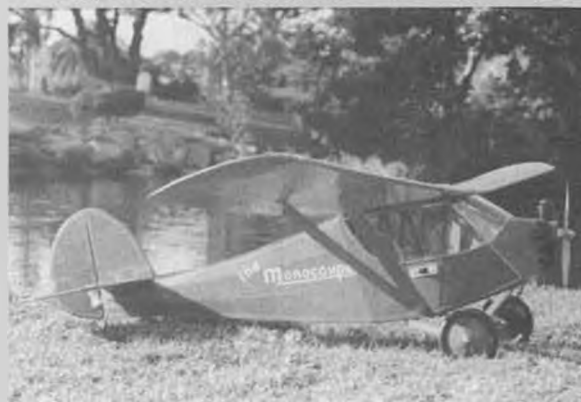
Wing span 49 inches, weight area 338 sq. inches, 2 or 3 channel radio, 049 glow or 05 electric.
