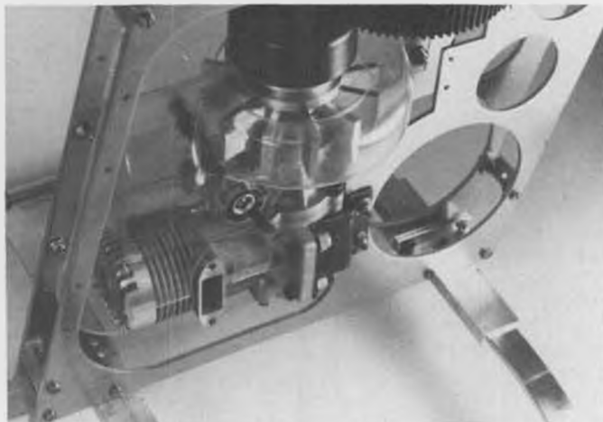
Clutch and gear assembly with transparent cooling fan housing, not yet painted.
