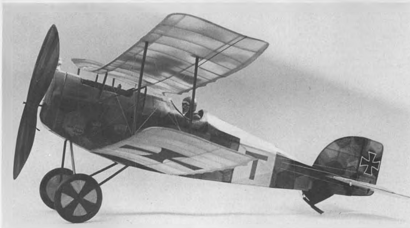
Another goodie by Bill Noonan. This time it's a one-inch scale Aviatik (Berg) D-1, built for the Flightmaster's Semi-Annual special WW-I rubber event. Span is 26 inches. The scale aileron washout and large tail surfaces should really enhance flight trim.
