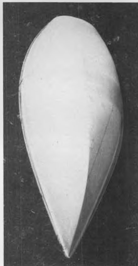
Good planing hull form for heavy air, in this model of the Olympic class boat.
