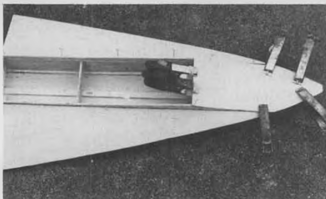
The top deck section is held in place with clamps. Don't try to apply decking without these extra "hands".
