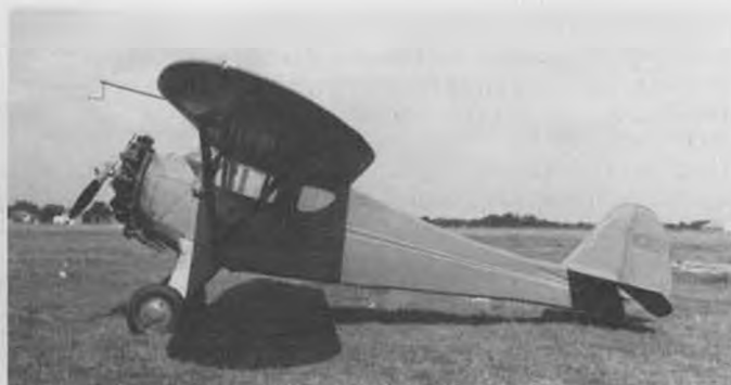
Model 110 powered by 110 hp Warner Scarab. Basic Model 90 airframe, but with single leg gear, braced with wires, shocks in fuselage.
