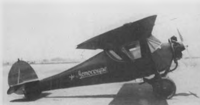
Model 113, so-named from ATC number, like earlier Model 1, but with Velie M-5 instead of Detroit Air-Cat engine. Top of 98 mph.
