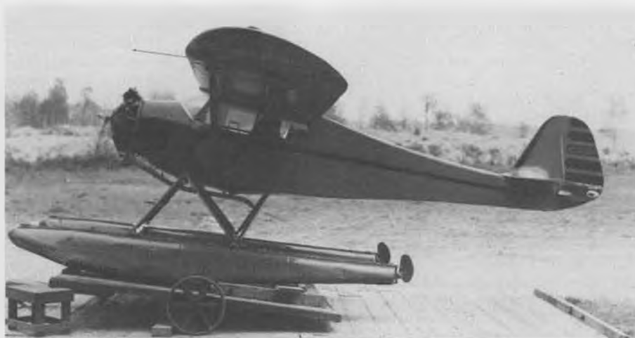
Seattle based Monocoupe 90 on Edo floats. Light area at base of fin is reflection from natural fabric fillet.
