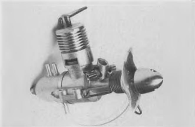
D-C Super Merlin .047 swings an 8 x 4 prop! That spring starter is the secret, for all you non-diesel persons.
