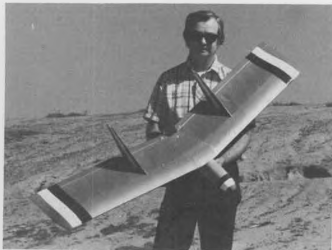
Cecil has modified the Little Plank by adding sweepback and twin fins. Ship doesn't stall, but "porpoises" when it needs downstick.
