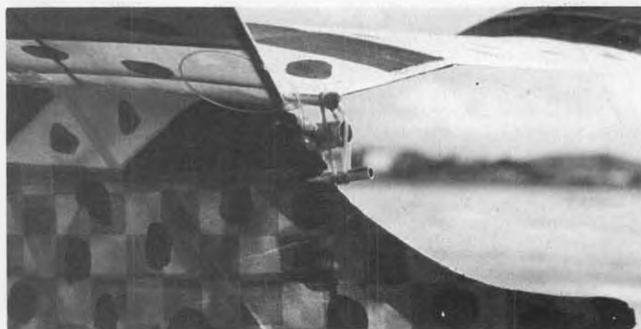
Close-up of stab DT rigging. Note that aft end of fuselage is pulled together into a triangle section which blends neatly into the skid/sub-fin.
