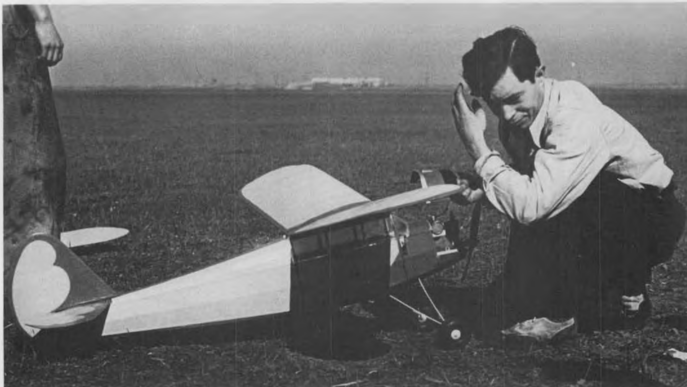
Now how does that cowl go back on? Leon Bazurto at Moffet NAS, in 1937, with TD Coupe (MB Plan No. 574-O.T., $3.50). Note original wood motor mount, as sold with Baby Cyclone. Tank seems to be raised above normal position.
