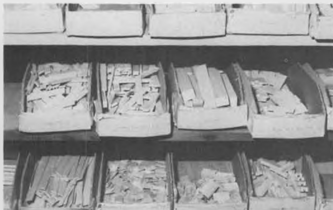
Parts are accumulated in sorting boxes, ready for transfer to kit boxes. These are wing tips, servo mounts, landing gear blocks, etc.
