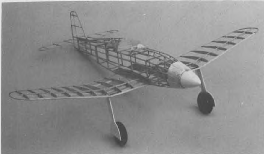
Fernando's only modification to the original Heinkel was in the use of laminated basswood for the outlines of the tail surfaces and wing.
