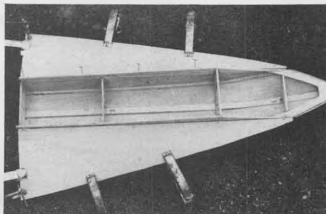
After motor mount is fitted, the deck siding can be applied.
