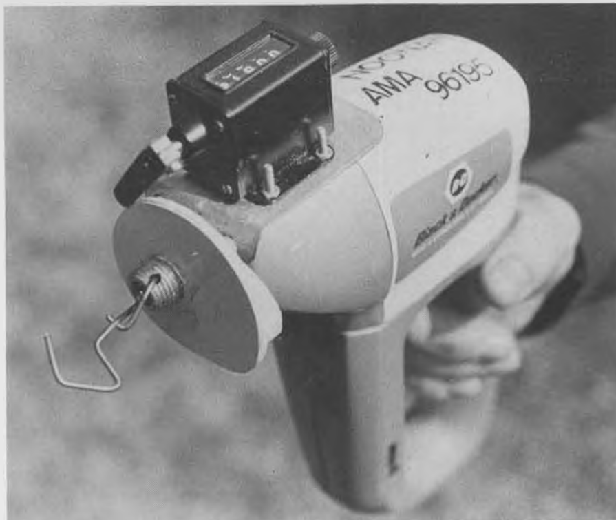
Black & Decker 9000 cordless drill. Handle is battery unit. Cam-activated mechanical stroke counter is mounted on drill. Reset knob visible at rear of counter. Exploded sketch of part
