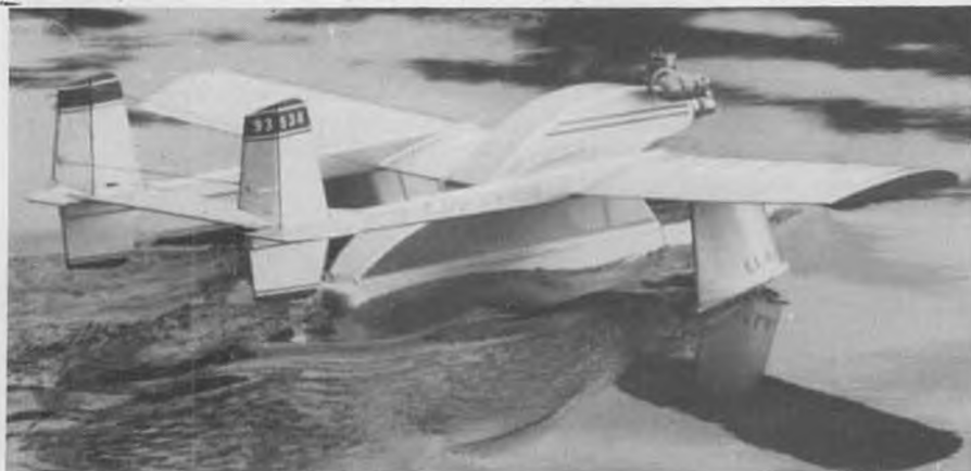
Gee Bee Line's "Islander" taxiing out for takeoff. Built by Dick Calderigi, it is powered by and Enya 40. Seaplane's hull is a Gee Bee float.
