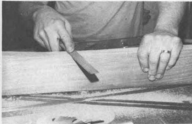
Line up both sides on flat surface and file even.
