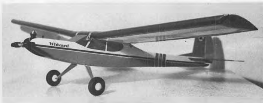
Ace R/C's "Whizard" is a nifty trainer. Designed for pulse rudder control, but it can handle up to three channels.
