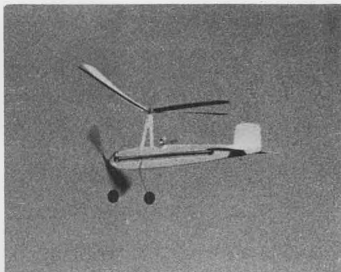
Modified Tyro-Gyro, built by Warren Shipp, in flight. Model descends vertically in autorotation, in the manner of a parachute.
