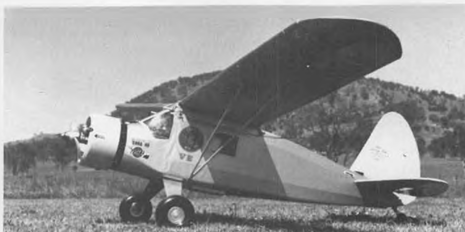
Monty Terrel's Dennyplane photographed against Australian background. Plane is equipped with Futaba radio and powered by a Webra 40 engine.
