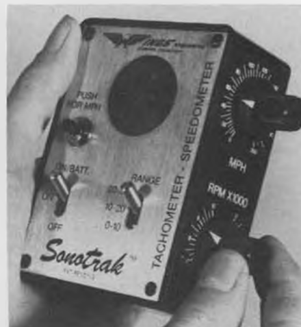
Sonotrak picks up RPM's in the air, and also figures speed of aircraft.
