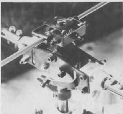
Main rotor head, less pushrods. Pitch arm has single ball installed for slow response version.
