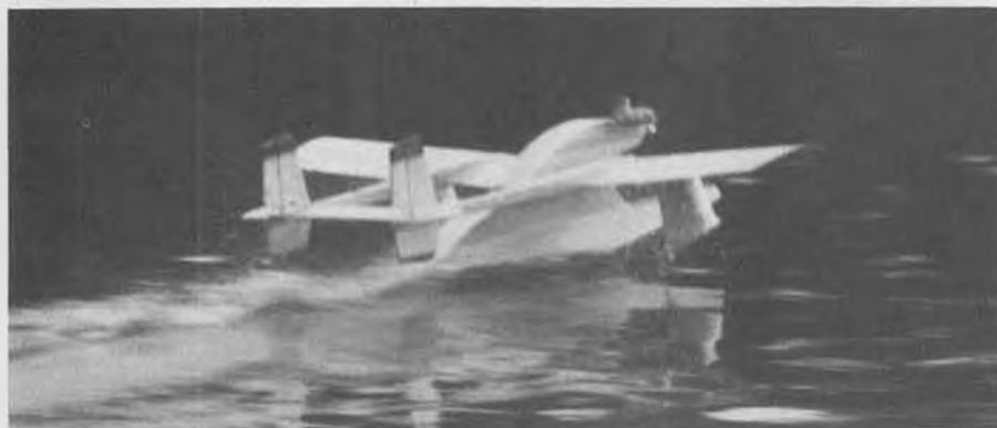
The "Islander" on a takeoff run. Note that tip floats are out of the water, and model is in perfect takeoff attitude. Just a little more flying speed . . .
