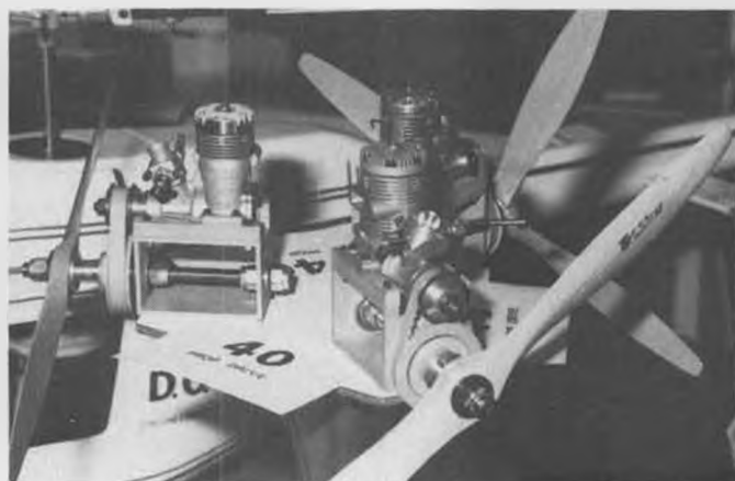
D.C. Engineering's 40-size belt prop drive.
