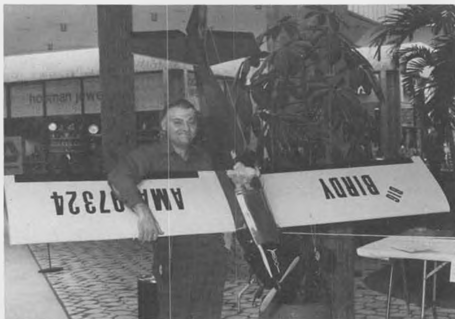
Don Jetter, Elkhart, Indiana, and his 23 pound, fully aerobatic, 1440 sq. in. model. Has smoke provision, foam wing, Heath radio, and 12 flights logged when the photo was taken.
