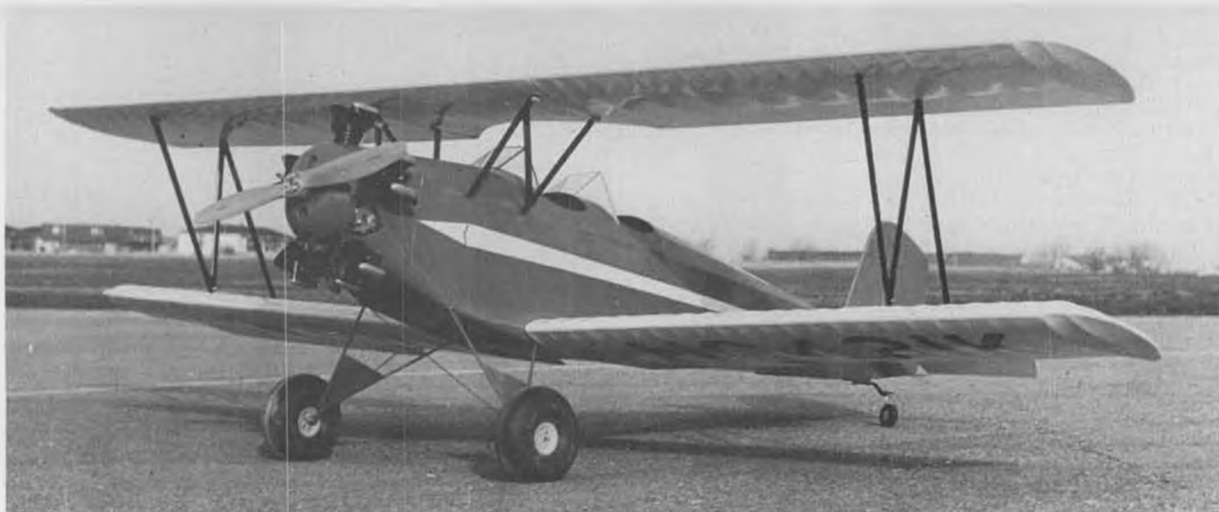
Quarter-scale Fleet Model 2, from the latest Concept Models kit (Box 7335, Madison, Wisc. 53711). Span is 7 feet, 1 inch, and it is designed around the Quadra engine. When you see the amount of strip-wood and the carefully machine-cut parts, the price of $179.95 is very reasonable.
