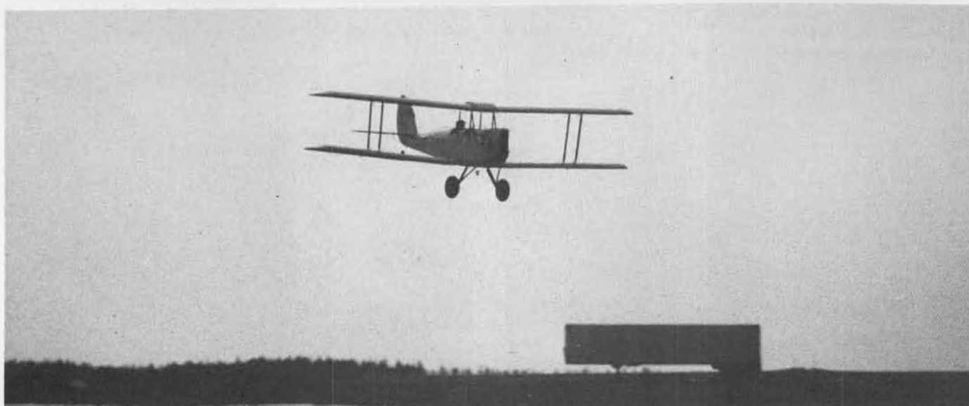
A Gipsy Moth on one of its maiden flights, in Nova Scotia. Built by Arie Hakkert, the Moth weighs 19 pounds, and is powered by a Quadra. A Kraft 5-channel Bi-Centennial radio works without interference from the ignition. Takeoff is as half-throttle, while cruising is at 1/3.
