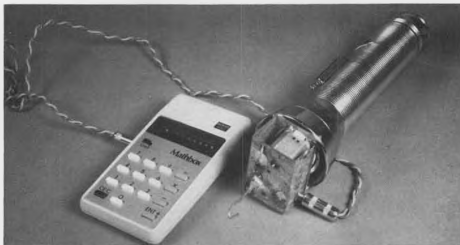
Electric winder developed by Joe Carter. A magnetic reed switch mounted on the winder picks up the count and transfers it to the inexpensive calculator.
