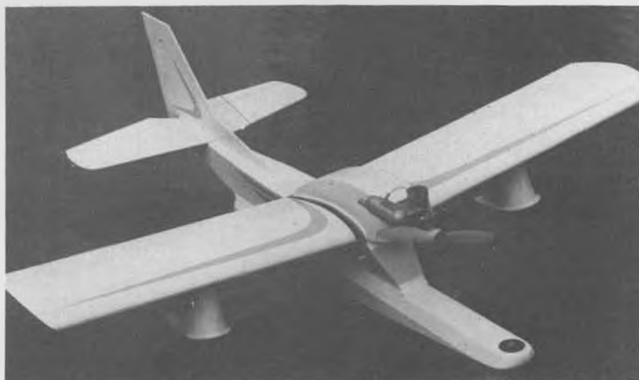
Gee Bee Line's "Mallard", again based on a single Gee Bee float. Power is an OS .30.
