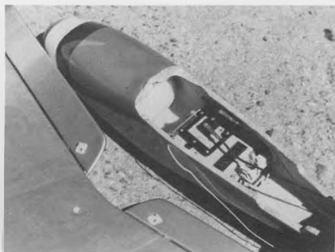
Plank uses a Kraft brick with mixer mounted directly on top, providing elevon control without sliding tray.
