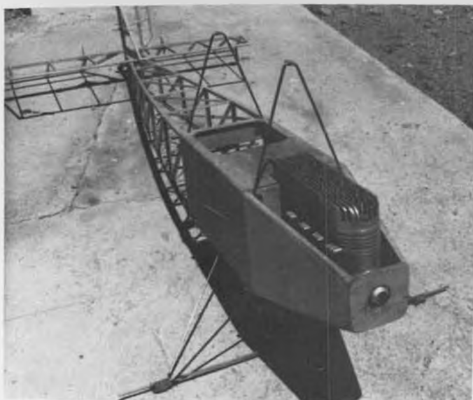
Unusual O.T. flying scale by Gordon Coddling. A Storms "Flying Flivver" with Evans Four, using Brown pistons and Cyke porting.
