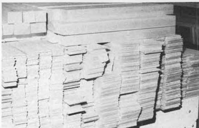
Sheet wood, after it has been cut, planed, and sanded, ready for die-cutting.
