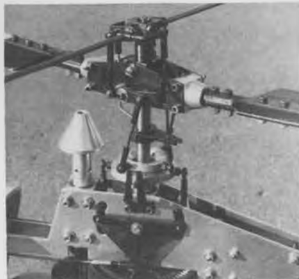
Main rotor head with pushrods. Pitch arm has mixing levers added for fast response version.
