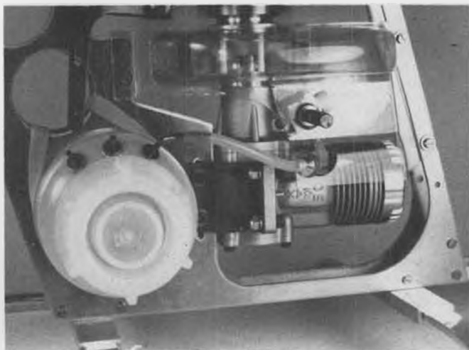
Mounting of engine and fuel tank in Schluter Heli-Boy. Tank is held in place by giant rubber band. Fuel line filter recommended.
