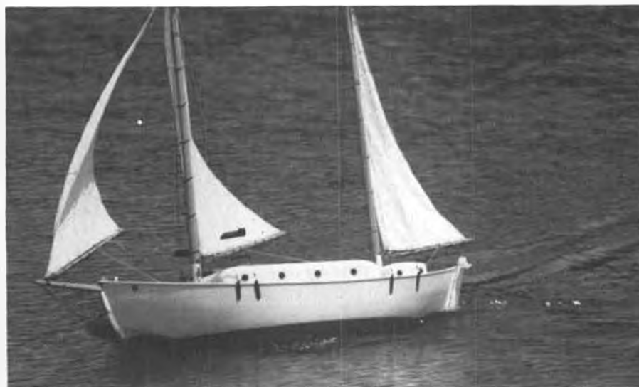
In a fairly strong breeze, "Mara" heels gently and really knifes through the water. Note bow wave, plus good hull wave form which keeps rudder well submerged for positive steering.
