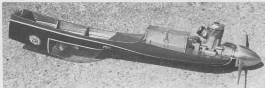
Removable engine pod allows complete power plant checks, even between heats. Radio system also becomes quickly accessible, making for easy maintenance.
