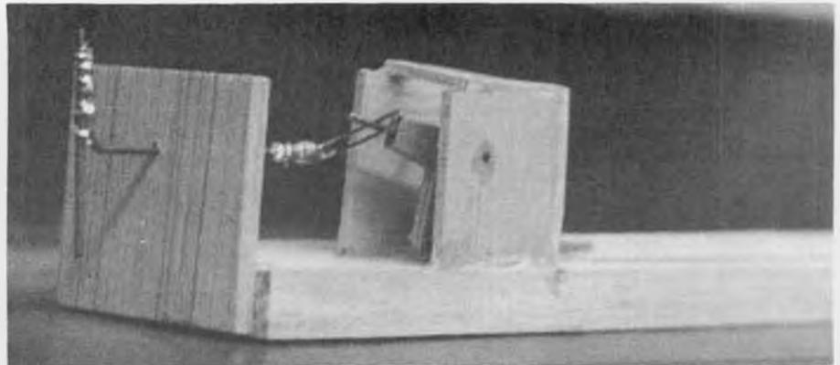
Motor end of Norm Beattie's torque-actuated Variable Incidence Tail system for Wakefields. Motor torque twists wire, provides motion to stab trailing edge.
