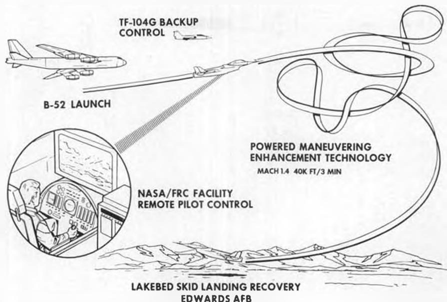
per hour and 6-g turns at 800 miles per hour at 30,000 ft. altitude. The flight tests can last up to an hour. Once the mission is over, the HiMAT will use skid type landing gear to land on the dry lakebed at Edwards Air Force Base, California.
