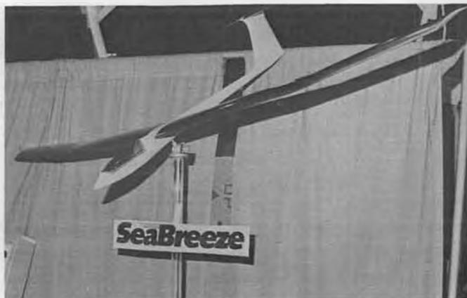
Sea Breeze is ready-to-fly (less radio installation) sailplane by Bob Smith R/C Aircraft. Fuse, wings, stab, all molded epoxy-glass.
