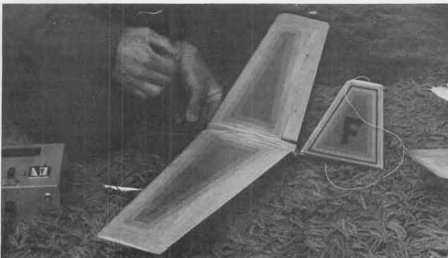
Alan Nelson's 12-ounce flying wing is a real performer. Wing is solid balsa, fuselage is glass reinforced with carbon fibers. Can you imagine what the control response must be like? Fast!
