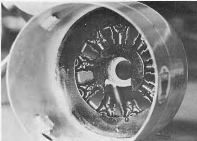
Williams Bros. engine first glued to small ply ring, then glued into cowl, followed by outside ply ring which holds all in place.
