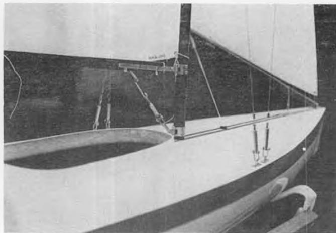
Boom Vang arrangement is strong, easily adjustable, and can be assembled from commercially available parts.
