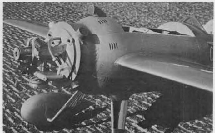
Engine plumbing. Pump and exhaust pressure are employed. Plywood knobs are cowl mounting stubs.
