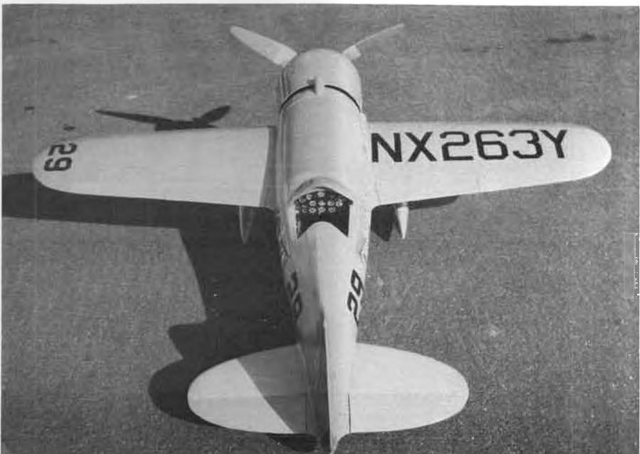
The scale outline has not been changed. As text reveals, original ship started with smaller, straight wing which would have been inadequate. Col. Bob is thankful for change!
