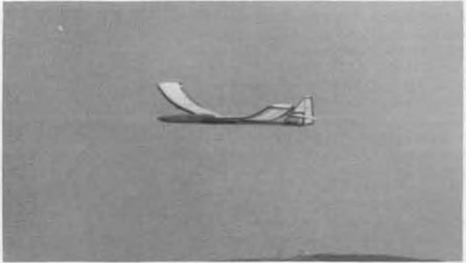
The Westwind II spans 75-1/2 inches, weighs 40 ounces without ballast. Note the very low fuselage profile.
