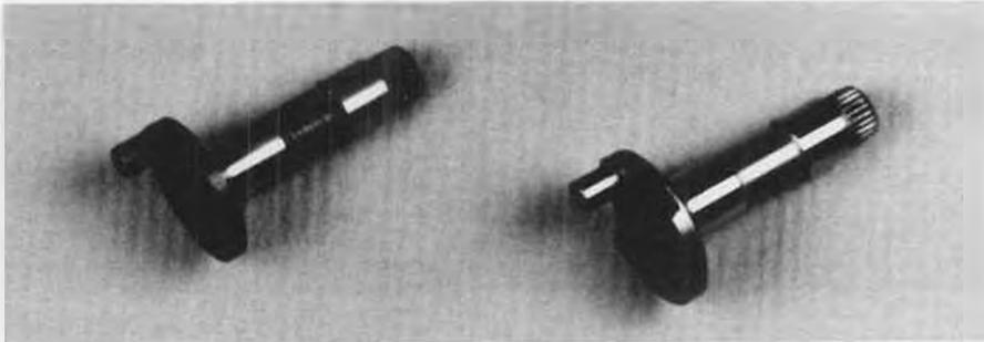
On the left, a heavy-duty crankshaft. On the right, a stock one. Note the difference in web thickness. Stock cranks sometimes break when used with high nitro fuel.
