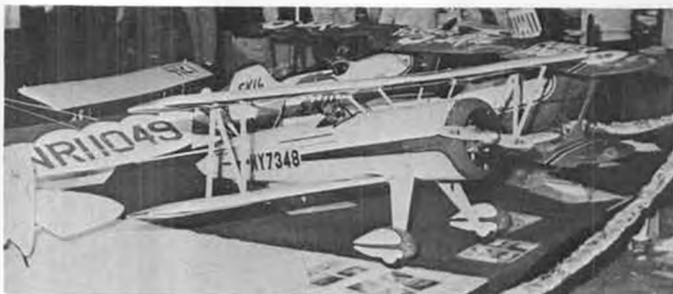
Quarter-scale Stearman designed and built by Don Godfrey. Span is 86 inches, weight 21 lbs., Quadra power, Zinger 20 x 8 prop.
