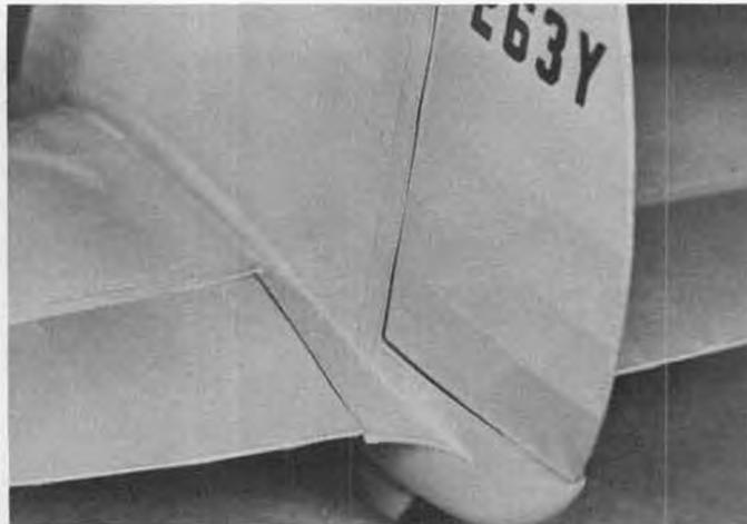
Gap fillers on control surfaces are made of tape used in Dymo Label Makers. The colonel describes two techniques in the text.
