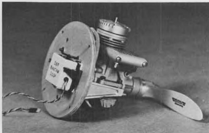
How's this for a servo vibration test? K&B 61 runs inverted. Note big chunk of lead banded to engine mount.
