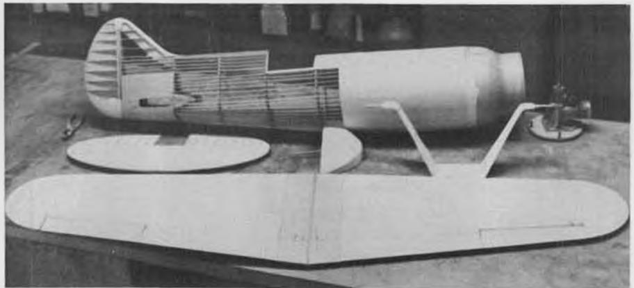
Some of the basic parts prior to the model becoming a one-piece aircraft. Wing is foam cored and cowl is fiberglass. The rest is cut wood and glue!
