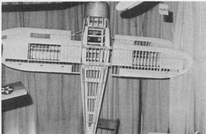
Latest kit from M.E.N., masters at lightweight plywood die-cutting, is this 1/4-scale Beech Staggerwing. Spun aluminum cowl.
