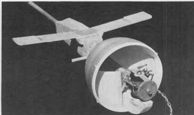
Two views of the completed nose section with the Ace Baby Twin actuator mounted in place. Receiver and battery are wrapped in foam rubber, then packed into the egg. Note the 1/8 sheet frames which support the rear half of the egg shell.
