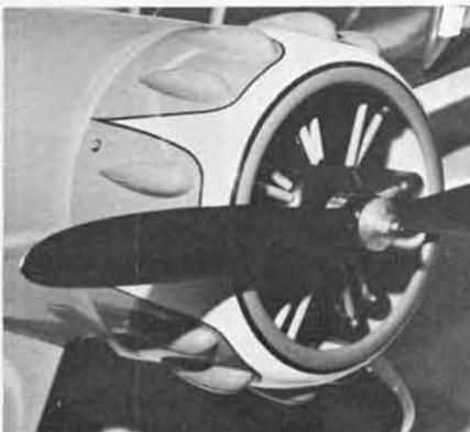
Valve covers on Tom Ingram's Waco, best Monokote winner, were individually covered, glued on, then filleted with narrow strips, using new iron from Top Flite, shown at right.
