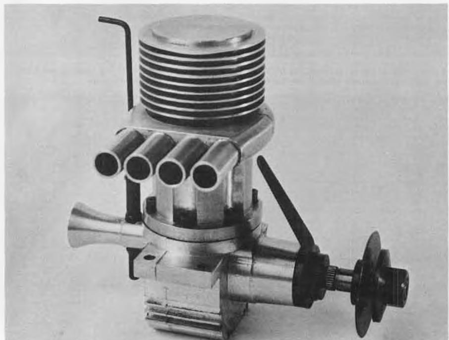
A homemade .30 cu. in. diesel built by Otto Bernhardt in 1946. It features a reed valve, bypass ports all the way around the cylinder, and adjustable compression by means of a crankshaft mounted off-center in a rotatable bearing (!). Photo by John Morrill.
