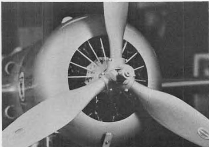
Prop hub is made from various bits and pieces, starting with plastic pipe and dowels. Blades are carved from pine or redwood.
