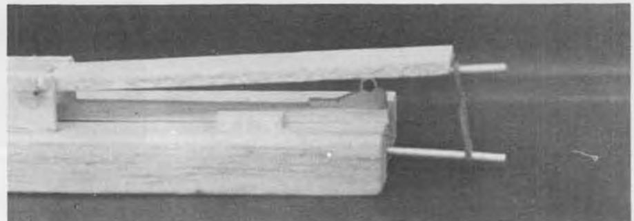
Stab end of Beattie's VIT system shows cam, which can be varied in shape to provide exact incidence variation with torque desired. See drawings below for clarification.
