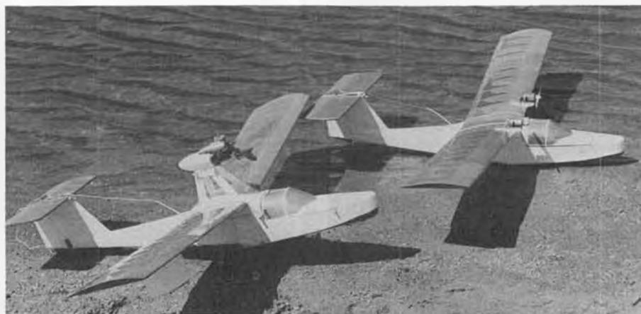
Two of Neil Whitman's original design seaplanes, both using the same fiberglass hull. Model in background has twin Astro 020's, one in front has an O.S. Max .10. Good fliers.
