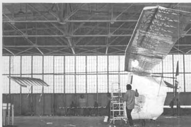
The Gossamer Albatross is a marvel of construction and design. Spans 96 feet, yet weighs less than 60 pounds!
