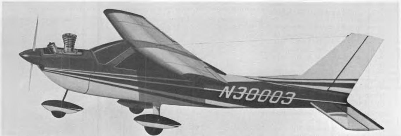
The all-foam Cessna Cardinal from Midwest is a good choice for the first-time R/C flier, as it goes together quickly, flies well, and is easy to repair, using 5-minute epoxy. Doesn't have to be painted and can fly with from one to three channels.
