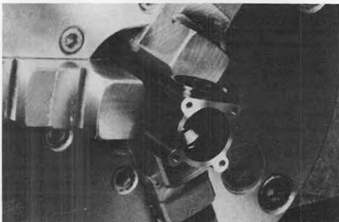
The rear of a Cox Black Widow crankcase that has been machined to decrease the crankcase volume.
