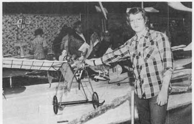
Garry Karner and "1910 Karner Monoplane". O&R Compact, homemade wheels, Douglas fir construction. Weighs 20 lbs.
