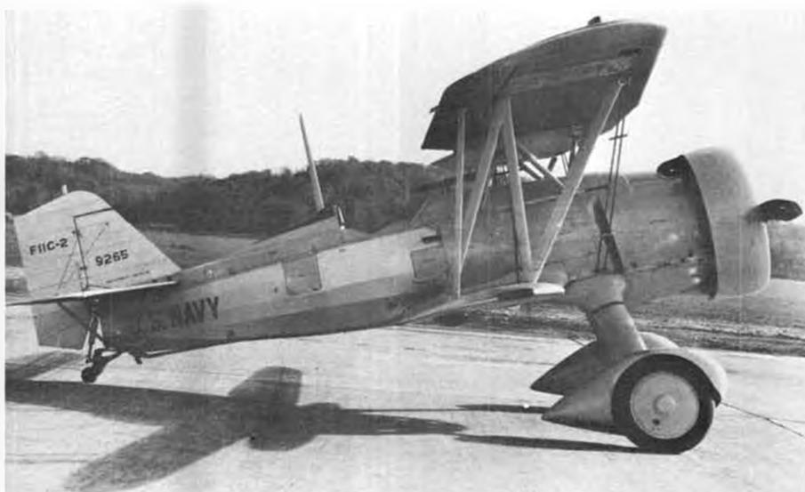
First of 27 production F11C-2s had a basic P-6E fuselage and tail, and the chord of the anti-drag ring has been increased from 12 to 18 inches. Smithsonian NASM photo.
