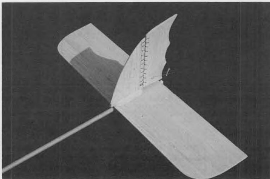
Percy's tail surfaces are simplicity in themselves. Figure-8 thread hinges are used on the rudder, are about the lightest and most friction-free type around, ideal for single channel.
