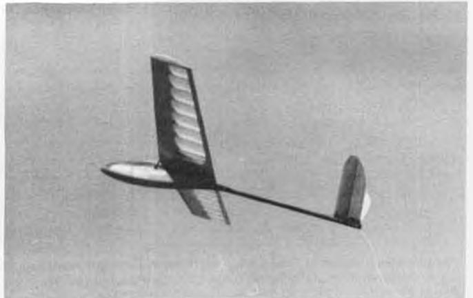
Two shots of Jay Juniper's original design V-tail mini-glider. Uses the ultra-small Kraft KPS-18 servos and small receiver and batteries. Total ready-to-fly weight is less than 12 ounces.
