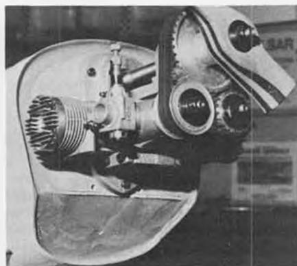
Is it a twin, or two engines? Belt drive unit combines two engines, by Cass Engineering.
