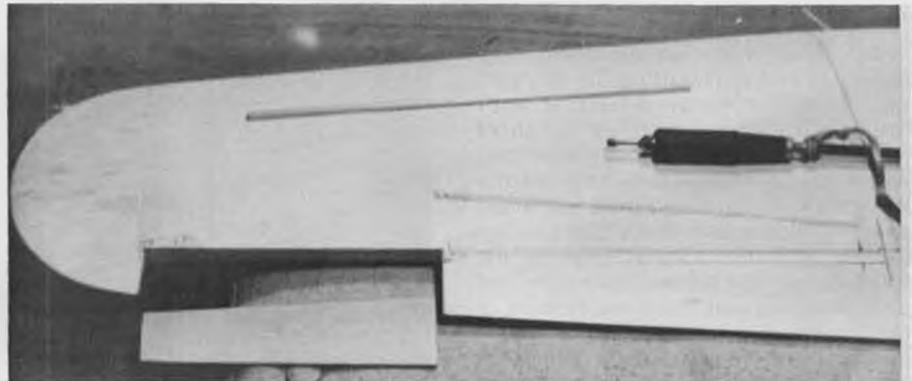
Aluminum tube torque rods buried in grooved foam core bend the ailerons. Wing finished with 3/4-ounce glass cloth.
