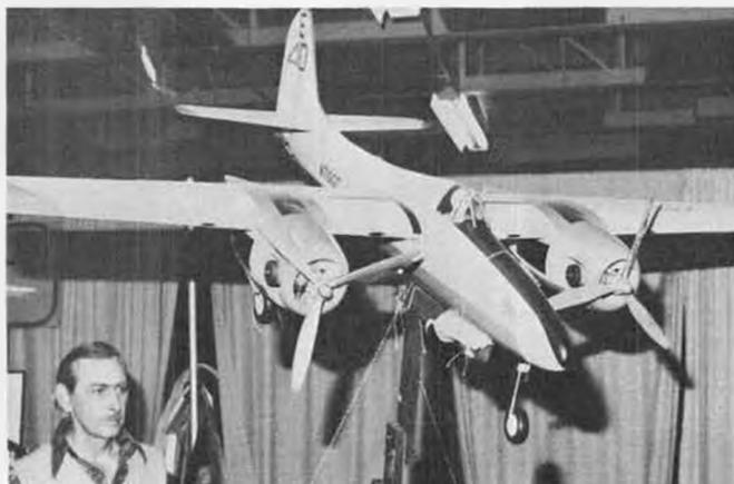
Frank Zwick and the F7F Tigercat he built from an R/C Kits . . . er, kit. Features built-up construction and foam cores.
