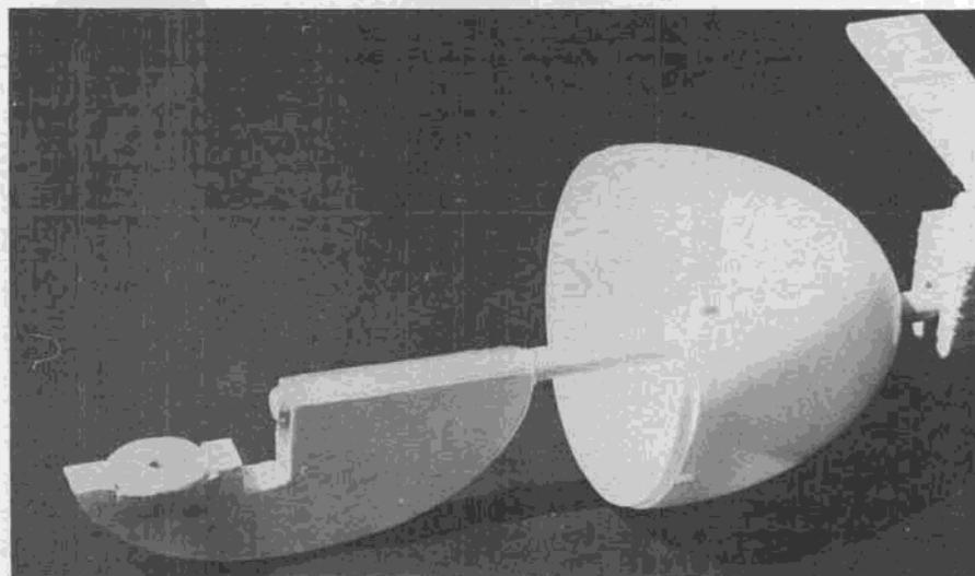
Actuator mount is a ply/balsa/ply sandwich and is contoured to fit inside of L'egg pantyhose container, then epoxied to arrow shaft. Rear half of egg shell is also epoxied in place.
