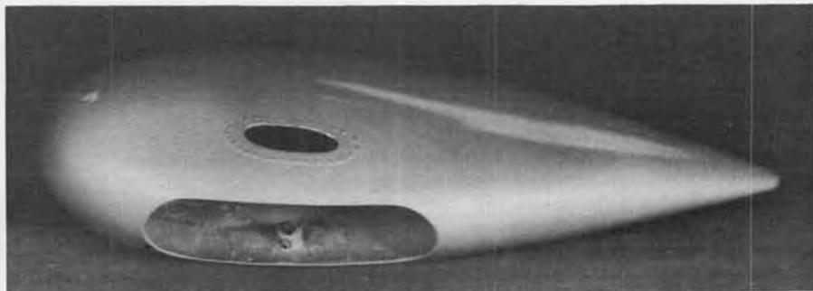
The colonel molded his own wheel pants over carved polyurethane foam molds. After glassing, foam was hogged out with an L-shaped piece of wire in a Dremel tool.
