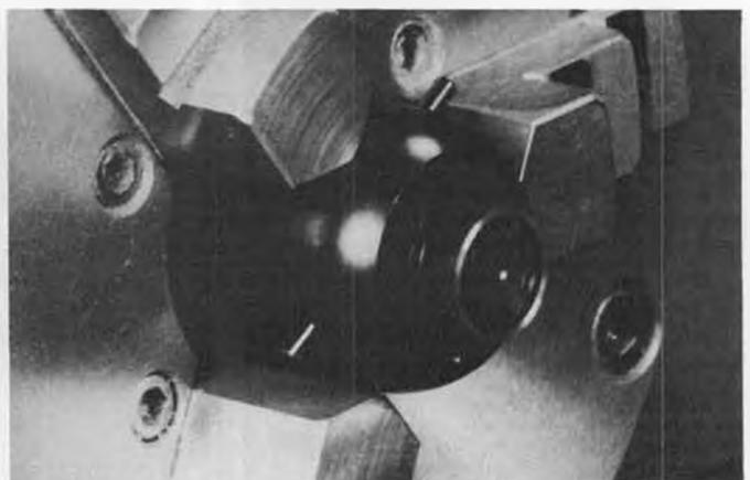
A Cox Black Widow tank that has been machined in the reed retainer area to prevent interference with the crankpin.
