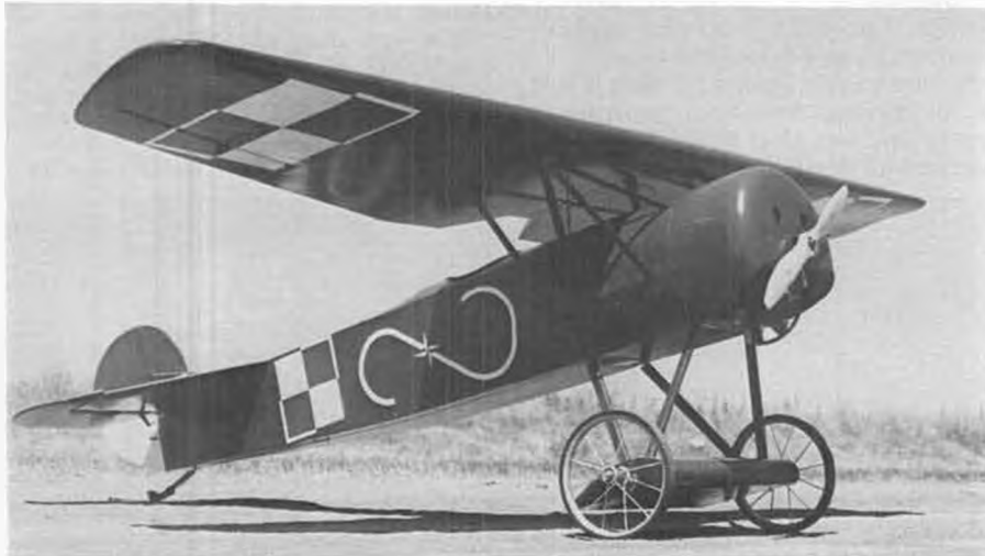
Bill Wendt's original scratch-built Fokker D-VIII is done up in Polish Air Force markings, finished in olive drab Permagloss Coverite. Span is just over nine feet, weight is about 27 lbs., and it's Quadra powered. Scale is 1 ft. = 1 meter . . . an unusual figure, but one that works very well, since the full-size ship was designed in meters; comes out to approximately 1/3 scale.
