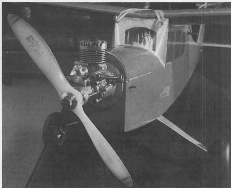
Charlie Bauer's Apprentice is powered by an Enya .35, about the most you'd want to use. Although not necessary, a side-mounted engine, with cowling, greatly improves the appearance.
