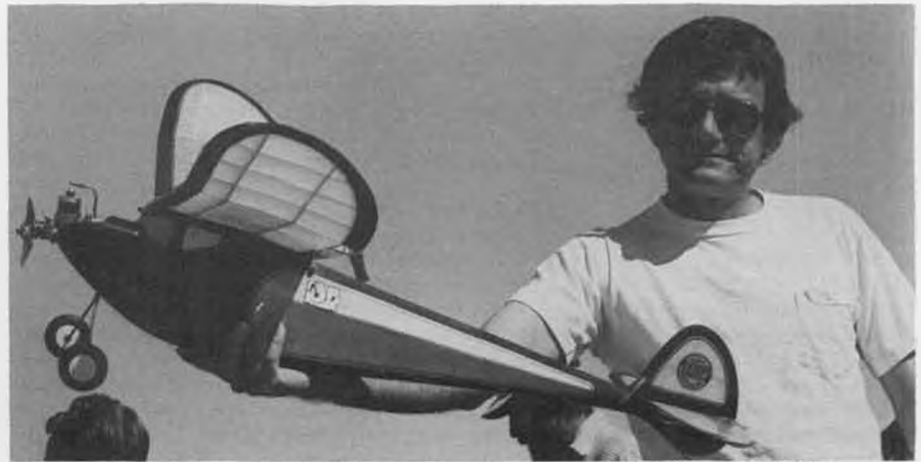
Very nicely done So-Long by VAMPS member Bill Holt garnered 4th place at VAMPS Annual. Powered by O.S. .15 with Bernhardt (77 Products) conversion. This and above pic by Stroman.
