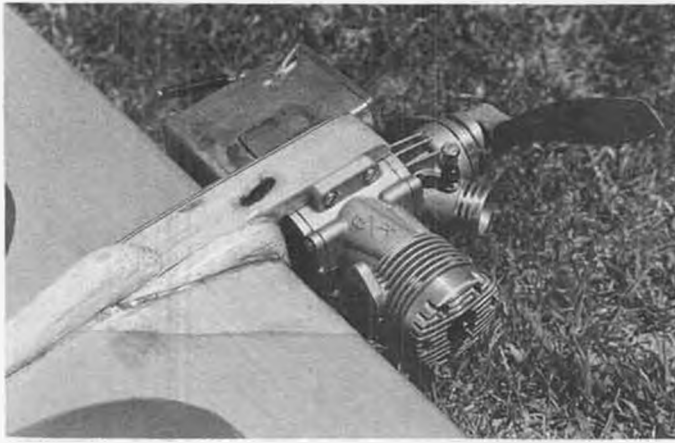
Outlawed for 1980-81 is this inboard tank set-up on Greg Hill's model. Tank is vented to run without a carb, but the same combination with swing carb should be capable of 120 mph or so.
