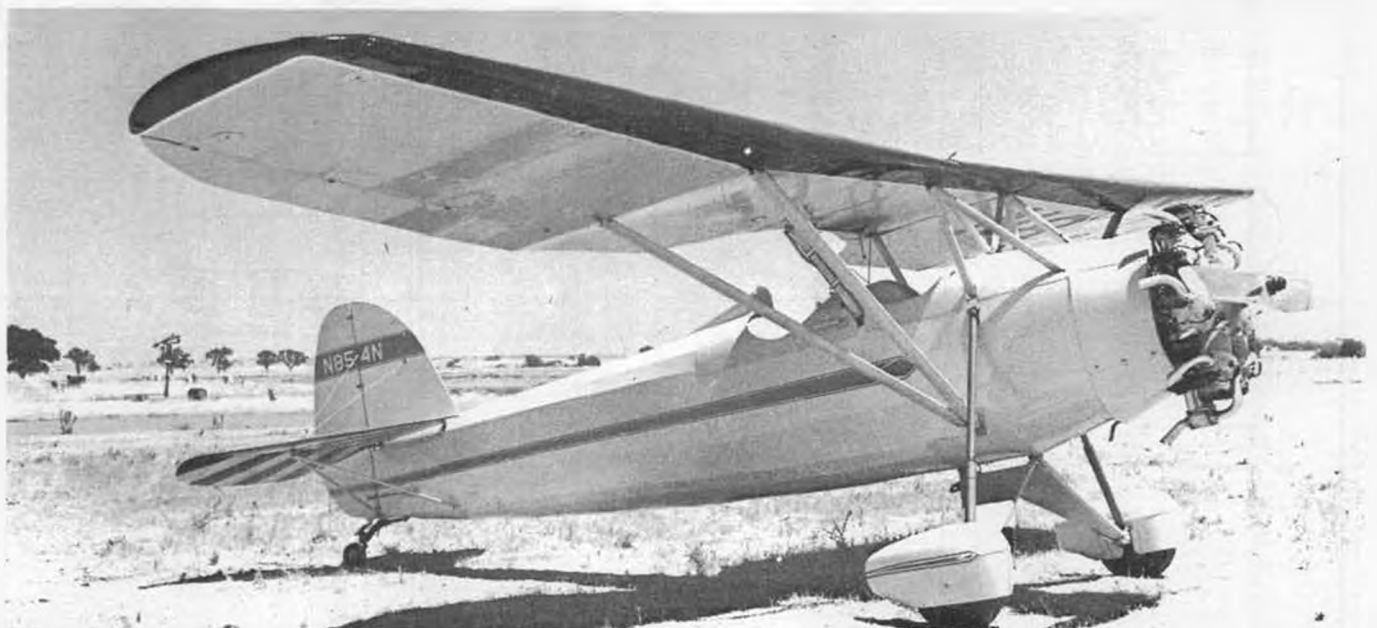
N-854N, a Davis D-1W, was rebuilt in 1965 by Joe Pfeifer of Columbia, California, with a 145 hp Warner and wheel pants from another plane. This and above photo from Pete Bowers.
