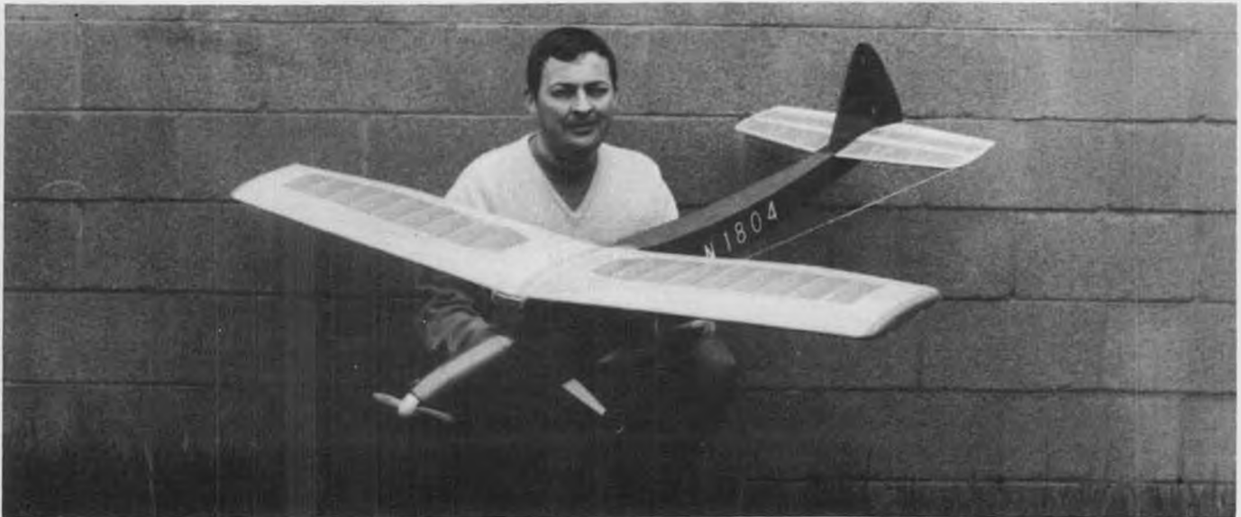
The only remaining photograph we have of the original Apprentice, taken in 1968. Weighing only 3-1/4 lbs., it flew very well with a Webra .20, was especially fun to do low-altitude "contour flying", a few feet off the ground and following the dips and rises of our grass field in Delaware.
