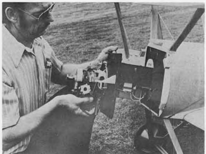
Ken shows the modular power unit on his Pup, held to the firewall with six bolts. Makes any engine servicing very easy.
