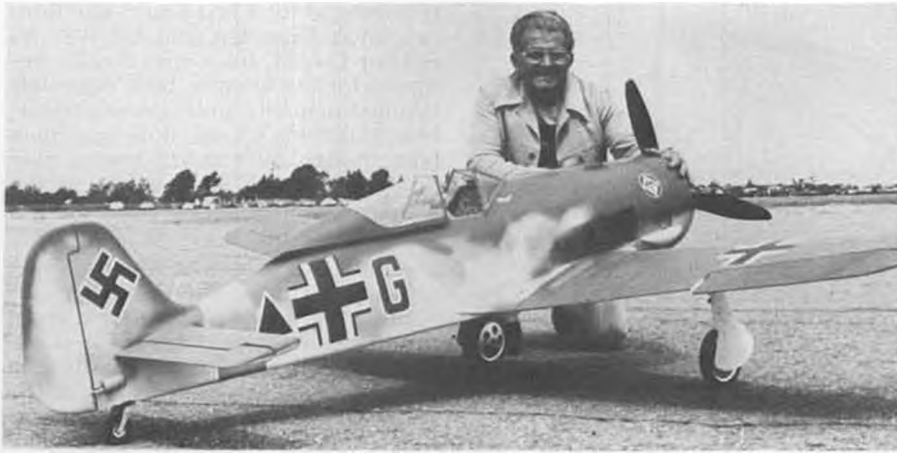
Ted Hyde show off his FW-190A, powered by a 3.6 cu. in. Poulan engine. Originally equipped with a Quadra, it was radically underpowered, can now loop from level flight!
