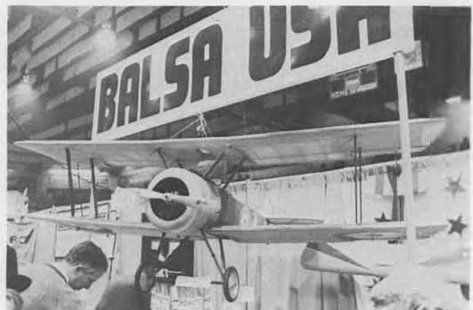
The nine-foot span Sopwith Pup by Balsa USA, has a wing chord of only 21"! Lots of redwood used in the construction.
