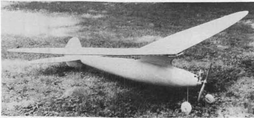
Speaking of Valkyries, here's one by SAM 7's George Armstead. Fuselage is 1/32 sheet wrapped over 1/16 longitudinal sheet, makes a light and strong framework. Brown Jr. power.
