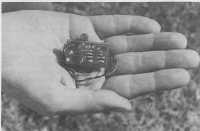
CFM's transmitter warning device mounts inside the case, light indicates that transmitter is on and also indicates low voltage.
