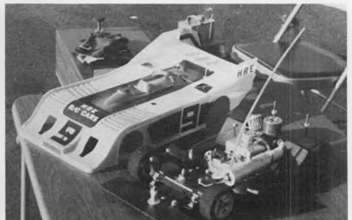
Mike Pino's H.R.E. car had an aerodynamic wing/tray, didn't use a rear wing or spoiler. Shows promise.
