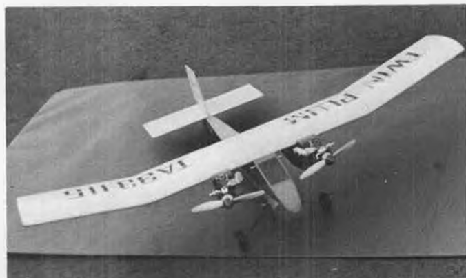
"Twin Plum", novel R/C design by Mr. Tate Bayashi, Japan, flies safely on one engine. Two .09 engines, 3-ch. radio. (Ichiro Yamada).
