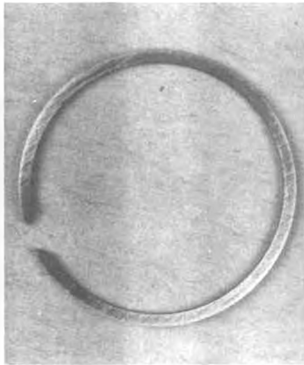
Photo 4. Ring has been lapped on a stone to loosen fit. Note cross-hatch lap marks.
