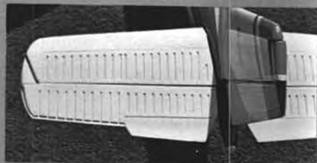
Other super scale features include vacuum-formed skin detailing for stabs and control surfaces.
