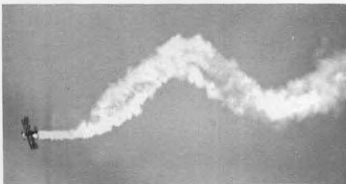
Obviously a heck of a lot more smoke than ever seen before, from a model or full size aircraft. Keeping the diesel fuel in the muffler chamber for a longer heating period completely vaporizes it, rather than spitting out raw fluid. Muffler available from Harris.
