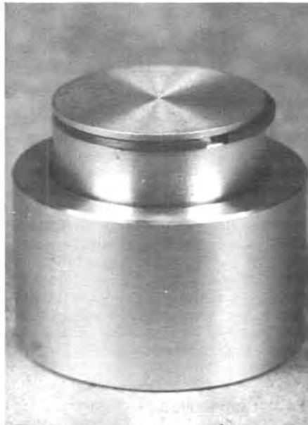
Photo 5. Ring compressor tool provides best way to get piston/ring in cylinder.
