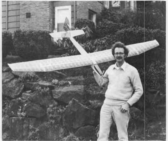
Mitch's Olympic II flies very well with Leisure Selected Stock motor, 8 x 4 prop, six 1.2 amp cells. Powered flights of 8 to 10 minutes.
