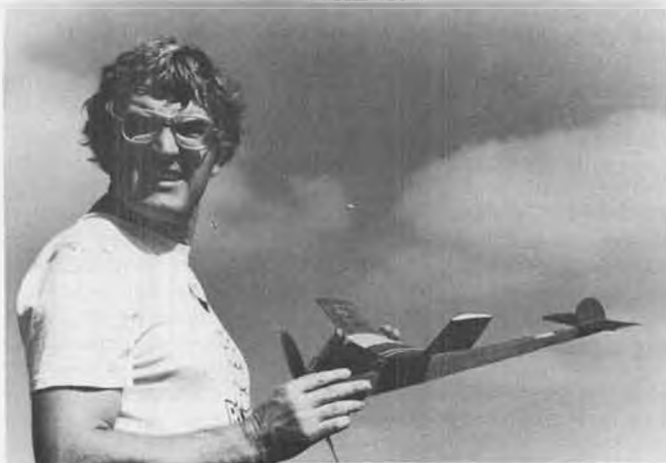
Above: Dave Hagen's P-30 uses wing from Comet Cloudbuster design. Warp in right wing caused total destruction during power burst. Right: Bob White shows off P-20 design for 1-minute maxes on small fields. See text for more on this. Photo by Toni White.
