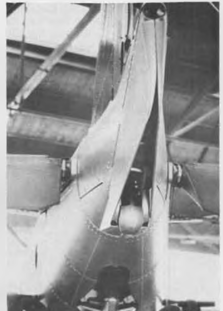
Spring loaded flaps on tail cone covered arresting gear hook. Hard rubber bumper inside flaps. (Walt Stampfli collection).
