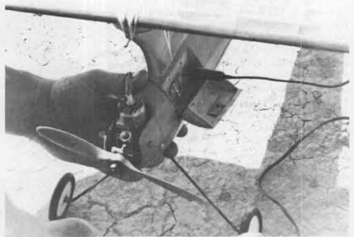
Photo 2. Neat ignition and timer enclosure keeps desert dust out of Al Heinrich's Ranger. Photo by Bill Stroman.
