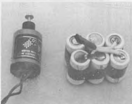
Potent Leisure Black Label motor, delivers 12,000 rpm on 6 x 4 prop with only six cells!
