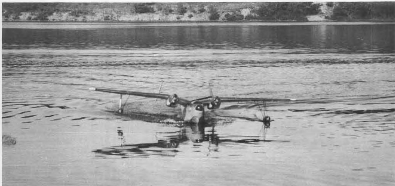
Seen at the annual Brimfield (Massachusetts) Hydro Contest, John Nicalaci's 40 pound PBM. It spans 13 feet, is powered by two St .71s with Eastcraft starters. Basic structure is foam. Has been around over 5 years, appeared on M.A.N.'s cover.
