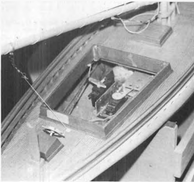
Radio equipment in hold of schooner Benjamin Lathum, built by Arnold Cross. Probar sail unit. Two-channel radio.
