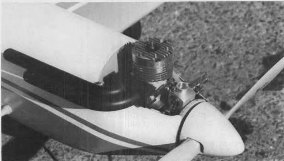
Enya 45 with Slimline muffler makes a perfect power combination for the FB-100, which will handle .40 to .60 size engines. Modern 60's are really more than enough. Top Flite 11x6.
