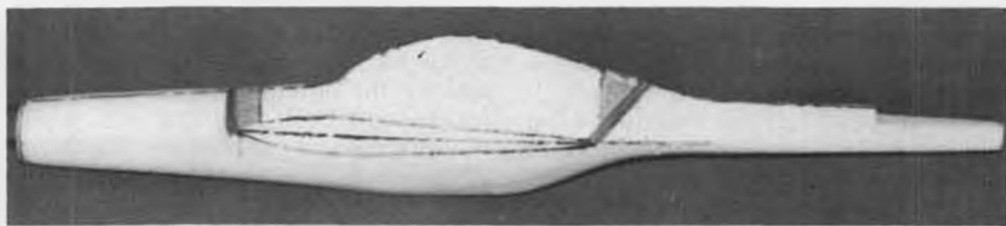
Separation bulkheads installed after fuselage shaping is completed.
