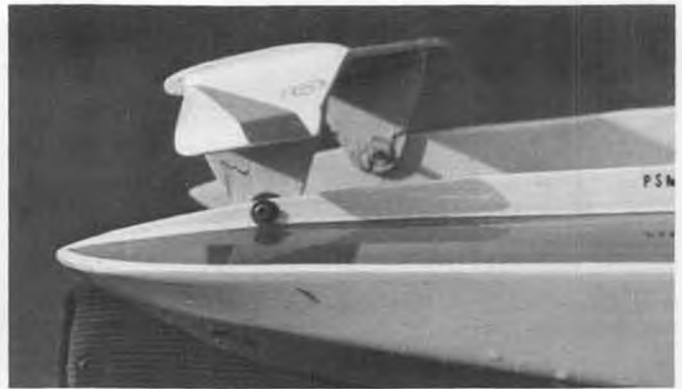
Side view of Excaliber II bow wing. Note 6-32 cap head bolt used for mounting wing.
