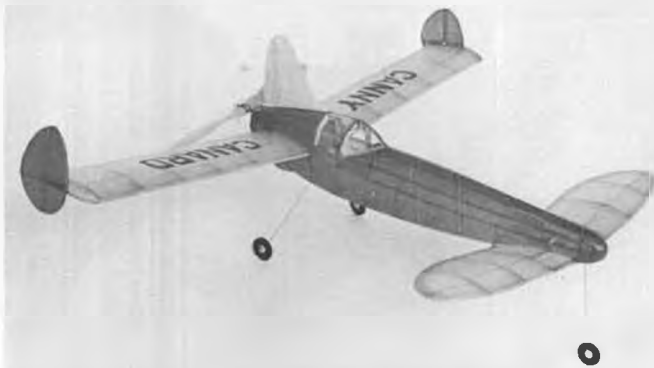
Canny Canard sport model designed by H.A. Thomas for M.A.N. Sheet fuselage modified to built-up by Mark Fineman, Hamden, CT.
