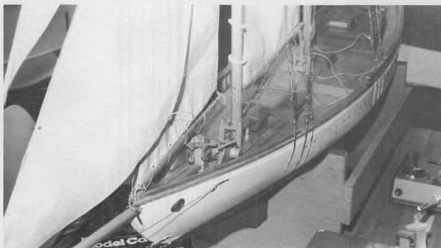
Another view of the R/C schooner Benjamin Latham, built by Arnold Cross. Hull is carved wood, using "bread and butter" system better known prior to fiberglass.
