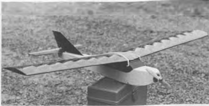
Astro Sport with Leisure Black Label motor, six 1.2 amp cells, 6 x 4 prop, 8 to 10 minutes of continuous powered flight.
