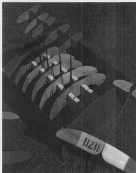
Carrying box helps organize gaggle of gliders. This one built from 1/8 veneer ply. Gliders rest in notches in 1-inch Styrofoam.
