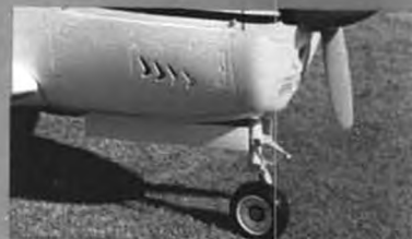
Scale effects include molded louvered inspection panel, landing light and grill plus scale nose gear strut, wheel doors, cowling flaps, engine exhaust & removable cowling.
