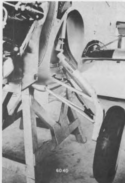
Landing gear design same as F2F. Cylinder and rod ahead of elbow is an air dampener to let the gear down easy. Grumman photo.
