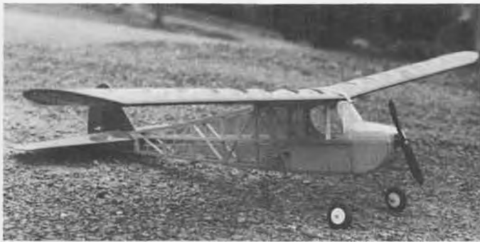
Berkeley Brigadier, with Leisure Selected Stock motor, 8 x 4 prop, six 1.2 amp cells, excellent flights of 8 to 10 minutes duration.
