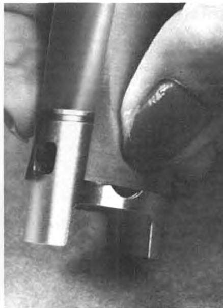
Photo 6. Shim brass stock will compress ring for inserting piston. Easier than making tool.
