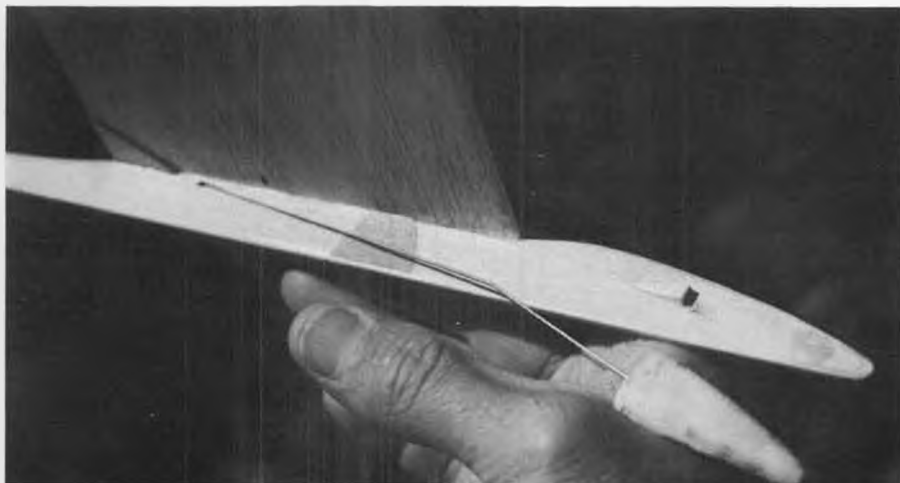
Simple D/T: Noseweight on swinging arm made from piano wire. Held in place by rubber band, it swings backward when fuse burns band in two.
