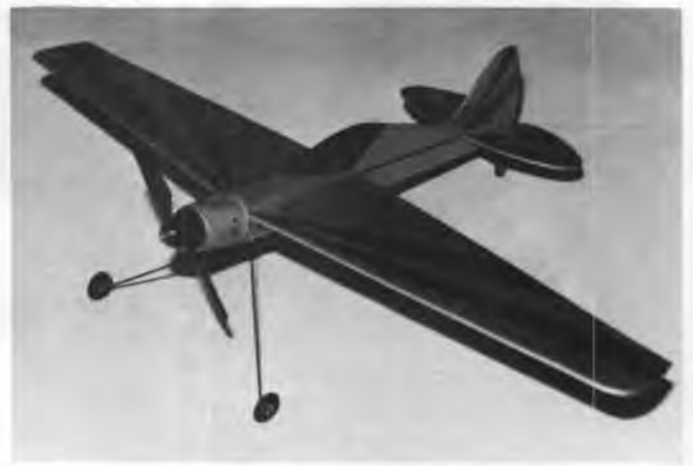
The "Challenger", by Electroline, electric powered control line with on-off control in handle.
