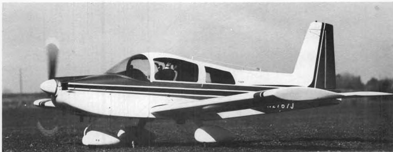
Chris Evans' version of the Hobby Lobby Grumman Tiger, modified by Chris to break down completely to fit into a small car. Six months old when this photo was taken, it died 10 minutes later from interference! Quadra powered, 24 pounds.
