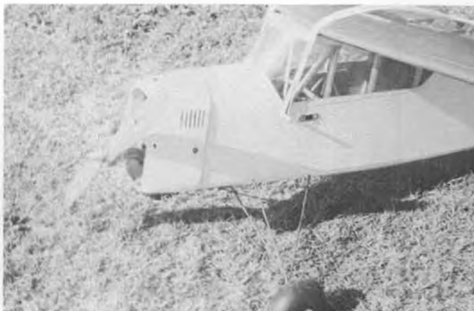
2. Close-up of special fiberglass cowl made by Speed Hughes for his Yates model.
