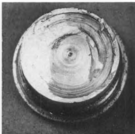
1. Overindulgence of electric starter was cause of this badly chewed up backplate.
