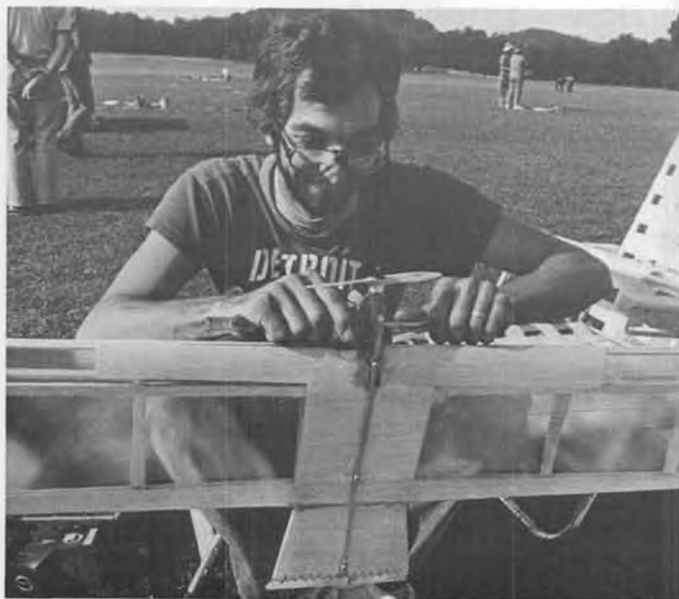
Ron Columbo doing a little maintenance. Note metal motor mount running full length of model. One was actually seen to break, however.
