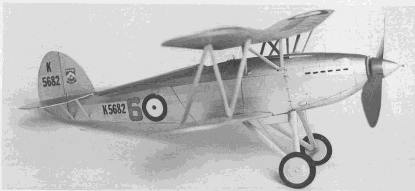
Hawker Fury I built from 22-inch plan originally published by Great Lakes Model Engineers, now available from Golden Age Reproductions. Slightly enlarged stab, modified airfoil. Excellent flier. Model and photo by Mark Fineman.
