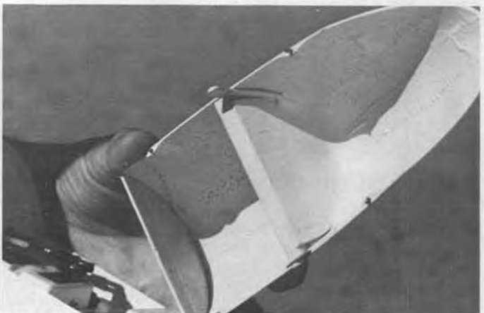
Here's a neat canopy or hatch hold-down device, demonstrated on Ralph Loveland's Swift. Pieces of spring steel with short section of dowel affixed near ends. Drill holes, epoxy springs in place, mark dowel locations with canopy/hatch in closed position. Clever!
