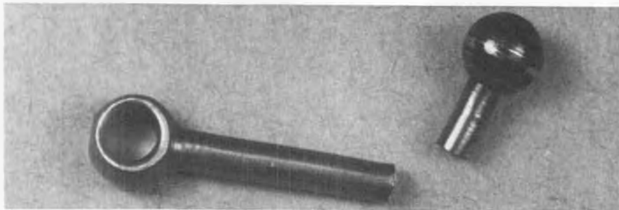
3 and 4. Ultimately, the ball-socket joint and the rod failed. If an engine doesn't fire immediately, back off the starter . . . Something's wrong, and grinding away doesn't help matters.
