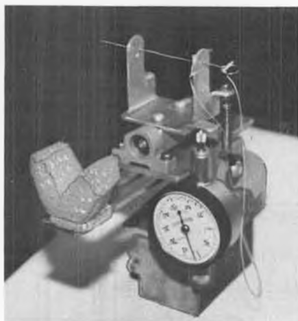
Ron Ganser's exotic torque meter. As motor is wound, holding stand twists, exerting pressure on the plunger of the readout meter. At right, model is in position, ready for winding . . . and measuring.
