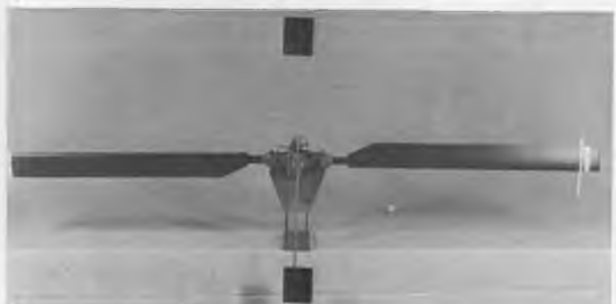
This small piece (on right tip) is all it took to give perfect spanwise balance. High-Point Balancer is sure sensitive!
