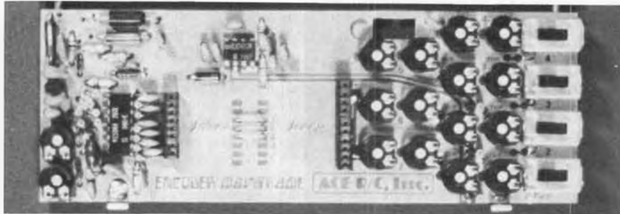
Main encoder board is the heart of the Silver Seven, contains all of the electronic wizardry that takes full advantage of the Signetics IC chip.
