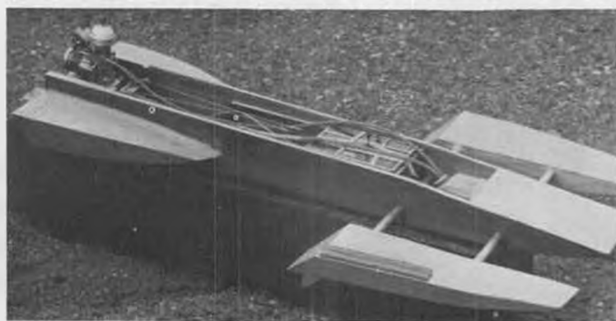
Removed hatch cover reveals forward placing of fuel tank. G&M radio box, Kraft radio, K&B 7.5 Outboard.
