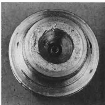
2. Spread of metal contamination damaged the chamber surface of the glow head.
