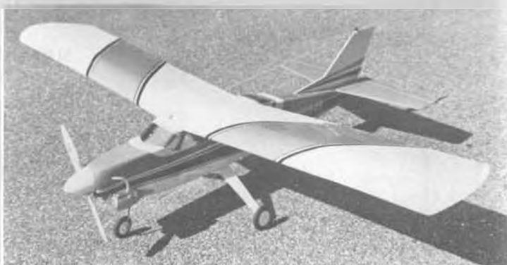
You may think you are looking at a Cessna scale model but it's actually Faye Stille's (Wilton, CT) Kadet Jr., duded up with an inverted S.T. 25 engine and scale colors. He kept it light, says it will do 3 vertical rolls.
