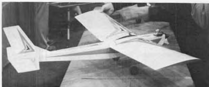
Craft-Air Cowboy 15 for .09 to .19 engines. Span 50 inches. Ply fuselage sides, three or four channels.
