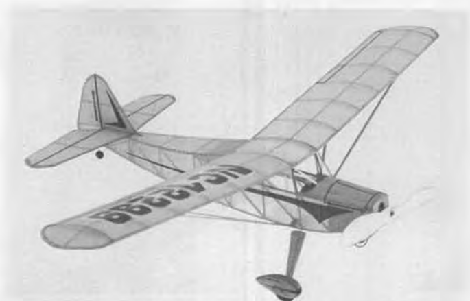
Semi-scale, 22" span Taylorcraft CO2 kit by Micro-X. Has done one minute, 34 seconds in highschool gym. Weighs 1-1/8 oz. total.
