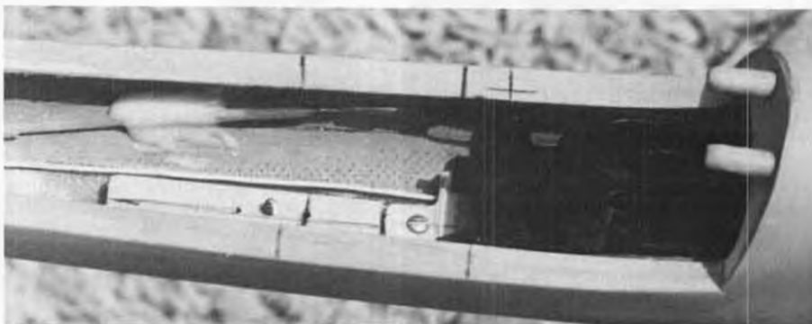
No canopy on Concept II. Radio gear slides forward into nose on tray, accessible through wing opening. Neat idea. More specs on plane in article.
