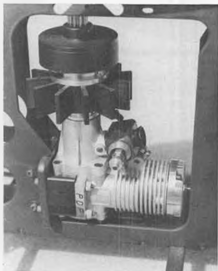
HB 40 PDP mounted in Super Mantis. Rossi-type carb in HB works flawlessly.
