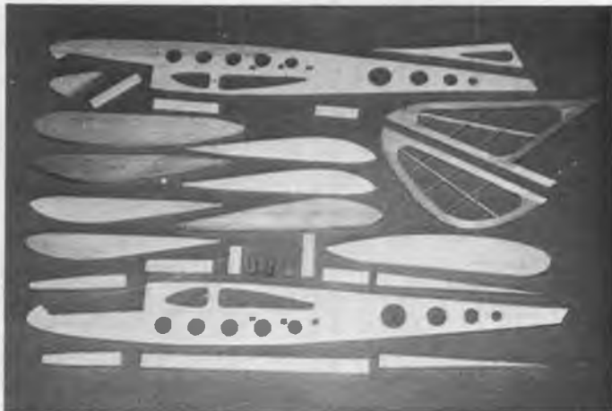
All fuselage parts "kitted out" and ready for assembly. Sides are 1/8 thick Lite Ply.
