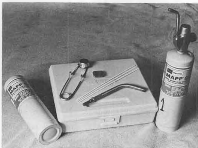
Al's Mapp Gas Torch, fully described in the text. Great for those heavy duty landing gear joints.
