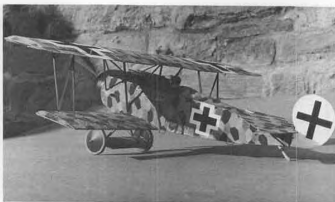
Mike Hetherington, England, built this 15-1/2" span Fokker D-VI. Tissue pre-colored with thin poster paint. Rotating engine, gearbox.
