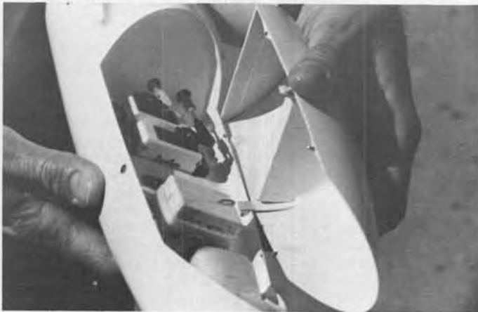
Here's a neat canopy or hatch hold-down device, demonstrated on Ralph Loveland's Swift. Pieces of spring steel with short section of dowel affixed near ends. Drill holes, epoxy springs in place, mark dowel locations with canopy/hatch in closed position. Clever!
