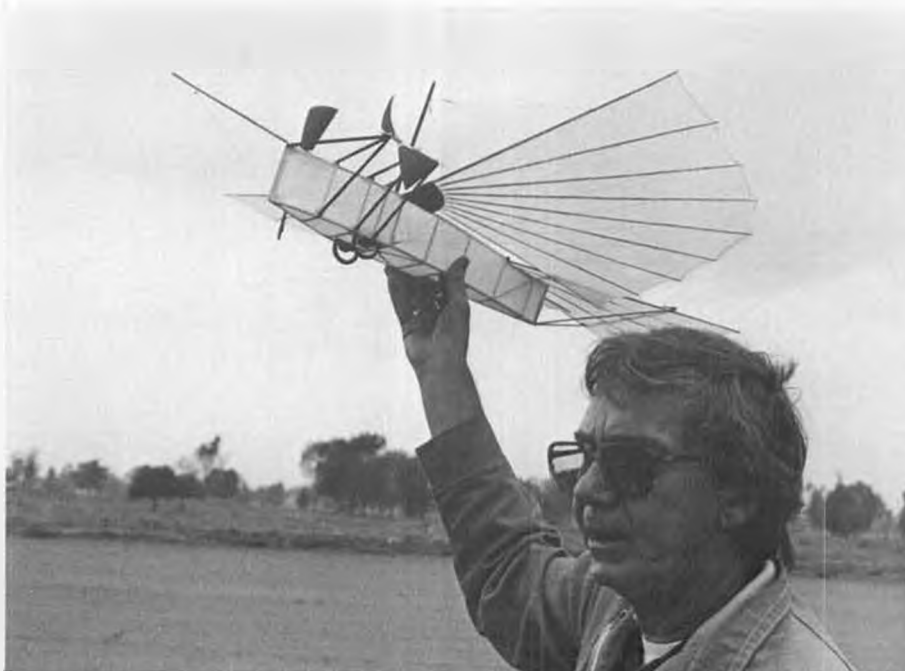
Original wings opened and folded like a Japanese fan. Model proves that it very well could have flown . . . and prior to the Wright Brothers at that!
