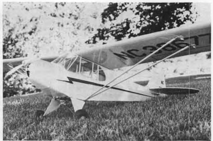
Scratch-built two-inch scale J-3 Cub by Bill Gilchrist, Oskaloosa, Iowa, powered by Astro 15 motor with 3:1 speed reducer, Zinger 13x8 prop. Excellent performance.
