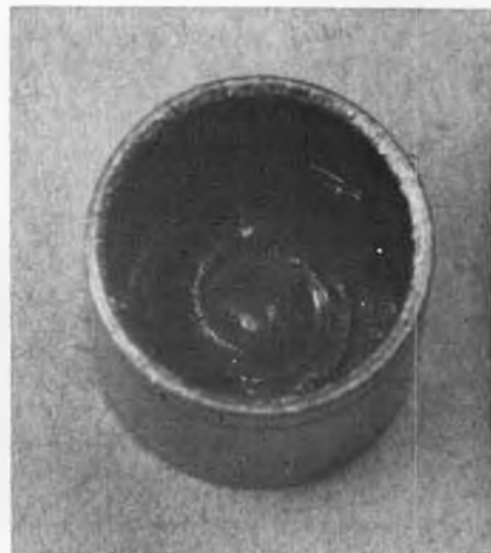
3 and 4. Ultimately, the ball-socket joint and the rod failed. If an engine doesn't fire immediately, back off the starter . . . Something's wrong, and grinding away doesn't help matters.
