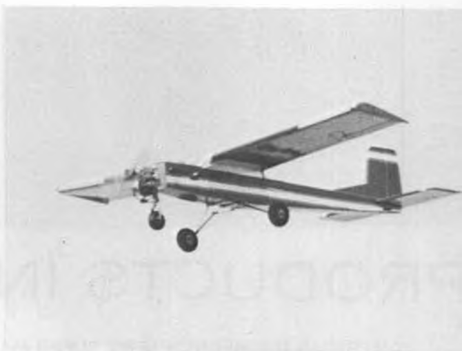
An 8-foot, Clark-Y airfoiled version of an RCM Trainer with a 1.3 Kawasaki turning a 16 x 6 cut down from 18 x 6.
