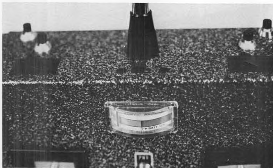
Close-up of author's transmitter, showing two-in-one meter and various switches as described in text.
