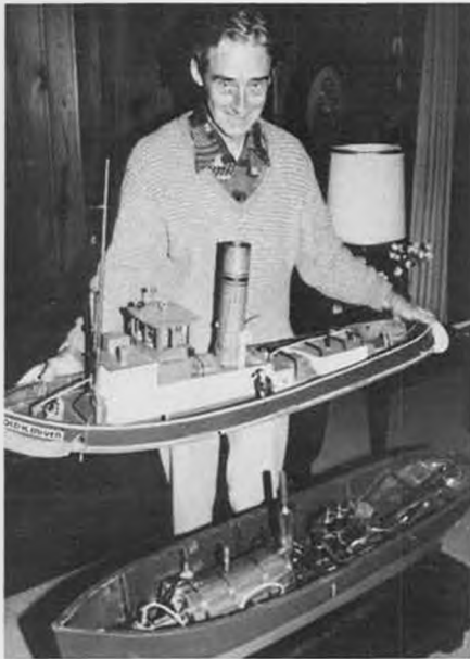
Bob McKibbin, Auckland, N.Z., displays his steam tug Harold H. Shriver . Features scratch-built boiler (5x10) which is propane fired.
