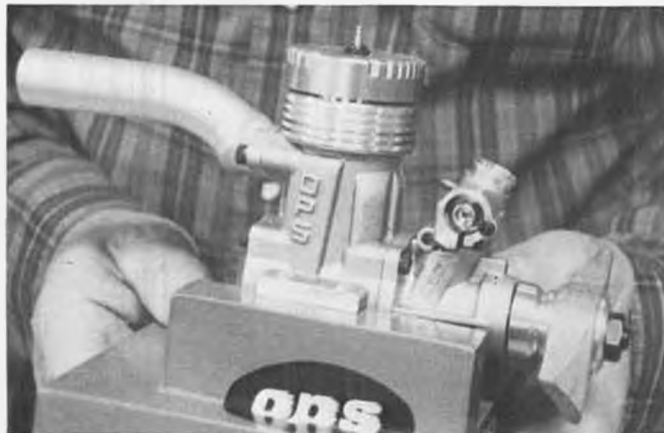
OPS "Super .60" is rated at 2-1/3 HP at 17,000 RPM, with FAI (no nitro) fuel. A five intake port engine.
