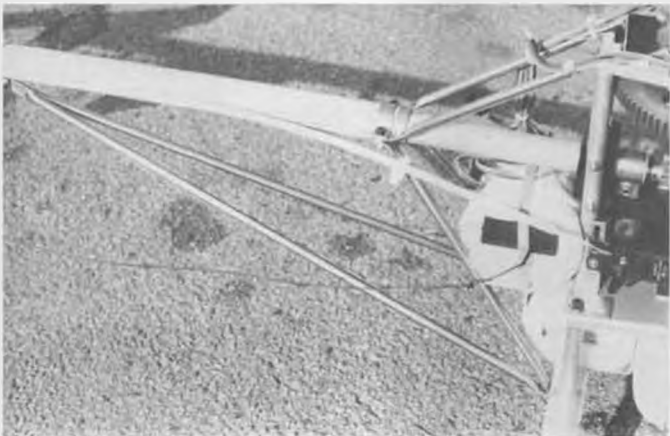
9. Tail boom braces. Tail boom joins main fuselage where short braces mount to boom. Text describes technique for assembly.
