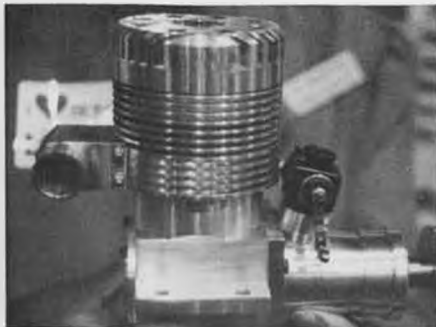
Nice looking 1.2 cu. in. bar stock engine for $250, weighs 2-1/2 lbs. D.M. Model Eng.
