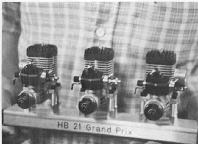
The HB 21 Grand Prix cylinder can be rotated to accommodate the the installation; right side, left side, or directly aft.
