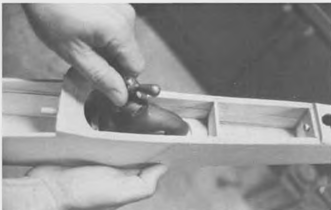
Okay, so water ballast is impractical in the Gemini. At least it has an unobstructed ballast box capable of holding four pounds of lead!
