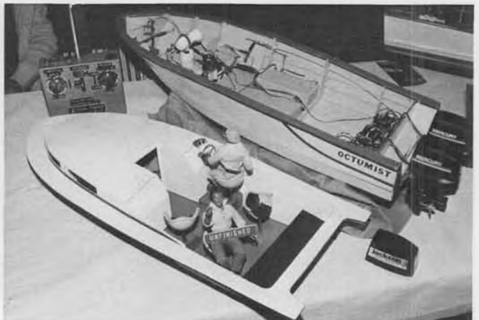
Harold Shriver sends these two photos of an unfinished Octumist double Jackson 54 powered outboard. Uses two 6v motorcycle wetcells, or four 6v gellcells. Average run is 25 min. Steering wheel turns with motors. L.O.A. 30 in., beam is 12 in., scale is 1-1/4 in. to the foot.
