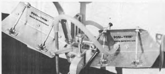
The Posi-Trim adjustable ride plate from Mach Enterprises. Can be used on inboard or outboard models.
