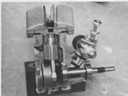
An OPS cutaway 3.5cc engine, showing design and construction details. Note porting.
