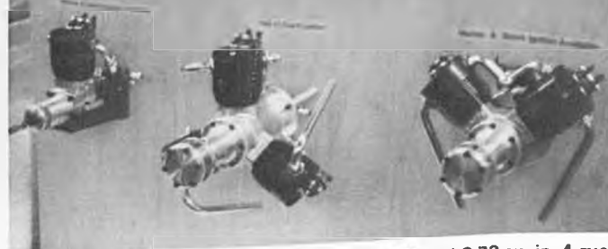
Not the Contempo Magnums, these .91, 1.82, and 2.73 cu. in. 4-cycle engines come from England. Beautifully made.
