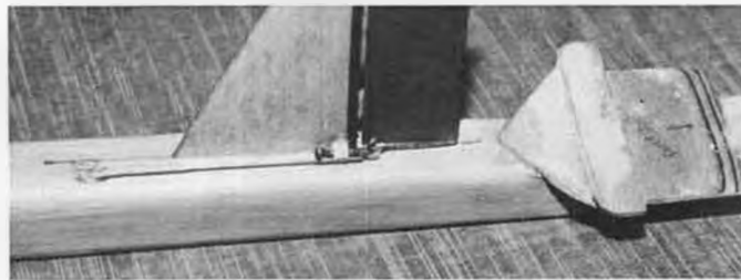
AMA gas model equipped with V.I.T. and autorudder. Stab mount is made from plywood. Model is Joe Foster's Buck 650.
