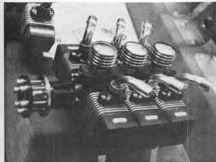
Horizontal opposed 6-cylinder, 3.6 cu. in. engine by Lou Ross.
