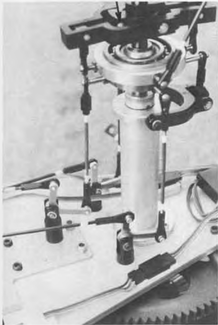
7. Anti-rotation link, swashplate, and washout control. See text for details concerning arrow.
