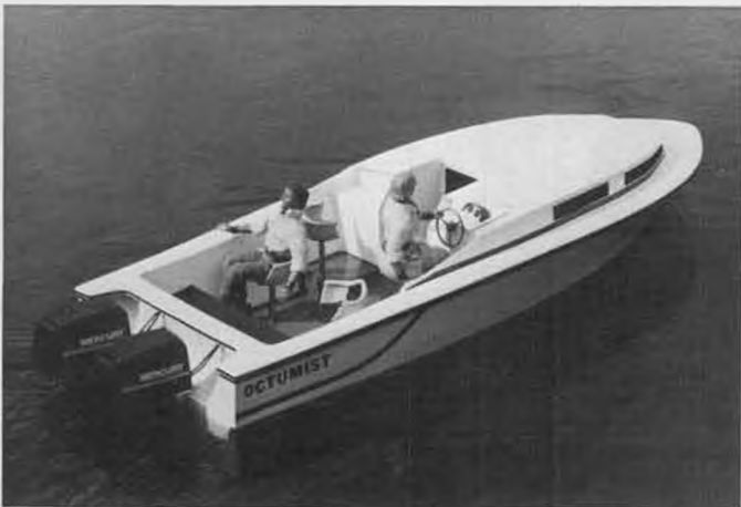
Harold Shriver sends these two photos of an unfinished Octumist double Jackson 54 powered outboard. Uses two 6v motorcycle wetcells, or four 6v gellcells. Average run is 25 min. Steering wheel turns with motors. L.O.A. 30 in., beam is 12 in., scale is 1-1/4 in. to the foot.
