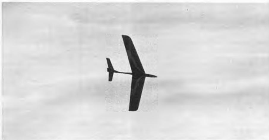
Dennis Cook's prototype Askant in flight. Production models do not have this much sweep in the wings. Ship is fully aerobatic, and very fast! Eppler 374 section, foam wings.
