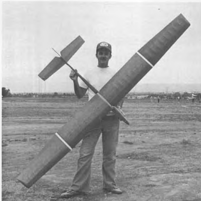
Mike Charles poses with the Gemini M.T.S. showing its top view. High tail volumes yield excellent handling characteristics.
