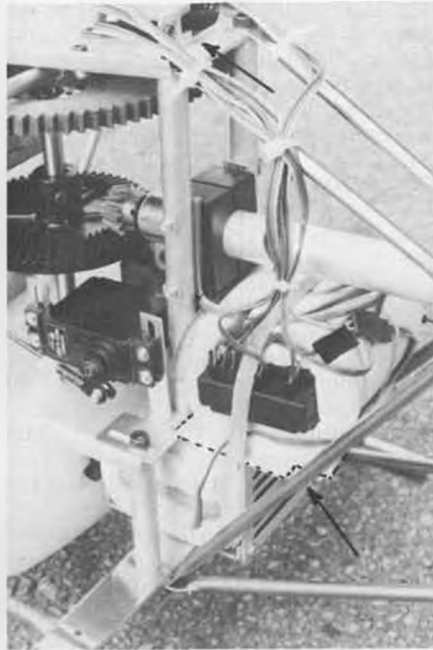
8. Throttle servo detail; 1/16 plywood plate (dotted line) supports receiver. Note arrows.
