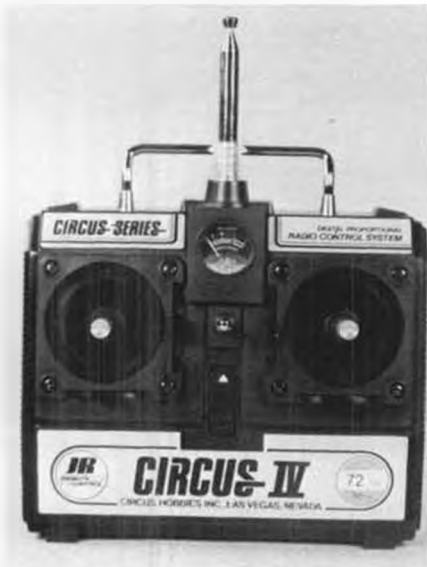
The DR-124 transmitter, as furnished with the Circus Hobbies Circus IV radio system. Commonly known as "The Hundred Dollar Radio".
