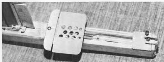
Typical double arm V.I.T. Magnesium stab mount. Springs are attached in middle of lines. Note the layout of the auto rudder at left.
