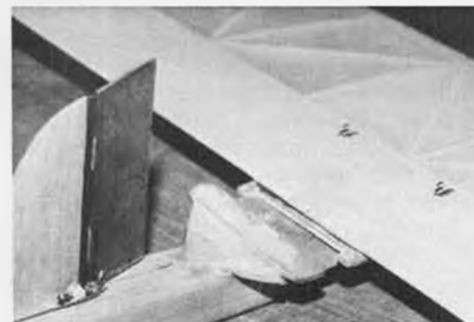
Same model as below. As in system on left, stab "ears" slide under mount.
