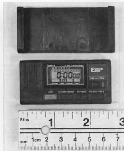
The Electric Eagle EE-1 Timer is intended for mounting to the front of the transmitter. Features: time, stop watch, countdown, more!
