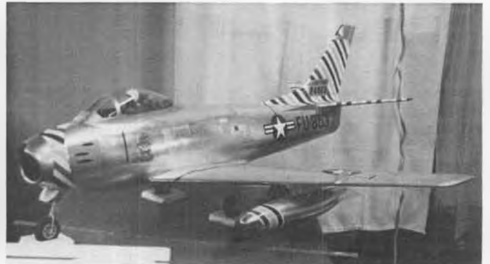
This F-86 ducted fan uses scale intake, no big hole in the bottom. To be kitted by Bob Violett. Contact him for details.
