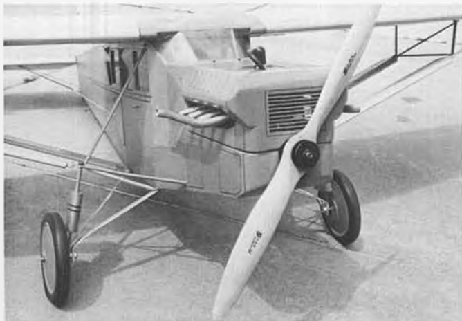
This close up of the Robin shows all of the various struts and braces . . . plus one safety hazard . . . rope starter trying to fake it as a prop washer.
