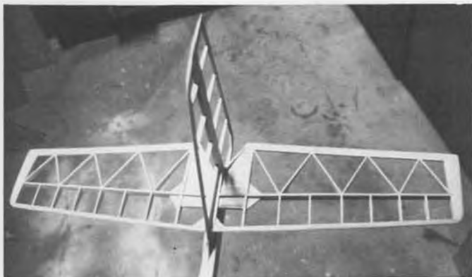
The all-moving horizontal stab features 1/2-inch thick airfoil, built-up spar, diagonal ribs, thick pivot tubes. This stab can take lots of abuse!
