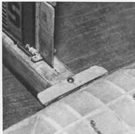
Stab "ears" slide under metal plate for a slop free fit. No hold-down bands needed.
