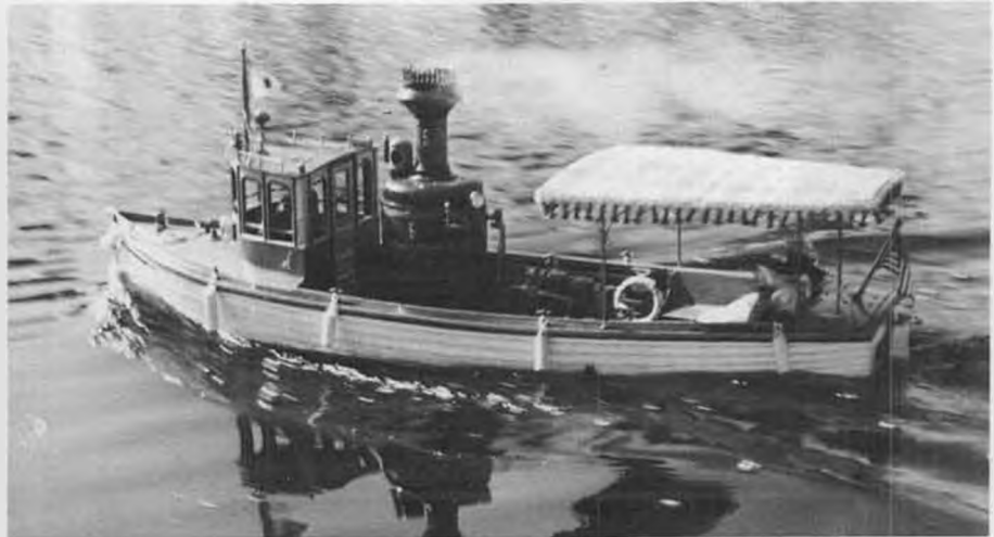
Here's another fantastic, scale R/C boat. This one is the Kaammaha , a 43-inch, Stuart Turner Double 10 steam engine with scratch-built 5x10 horizontal boiler (propane).
