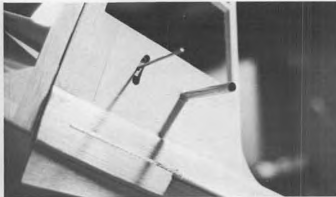
The author chose nylon bellcrank over 1/16 ply 'crank provided in the kit. Wide pivot tube, aerodynamically balanced stab are flutter-proof.
