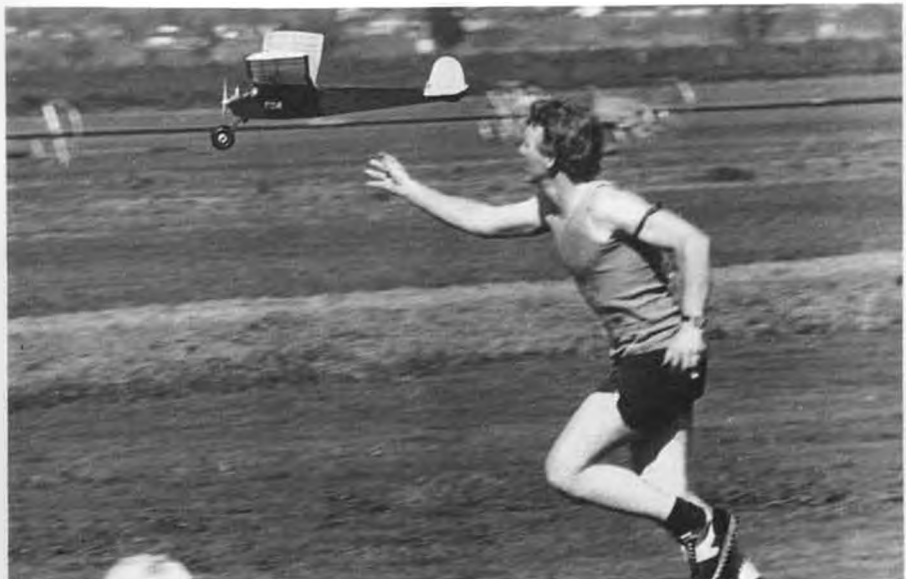
Steve Rothwell is one of very few model engine builders in Australia. Action shot shows him launching a Scramble model powered by one of the R-100 diesels he manufactures. Fuel supply is strapped to left forearm and filling syringe is seen between his fingers. Scramble event is unheard of in America.
