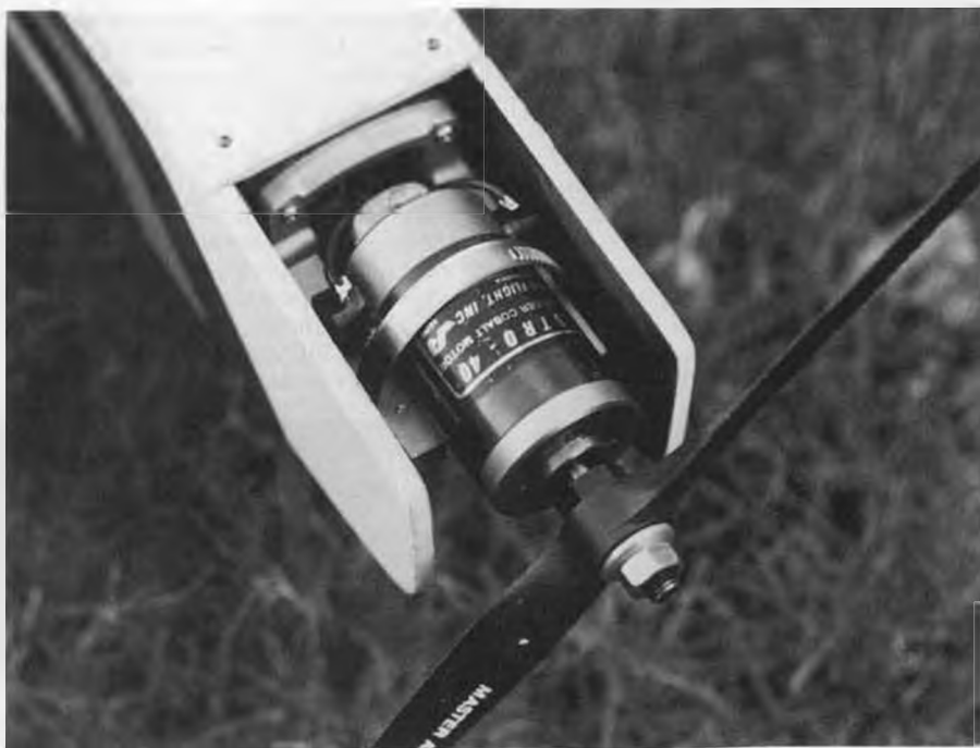
An Astro 40 in Royal Air 40S; hose clamp is used to hold motor in place.
