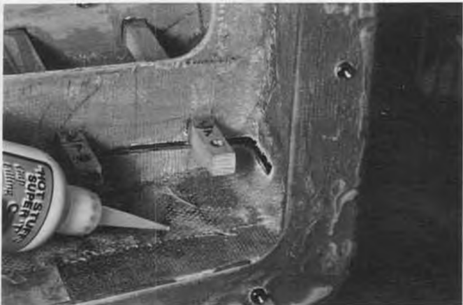
Glassing the fuselage former.
