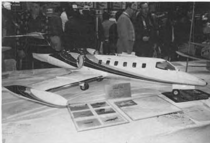
The winner in Non-Military Stand-off was Mark Frankel of Gladwyne, Pennsylvania with his Gates Learjet 35A. A large model at 1/6 scale, it spans 83.5 inches and is powered by two Rossi .65s.
