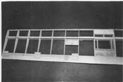
Ailerons are built as part of wing, then cut apart later to assure proper fit.
