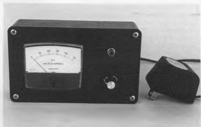
An externally powered variable-metered Constant Current Charger, built from the schematic by Laura Novak, at left. Such a charger is handy if you use a lot of different batteries requiring different charging rates.
