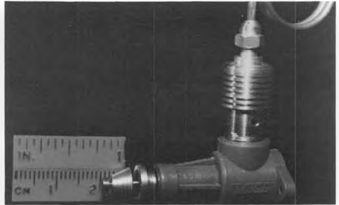
Steel cylinder is rotated up-down to control speed of Modelar CO 2 . Piston, crankcase and rear cover are plastic moldings. This is a motor, not an engine. Text tells why.
