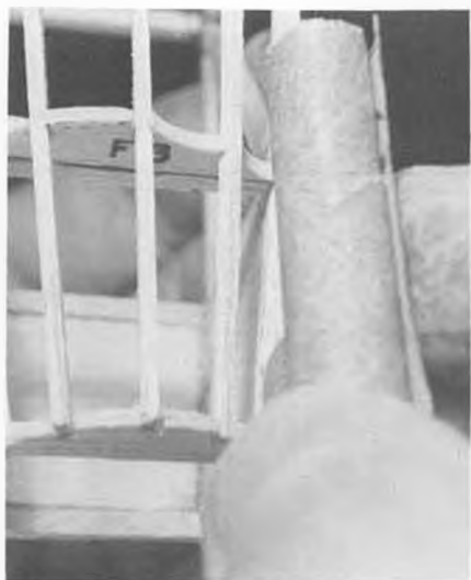
Pinch the tail portion of the fuselage with triangles and glue when it is lined up directly over plan view.
