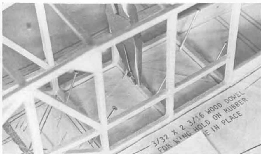
Sand the first(right-hand) side lightly with sanding block before covering with Saran Wrap to build the other side on top.
