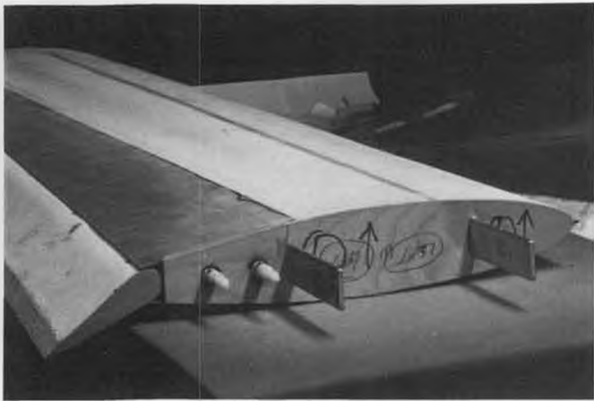
The plug-in wing just before glassing.
