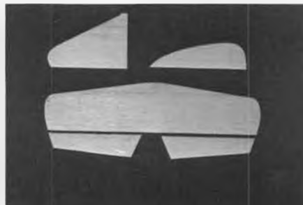
Completed airframe ready for covering. Simple sheet structure is light and strong.
