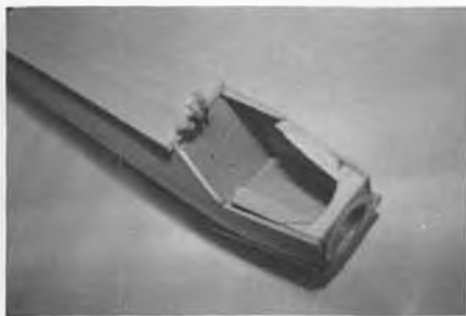
Engine compartment before shaping and painting inside with polyester resin.
