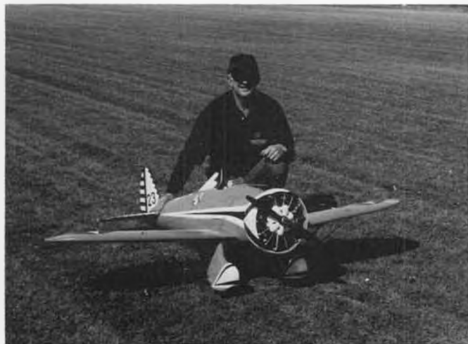
Mammoth Scale P-26 Pea Shooter by Geoff Burfield spans 88 inches and weighs 27 pounds. JR radio and Webra Bully on board.
