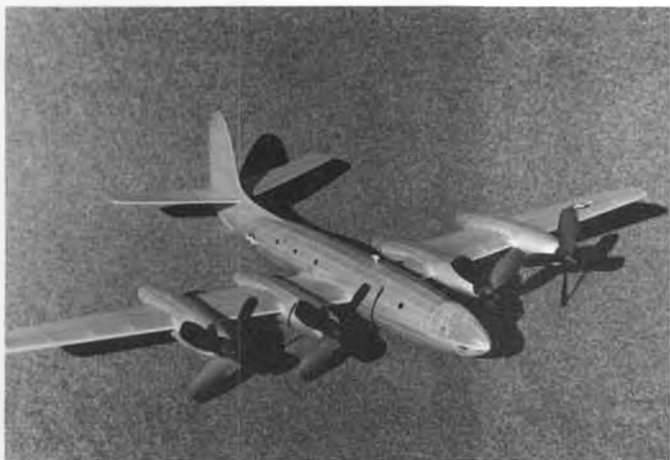
Republic Rainbow by Dick Howard weighs 65 grams and is powered by four rubber motors. Props are cottage cheese type.
