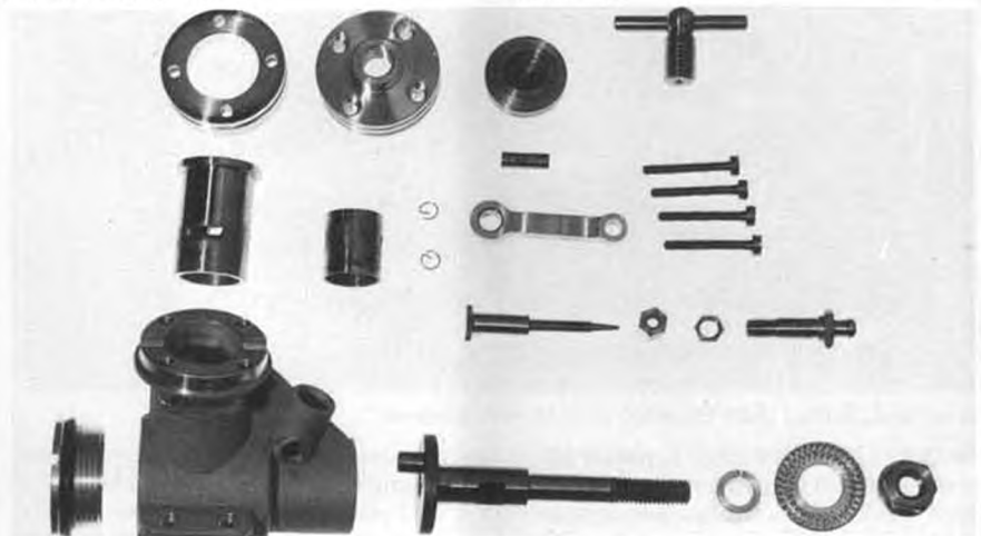
R-100 parts show chromed sleeve with conservative porting, 'O' ring rear crankcase seal, bushed con rod, deeply knurled prop drive washer, massive crankcase casting, square intake window and tapered split collet. Naturally weight is high for the displacement. Scramble event requires high crash resistant engines!
