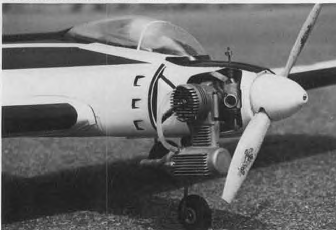
The Super Tigre S40 appears to have been shoehorned into the Invader.
