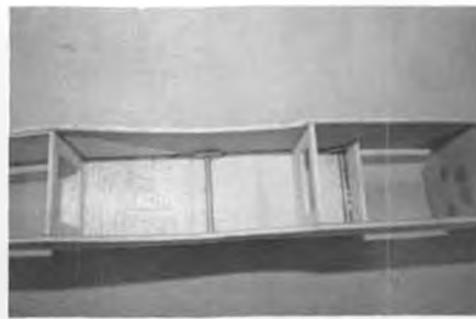
Inside of the fuselage. Note brass tubing epoxied in for cabane struts.
