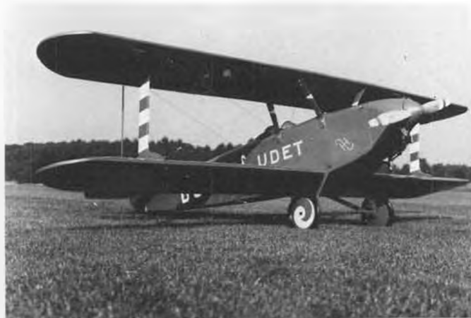
The Flamingo, powered by 2.2 chainsaw engine with gear reduction that turns 32x18 prop at about 2800 rpm.
