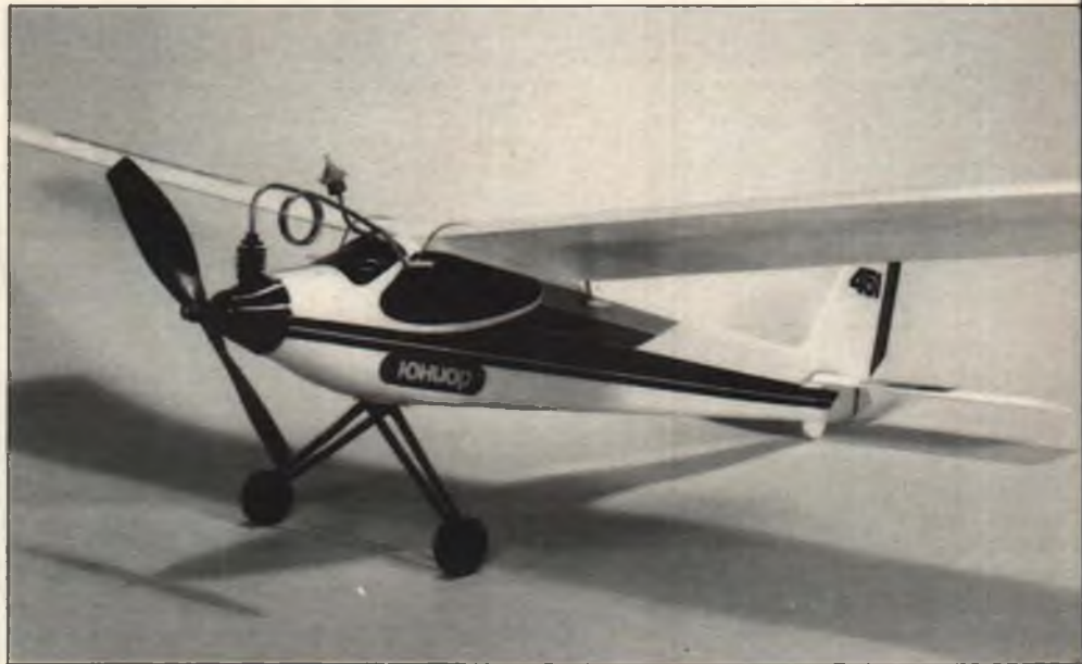
The Russian Polus CO 2 powered almost-ready-to-fly FF model from D&B Import/Export. The engine and accessories are also available separately, as described in the text.
