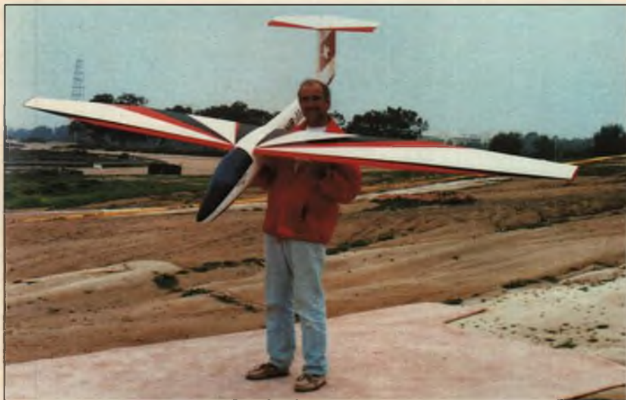
■ ABOVE: Victor Lanz of Carlsbad, California and his 1/4-scale Robergs Pilatus B4. Model spans 3.75 meters, or just over 12 feet. This is Victor's third exact same model B4—he really likes 'em! Weighs 12 pounds, has a modified Ritz #3 airfoil (semi-symmetrical) and is fully aerobatic. ■ RIGHT: Talk about the crowded sky! This was a typical scene during the weekend's activities. Full-scale sailplanes, paragliders, hang gliders and RC models shared the sky both days with no conflicts. City of La Jolla in the background.
