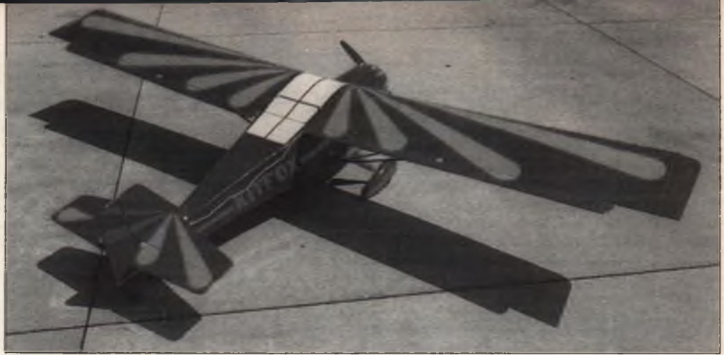
Author copied the colors and sunburst trim scheme of the original full-size aircraft. The only real deviation from scale was done for simplicity; the ailerons, instead of being the full-flying type suspended below the trailing edge of the wing as on the full-size ship, are instead hinged directly to the wing.
