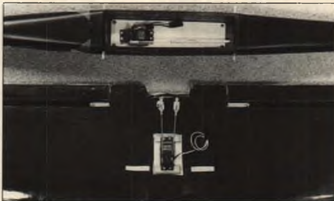
The elevator servo mounts on a plywood tray cut to fit the molded fuselage. The aileron servo mounts in the wing and is hooked to the ailerons via torque rods. Radio receiver and battery slide up into the nose when the servo tray is removed.
