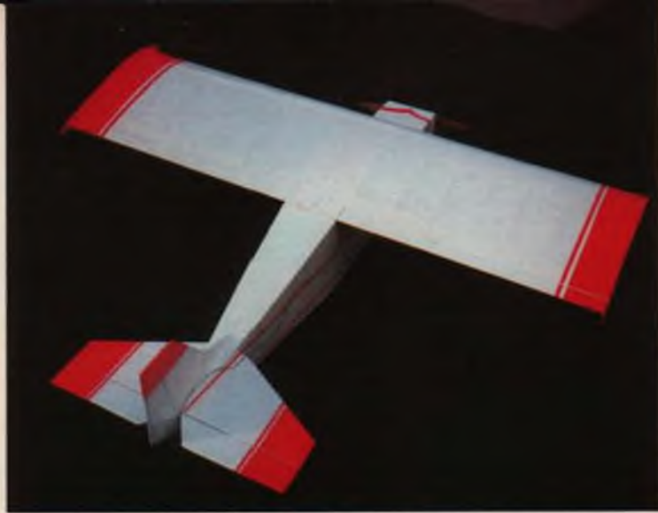
Roger's scratch-built 1/5-scale Lacey M-10 was inspired by the Peck-Polymers Peanut Scale kit. Model spans 48 inches and performs quite well with a geared Astro 15.
