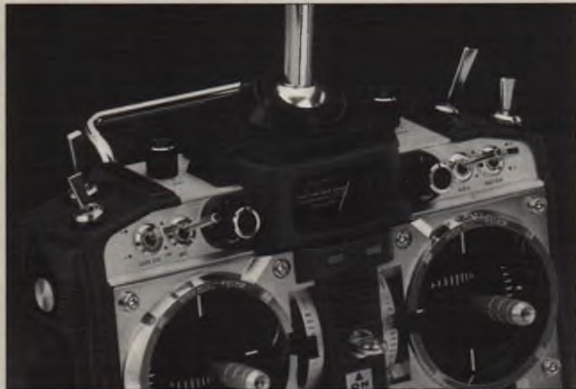
■ LEFT: This month James discusses the PCM-10S's dual rate switch settings. The Elev, Aile and Aux 2 switches can be seen here. James programs the "0" position to be high-rate and the "1" position to be low-rate. The Aux 2 switch is used for dual rate gyro. The Elev and Aile are shown in the high-rate position. Aux 2 is shown at the low-rate gyro position. ■ ABOVE: The top-of-the-line PCM-10S comes with the MER-D940S ZPCM receiver and five MES-4131 servos. The 4131 is a double ball bearing servo with coreless motor. These are used in the author's Concept 60. The less expensive seven-channel FM receiver and JR-507 servos are used in his Concept 30.
