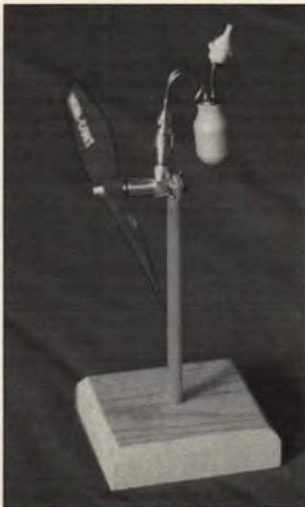
Soon to be marketed, this Werner Heise-designed Heibi CO 2 engine from Switzerland runs about three minutes per filling on the 3cc tank. Photo via Thomas Ogden.
