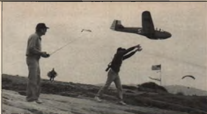
The father-and-son team of Fogel and Fogel launch their Schweizer TG-3, built from Model Aviation plans. Model features very simple rudder/elevator control but would really benefit from ailerons, according to Dr. Fogel.
