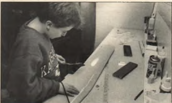
Lou covers the skinned wings with Coverite Black Baron Film to seal the structure and provide a base for colorful markings.
