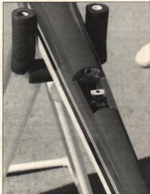
This is one way to get the weight out of the nose. The servos in Bob Crump's Typhoon are beneath a hatch in the rear fuselage. Rick Allison photo.
