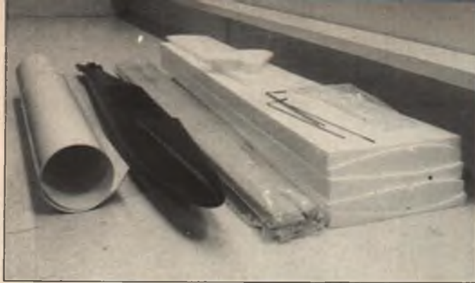
The Super Cheetah kit consists of foam cores for the wings, fin and stab; spruce spars, balsa leading and sub-trailing edge stock, aileron stock, rotationally molded cross-linked polyethylene fuselage (available in six different colors), "Kromekoat" wing sheeting material, and instructions.
