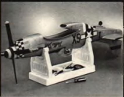
Soon to be marketed, this Werner Heise-designed Heibi CO 2 engine from Switzerland runs about three minutes per filling on the 3cc tank. Photo via Thomas Ogden.
