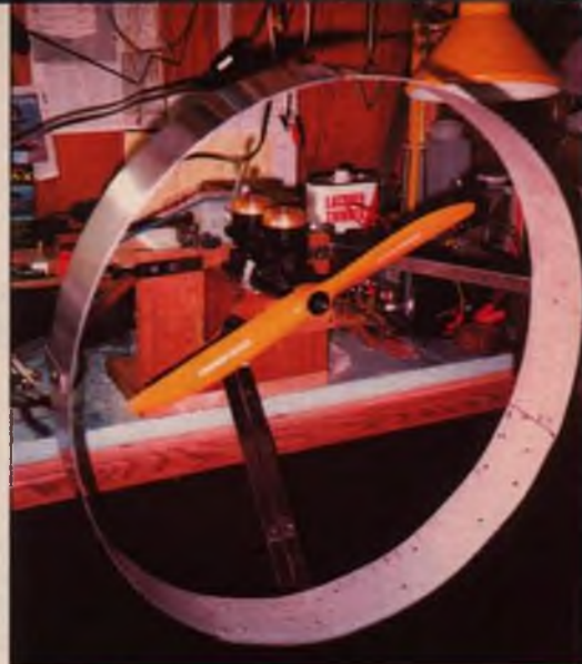
■ LEFT: Allan Poinsett flies this Megow Flying Quaker at night. It's equipped with running lights, two strobes and two wing-mounted landing lights. Molded ABS plastic floats are made by Stream Inc. Model was photographed at the 1993 Northwest Model Expo. ■ RIGHT: J.E. Boucher designed this simple aluminum shroud for some additional protection while bench running his engines. Keeps hands from inadvertently tangling with the prop while at the same time allowing easy access to all parts of the engine.
