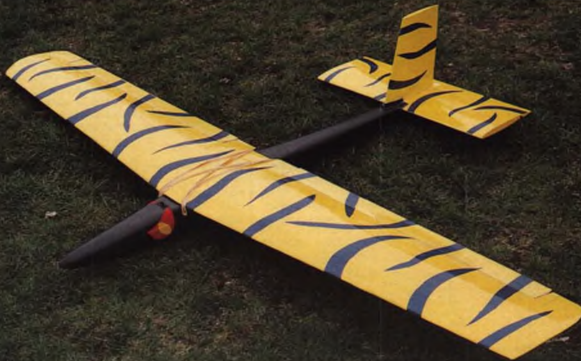
Completed Super Cheetah weighed in at just over 47 ounces with standard Futaba S148 servos and a 500-mAH battery pack aboard. Wing and tail surfaces were covered and trimmed with Coverite Black Baron film; shark mouth and eye markings on the fuselage were made with Sig Super Trim stick-on film. Photo by Dave Garwood.
