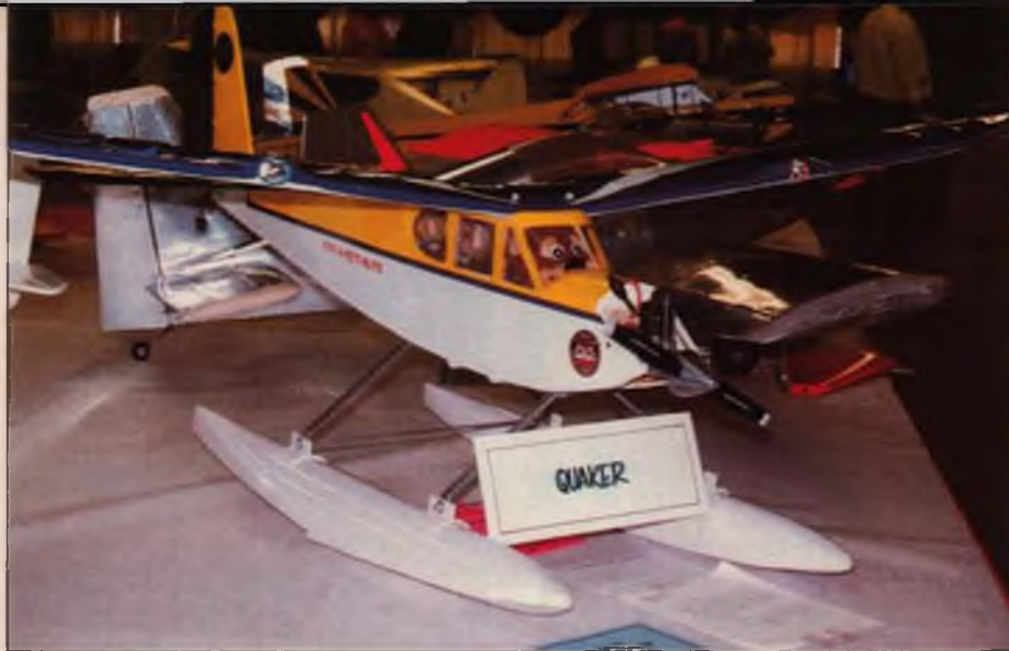
■ LEFT: Allan Poinsett flies this Megow Flying Quaker at night. It's equipped with running lights, two strobes and two wing-mounted landing lights. Molded ABS plastic floats are made by Stream Inc. Model was photographed at the 1993 Northwest Model Expo. ■ RIGHT: J.E. Boucher designed this simple aluminum shroud for some additional protection while bench running his engines. Keeps hands from inadvertently tangling with the prop while at the same time allowing easy access to all parts of the engine.
