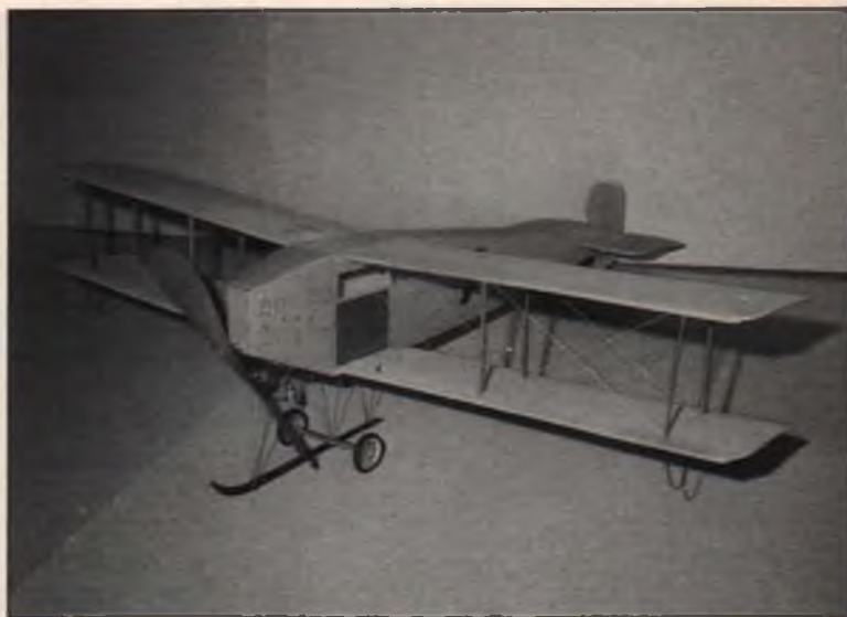
This 15-inch span Brown CO 2 powered Avro G was built by Al Backstrom, of Texas, from the July 1972 Model Builder centerspread plans.
