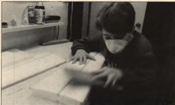
Leading edge and sub-trailing edge balsa stock are attached to the wing cores with Titebond aliphatic resin carpenter's glue. When dry, they are sanded down, blending them smoothly into the airfoil shape. A long sanding block with fresh sandpaper makes this a quick job.
