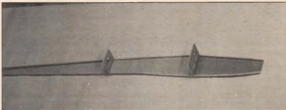
New fuselage formers F-2 and F-3 are made of 1/8 balsa with 1/64 plywood faces on both sides. Forward of F-2, the fuselage sides are doubled on the inside with 1/64 ply; between F-2 and F-3, doublers are vertical grain 1/16 sheet balsa.
