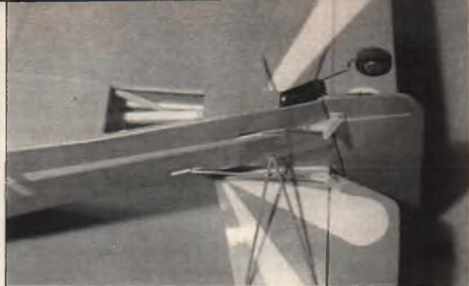
Underside view of the tail end reveals the cooling air outlet opening and clearly shows the stab support struts. These struts are functional—don't omit 'em! Note also how the tailwheel wire is cleverly connected to the rudder with a common cotter pin. Author used similar cotter pins for the wing strut connections as well.
