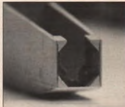
After the motor mount is permanently installed, the forward corners are filled in with triangular balsa blocks and will be carved to conform to the spinner.
