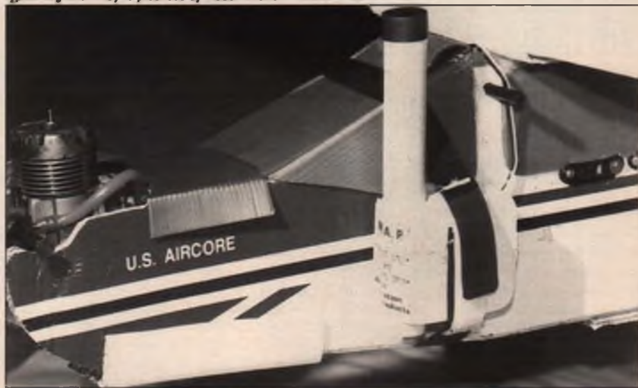
Duane Sanders' paint ball dropper is seen mounted on a U.S. AirCore plane. Several of these units could fit inside a typical Big Bird. They're produced by Model Aviation Products—see text.
