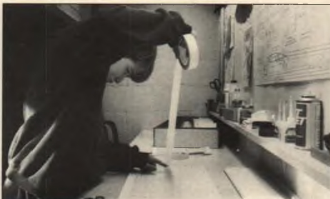
The recommended adhesive for attaching the KromeKoat wing skins to the foam cores is thin double-sided tape (available separately from Cheetah Models). It's plenty strong and easy to use for less-experienced foam wing builders. "KromeKoat" is .010-inch thick—.008 on the tail surfaces—white card stock with a shiny surface, and makes for an extremely durable model.
