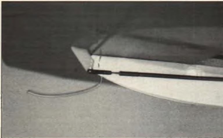
A steerable tailskid, such as that used by the author on his lightweight fun-fly design, can be simple, light and very effective. Design features are discussed in text.
