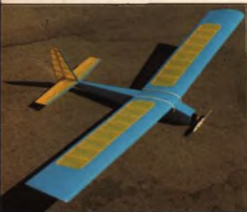
The "Toot-E" is the author's electric conversion of Jim Bigley's "Tooter," a 66-inch span, .10-powered motorglider. Model has a direct-drive Astro 05 and except for the wing leading edge and the elimination of a plywood bulkhead, is built completely according to the original plan.
