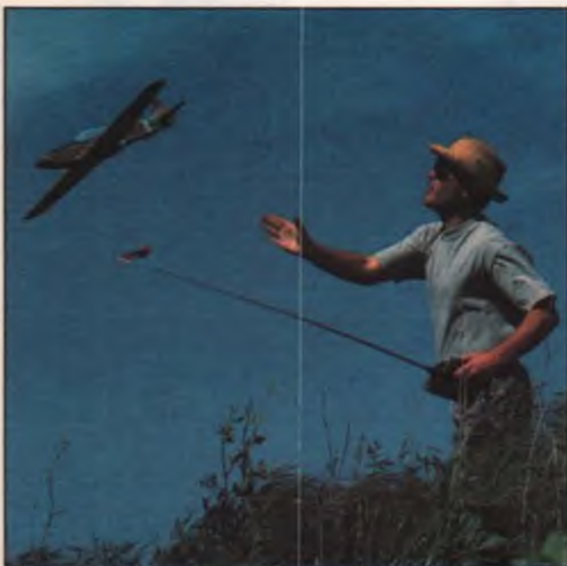
LEFT: We met up with Dave Sanders at a local slope and took this shot of him launching his own Ki-61. Unlike the lightweight film-covered versions, this one has been glassed and painted and weighs 22 ounces. Note how Dave is careful to keep the nose down until the little ship has built up a good head of steam. RIGHT: Despite their small size, these models have enough room inside for standard-size radio gear. Dennis wanted a lightweight model, so he installed Hitec RCD micro equipment—a 535 receiver, HS-80 servo for the elevator, and two of the new super-micro HS-60 servos for the ailerons, electronically mixed for spoileron control. All-up weight even with a 500-mAH battery aboard is only 14 ounces.
