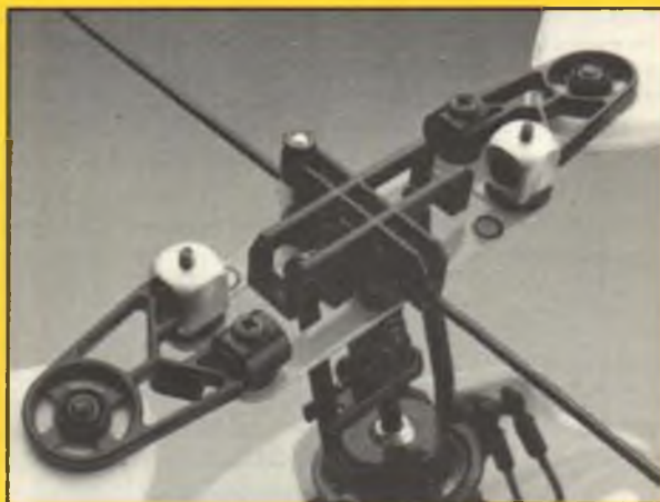
Just before going to press we learned that Great Planes, U.S. distributor of the HyperFly and other Kyosho products, is now offering a HyperFly Adjustable Pitch Kit, a $18.00 option that makes for easier and more precise pitch adjustments. The kit replaces the HyperFly's stock loading blade grip holder with an aluminum unit that incorporates a rubber governor and hex-socket screw. Pitch adjustments are easily made with a hex wrench or ball driver, as opposed to twisting or adding shims. All parts, instructions and a blade pitch gauge are included.
