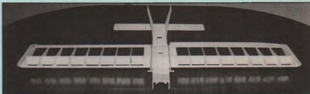
All framed up and ready to cover—total airframe weight is about 5.5 ounces at this point. Note how the two fins angle outward at the top.
