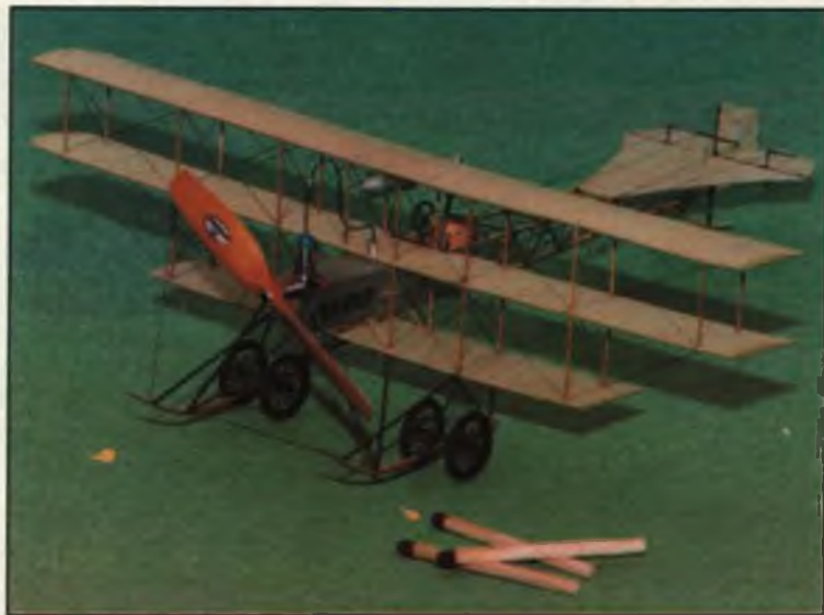
Frantisek Barta, of the Czech Republic, created this intricate Pistachio AVRO IV triplane, powered by Stefan Gasparin's jewel-like G5 CO 2 powerplant. Model features movable controls and shock-absorbing landing gear. At least three Model Builder advertisers market the Gasparin motors. In case you may care to try your hand at miniature powered flight.
