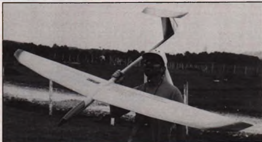
■ RIGHT: A member of the U.S. contingent and a top-rated pilot, Fred Mallett studies the sky prior to launch. Fred's plane, the Esteem, produced by Inventive, is a super-lightweight T-tail design featuring obochi-sheathed foam wings, voided fiberglass fuselage and T-tail. Columnist Forrey is gathering info on this hot new ship for a future column. Fred placed 3rd in the competition.
