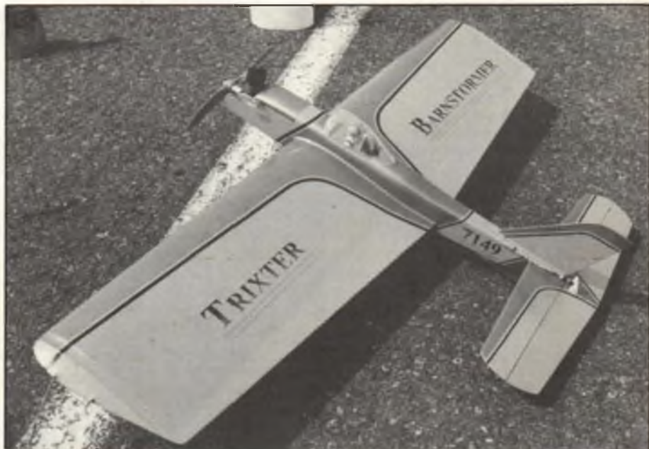
One of the more popular designs for Old Time Stunt is the Trixter Barnstormer, originally kitted by Gullflow. This one's powered by the venerable McCoy Red Head stunt engine.
