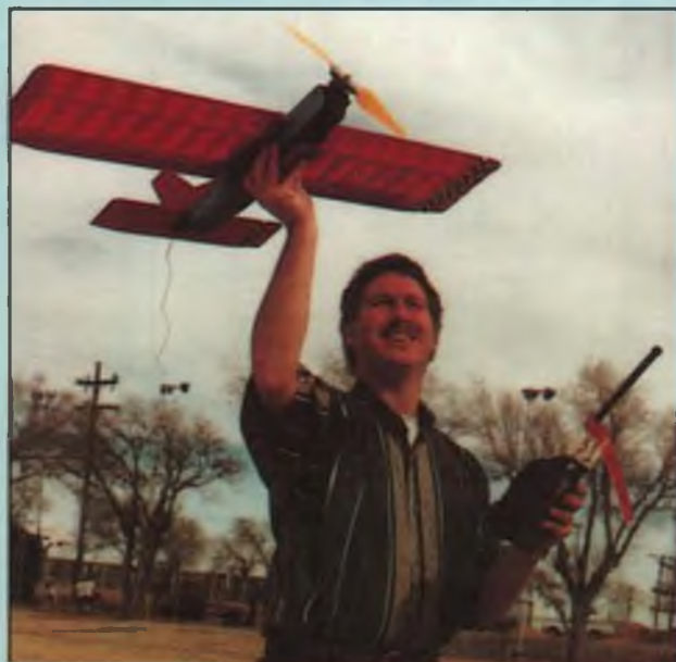
Designer Scott Hartman strikes a launch pose for photographer Don Rice. Scott recommends a fairly steep nose-up angle for launch, as the model will tend to bobble until it picks up enough speed to get "on step."
