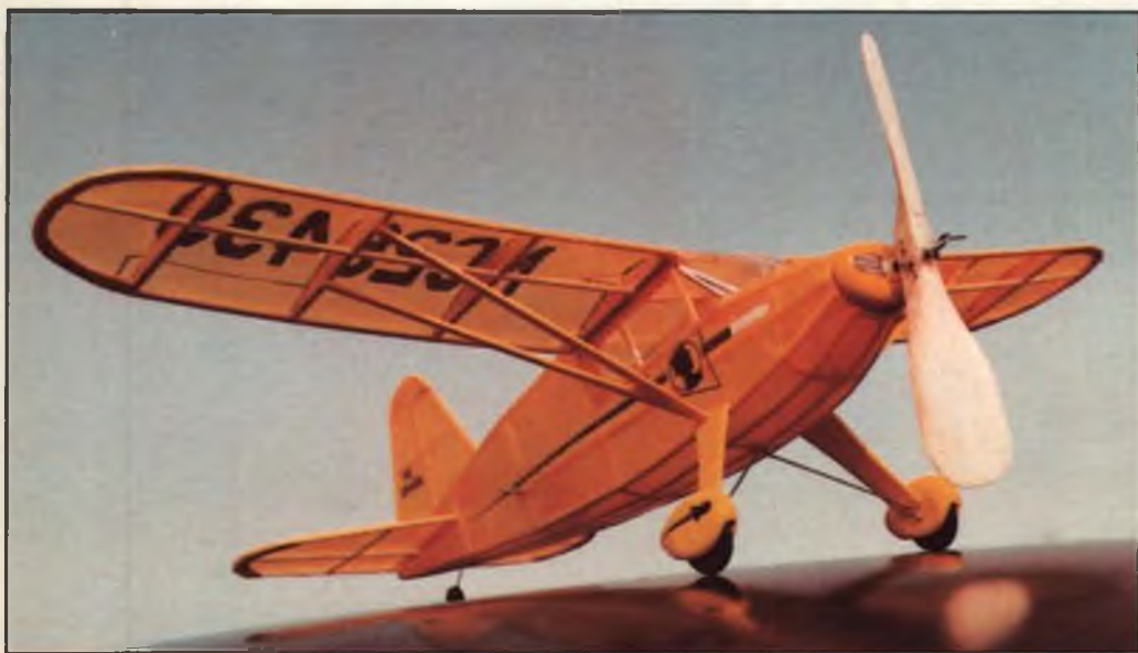
Mark Fineman's Cornet III Stinson features unusual Charlie McCarthy markings, as explained in the text. Note single-surface tissue covering, which was typical of early 10c models.
