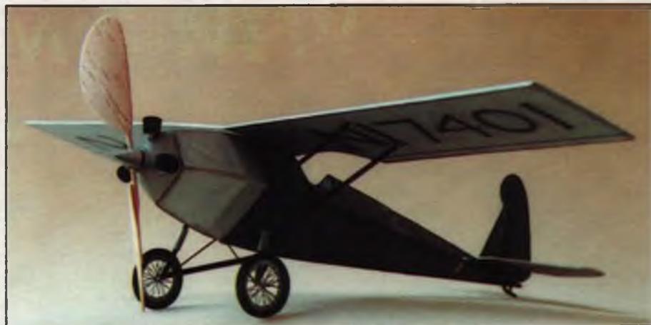
This angle illustrates the diamond-shaped fuselage that is the trademark of Prest designs. Details on making those great looking spoked wheels are contained in an illustrated booklet available for $10 from the author; write to Stan Fink, 1810 Pine St., Philadelphia, PA 19103.
