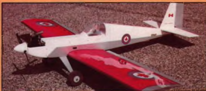
In the February '93 "Plane Talk" column we ran these photos of Jim Stevens' "kit bashed" Bingo, in which he designed his own set of biplane wings and can switch from monoplane to biplane and back in a matter of minutes. On the biplane version, the wire cage fastens to the sides of the fuselage with nylon bolts; no interplane struts are used. Shows what you can do with a little ingenuity. Creative Bingo 40 builders might want to do something similar.
