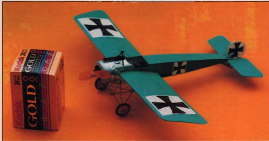
Another of Frantisek Barta's fabulous miniatures is this Pistachio-size Gasparin GS CO 2 powered Folder Eindecker, which weighs only a bit over 8 grams and has an indoor flight duration of more than 50 seconds. Otakar Salbek photograph, via Fritz Mueller.
