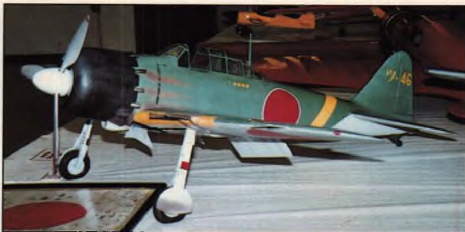
Bob Benjamin took 1st place in electric scale with this Platt Zero, powered by a geared Astro 90 running on 36 1800-mAH cells.
