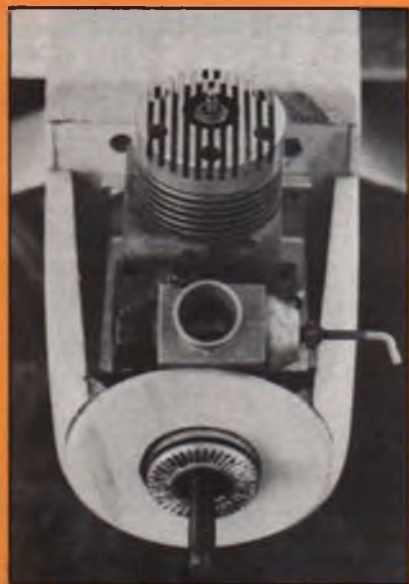
K&B .40 installation in the Bingo's nose. Covering is built up of balsa blocks, carved to shape.
