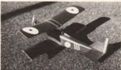
No. 6782 VEST POCKET SESA $6.50 For pulse rudder RC, this 22-inch span bug uses Cox .020 Pee Wee. By Fred Angel.
