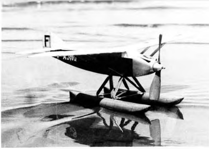
Walt Mooney's LAT 283. Float tops are single balsa sheet molded over form. Excellent takeoffs.
