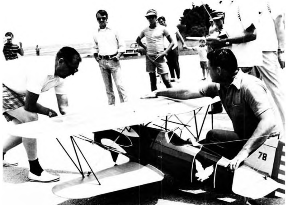
Tom Gardner, Titusville, Fla. (left) built this P-6E. Power is a 1.4 cu. in. Cox chain saw motor with Korbo mods. Lack of power has prevented flight of this 28 lb. beast. We'll keep you posted.
