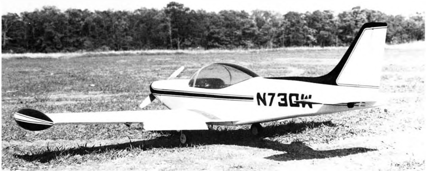
Walt Moucha's latest scale ship is this 2"=1' Waco Meteor. Webra 61, Goldberg retracts, flaps, 8-3/4 lbs., RS Systems radio. Model already has a 1st and a 4th place win in scale events. Finish is K & B Super Pox. Flies fast.
