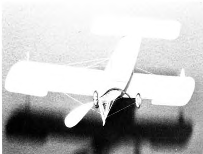
Underside shot of the Bleriot displays the leaf-spring landing gear. Prop would have to be shortened for R.O.G. flights.
