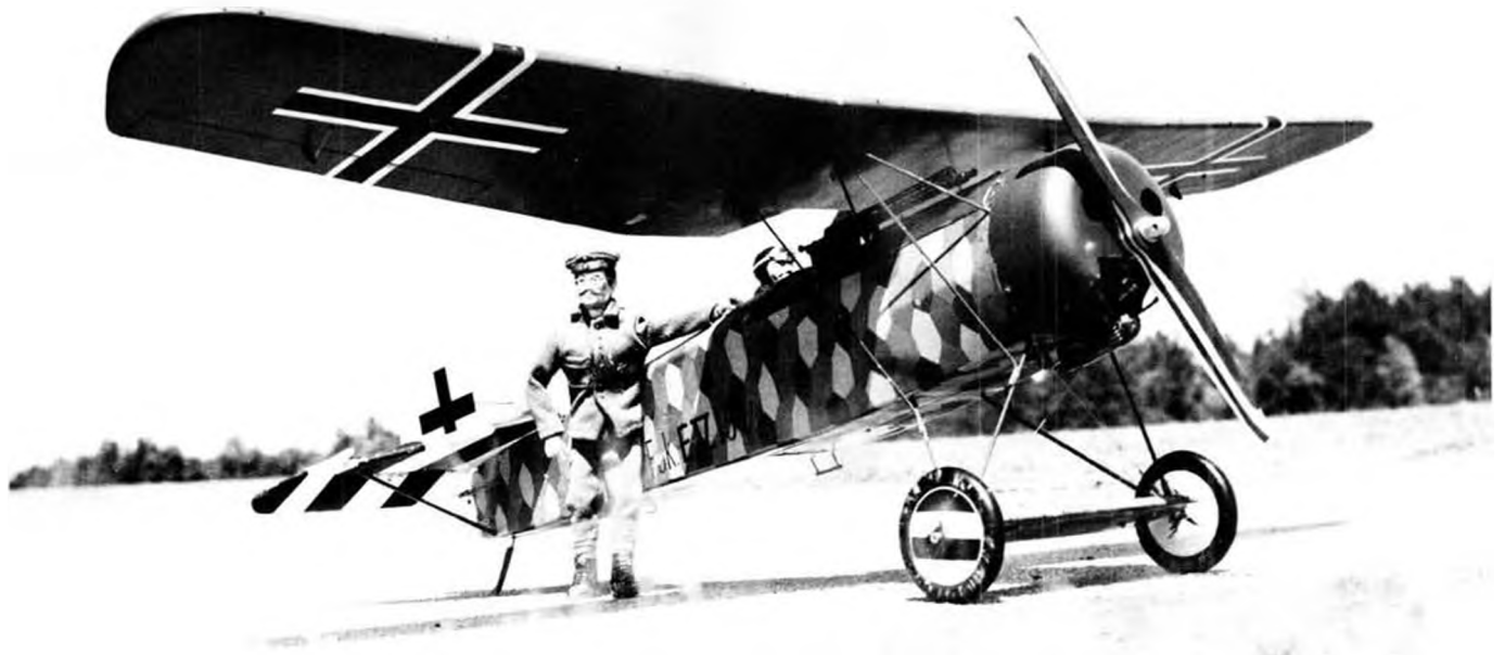
"Good grief, Emily, Teddy's gone over to the other side!" This Wankel powered Fokker E-V was built from a Schuco-Hegi kit. Ship is flown R.E.M., with the 4th channel dropping boots and scarf on Allied Aerodromes! Heath radio. Finish is silk and dope, Monokote, and Solarfilm. "Flying Razor" was built by Col. John Wormley, weighs 4-1/2 lbs. and is good flyer, with excellent glide.
