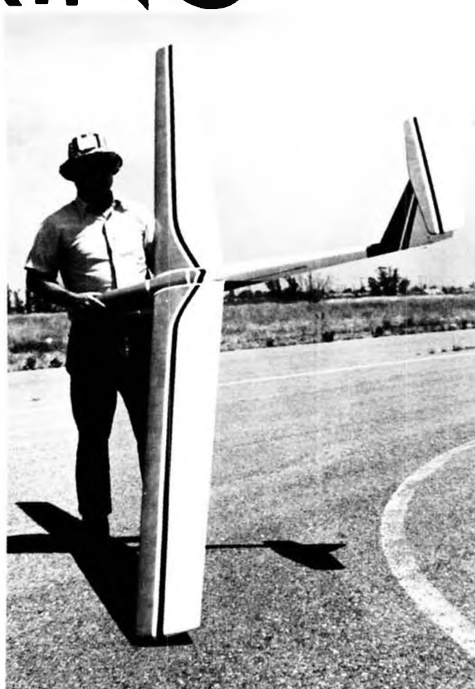
Glen Cunningham's beautiful T-tail original is all balsa construction. Tow ring jammed once . . . he had 3-1/2 minute flight while hooked!
