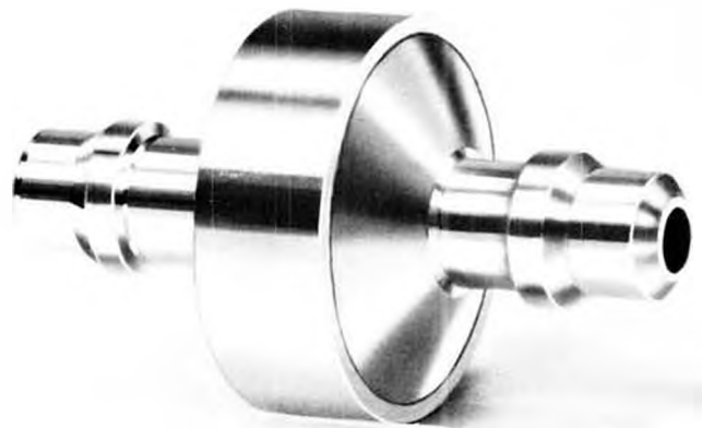
New in-line fuel filter by Perry Automotive. Sealed unit is cleaned by reverse flushing. Filter element is polypropylene.
