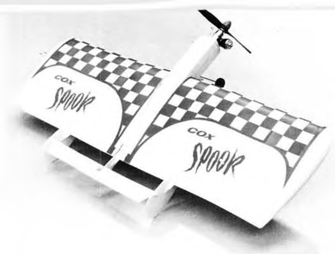
All-plastic 1/2A stunt kit by Cox. Real performer on 40' of .008 braided lines and the Cox 290 engine. (See text)
