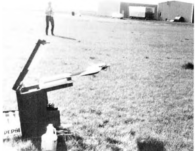
Interesting self-launching rig by Steve Fauble; great for combat types. Foam holds wings, spring released by pilot. Near-future MB article.
