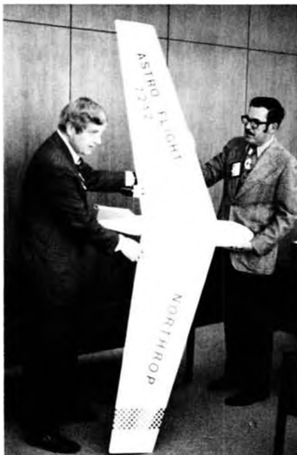
RPV designed and built by Astro Flight, Bob Boucher on right. Uses two electric motors.
