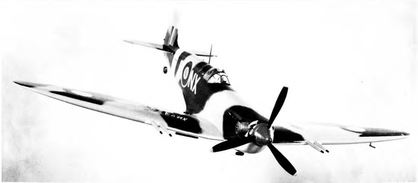
This Spitfire is built from the kit by Royal Products Corp. At 1-3/4"=1' scale, the wingspan is 64-1/2", length 52-1/8". Ship is of all balsa construction and is for .60 to .80 size engines.
