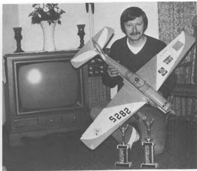
Midwest foam Chipmunk, by Bill Mohrbacher, Beaver Falls, Pa. has Fox .19 power, Heath GD-19 radio, Sig Plastinamel finish.
