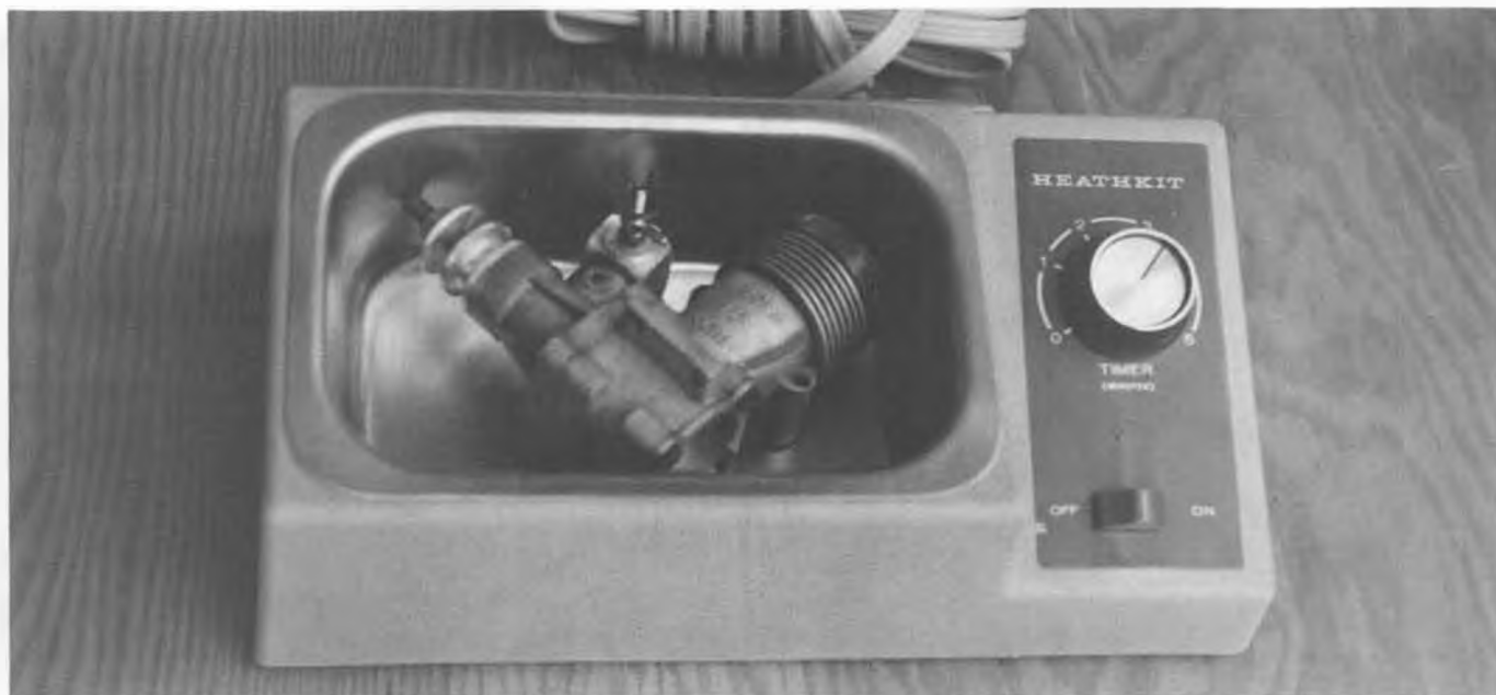
The completed Heathkit GD-1150 Ultrasonic Cleaner. A Webra Blackhead .61 R/C rests in the stainless steel tank to indicate capacity.
