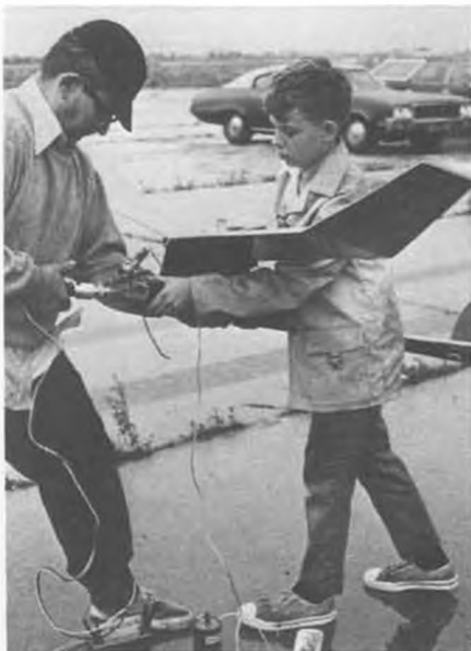
Joe and Wayne Friebus demonstrate use of electric starter to give engine a kick. An extremely useful tool for the free flyer, especially if he's using a pacifier system.
