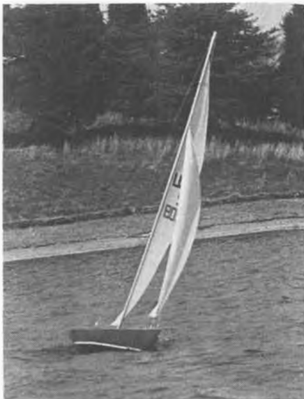
Here is an East Coast 12 trying to go to windward. Her booms appear to be set properly, but in each case, more downward tension is required of the main sheets to take the twist out of the sail. Top of the main has twisted out so far that she is already luffing, and it's sure that the boat could point 20° closer to the wind with increased sheet tensions. Also, jib club swivel needs to be moved aft on the club to help tighten the jib leach.
