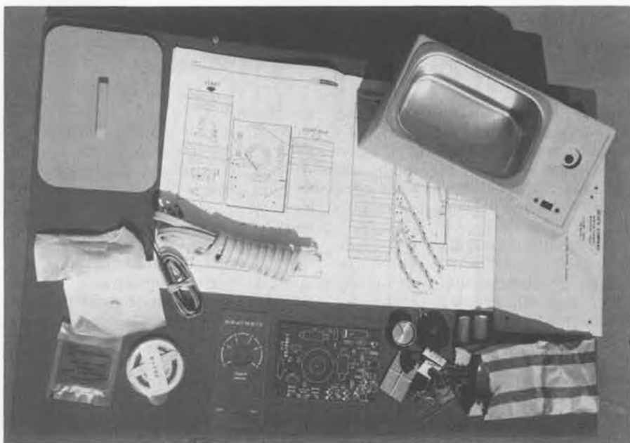
Ultrasonic cleaner parts spread out before the project was started. Actual working time to finish assembly of the kit was under two hours. Wives will like the way it cleans jewelry.
