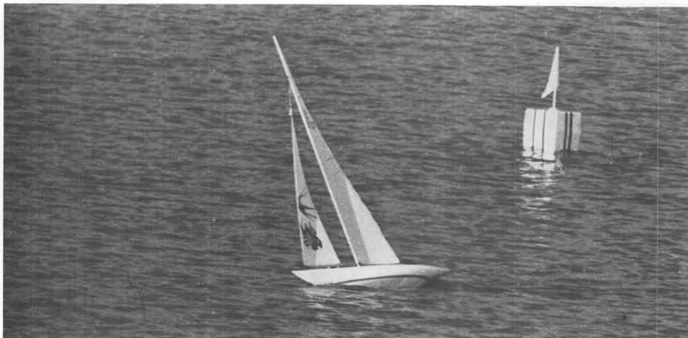
A well trimmed EC/12, No. 37 was the winner of the 1971 ACCR for that class. The sails look as if they are working together, the slot is open, and there is little twist allowed on this light air beat, in order that the boat points high and yet stays moving. Though one of the earliest boats in the class, this hull continues to be a potent threat on regatta day!!
