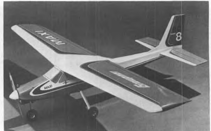
The "Maxi" is an advanced trainer, which can be flown with or without ailerons. Span is 63, powered by .40 engine. Graupner kit.
