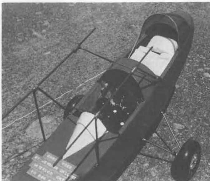
Though cockpits have been left open, Chris says no exhaust residue gets in. Pilot and passenger on hatch/floors could be added.
