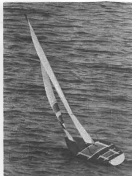
This Flying Eagle 50/800 shows good form going to weather. The twist induced in the main was done on purpose to allow some air to spill from the main head and reduce the heel on this tender hull. Note that the lower batten is parallel to the boat centerline. Also, curve of both leeches seem to follow one another, and not close the slot excessively. Only suggestion would be to slacken off the foot outhaul to let a little more camber develop in the foot of the jib.
