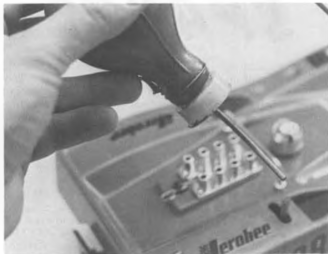
Allowing the fuel fill line to protrude through the car body permits you to make fast pit stops.
