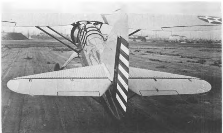
Tail-on shot shows the canopy to fin fairing. LH elevator was flipped over and used on right side, was identical except for drain holes. Trim tab control on bottom left, top right. Note square cars!
