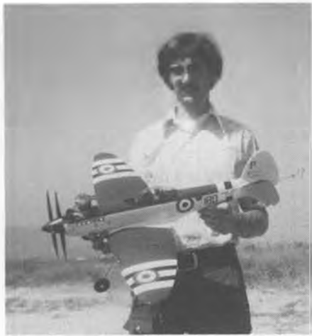
John Swift and magnificent Sea Fire AMA carrier. Veco 61R/C, 49 oz., throttle, flaps.
