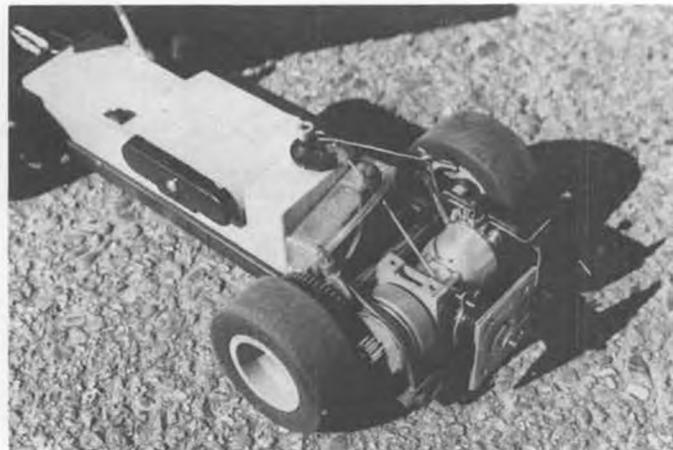
Another heat sink arrangement. Note also the fuel tank and brake band.
