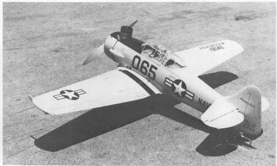
The center throttle wire through the wing is obvious in the photo. Sig kit decals are excellent.
