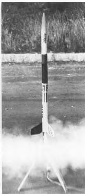
Modified Estes Patriot. Extra tube and FSI D20 engine. At Rochester Rocket Soc. field.
