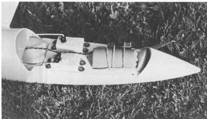
Radio installation in W-21. Note that control tubes appear to be built into fuselage shell.
