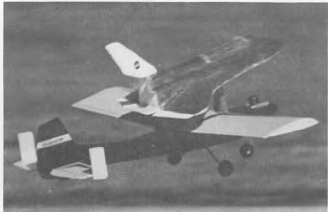
Carrier and Orbiter at takeoff. Scale model 747 has since been built for more accurate simulation of separation tests.
