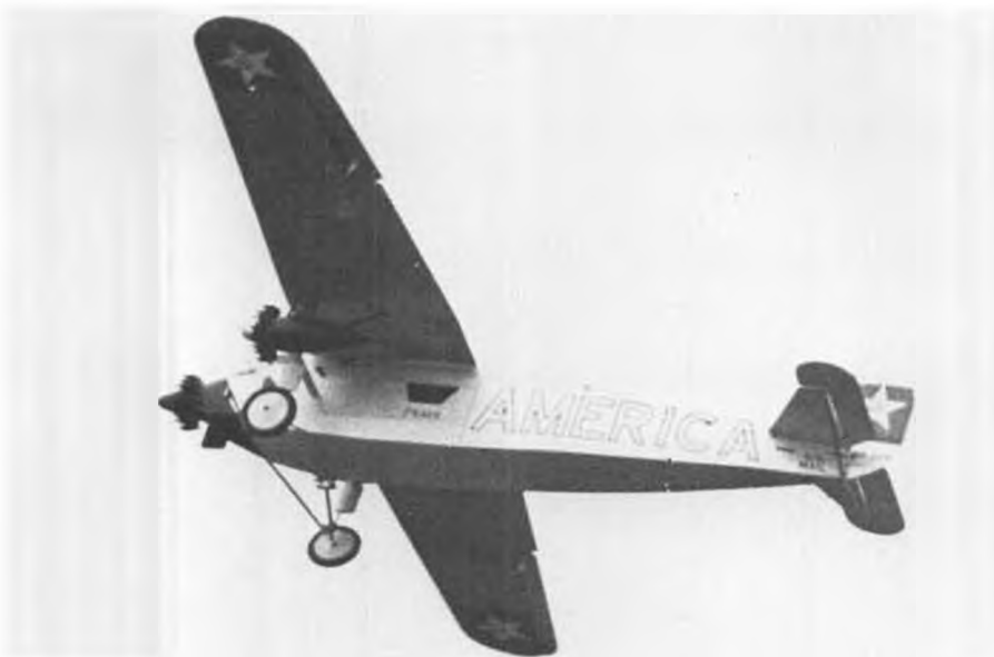
The Fokker rumbles overhead after takeoff. Long tail moment makes up for the small surface area of the horizontal and vertical stabilizers.
