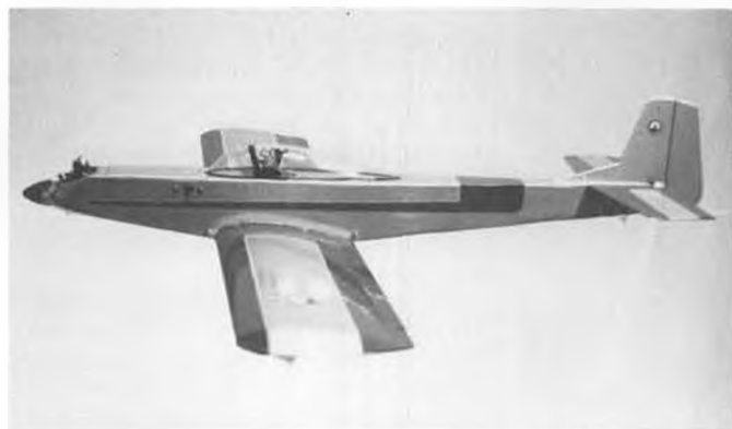
GMC's Half-A Chaos (Kaos?) has been modified with Sig canopy and starlight Ace wing, to look like Quick Fly. Aileron and elevator.
