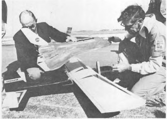
The Orbiter model being fitted to the pylon attachment system. Both models ballasted to simulate actual vehicle loads.
