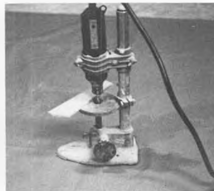
Dremel tool set-up for cutting grooves for 1/64 plywood inserts in sheet tail surfaces.
