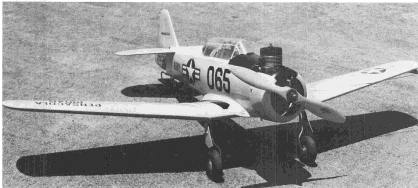
Wings of the modified Sig kit T-6/SNJ are sheeted with 1/16 balsa, replacing the silkspan provided. A Testor's .35 engine is a neat fit in the cowl.
