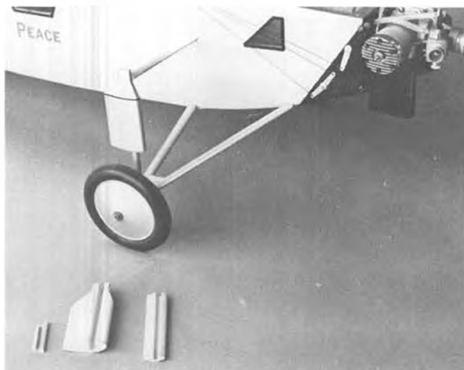
Strut fairing construction is shown. Also note exhaust extension and prop shaft extension.
