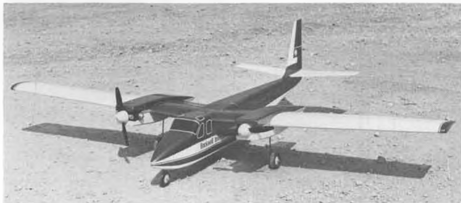
Ace R/C's 48 inch span Aero Commander for 3-channel radio and two .049/.051 Tee Dees. Foam wings. $29.95.
