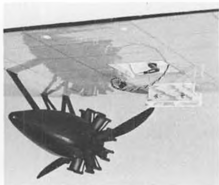
Underside of center section. Plywood wing retainer fits under notch in top of main cabin.
