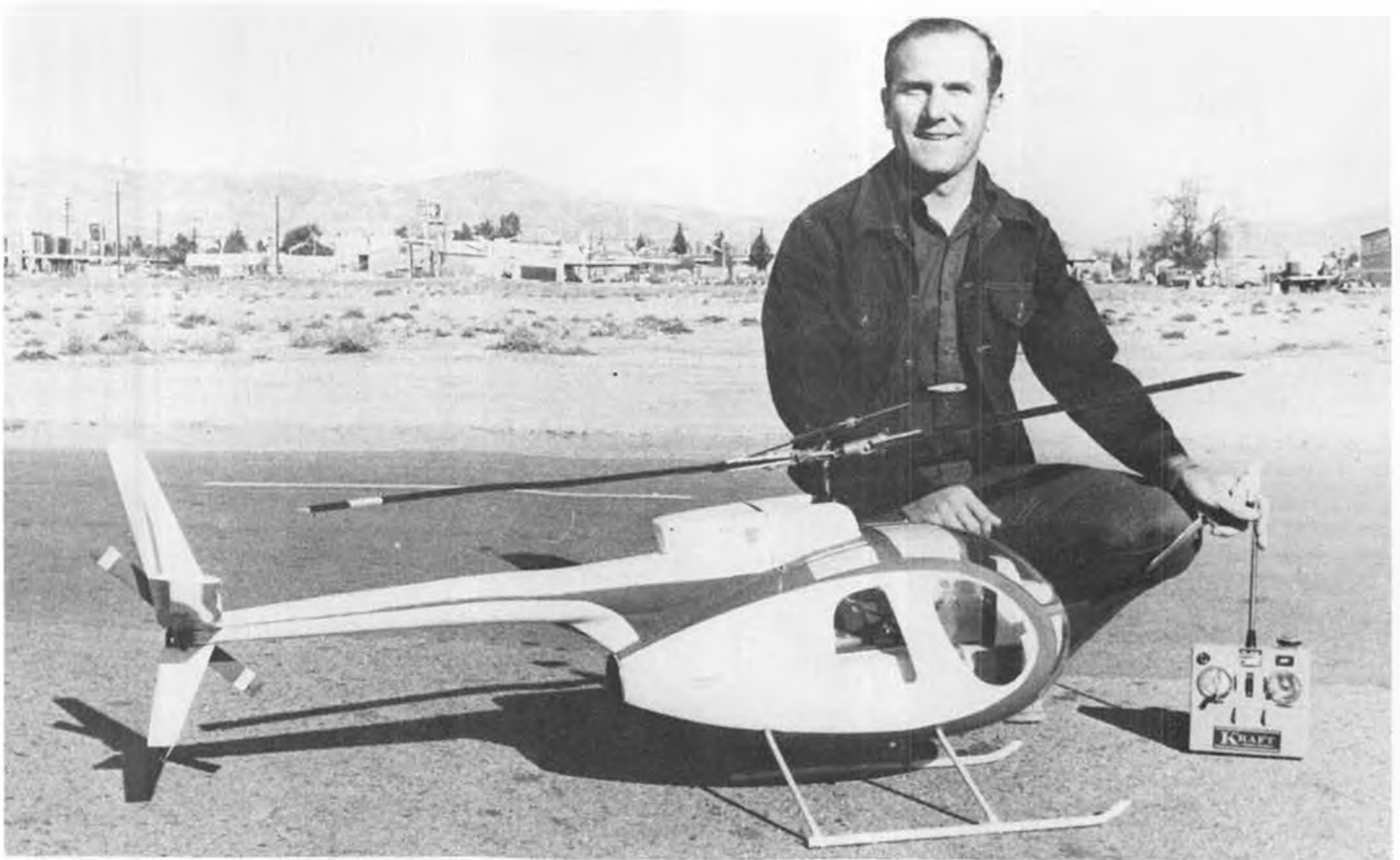
John Minasian (of Helicopters Anonymous), and his Hughes 500 chopper. John installed Kavan Jet Ranger mechanics in this fuselage shell that was originally molded in fiberglass by Charlie Gilbert. Charlie had dropped the project to develop his successful electric chopper.
