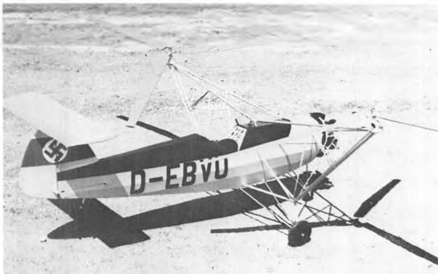
Skip Ruff's full-scale Focke-Achgelis 61 helicopter actually operates as an autogyro, and very well at that. Weight 4 pounds, OS .35, 3-channel, 37 inch rotor diameter.
