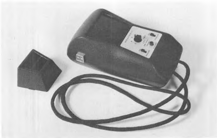
Heathkit Delux Digital Stopwatch. Sun shield is clipped over read-out window for use in bright sunlight. Unit is powered by 6 rechargeable nickel-cadmium pen-cells.
