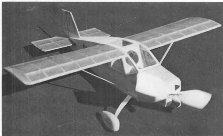
Couldn't be simpler . . . a box fuselage, and straight-edged surfaces. It's obvious the designer had good visibility in mind when he drew this one up.
