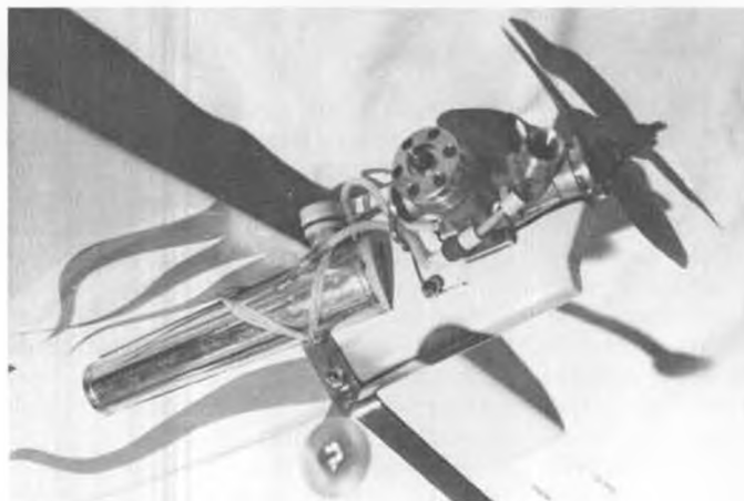
General view of engine/shut-off/tank arrangement. Avoid complicated set-ups. Simplicity is next to reliability . . . and that wins races!
