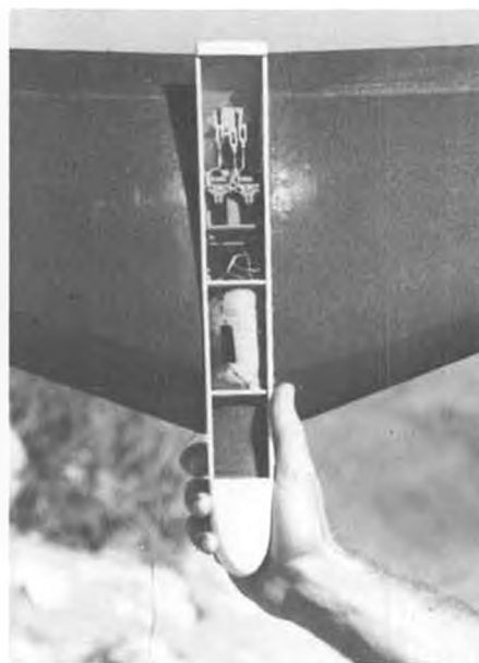
Snug radio installation in glider version uses two-servo brick and 225 mah battery.
