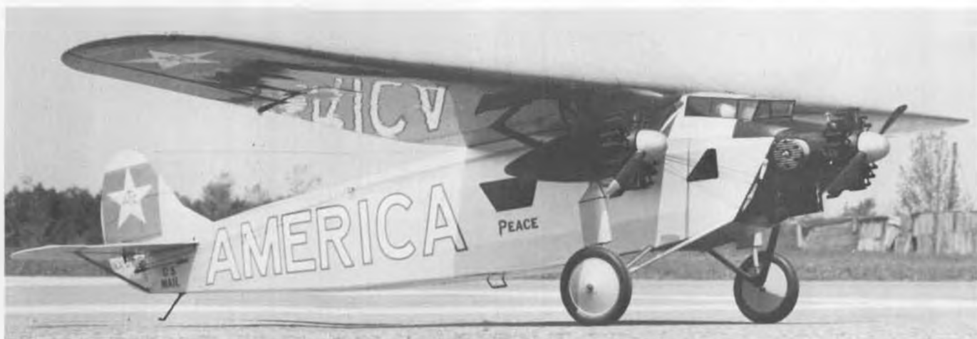
The "give-away" side of the Fokker, showing the head of the OS .40 engine in the nose. Of course, the outboard engines are dummies, with the scale-like props being allowed to free-wheel. High pitch on these reduces drag. Note external control cables (scale only).
