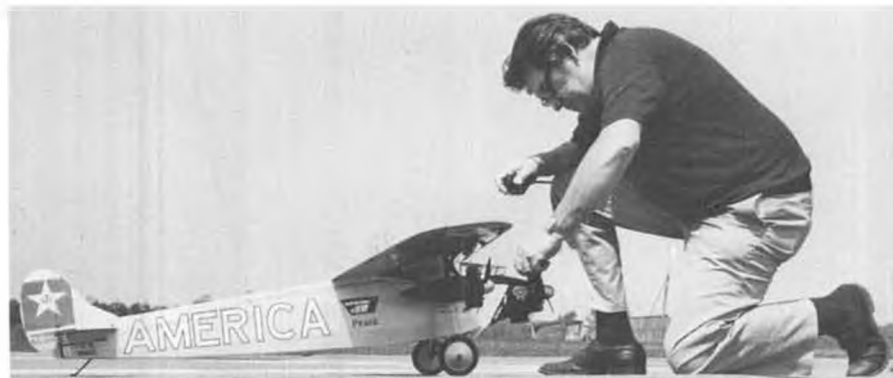
Author/designer George Clapp preps the OS engine for flight. Note pushrod showing through aft cabin window.
