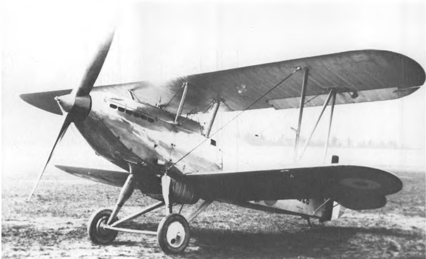
K1926 was the first of 117 production Mk I's. It was tested extensively at Martlesham Heath, the Wright Field of the RAF. Incidence wires were replaced by 'N' cabanes on later production models.
