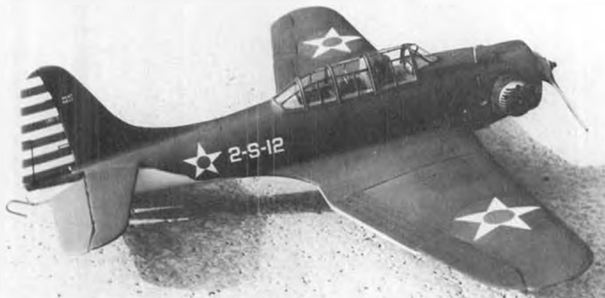
Another view of the author's "Dauntless", showing neat cowling of the engine. Split flaps can be made operational, adding much to realism of model.
