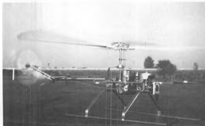
Dr. Emery "Lee" Wayman's Moody helicopter in flight, without body. Note heat sink and muffler on forward-placed engine.
