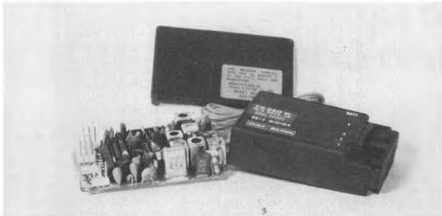
Cox/Sanwa receiver with sturdy case removed. Surprisingly, no IC's are used. Components are grouped in packages that appear to be IC's. PC board is of the strong, plated-through type.
