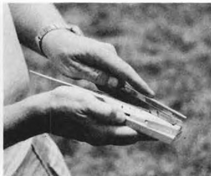
Art Arro shows his jig for reworking Form 1 props. Cut on left determines blade length and tip angle, while second cut controls blade shape and area. Once set, every prop will be the same.
