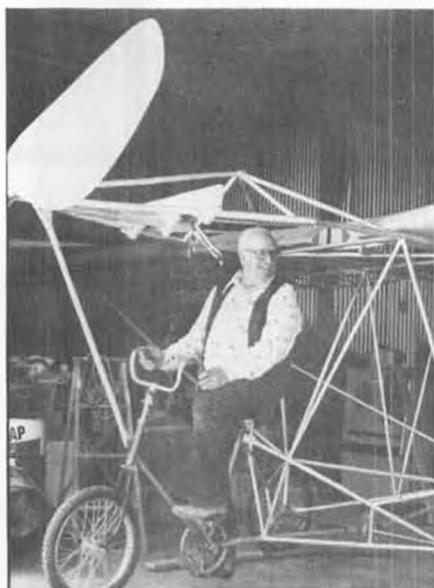
Clyde D. (Daring) Goehring at the power/control center of his MP aircraft described last mo.
