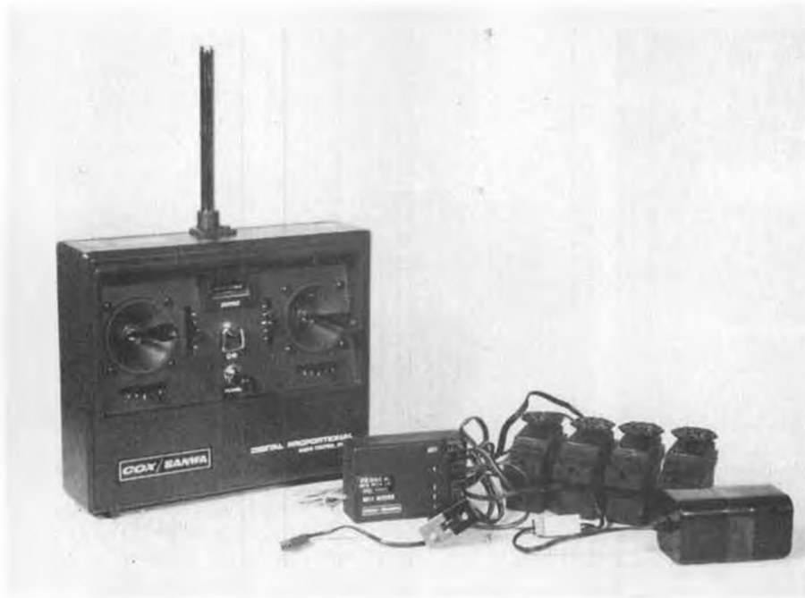
The Cox/Sanwa 4-channel radio system as reviewed by Eloy Marez. Long servo leads (10") plug directly into receiver. An extension lead is provided for aileron connection. On-off switch locks.
