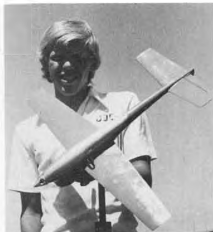
Joe Kall and his record-holding (153 mph . . . proto speed) Formula 40 . . . 3/4 pan, inverted K&B 40, "V" stab. Flies clockwise (standard in the southern hemisphere, but unusual here).
