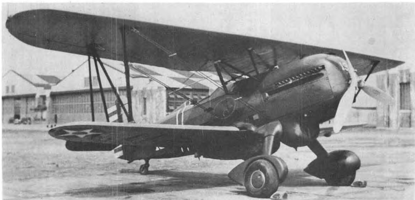
Insignia on this P-6E is of the 33rd Pursuit Squadron, which flew out of Langley Field, Virginia. Half-pants on low pressure tires were a service modification to enable caked mud to be hosed out. No, Mabel, they didn't have many paved runways in those days!
