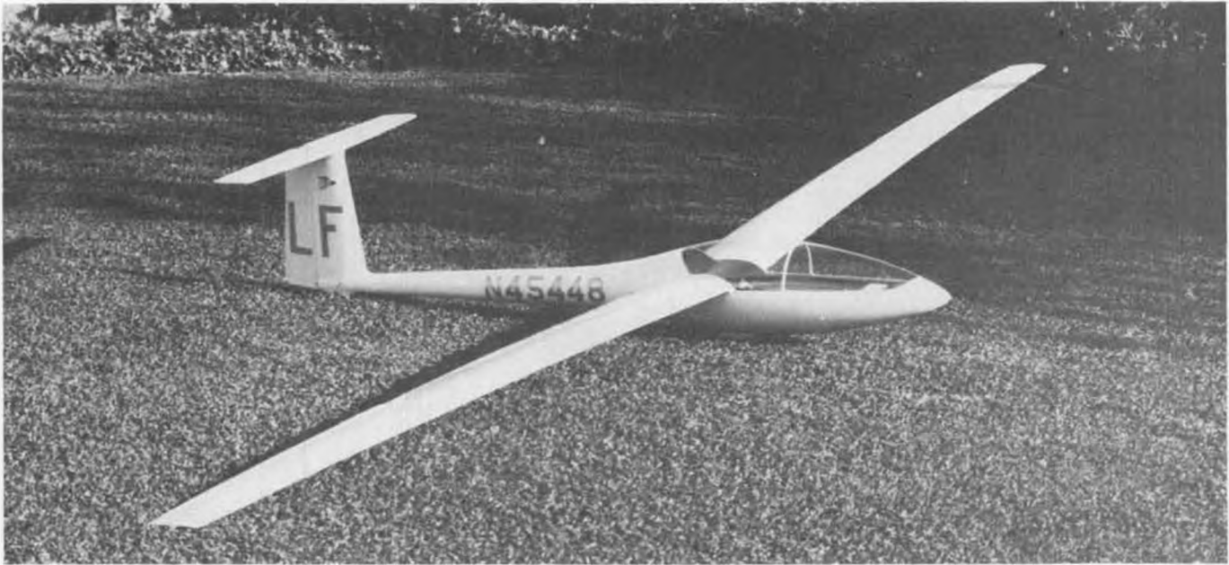
The author's beautiful quarter-scale Kestrel 17, built from Ralph Learmont kit. Span is 14 feet, and the weight, with retracting wheel, is 8 pounds.
