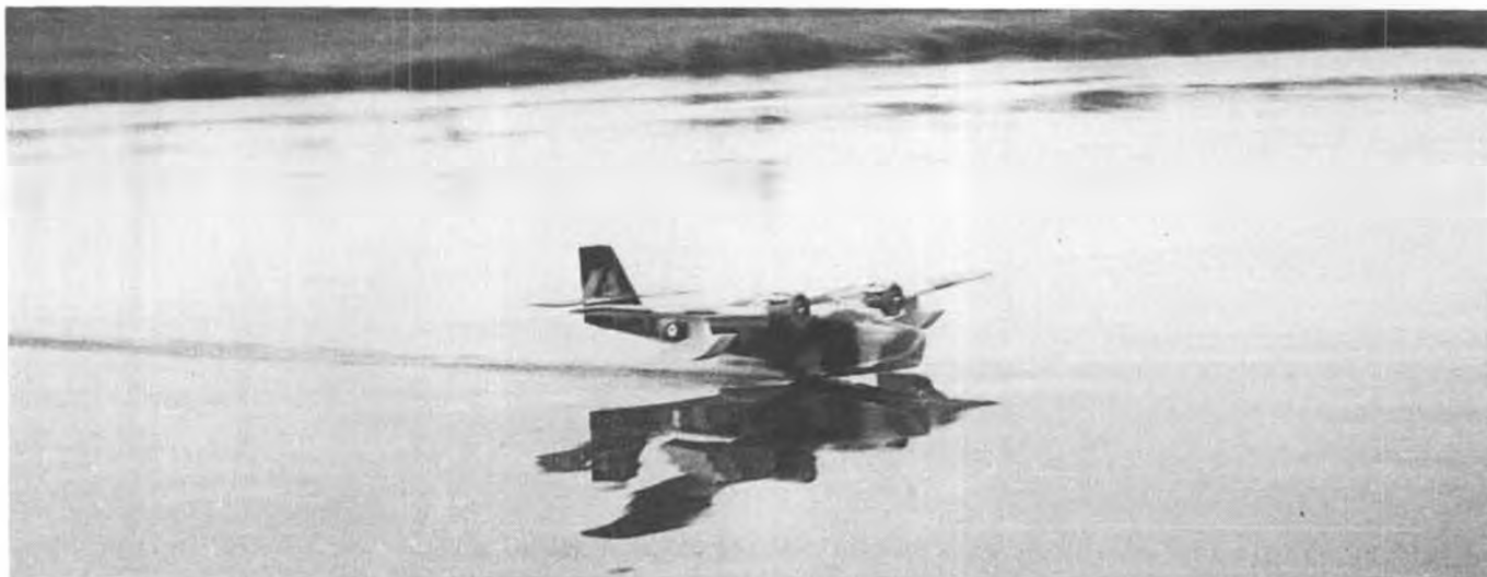
Cleopatra in full flight, with just the aft point of the forward step cutting a small track in the smooth water. A touch of up elevator and it will become completely airborne. Twin OS .40's give plenty of takeoff power for the 8 foot span flying boat.
