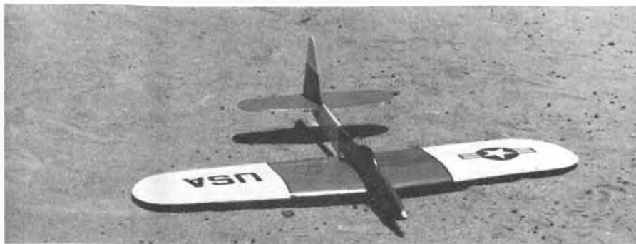
Kirt Hanson's profile C/L P-63 which he converted to R/C slope soarer for pylon racing. Battery is mounted in the nose, while all other R/C gear is in the wing.
