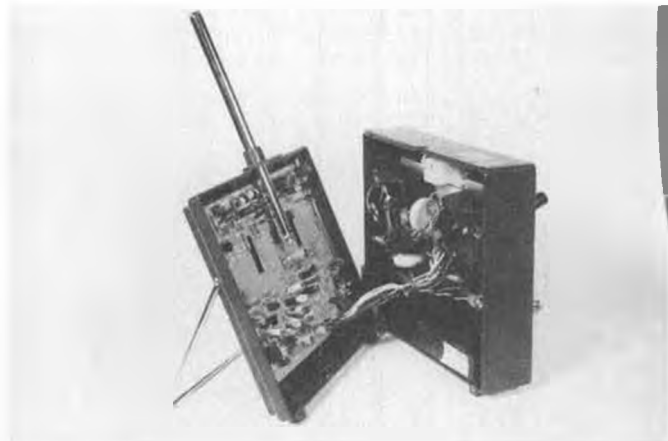
Transmitter case opened up, with the stick assemblies on the right, and the single PC board with all electronics on the left.
