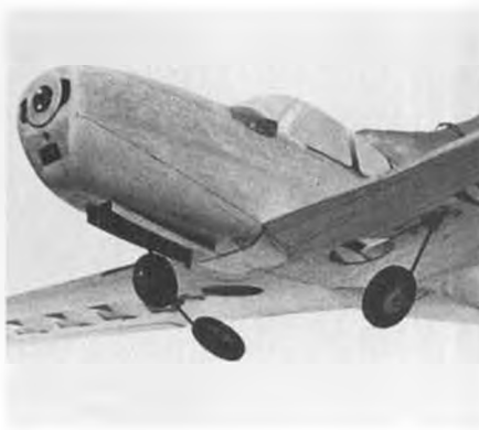
Retract units for 1/2A models, weigh 1/3 oz. each, by Robart.
