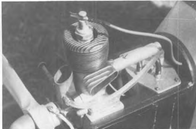
Otto Bernhardt (Mr. 77 Products) put front rotor assembly on side-port Ohlsson 60. Ship is wife Marge's "Trenton Terror."
