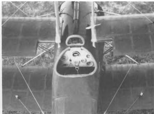
Cowling and cockpit close-ups of Dr. Clapp's Sopwith Triplane also reveal a multitude of rigging wires. Covering is silk and dope. Routine assembly must need check list!
