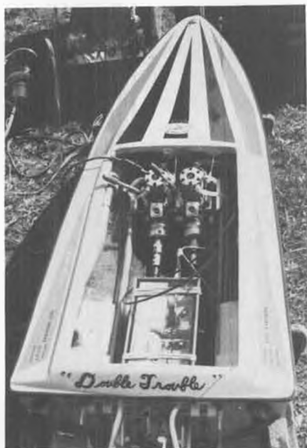
Skip Horstman's twin 21 powered deep vee. Complex exhaust throttle linkage.
