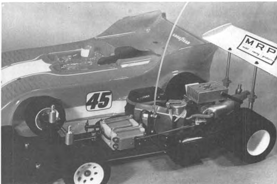
Another angle on completed car, with body in the background. Receiver and battery pack mounted on side pans.
