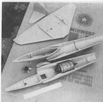
Complex internal ducting of Midwest A4D-1 Skyhawk for 1/2A power.
