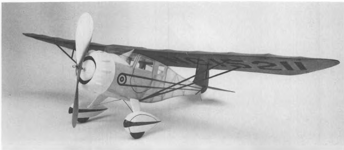
Mark Fineman, Hamden, Connecticut, built this 30 inch span Monocoupe from Megow plans. Modifications include 1/16 sheet filling in forward fuselage (Cleveland style) and turned balsa wheels.
