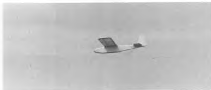
Bob Simon's pocket slope soarer spans 25 inches. Controlled by 2-channel rig, it is a bit squirrely, but very aerobatic.
