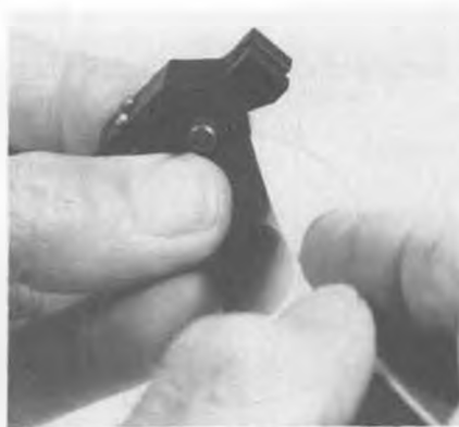
Photo 8. Final trimming of cut with finger nail emery board.
