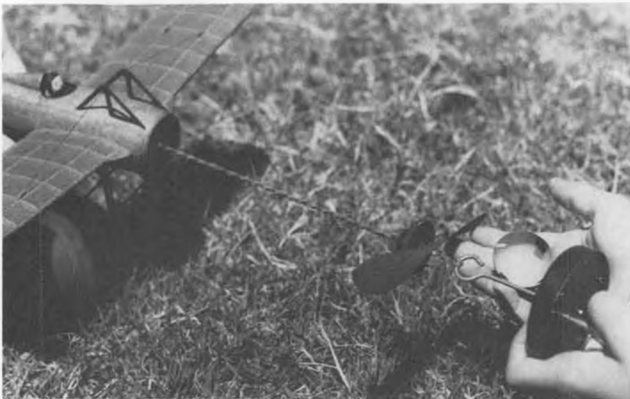
Winding with spinner cap pulled off. Small bits of Velcro hold spinner to back-plate.
