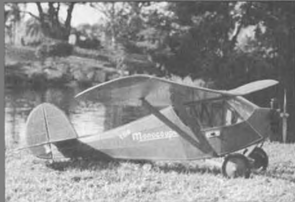
Wing span 49 inches, weight area 338 sq. inches, 2 or 3 channel radio, 049 glow or 05 electric.
