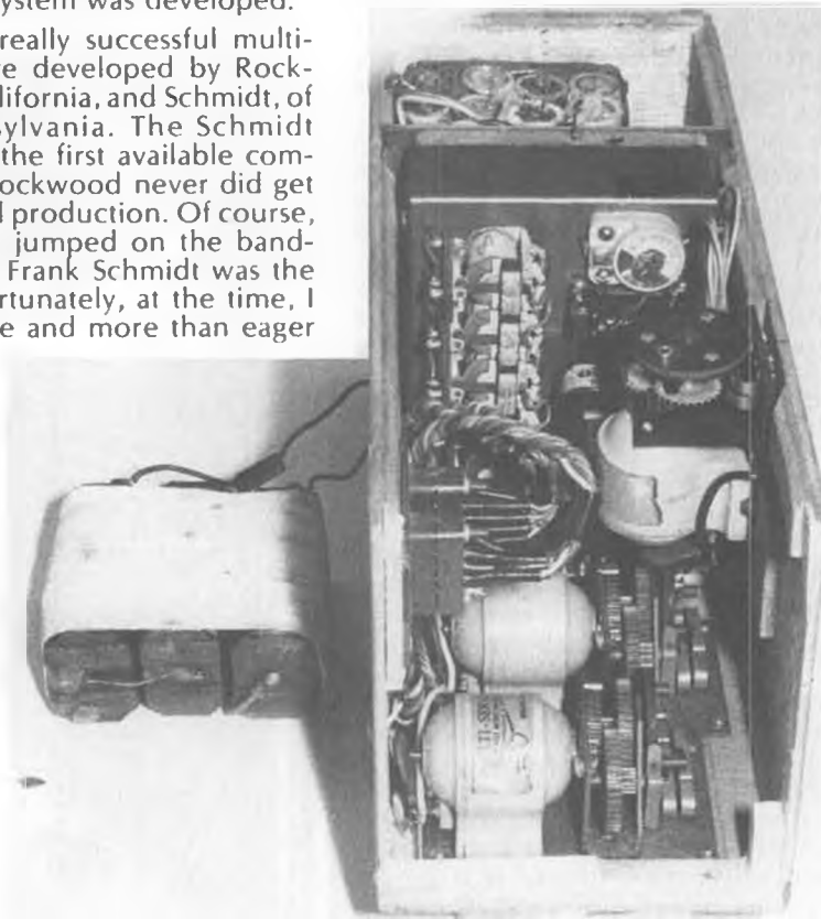
This is a removable R/C unit as used in a multi model during the late 50's. In this case, a 5-channel "Bramco" receiver operating multi-servos. The battery on the left is the "B" battery, the pen cells were the "A" and servo supply. The lower servos were "multi-channel" types, each requiring two channels for operation. The upper servo was a "single channel" type used with the 5th channel for engine control. This "unit" or box measured 3-1/2 x 4 x 8 inches, weighed 36 oz!
