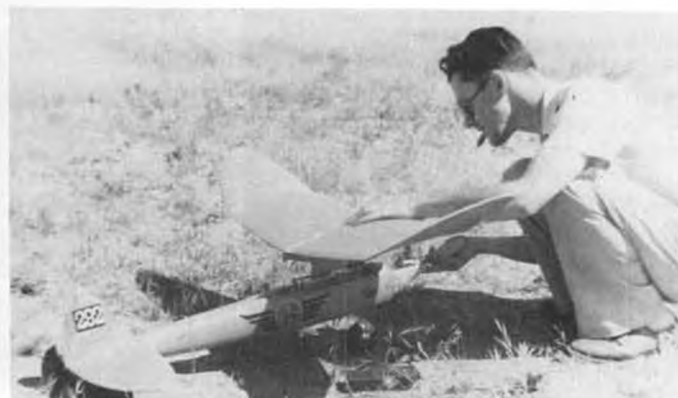
Virgil Rice built his Zipper with sliding pylon to enable him to use different engines while maintaining the same CG. Photo in 1940.
