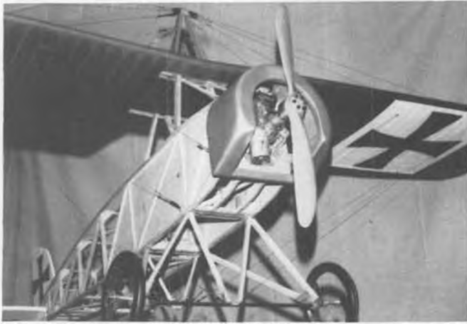
Cox Roper 1.4 cu. in. ignition engine powers this Pfalz A-2 by Chuck Nellis. Span 8½ ft., 16 pounds.
