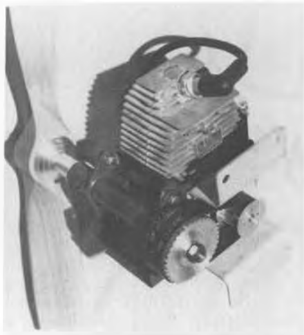
Belt reduction drive for Quadra, by Andy Sheber, Inc.
