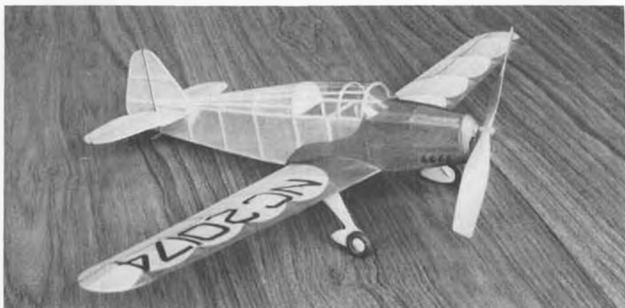
Tom "modernized" construction with sliced ribs, and laminated wing tips and tail surface outlines.
