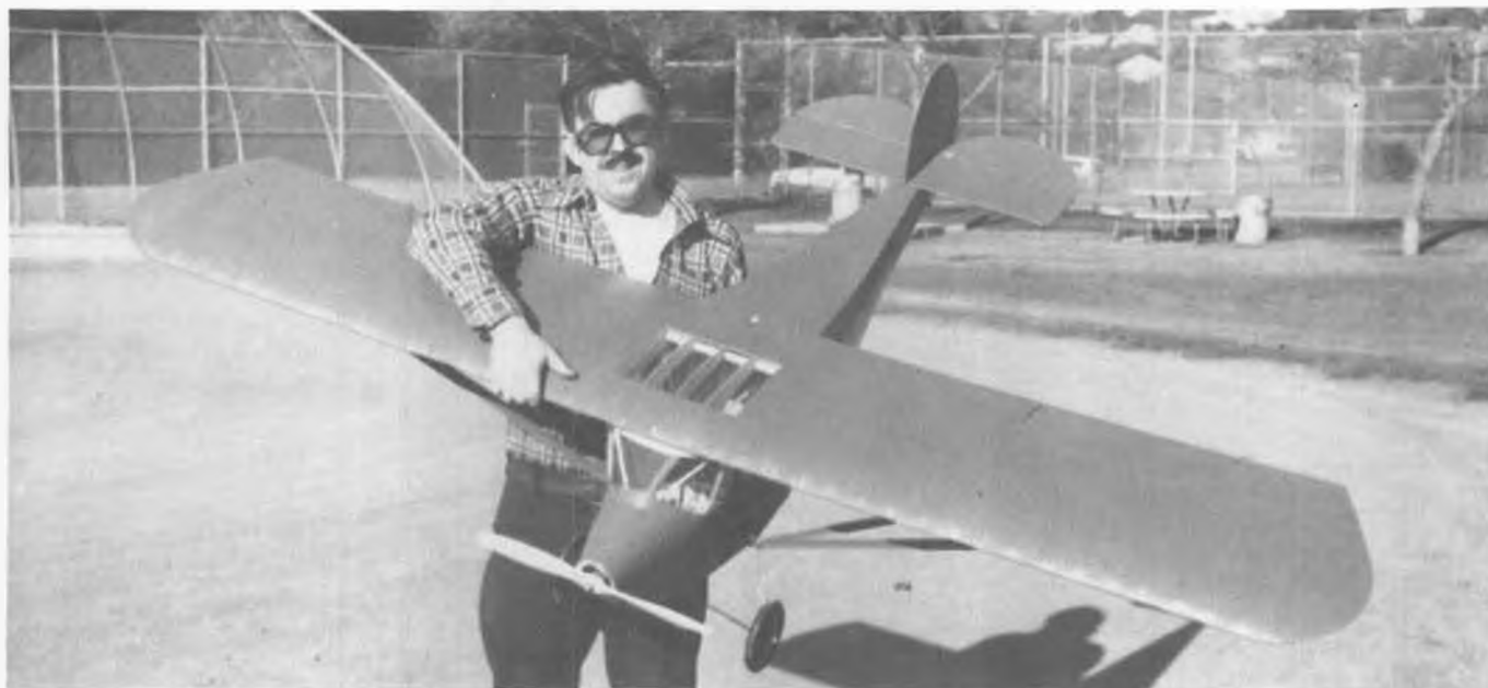
Bob Boucher with his Mammoth Monocoupe, during first flight tests. Design is enlargement of his Astro Flight 50 inch kit for 1/2A glow or .05 electric.
