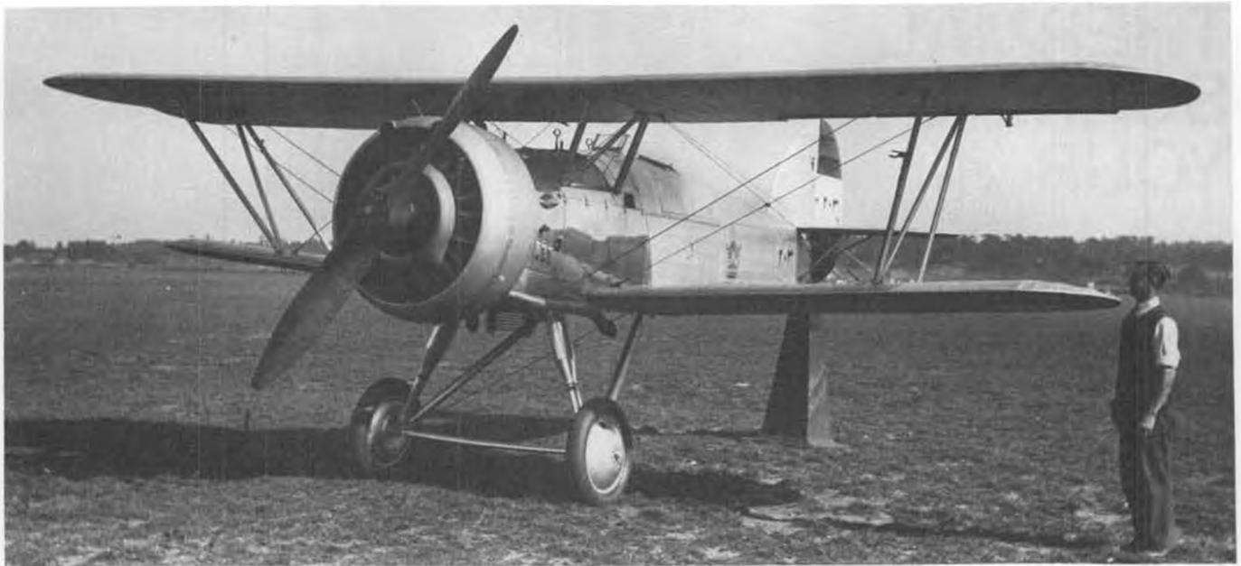
Cooling problems with the crankcase shutter on the Pratt & Whitney Hornet engine were serious enough to warrant changing to the Bristol Mercury VI radial engine. The Mercury was designed with an exhaust ring in front of the crankcase, making it suitable for desert operation.
