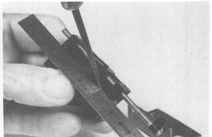
Photo 6. Scribing line to indicate portion to be cut away.
