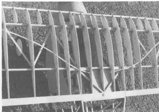
One bolt and one dowel hold wing in place. Struts are functional. Cap ribs if using silk and dope!
