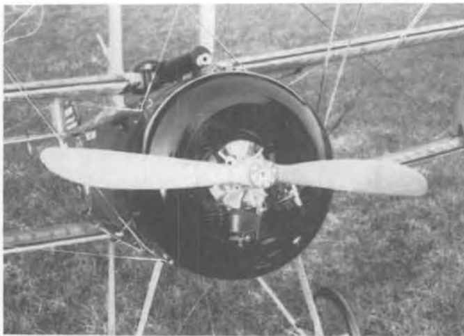
Cowling and cockpit close-ups of Dr. Clapp's Sopwith Triplane also reveal a multitude of rigging wires. Covering is silk and dope. Routine assembly must need check list!
