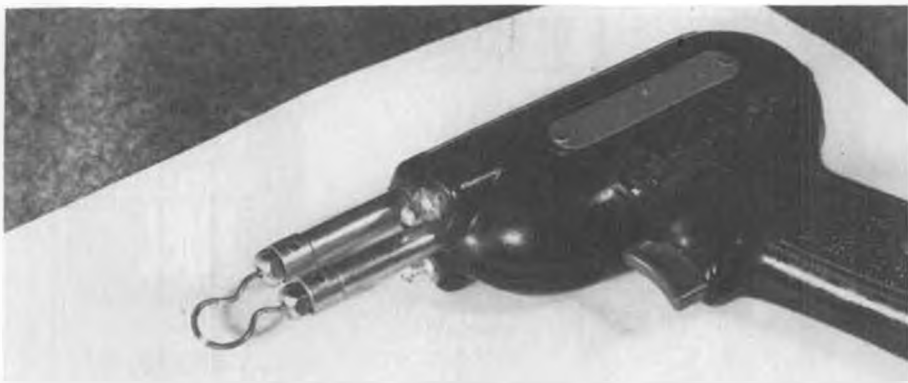
Foam hollowing gadget . . . copper wire loop heated by soldering gun.
