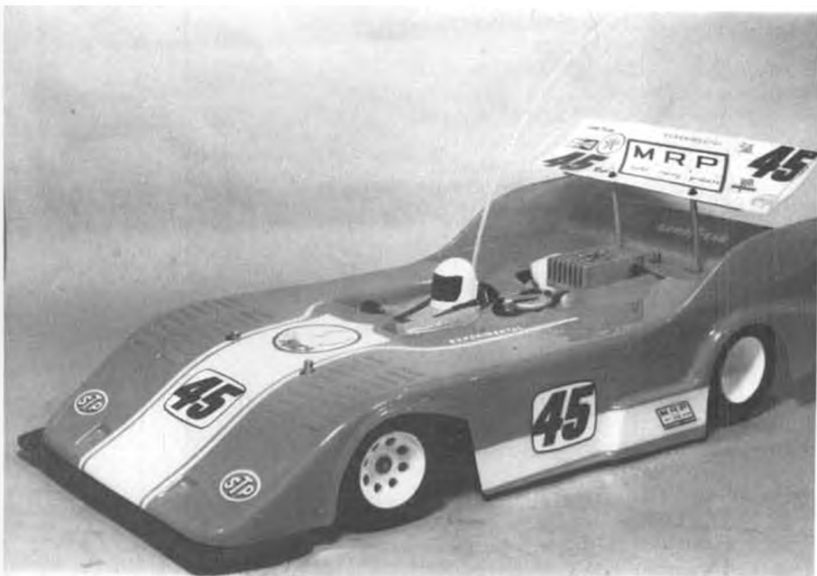
Photo taken after several practice sessions and one race. Body is Abarth Can-Am, in orange. Wing tubes bent forward for more down-force at rear. It works!
