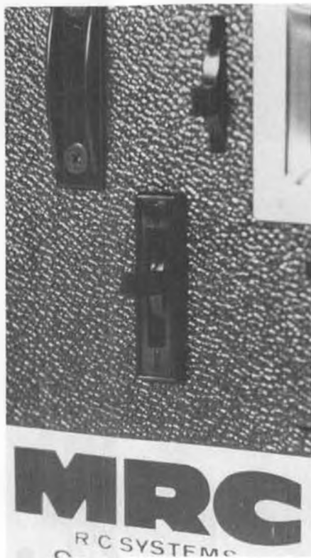
Extra channel control lever mounted on MRC test transmitter.
