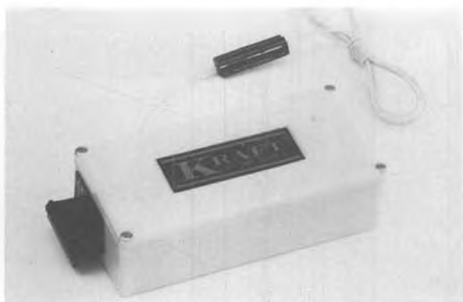
Kraft antenna connector. Allows you to build in antenna.
