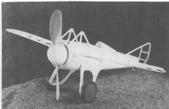
It's a big spinner, but avoids necessity of making up dummy rotary engine.
