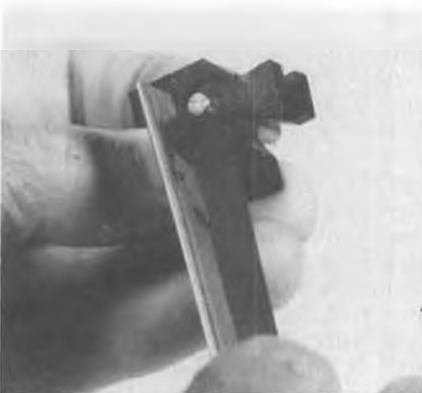
Photo 7. Cutting away material with Zona saw.
