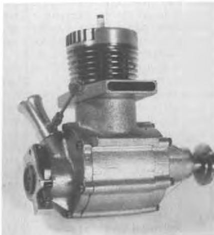
So what's new about gear reduction? This ignition .60 with 1-1/2 to 1 reduction gearing built by Otto Bernhardt in 1946.
