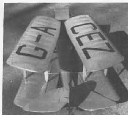
Designed for compact storage, folding wings also handy on model.
