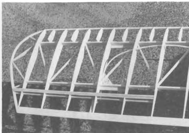
Wing structure is light. Ailerons not separated at this time. Note Nyrod control tubing.
