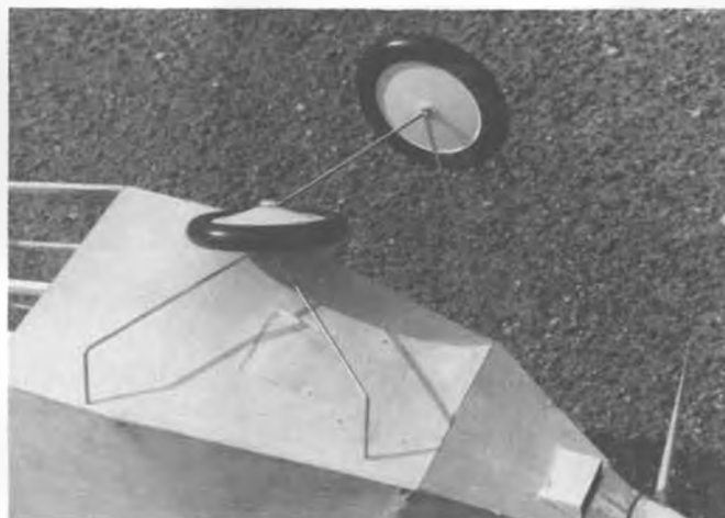
Simple wire struts plug into brass tubing. Add fairings to improve their appearance.
