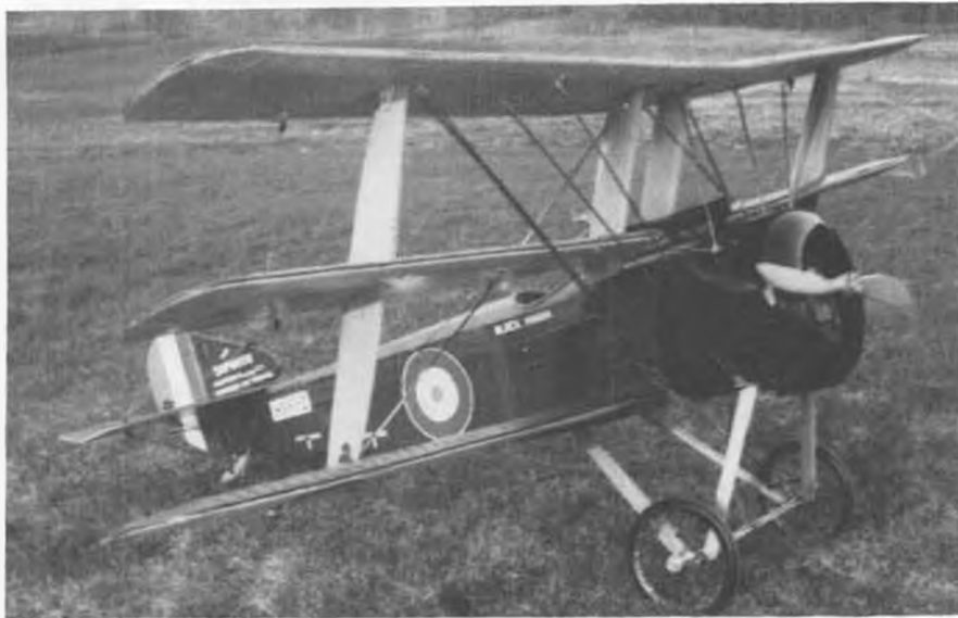
Dr. George Clapp, dental surgeon from upstate New York, built this 1/4-scale Sopwith Triplane. Quadra powered, it weighs 19 pounds, and is built entirely from bass and plywood...no balsa. It's his first R/C model! Photo on right answers obvious question.
