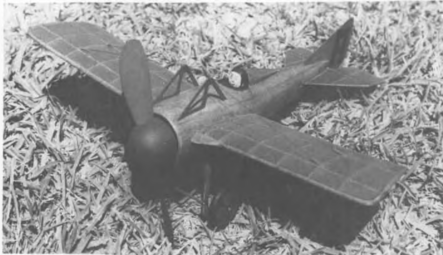
There's plenty of clearance for large props with scale gear legs and wheels.
