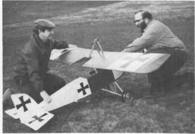
Pfalz features actual wing warping for scale aileron action. Bob Dunn, left, holds on while Chuck cranks.
