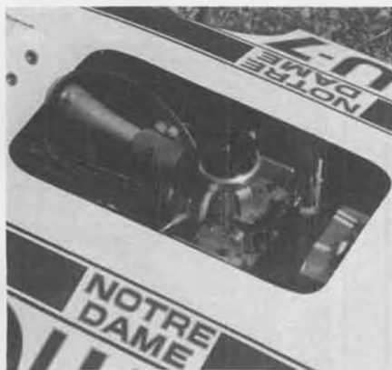
The new Picco .65 ABC racing engine nestled in Les Ruggles' Notre Dame. Engine is available through Mutiny Model Marine; see text.
