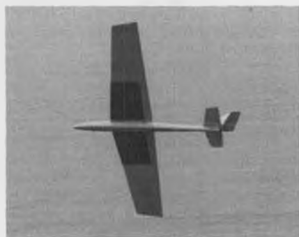
Brian Irvine's ship in a tight pylon turn. Note the extremely small stab.
