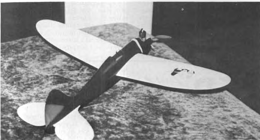
Photo No. 10. One of the two 1980 replicas of the 1940 Fireball control liner, built by Frank Macy. Fuselage is carved and hollowed, finished in automotive acrylic lacquer.
