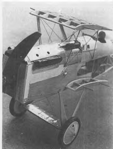
Cedric dela Nougerede's latest is this 1/10 scale SE-5, a little over 30-inch span. Uses lots of thin sheet metal in nose section.
