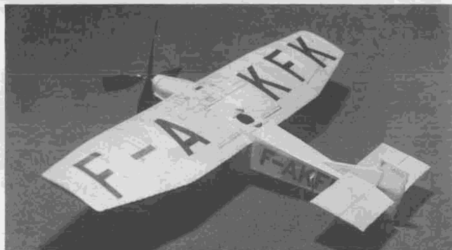
Upper photo shows the Farman as originally built with the scale size (i.e., almost nonexistent) vertical tail, which gave problems. Enlarged vertical surface (lower photo) was the answer.
