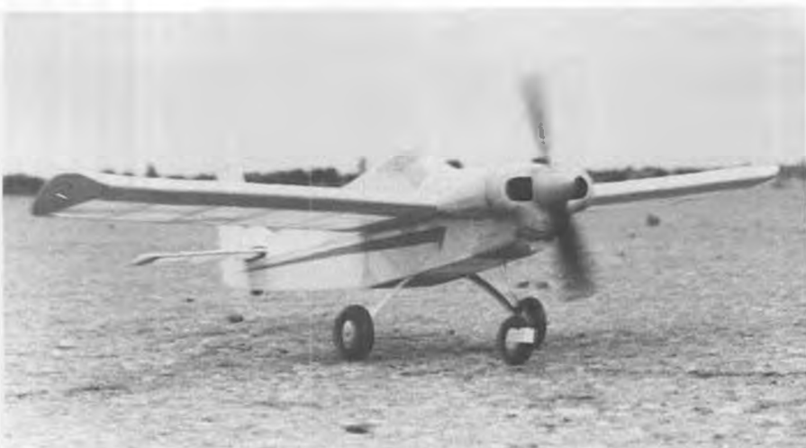
The Pottier just beginning to rotate for takeoff. Nose gear permits straight, stable ground runs, is a real lifesaver when landing in rough areas.
