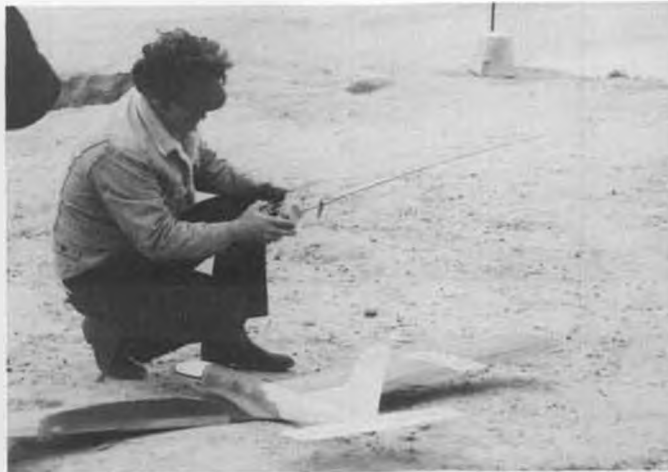
Another super-fast racer is the "Grand Boss" designed and built by Jerry Arana. Equipped with flaps for light-air flying.
