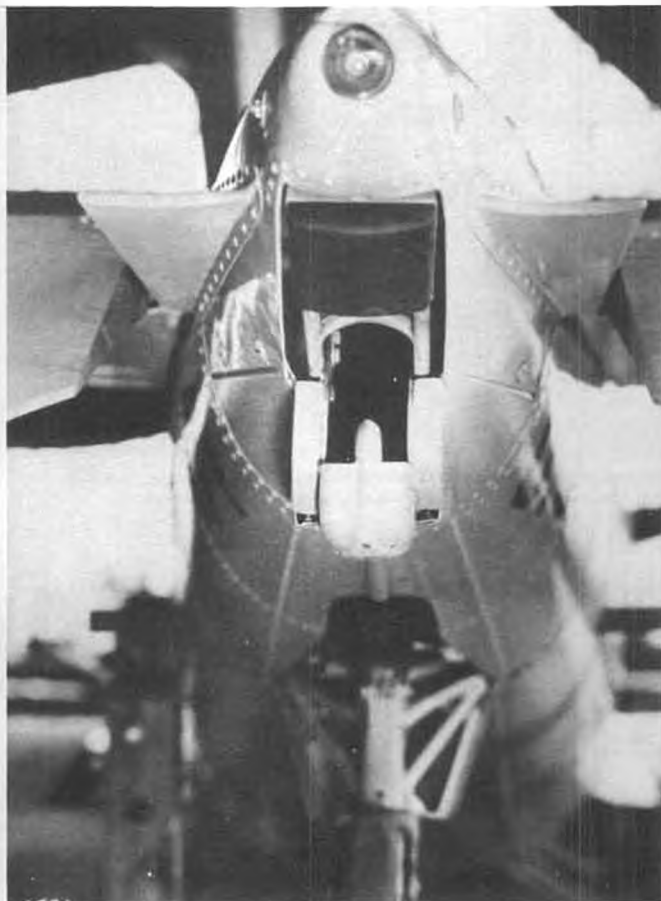
Tail hook was retractable into the fuselage. Hard rubber bumper took rebound. National Archives photo.
