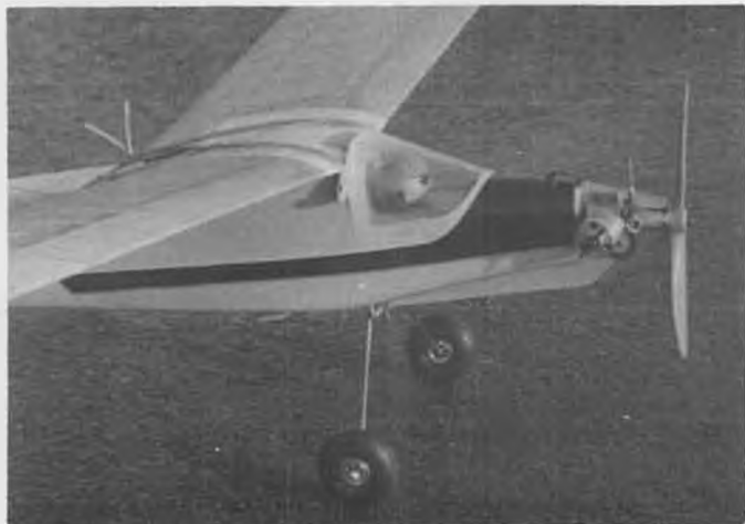
Powered version uses a Russian MVVS .09 diesel, gives long, satisfying flights with a 4-oz tank. Note plywood nose skid.
