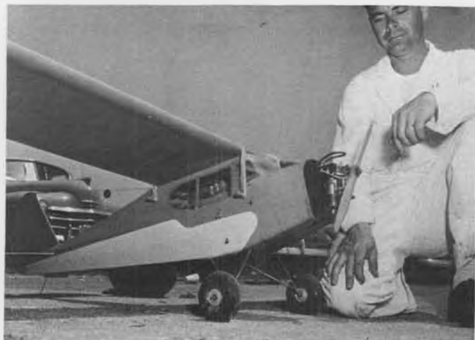
Spitfire .60 on ignition powered Schneider's Cubs. Note 3-tube receiver in cabin. Tubes rubber-banded to prevent vibration failures.
