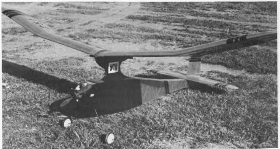
Photo No. 7. Pond's at it again! This time it's a scaled-up Playboy Jr. with K&B 3.5. Scaling the small one up has certain advantages over scaling the big one down...see text.
