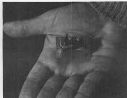
Bill uses a 77 Products (see ad p. 109) ignition cutoff timer, runs 35 seconds max.
