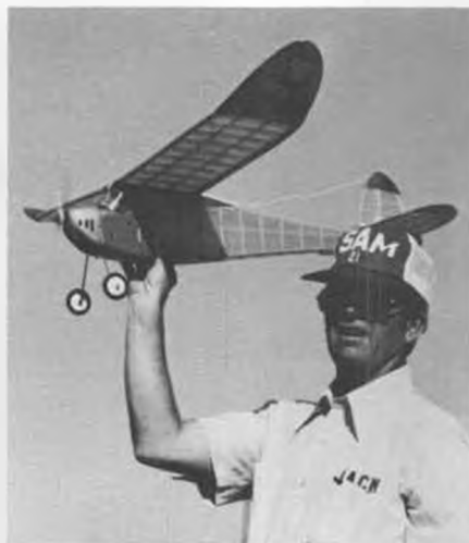
Photo No. 8. Jack Alten about to launch Ted Kafer's 1/2A Challenger. Big props and low nitro give 6 to 7 minute engine runs.
