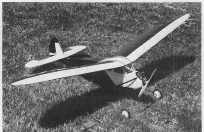
Photo No. 4. Jack Alten did a fine restoration and R/C conversion of John Pond's old F/F Scram. Now uses Saito 4-cycle power.
