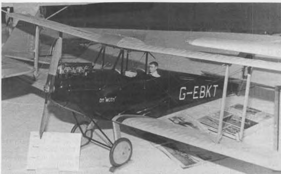
M.A. Zimmerman's Gipsy Moth placed a creditable 3rd in Non-Military Sport Scale at Toledo, but in our opinion it should have been 1st. In addition to the flawless finish and superb detailing is the fact that it sports a working replica of a Mk. 1 Cirrus engine! Featuring four cylinders and overhead valves, the engine displaces 1.11 cu. in., weighs 30 oz., and turns a 12-1/2x8 at 8800 rpm. Yes, it has flown.
