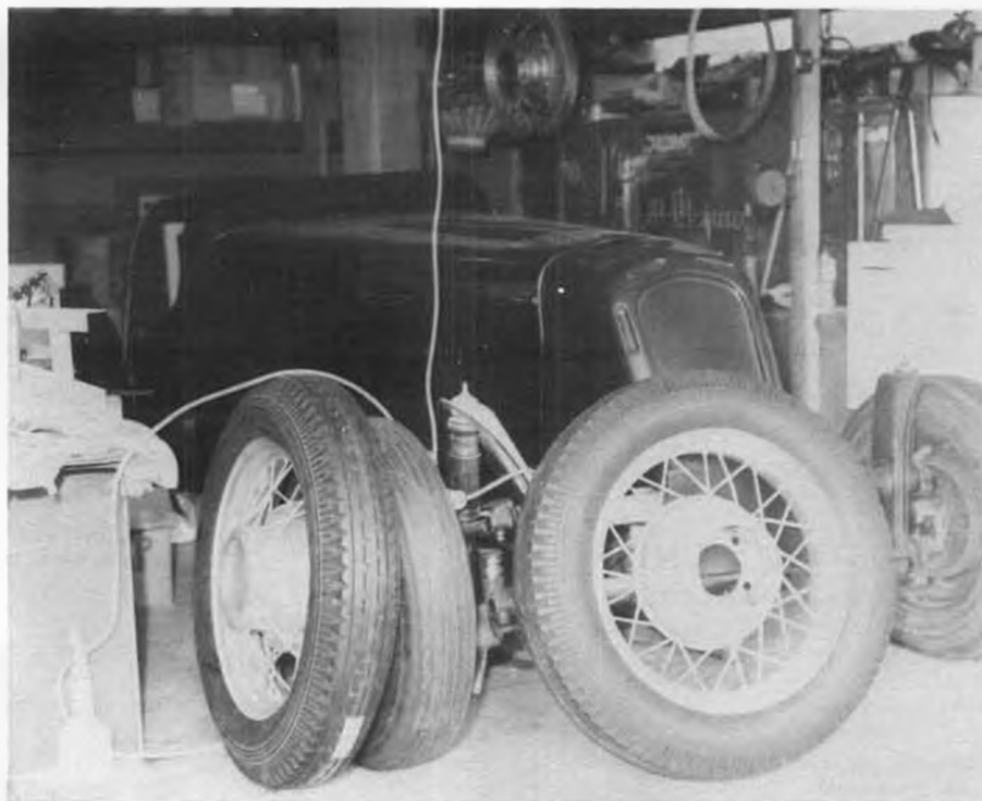
Progress report on our '31 Alfa replicar. Fiberglass body is in position to check for proper fit. The original Volkswagon wheels are still on, but the 1932 Ford 18" wheels have been silver spray-painted, new 550 x 18 tires added, and are ready to mount with special adaptors. Gear shift and pedal assembly still have to be moved back about 3 feet, steering column extended the same amount. Progress is very slow. Detroit we ain't!
