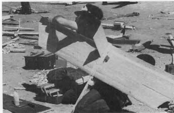
Another successful tailless was this no-sweep plank type by Steve Manganelli. Must have used an electronic mixer for the elevons.
