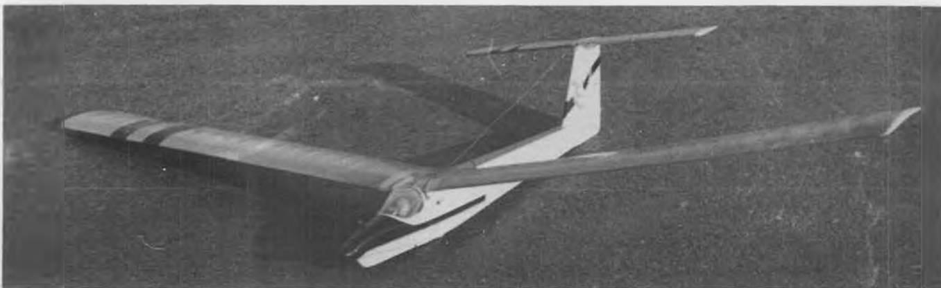
All set to go gliding! Conversion from powered to glider modes takes only a couple of minutes. Pavel prefers flying the model with two channels (rudder/throttle), but the plans show an optional full-flying tail arrangement for those who prefer this type of set-up.
