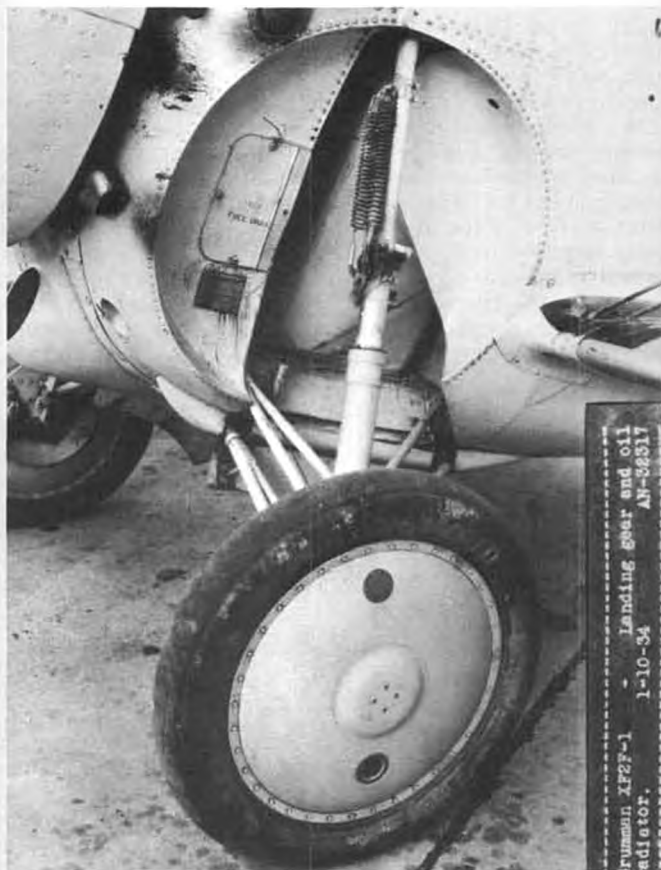
Landing gear was operated by sprocket chains from a shaft going back to a crank at pilot's right knee. Large 30x5 wheels were responsible for F2F-1's potbellied appearance.
