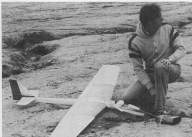
Rich Spicer with Brian Irvine's more serious approach to slope racing. Weighs 5 lbs. empty, can be ballasted up to 11 lbs.
