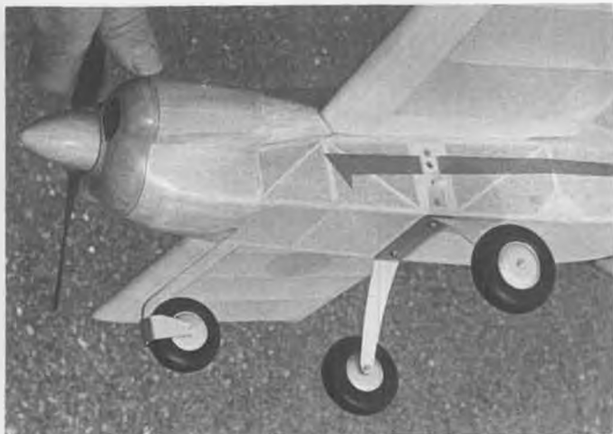
Landing gear is simple and straightforward. McCracken used plywood and screws to mount main gear; easy to remove if needed.
