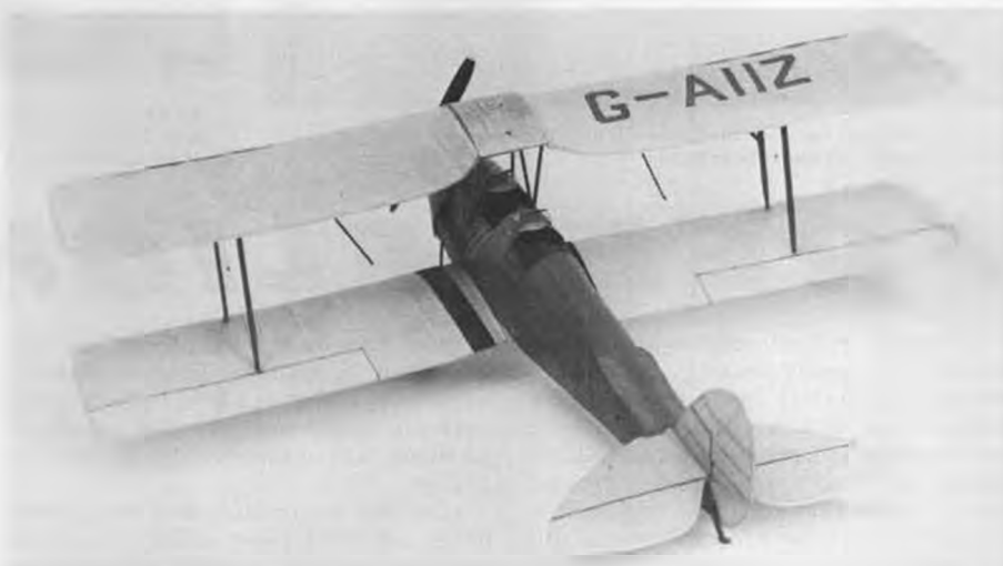
Cedric dela Nougerede's Peanut Tiger Moth sports just as much detailing as its bigger brothers. Note "spin strakes" on top rear fuselage, used on the full-size Moth to improve spin recovery.
