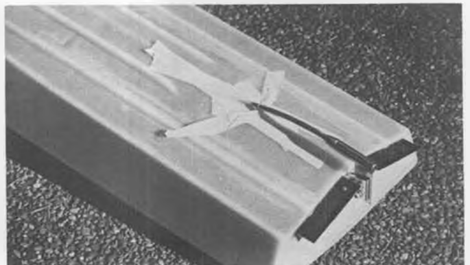
Masking tape on the bottom keeps epoxy from running through shaft log opening. Hardware is from Prather hardware kit.
