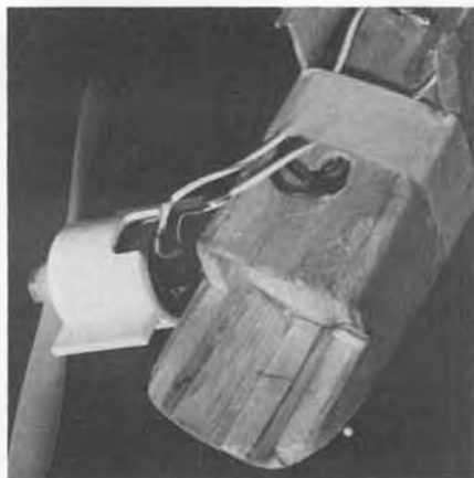
Bill Baker's quick-and-dirty method of mounting an Astro 02. Light weight is essential.
