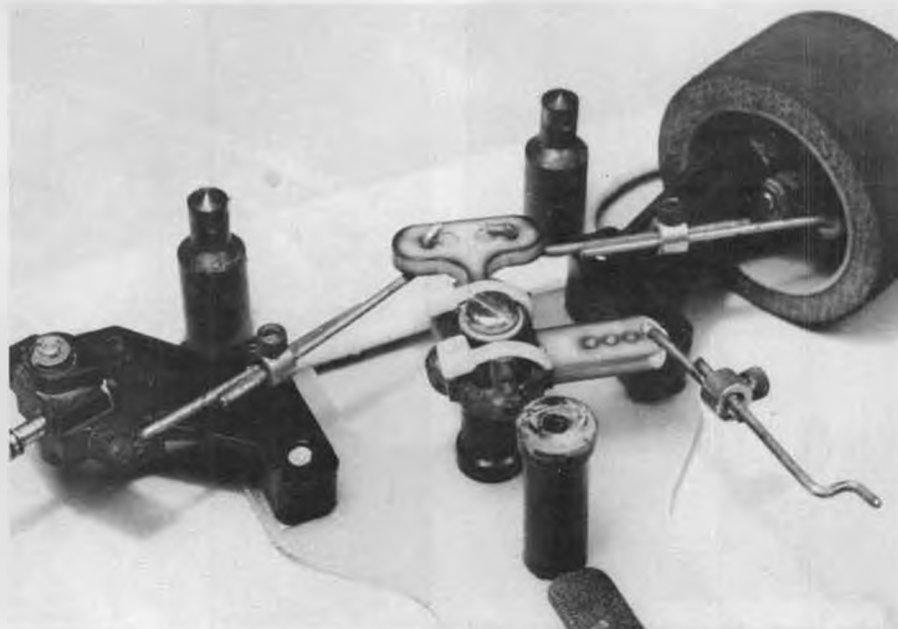
Front end on 12E: nylon ties on servo saver increase loads transferred to servo, but also tighten up steering response. Tire is new molded number from Twinn-K.
