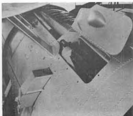
A .30 caliber Browning gun was installed on the left side, a .50 caliber on the right. The telescopic sight was primarily for bombing, but also had ring-and-bead sights on the left and right sides.
