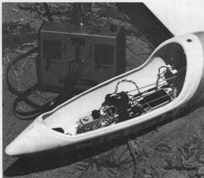
Switching set-up in Steve's quarter-scale Carrera Mistral-C. Micro switch is mounted directly on extra switching servo.
