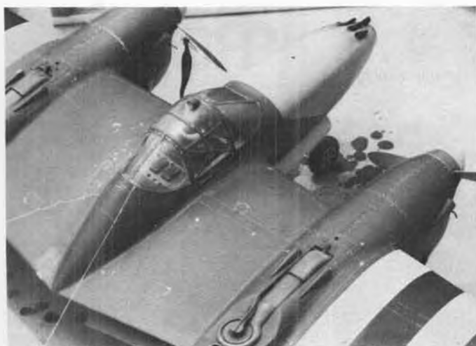
Bob Pray's Royal P-38, two ST .60's, Kraft radio, retracts, Fowler flaps. Ticked prop on low pass, but survived.
