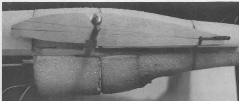
After carving to shape and hollowing, blocks are glued into place. Bulge in fuselage profile below wing root is for installation of switch as shown at right.
