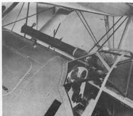
A .30 caliber Browning gun was installed on the left side, a .50 caliber on the right. The telescopic sight was primarily for bombing, but also had ring-and-bead sights on the left and right sides.
