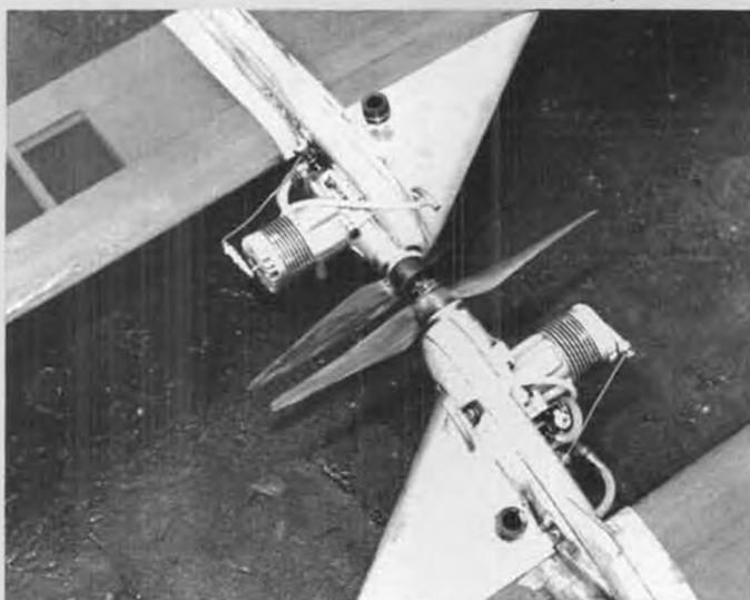
Secret of getting plane in fast after shutdown is good balance. Len Ascher moved engine back on plane at left.
