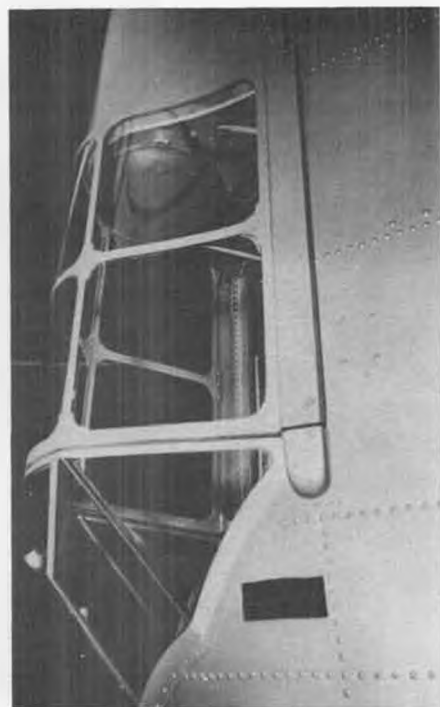
Sliding canopy changed from flat side at front to curve at aft end. Life raft stowed in tube behind headrest.
