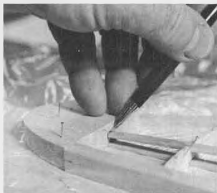
Tip butts against L.E. and spars; T.E. continues. Mark and trim before gluing in place.
