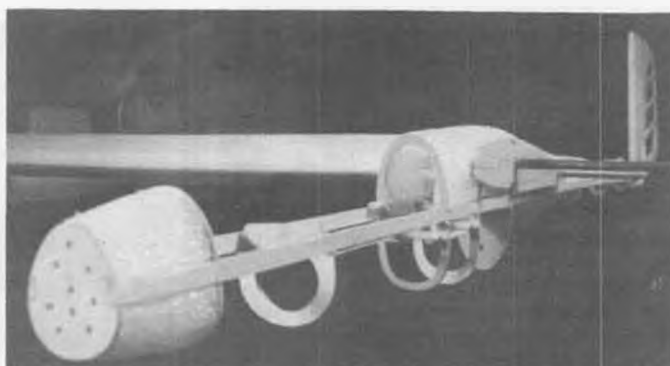
Foam blocks are cut for snug fit between bulkheads. Stay in place while being carved to shape.
