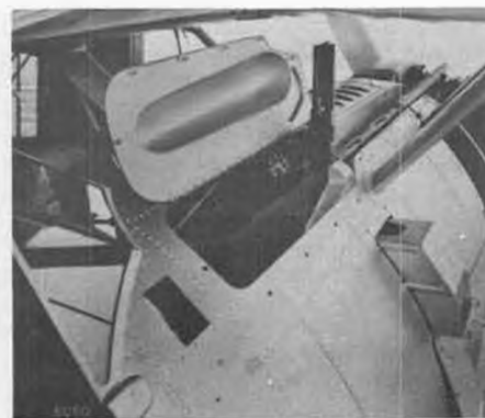
A .30 caliber Browning gun was installed on the left side, a .50 caliber on the right. The telescopic sight was primarily for bombing, but also had ring-and-bead sights on the left and right sides.
