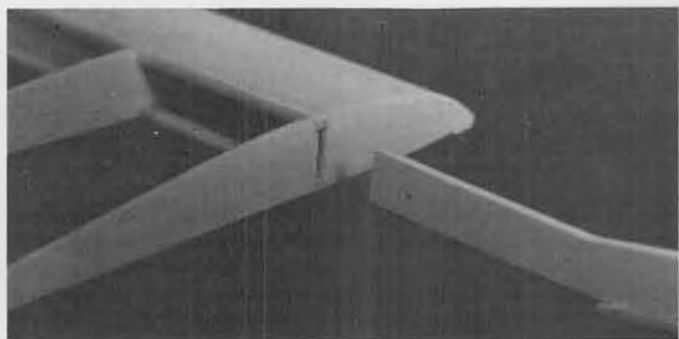
Slot in inner panel about to receive dihedral brace already attached to outer panel.
