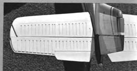
Other super scale features include vacuumed-formed skin detailing for stabs and control surfaces.
