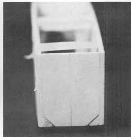
Above: Triangular fuselage corner stock is tapered at rear for joining of fuselage sides. Right: Bottom of front bulkhead is cut away to clear triangular fuselage corner stock.
