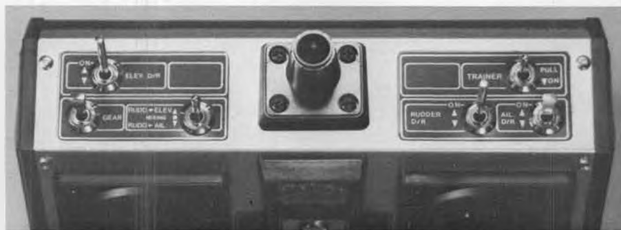
All of the auxiliary function switches are located on the top, within easy reach, also having different levers so you can get to recognize them by feel, no need to look down.
