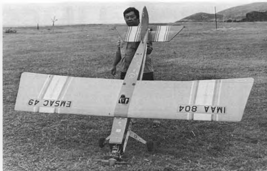
Darrell Wong with his Hobby Shack Giant Stick. He added shear webbing to wing, more vertical stab support, substituted weak stab with unit from Cunningham "Eindecker".
