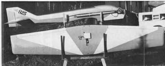
Photo D. Monokote saved weight of 8 ounces compared to painted version.
