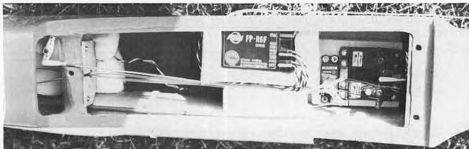
Photo E. Lightweight fishing line in tubes for nose gear steering . . . much lighter than wire.
