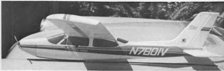
The Kraft Cardinal with gear retracted (well, it looks that way!) and Leisure 05 power. Note Hoerner tips.
