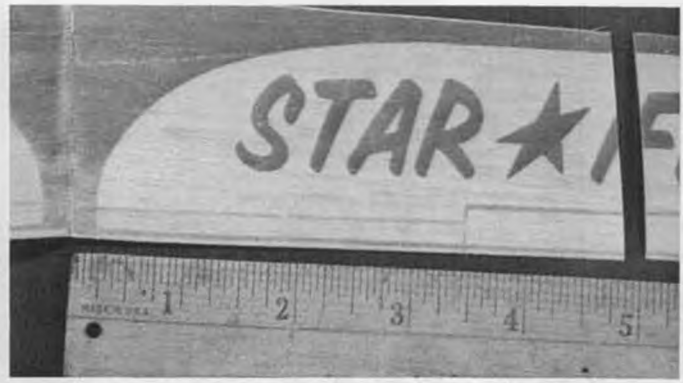
Kit wings have sweepback . . . be sure to allow for this when cutting polyhedral breaks.
