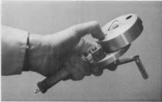
Bob Hatschek shows off panic release of his homemade towline winch. Note folding handle and counter.
