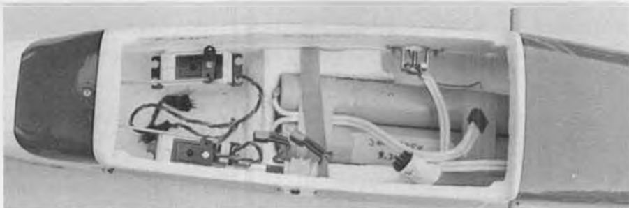
Leisure 05 battery pack in bottom of Cardinal. Plenty of room.
