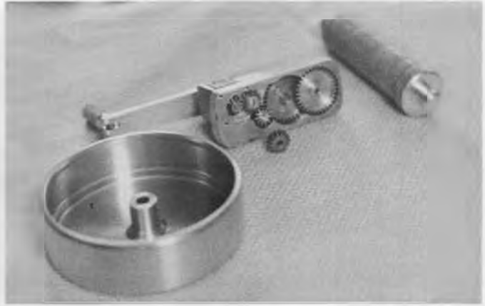
Internal mechanism of Hatschek winches . . . nice workmanship is evident.
