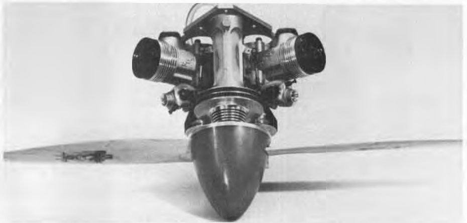
Two Rossi 80's bolted together and linked to a 1 to .56 reduction belt drive. Check with Condor Hobbies for future availability.
