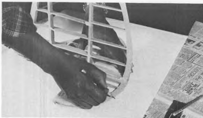
After removing half of stab, rudder could be laid down flat to trace outline. Everything was traced directly from model parts.
