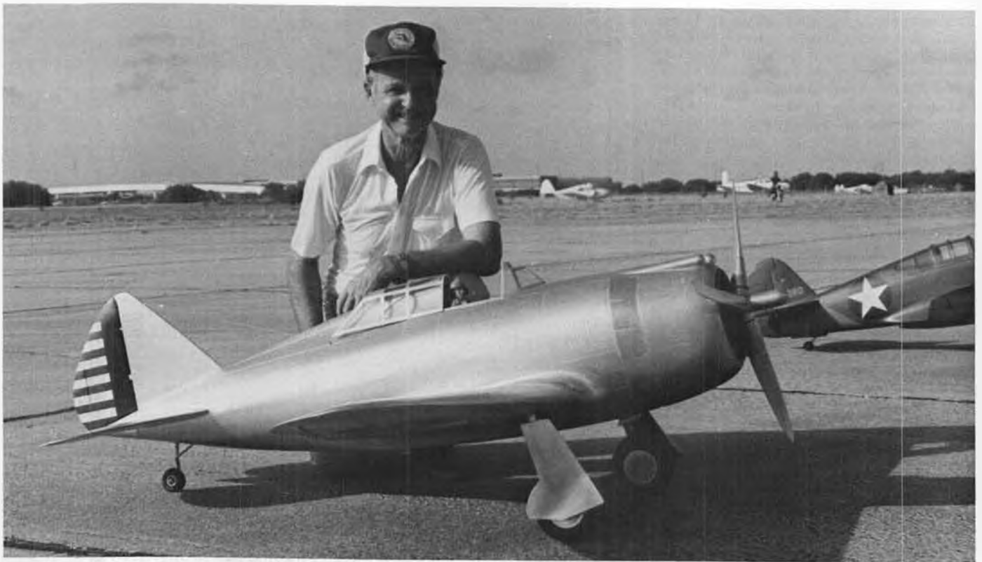
The latest from Col. Art Johnson, Delray Beach, Florida, is this P-43 Lancer, forerunner of the P-47 'Jug'. It weighs 20 pounds, is Quadra powered, and is a great flier. It will be a future construction article.
