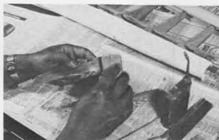
Sanding rib smooth before tracing. There were no short cuts to this job!
