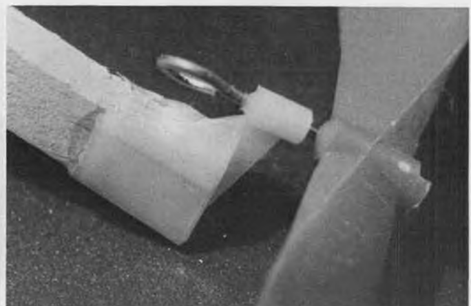
Close-up of prop hanger, showing cut-away portion for rubber clearance.
