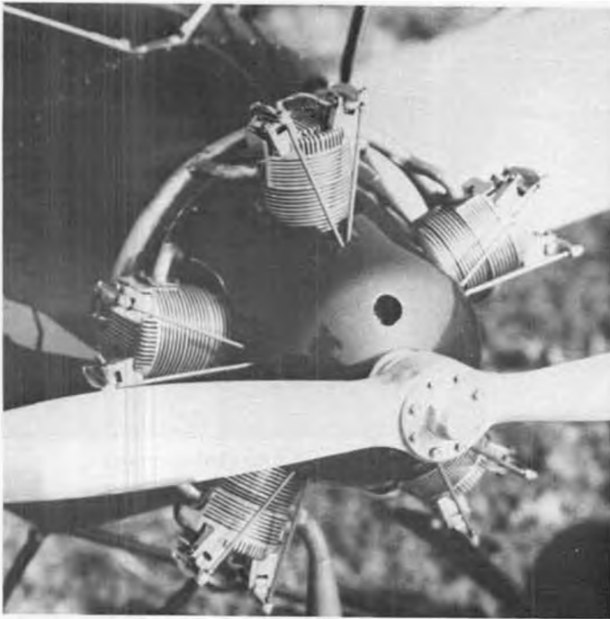
Forrest Edwards, San Pedro, scratch-built this fine running radial 4-cycle. Mucho power for his Concept 1/4-scale Fleet.
