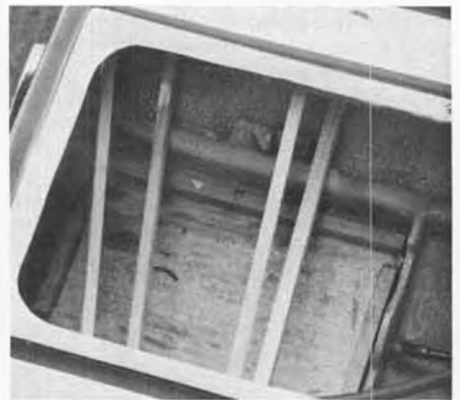
Internal bracing holds ply patch in place while epoxy cures.
