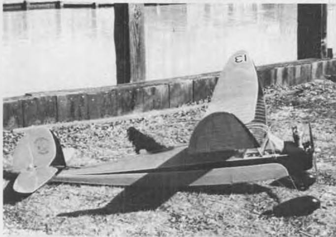
14. Really dooded up Comet Clipper with wheel spats and cowl, by Woody Woodman. Super Cyclone power.
