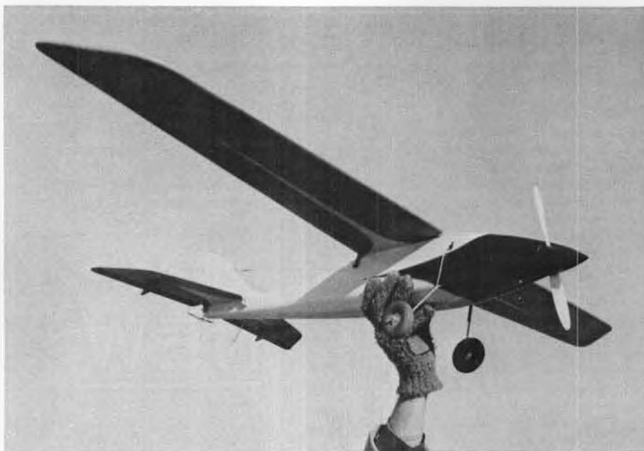
"Smooth Hare" was short lived (bad battery in pulse box) follow-on "Square Hare" by MB's Editor, dating February 1963. Won Intermediate Design trophy at Weak Signals Toledo Show. Cameron .19, Kraft single-channel, Galloping Ghost for proportional rudder and elevator. Note typical GG "birdcage" wire crank linkage on elevators.
