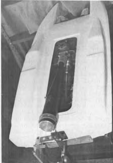
Stock K&B pipe. Prather pipe (above) gave 700 to 1000 more RPM.
