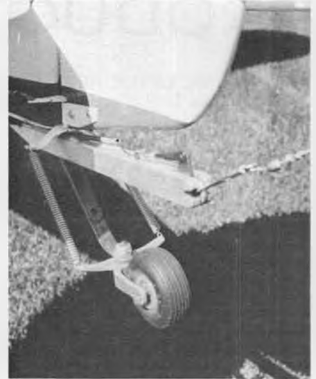
Super Cub tow bracket and release mechanism. Herb has towed two gliders at once.
