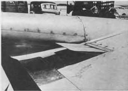
Drive shaft housing and exhaust port. Flap restricted hot gasses to warm cold engine.
