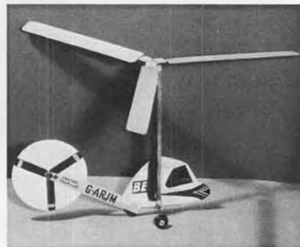
Ray Malmstrom, England, designed and built this just-for-fun rubber powered helicopter with a 16-inch rotor.
