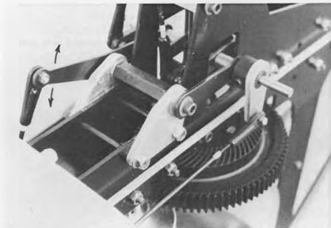
Collective yoke detail. Collective rod moves arm up and down (arrows) for pitch changes.
