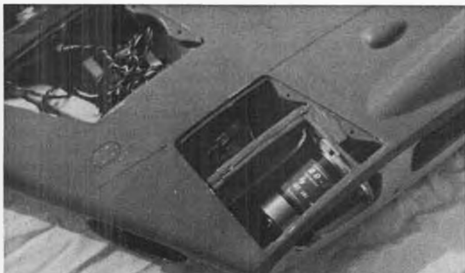
The N9M-A model uses two Astro 05 cobalt motors with long drive shafts. Scale airfoil yields lots of room inside.
