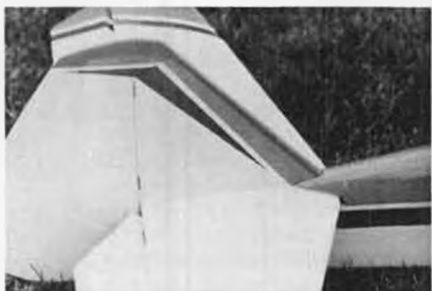
Photo No. 5. Empennage details. Vertical fin bolts through stab and aligns itself.
