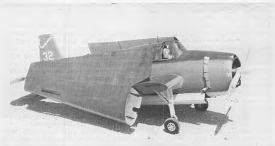
Best Mechanical Option Award winner. This TBM-3 Avenger built by Dennis Crooks featured R/C operated wing folding mechanism and locking pins. Weighs 22 lbs; belt drive OS-90.
