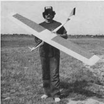
Rick Schrameck (U.S.A.) and Electrocuttioner. Whisper F/G fuselage, E-178, Astro 40/18.
