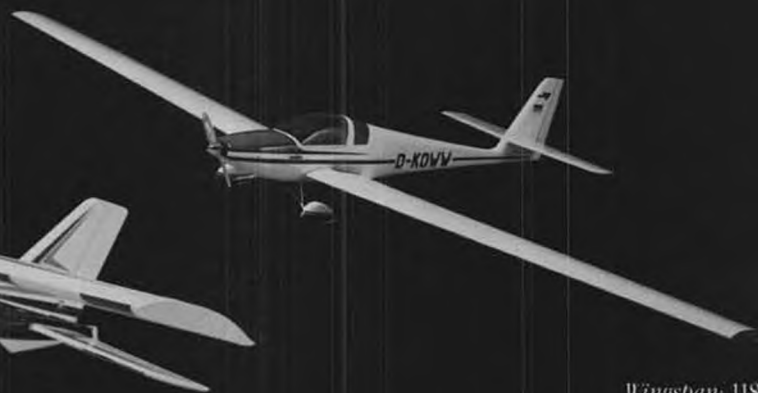
Wingspan: 118" Wing Area: 1038 Sq. In. Flying Weight: 7¾ lbs. Engine: .19-.40
