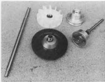
Detail of main shaft, cooling fan, main gear, clutch pulley, clutch assembly.
