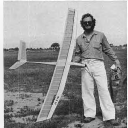
Mike Neverdosky and "Man of Leisure," E-205 wing, Leisure Gear Motor (LT50, 3.6:1), 7-cell.
