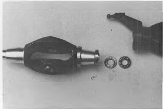
Machined yoke (left) with two bearings for feathering action and a thrust bearing for centrifugal loads. Modern!
