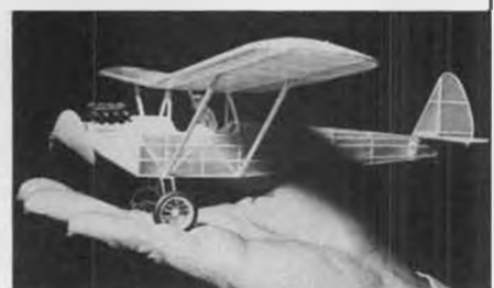
This indoor “peanut” scale Heath Parasol was built by Ray to an all-up flying weight of only 7¼ grams. That’s ¼ ounce!
