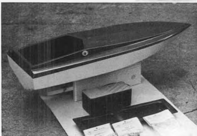
The Stingray sits on its factory-designed wooden starting stand. Bottom pan for radio and tank visible.
