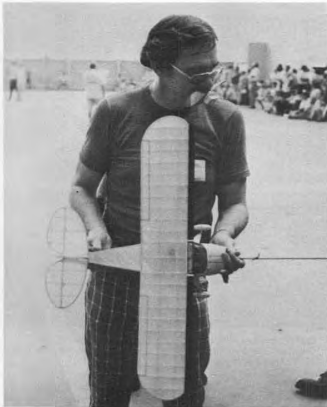
Ken Johnson's indoor Vagabond at California Nats. Note that the rubber knot is in the center of the motor. It's easier to count winds with prop in your mouth. Bob Roha photo.
