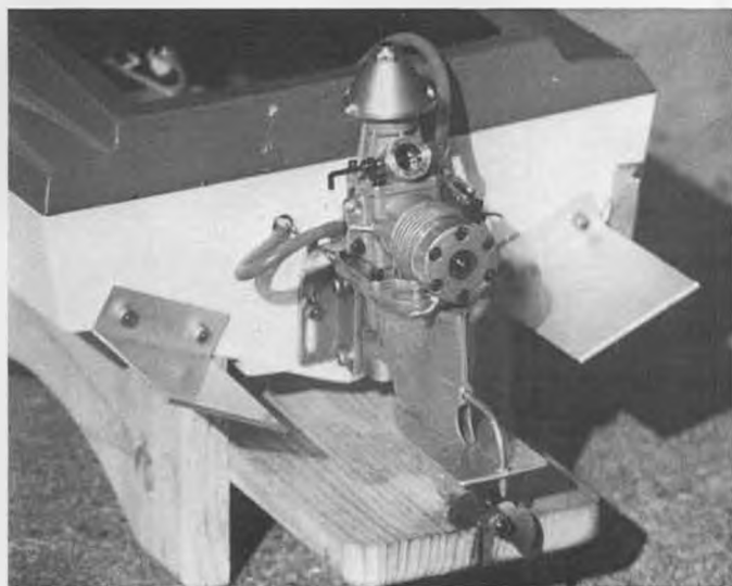
This transom view shows Teague-modified K&B 3.5 motor, spray bar (no carb), exhaust throttle, crankcase pressure fitting . . .
