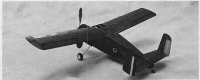
Build this model with lots of downthrust because of the relative small size of the horizontal stabilizer.
