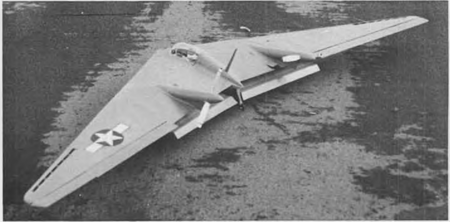
N9M-A model on static display with landing flaps deflected. Top of the aircraft is a medium blue, the bottom is orange-yellow. Model does not feature the split surface yaw control.
