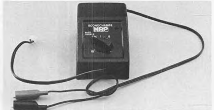
Econocharger from MRP. Features a simple timer with auto-trickle. Ideal for ESV meter as in May '83 Model Builder.
