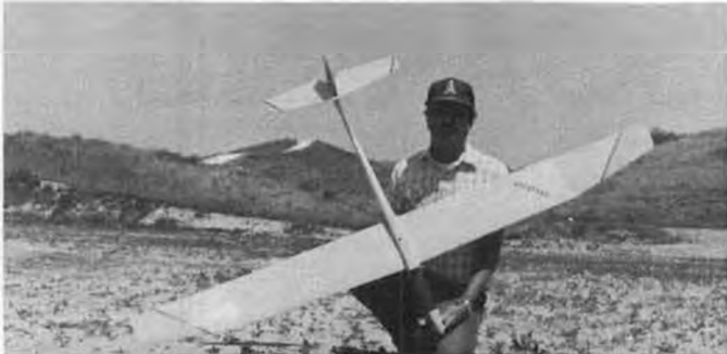
Bill Turner and his Predator. Jack Chambers 7.8% (no. 14) section, blue foam core wing with I-beam spar, sub-spar, and 1/16 balsa sheeting.
