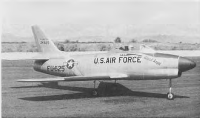
Charlie Beverson, Phoenix, Arizona, brought this Rossi .81 powered Byron F-86D. Rossi/Byron fan combo is a very powerful system.
