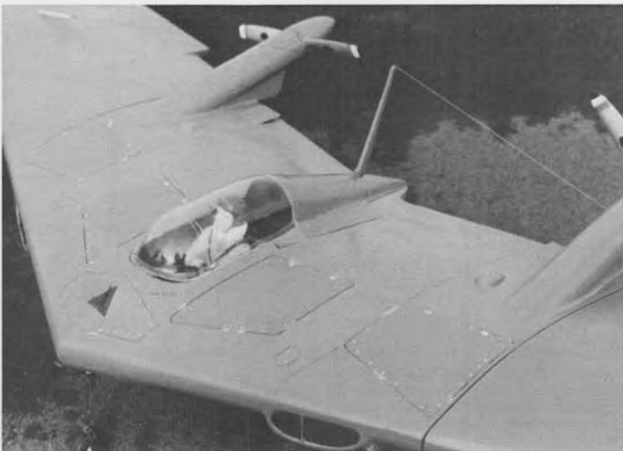
Here's a close-up shot of center section scale details. Canopy is cut-down Sig part. Props are 7x4 Rev-Ups. Northrop logo is red and black.
