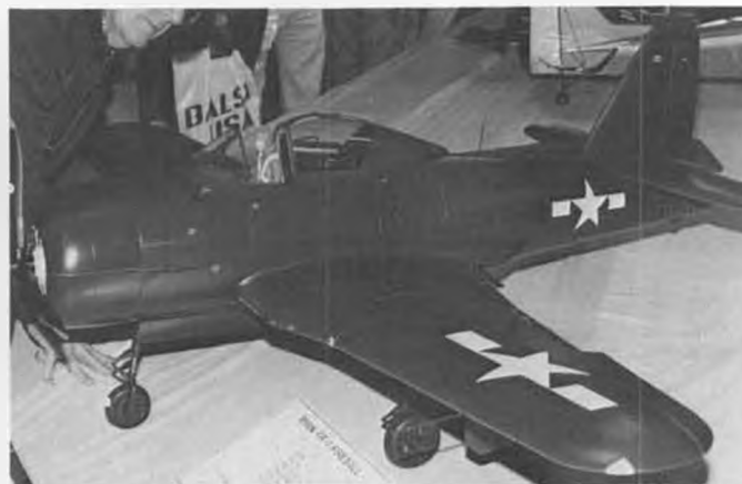
Ryan FR-1 Fireball by Hal Parenti combines the power of a ducted fan and a regular glow engine. I guess it is classed as a twin.
