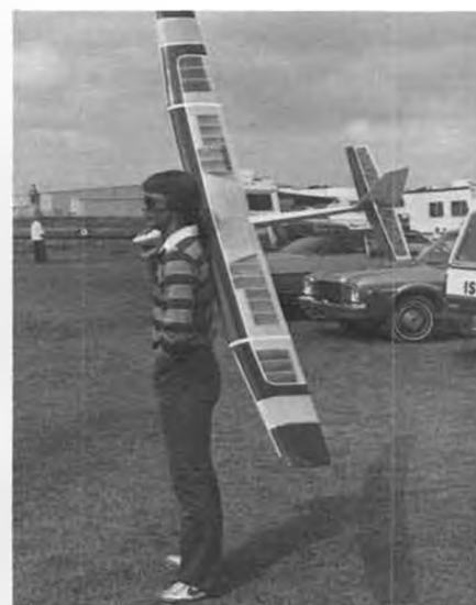
Keith Kindrick and his Gemini MTS contest ship. Very strong wings. Handles well. Many build this 100-inch up to 112- or 120-inch span.
