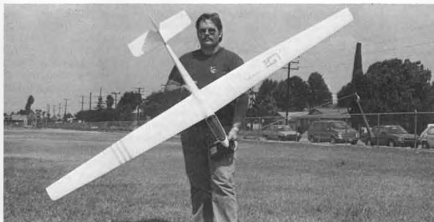
Astro's ASW-15 held by Mike Reed, its builder/flier. An older design, it has a plastic fuselage which is one less thing to build. V-dihedral wings are less responsive than polyhedral wings when they have normal amounts of dihedral.
