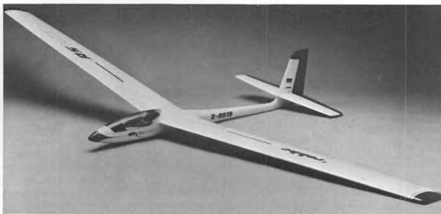
Robbe's ASW-17 looks like a lot of fun. ARF construction means less building time, but at a higher cost. Flat-bottom airfoil offers good thermalling ability.
