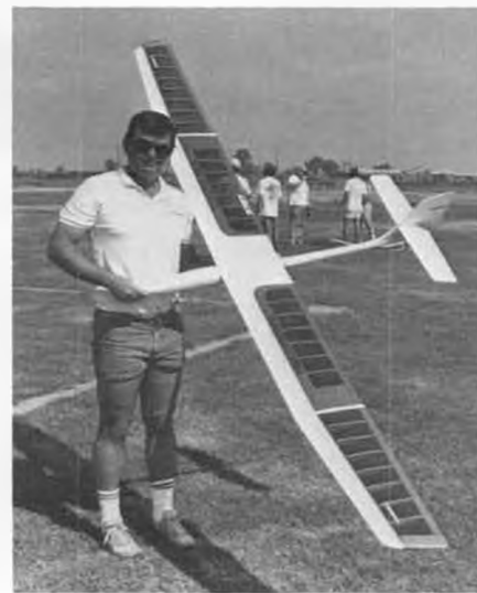
Ed Holder and the Airtronics Cumic Plus, a contest ship you can build as a 100- or 118-inch span model with or without ailerons.
