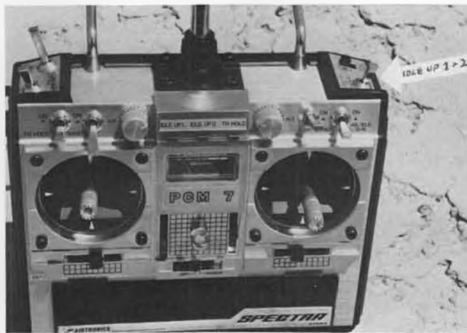
Three-position switch for Idle Up 1, Idle Up 2, and Normal.
