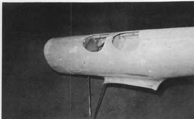
The fuel tank is removable from the front cockpit. Lower wing fillets and front access doors and headrest complete the fuselage.
