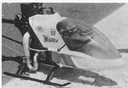
X-Cell 60's unpainted part of canopy shows fuel tank (arrow).
