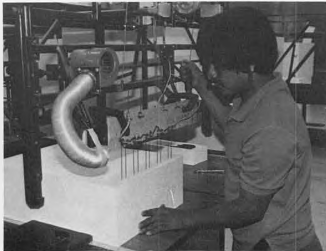
A worker operates the industrial hot wire cutting machine at the Star-Foam Company in Vista, California.
