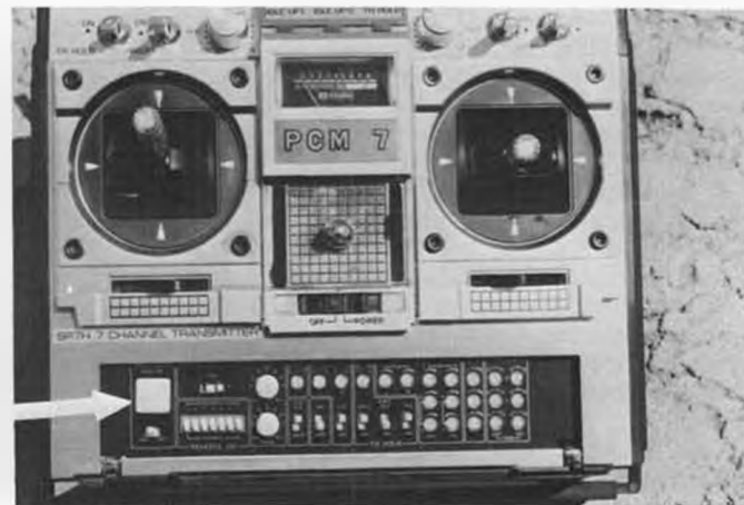
Front panel lowered to reveal trimmer dials and fail-safe button, shown by arrow.
