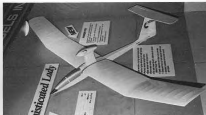
Goldberg's Sophisticated Lady is a good first or second model. Same basic construction as the Gentle Lady, with laminated vertical stab and extended sheeting on the wing, and a canopy with cockpit.
