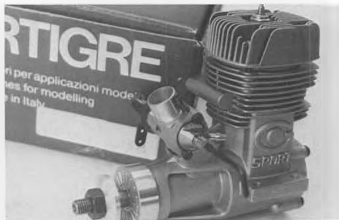
The engines have identical outward appearances, and have either "40" or "49" embossed above the word Sport. The G-40 is better-suited for the novice R/Cer as performance figures show a slower idle.
