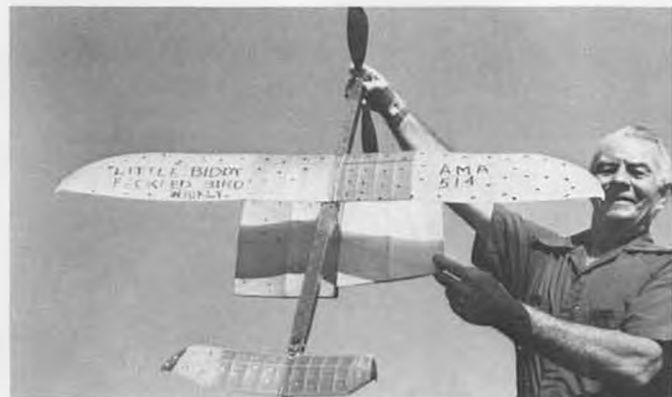
George Perryman's Little Biddy Speckled Bird Whirly with square rotor on underside of fuselage. It holds AMA Category I and II autogyro records. Photo: David Raymond.
