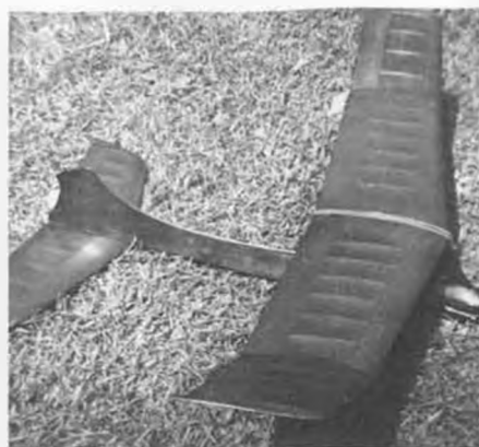
The Meteor I by Ed Mate. Note floating tab, used on left wing of original model. Later designs, including this month's 3-view, omit this feature from the model.
