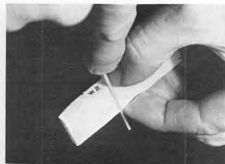
Make a notcher from a piece of 1/16x1/8 spar stock using sandpaper along the edge. Sand-in notches on rib stack.
