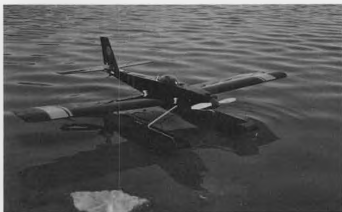
Gage Cauchois' Ridge Rat, usually a slope soarer, here is equipped for ROW. Floats do slow down the Astro 05, so he's going to try a cobalt 15 with 12 cells.
