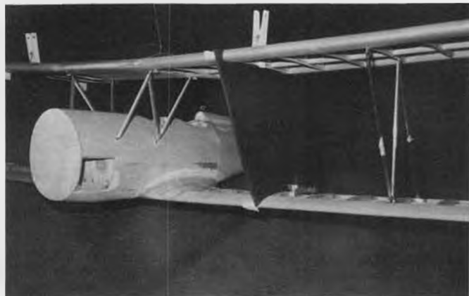
The top wing can be accurately mounted by making simple jigs that hold it in place while the cabane and 'N' struts are fit.
