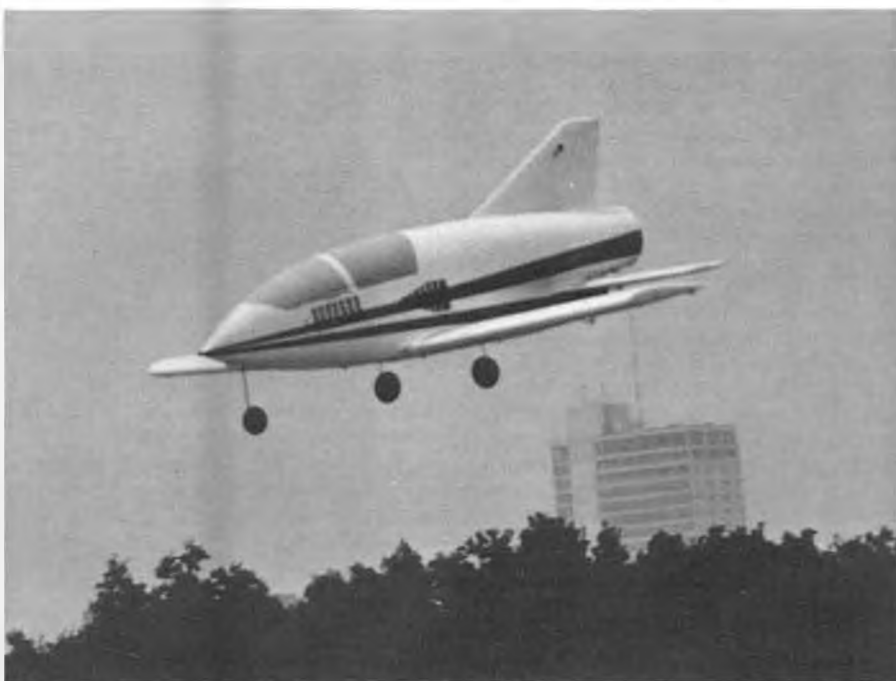
Faster than a speeding bullet, or at least it seemed that way, was Jim Barrett's BD-5 powered by a Byron fan and an OPS .65.
