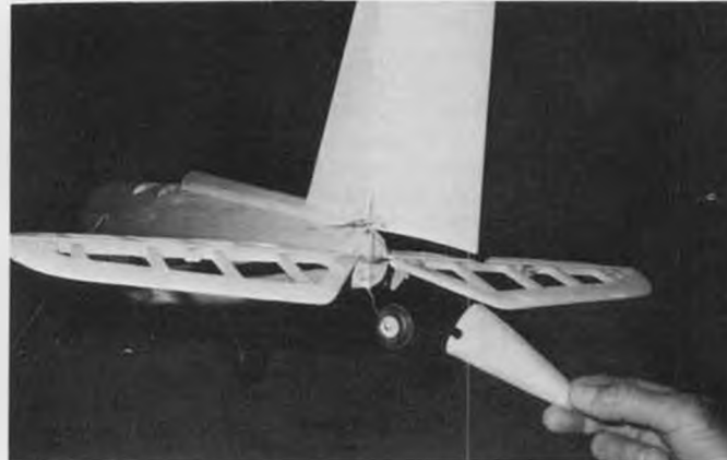
Tail cone is bonded or screwed into place. Picture shows generous rudder area.
