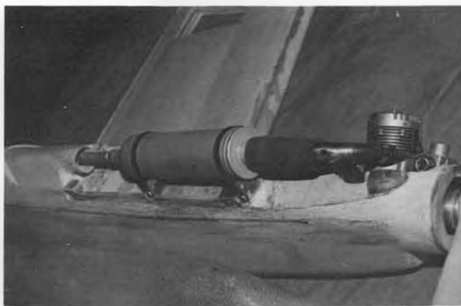
Magic Muffler will be completely covered by the fiberglass canopy of this .40-size sport model being built by Bob Carpenter of Australia.
