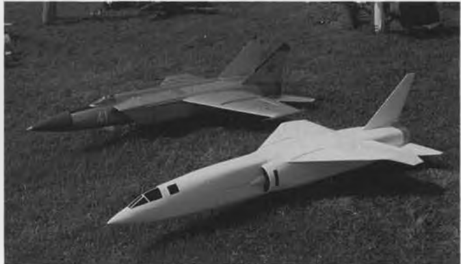
Two of Reg Smith's own-designed scratch-builts include a Mig 25 (two O.S. 46's with Turbax/Micromold fans) and English Electric TSR2.
