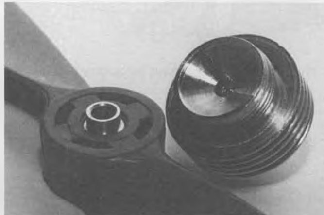
The turned aluminum insert fits into props made for larger engines and provides precise centering. The combustion chamber of the #315 glow plug matches that for the high performance Cox Tee Dee .049 engine.
