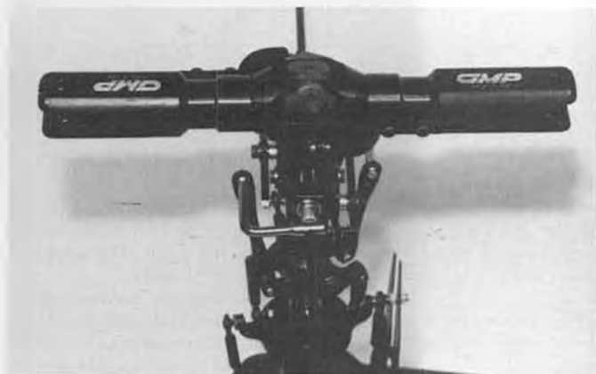
Also on display at Toledo was the new GMP FA1 rotor head, a beautifully designed and built piece of machine work. Absolutely no slop, and it has a 90% Bell-Hiller mixing ratio for superb stability. Not inexpensive, but for those who demand the very best, this is it.
