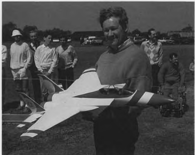
The famed Alex Cornish Trestrall's scratch-built F-15 features a fiberglass fuselage and two O.S. .25/Kress RK 720 fan systems. Great flier!
