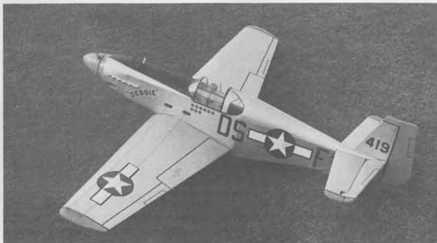
An original design built by our author several years ago featured foam wing, fuselage, and tail surface cores covered with .008" Mylar. See text for pros and cons of this construction.
