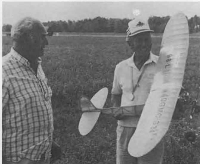
3. Sal Taibi gives Bob's full-size Wasp the once-over. With a Brown Jr. up front, this five-footer really performs. Note triangular fuselage aft of pylon.
