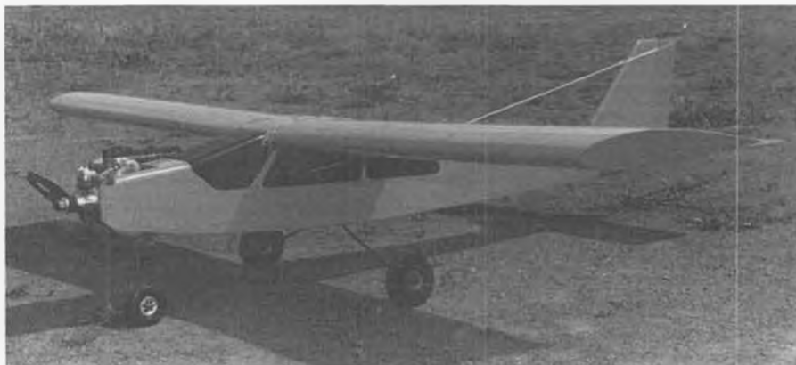
This month our columnist reviews the "Starhawk" as produced by Thorpe Engineering Corp. Clean lines make for snappy performance. Oversize wheels were fitted for operating off of a dirt strip.
