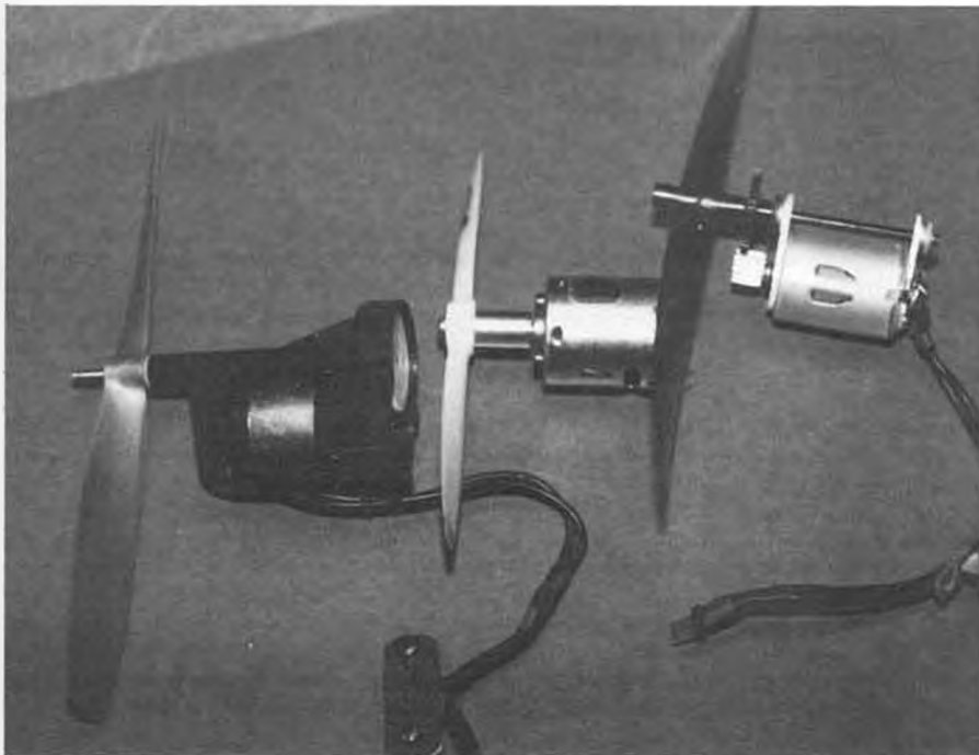
Three of the power systems used by Jack Dobbins are, from left: MRC's Cessna 177 geared unit, the Hi Line IMP 30 direct drive motor, and the geared system from the Cox "Kitty."
