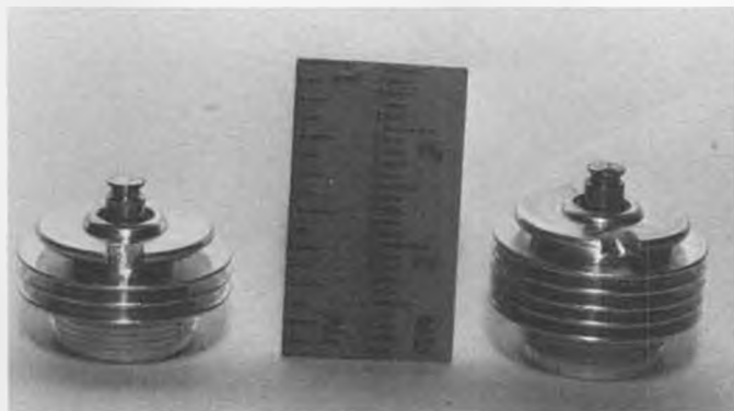
On the left is the standard Cox #325 glow head with three cooling fins, as used on the Black Widow. The new Texaco .049's #315 glow head has five cooling fins that provide added cooling.
