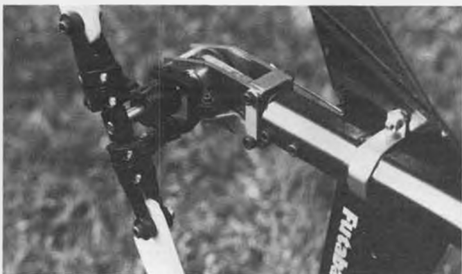
Our author uses the GMP Legend's tail rotor assembly on one of his Storks because he likes the all-metal construction and triple bearing blade grips.
