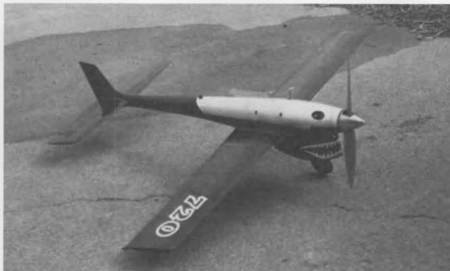
The nose trim on George Lieb's Formula 40 speed ship should be good for an extra ten mph at least. Power is a K&B .40 with a few Nelson parts thrown in for good measure.
