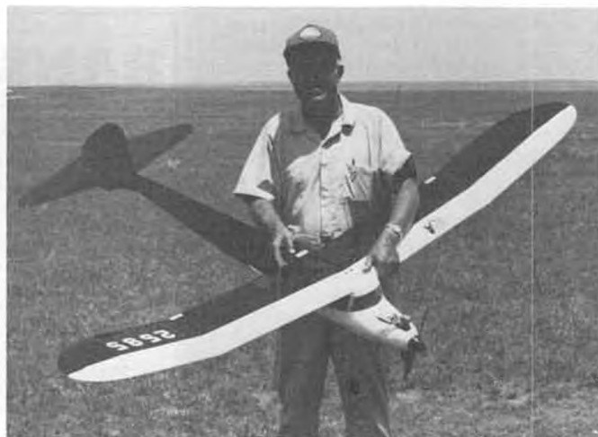
10. Good-looking Andrew Peterson "Cruiser" by Ed Smull was scaled up 150% to make it large enough for an O.S. .40 four-stroke. Model features a high aspect ratio wing and long tail moment. Ed reports it's a fine flier.
