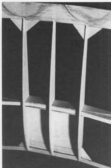
Wing spar has 1/16" ply doublers on both sides. Spar must be spruce or basswood, not balsa, for adequate strength.
