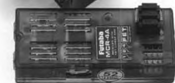
The MCR-4A four channel receiver/MOSFET speed control weighs just 1.5 oz. and can easily handle 280 to 540 size electric motors. 1.24" x 2.92" x 0.63"
