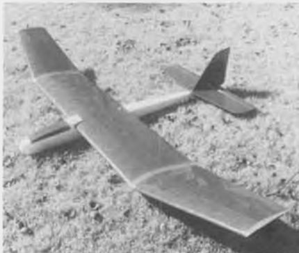
From Alabama's Rick Durden comes this photo of his reduced Olympic 650, scaled down to AMA Class A hand-launch size. Rick says it flies well at 15 oz., 430 sq. in.
