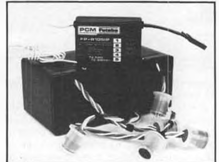
The Cynpahap receiver, with a Futaba Conquest receiver perched on top for size comparison. Note the large number of conductors in the servo leads and the monster plugs at the end of each.
