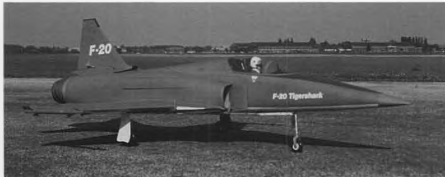
A K&B 7.5/Thorjet fan combo powers Ron Sweeney's 8-3/4 pound Northrop F-20, built from Thorpe plans. In the U.S., Thorpe plans are available from Bob Holman.
