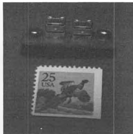
Homemade fuse holder for ultra-small electrics mounts in the fuselage side with the terminals exposed on the outside; plugging a fuse in place automatically turns on the motor. Simple and light, and it gives the added protection of having a fuse in the circuit—a good idea on any size electric. Photo from Jack Dobbins.
