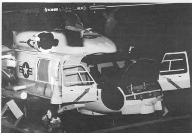
Mike Robin's awesome looking Sikorsky SH-60B uses X-Cell mechanics, a Schluter four-bladed head, Rossi .61 engine, and weighs 14 pounds. Drops torpedos and has blinking LED's on the instrument panel.
