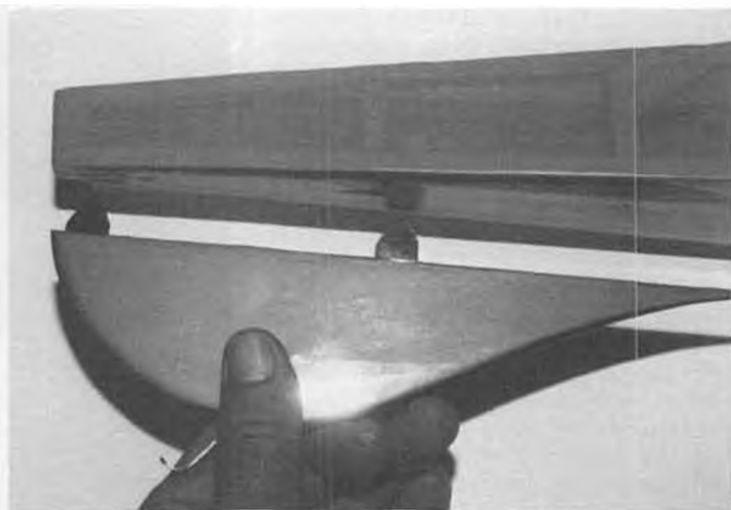
Two small tabs of .007" carbon fiber strengthen the sub-fin mounting to the fuselage.
