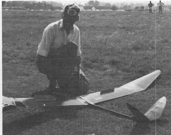
Nicely built Bird of Time variant by George Chastell spans about 12 feet and sports an interesting V-tail arrangement.
