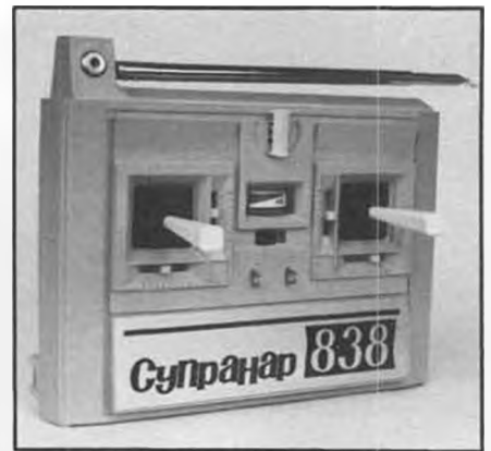
R/C, USSR style! Would you believe this Russian Cynpahap 838 system was considered "modern" in that country as recently as 1983? Four channels, no bells and whistles at all.
