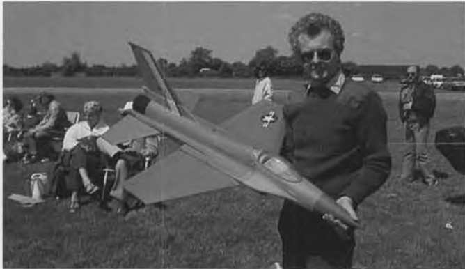
Graham Dennets converted a prop-driven F-16 (a Leicester Models kit) to a ducted fan using a K&B 7.5/Thorjet system.
