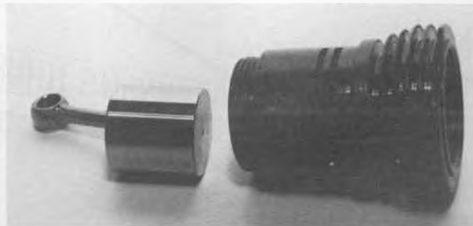
The success of Cox engines is largely due to the precise machining of their pistons and cylinders. The whole piston is copper plated, then the O.D. is ground to finish. Cylinder has slight taper—piston fits tightest at TDC.
