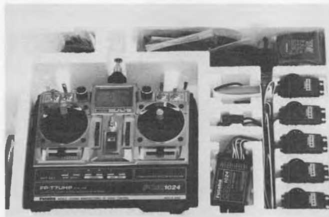
The Futaba 7UHP system comes with a 1000 mAh Ni-Cd receiver pack, which is big enough to run both the on-board radio and a yaw rate gyro. The S5101 servos replace the old S130's. Five servos are supplied.
