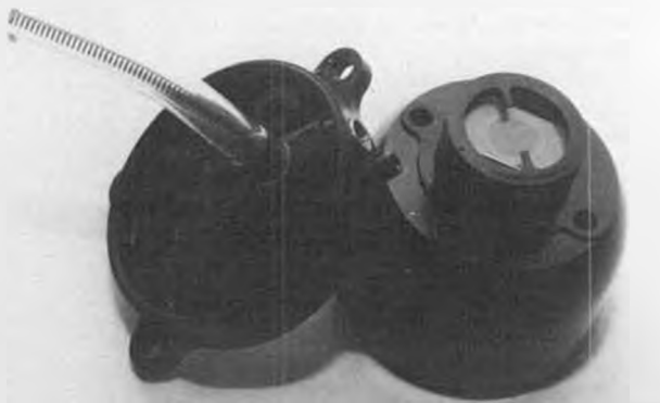
This view shows the special tank and new lightweight backplate. Top hat style retainer for the reed valve replaces the old spring retainer.
