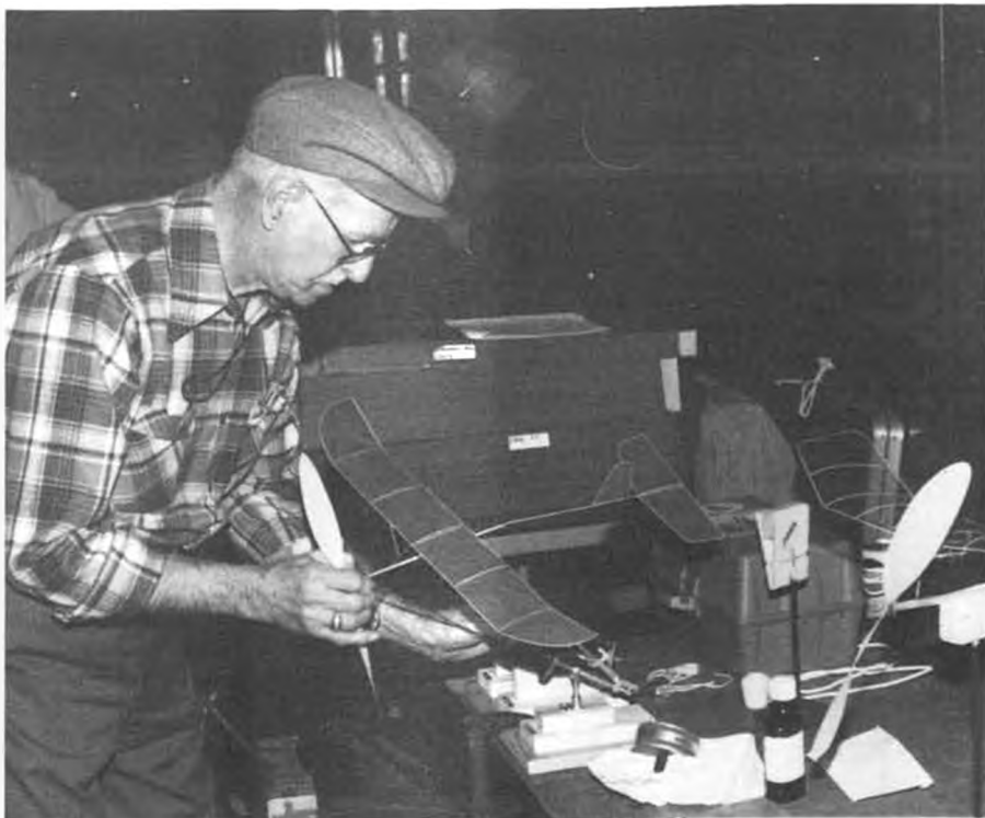
Like all indoor models, Easy B's require a delicate touch. NFFS founding father, Carl Fries, transfers a fully wound motor from a torque meter to his condenser paper covered ship.
