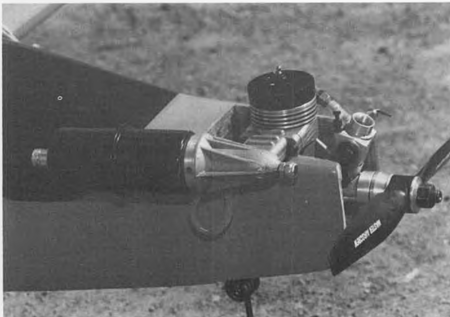
Our author powers his Starhawk with a Rossi .40 equipped with a J'Tec "Snuf-Ler" muffler, which does an excellent job of taming down the Rossi's notoriously loud exhaust. No drop in rpm, either.
