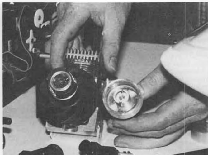
The self-aligning clutch on the Excallbur. Our columnist plans to discuss the importance of clutch alignment in a future "Chopper Chatter" column.
