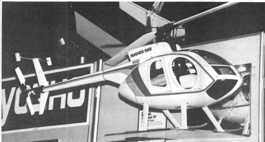
This Hughes 500 is one of three scale retrofit body kits that Kyosho is importing for its popular Concept 30 helicopter; the others are a Bell Jet Ranger and Hughes 300. All are molded plastic.
