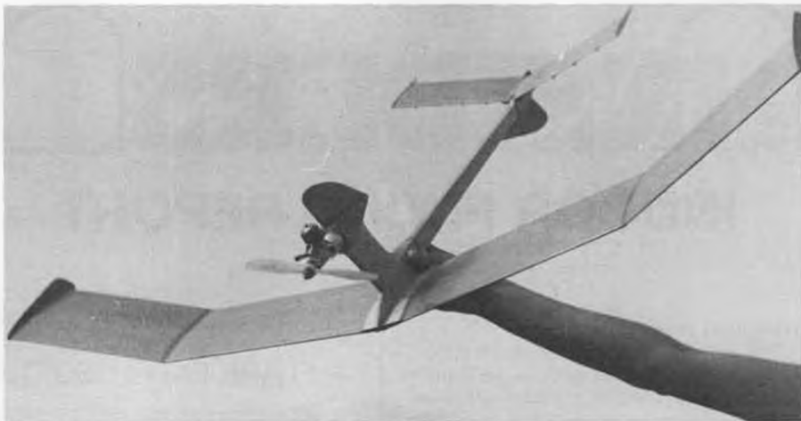
At first glance you probably thought this was some sort of canard, but it's not. It's an all-balsa 1/2A ship built by Keith Hoover in 1961 as an experiment in VHTL (very high thrust line) design. Note the triplets and dihedralized stabilizer. Holland Hornet engine. More details in text.
