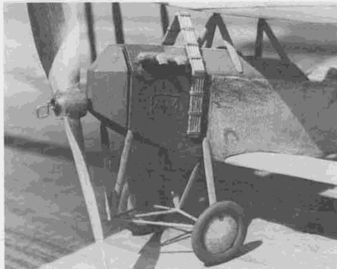
Strut arrangements and cowling details of the 120-hp “Ack” are clear in this photo. Plans also show details of the later 160-hp variant, which had a more conventional nose and landing gear.
