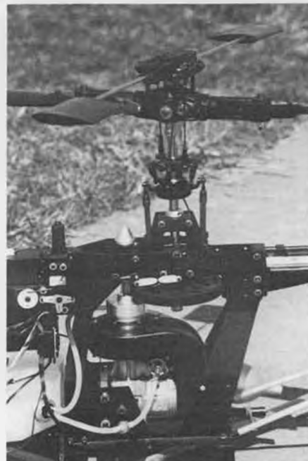
The soft, individually flapping DDF main rotor head gives the Stork extremely docile hover and forward flight characteristics.
