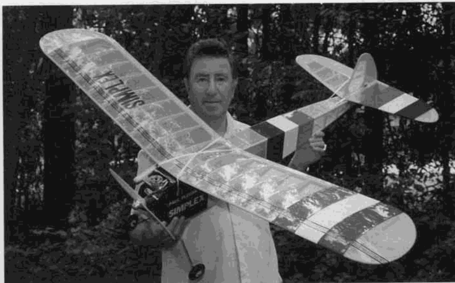
Stu used transparent yellow film on the top of the wing and stab, opaque dark blue on the bottom. Dark colors make for excellent in-flight visibility, especially at high altitudes.
