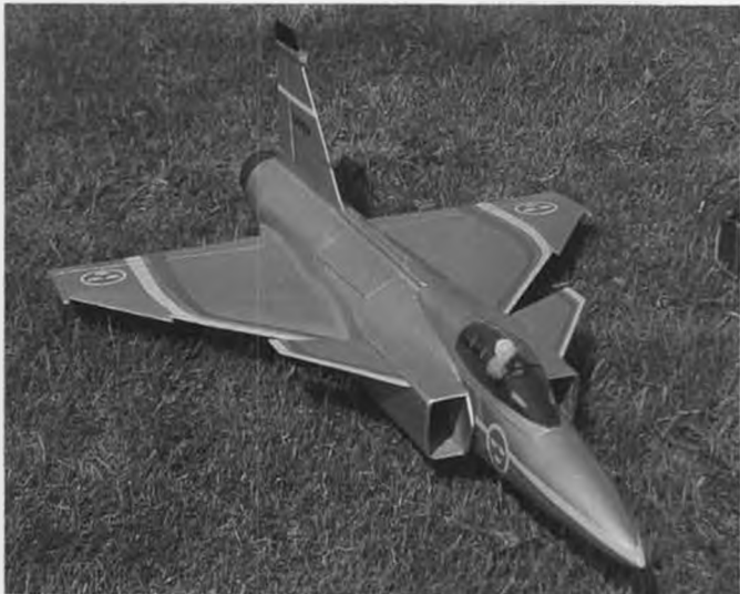
Interesting SAAB Gripen canard jet fighter with O.S. .46/Thorjet power was scratch-built by John Richards.
