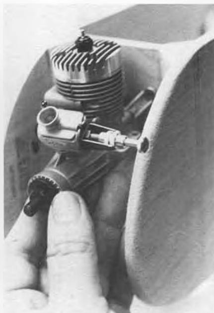
The K&B .20's spider mount works ideally. An aluminum or glass-filled nylon radial mount or hardwood beam mounts can be substituted for other engines.
