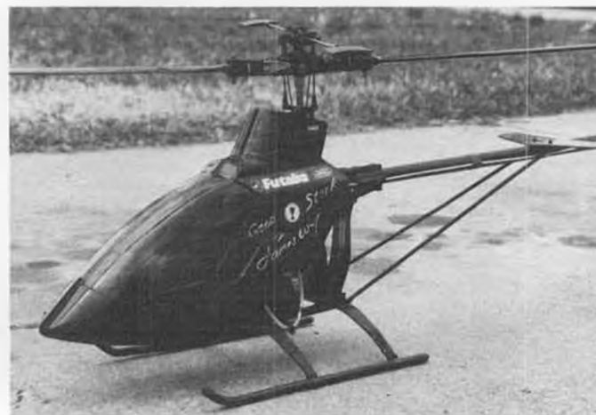
Always after more speed, our author added a fairing in front of the mixer and swashplate to reduce profile and parasitic drag.
