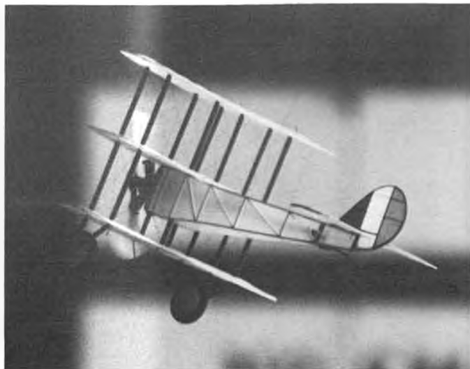
Cute Caproni-Pensutti triplane by Rich MacEntee flies well despite zero dihedral. Photographed by Jake Larson at MacDIII AFB.
