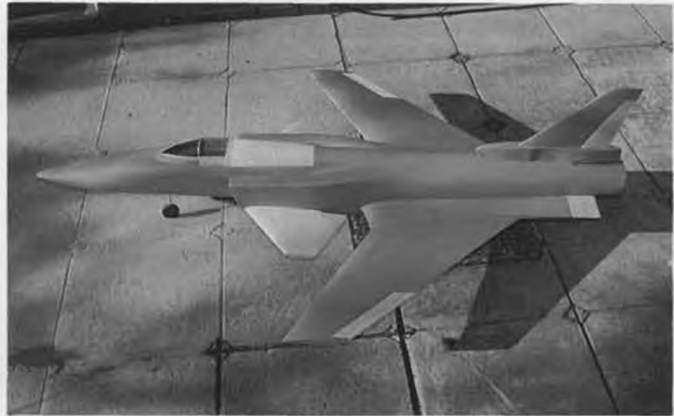
Two more shots of the partially completed Grumman X-29, to use a Picco .80/Byrojet fan setup. The full-size X-29 is said to be so unstable that the pilot could not even begin to fly it without help from on-board computers. Let's hope this one handles a little easier!
