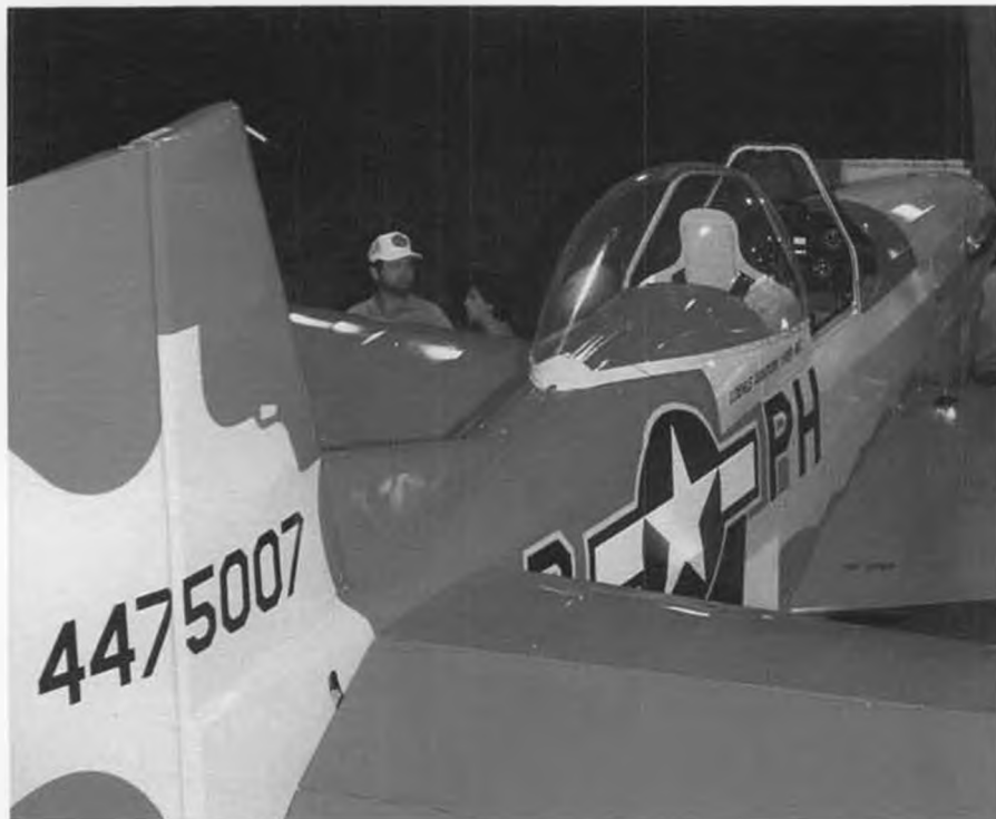
Mike and Carl Loehle brought their ultra-light/homebuilt 3/4-scale P-51 to Atlanta, and it was a real show stopper. Built like a typical model, with wood longeron box frame, ply bulkheads and formers, and wood stringers. Had retractors, Rotax engine, beautiful bubble canopy. They took over the late Gerry Ritz propeller business.
