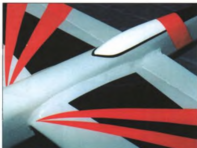
The fillets on this stunter built by our columnist turned out badly, due to paint bubbling. Text tells how to avoid this problem.
