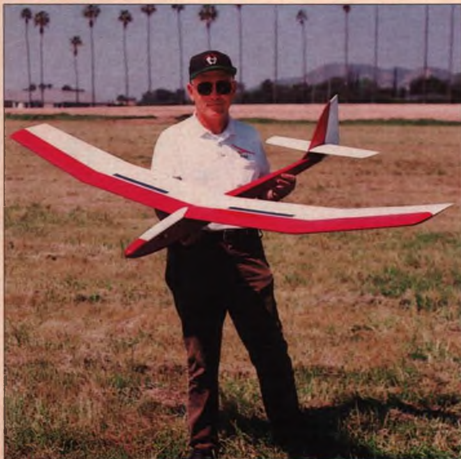
Larry Jolly divots the turf right on time and right on the center of the landing strip. It isn't pretty, but it is effective! It's also a testimonial to the strength of the Volant's fiberglass fuselage. Wings are a conventional, all-balsa, D-tube polyhedral design with capped ribs and spoilers.
