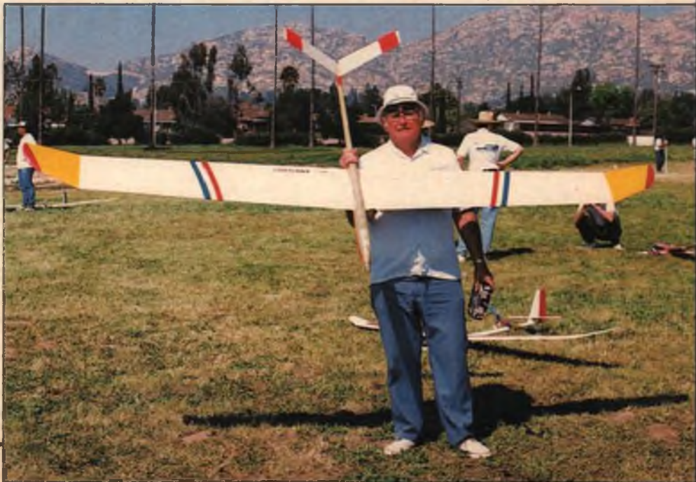
Bob Brown used one of Fred Sage's three different sizes of pre-built aftermarket V-tails to convert his Shadow into a "Shadow-V," leaving the wings box-stock. Bob says the modification makes the Shadow fly even better than before.
