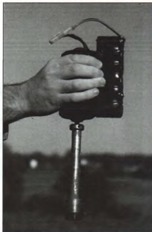
Ralph Dalesio made a cordless electric starter by taping twelve 1200-mAH NiCd batteries to his 12-volt starter. One charge lasts a whole day of flying. The batteries are strategically placed to give the best balance.
