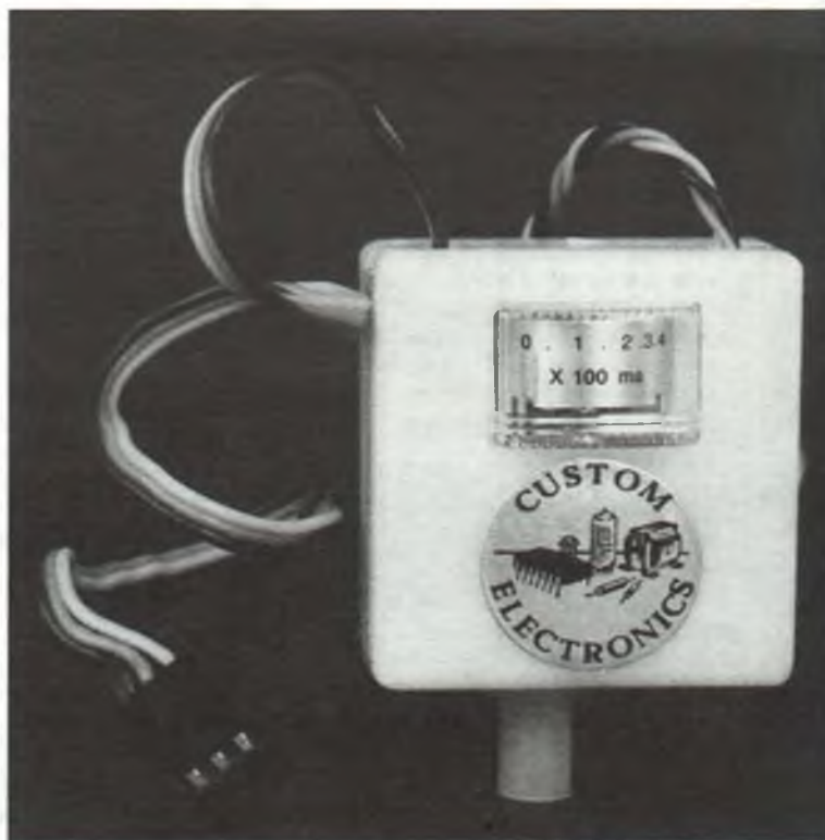
The Custom Electronics Servo Analyzer is a small transmitter meter type of instrument intended to show variations in servo operation, which are indications of possible problems.
