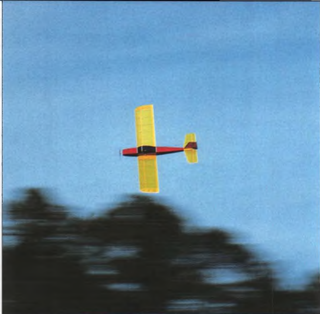
Low and close-in—the fun way to fly! The use of plenty of dihedral and rudder/elevator controls results in decent axial rolls as well as great snap rolls and spins. We've seen a video of this model in action and can attest to its aerobatic capabilities—including outside loops!
