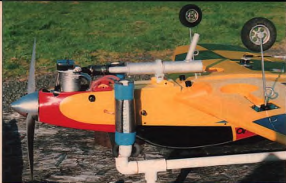
The new .91 short exhaust system from Advanced Aero Products installed on a Cursor/Saito .91 combo. Works great, and so does the airplane and engine.
