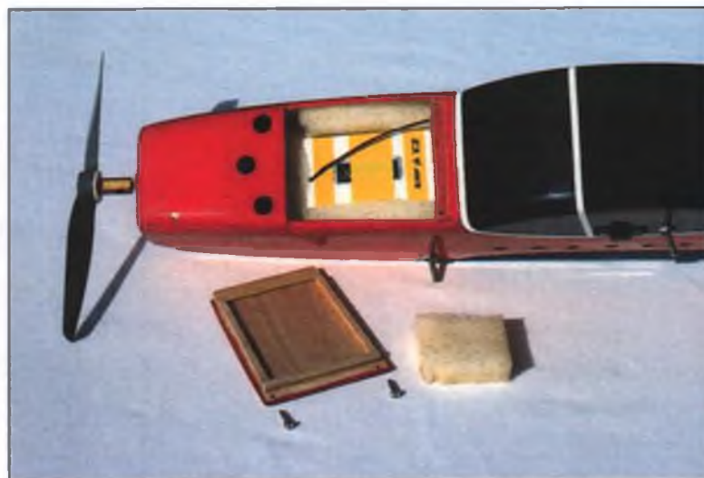
Removing the forward hatch reveals the Ace Silver Seven receiver; a High Sky on-off motor controller lies underneath and is taped to the receiver.
