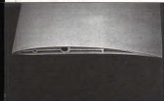
Molded ABS wing roots come already installed in the wing panels and have the brass tubes for both wing rods already in place.
