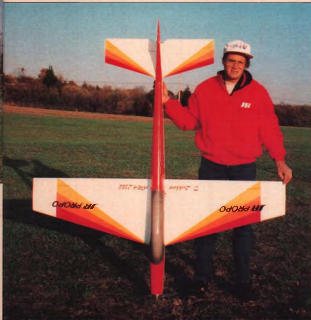
Dave Lockhart and his new Gymodels Elan. YS 1.20, JR PCM-10S, and only 8 pounds 14 ounces. Dave Lockhart photo.
