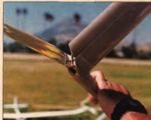
Close-up of Fred Sage's V-tail mod for contest ships. A small portion of the fin is left as a gluing surface for a balsa block stab saddle. The joined V-stab is glued to the notched balsa block, then the three elements are fiberglassed together. Complete job takes about two hours. More details in text.
