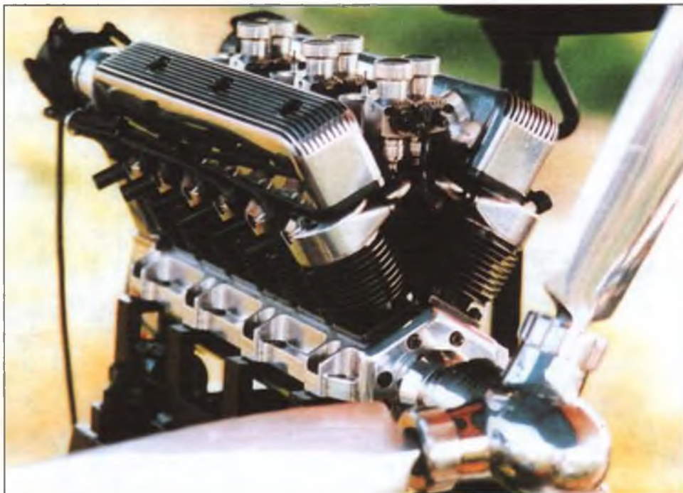
Master craftsman Wim Van Der Hoek of Holland turned out these incredible working examples of the machinist's art, a V-12 with variable-pitch prop and a two-row 18-cylinder radial. This is the sort of thing you'll find in Strictly I.C. , a magazine targeted at amateur machinists. Details in text.
