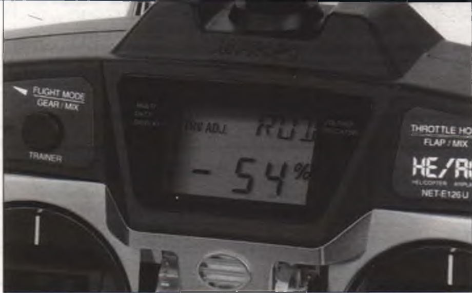
The clearly defined 7/8x1-3/8-inch Liquid Crystal Display screen is easy to read even in bright sunlight. It displays all pertinent condition and flight information.
