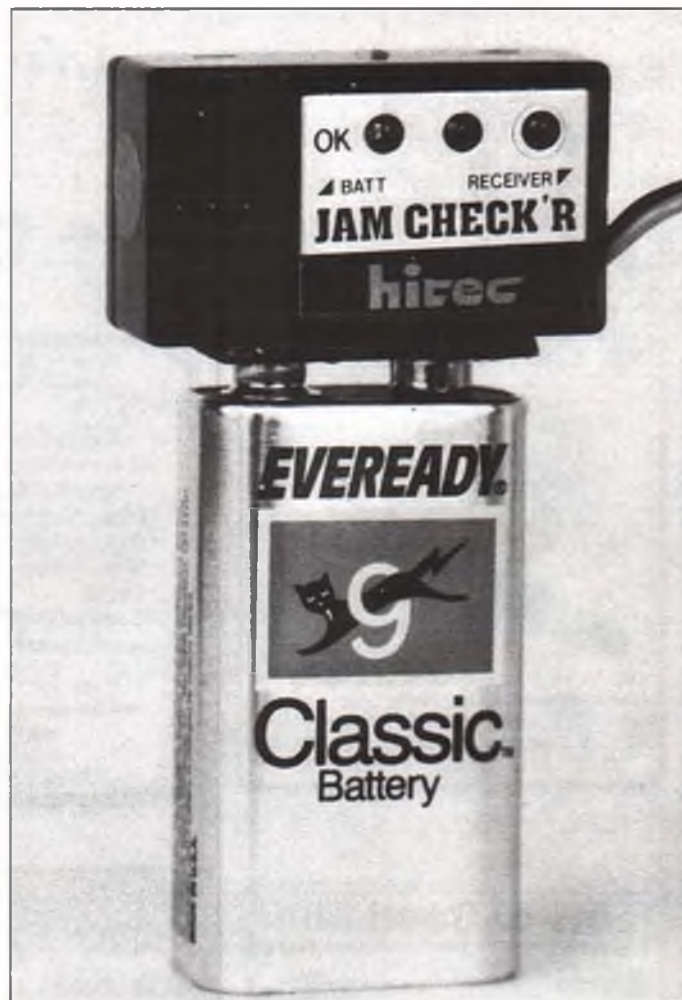
Seen here perched atop a 9-volt battery to illustrate its small size, Hitec RCD's Jam Check'r uses three different colored LEDs to indicate normal or excessively high current drains.
