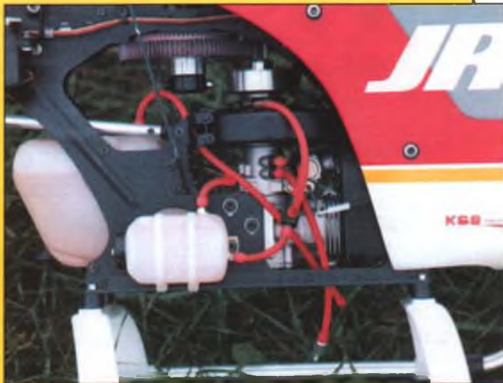
The plumbing in Len Sabato's Kalt Baron Alpha II helicopter, equipped with a ringed YS .61 SF. Note the small feeder tank on the side. With fuel lines running every which way, you can see why a pod-and-boom machine like this is so much easier to service than a full-fuselage model.
