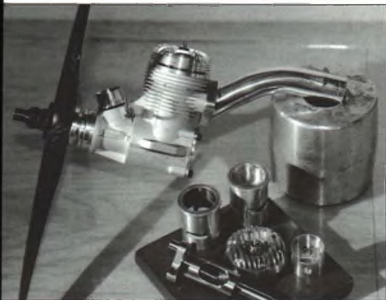
The Aero .40 is produced by Henry Nelson and Randy Smith for precision aerobatics.
