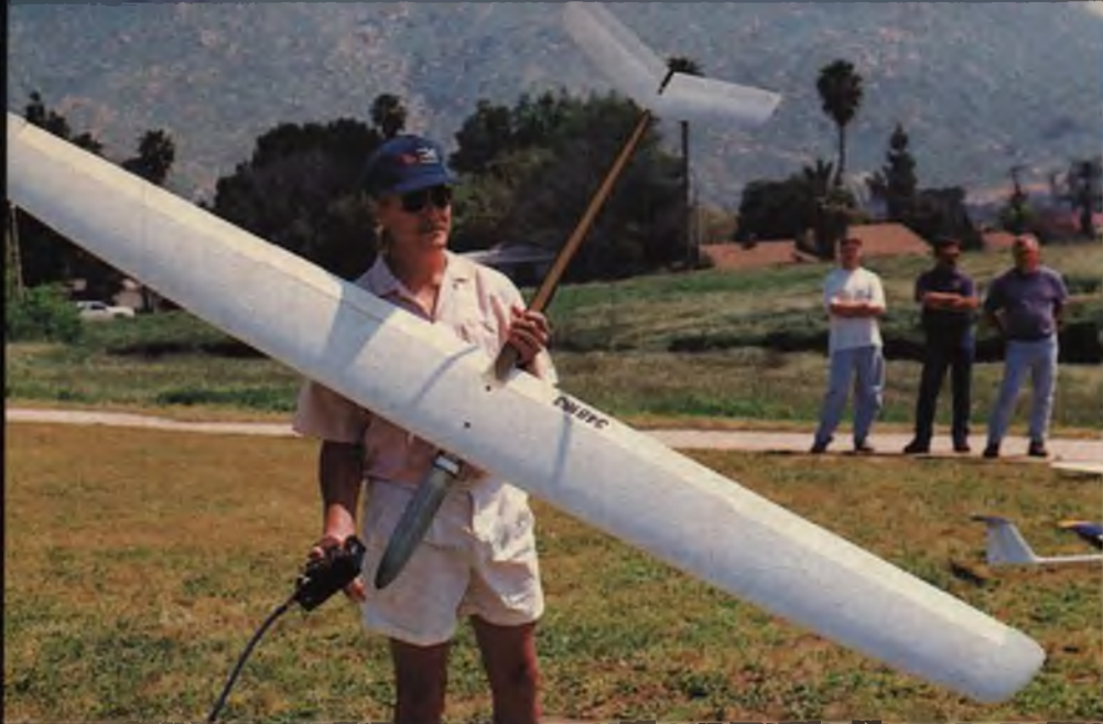
Jim Markle shows off his new F3B ship, the "X-cellent III" from Hans Mueller of Germany. All-molded model features extensive fiberglass-Nomex (honeycomb) sandwich construction in the wing and fuselage. Features the RG-15 airfoil, 107-inch span, 940 square inches of wing area, and 70 ounces. Contact Northeast Sailplane Products for availability and cost.
