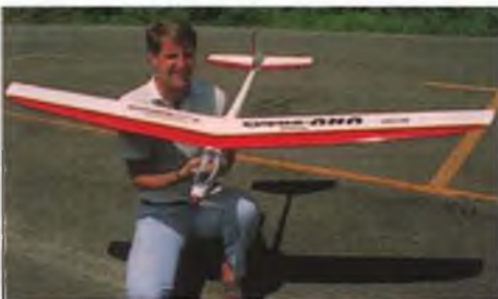
GR4207 Elektro UHU ..... $97.00 75" span soarer with ready built strong plastic fuselage and rib and spar wing.
