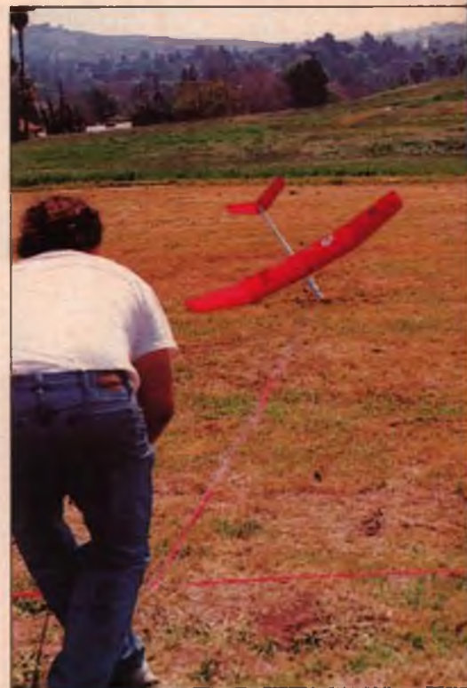
Larry Jolly divots the turf right on time and right on the center of the landing strip. It isn't pretty, but it is effective! It's also a testimonial to the strength of the Volant's fiberglass fuselage. Wings are a conventional, all-balsa, D-tube polyhedral design with capped ribs and spoilers.
