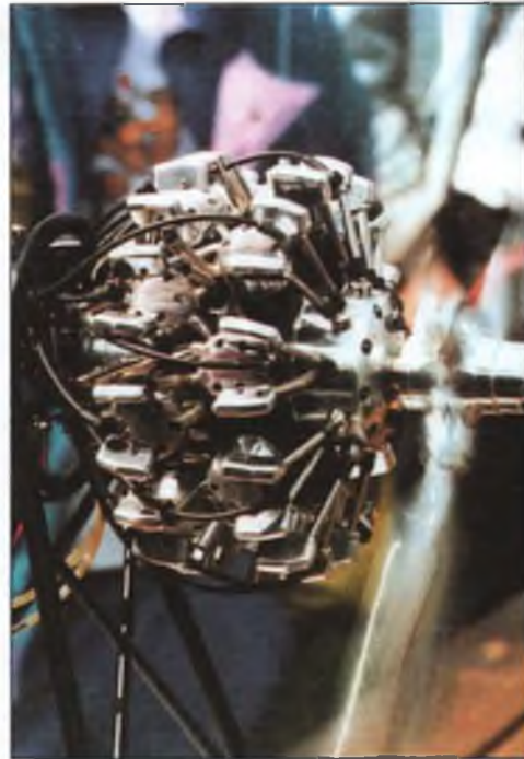
Master craftsman Wim Van Der Hoek of Holland turned out these incredible working examples of the machinist's art, a V-12 with variable-pitch prop and a two-row 18-cylinder radial. This is the sort of thing you'll find in Strictly I.C. , a magazine targeted at amateur machinists. Details in text.
