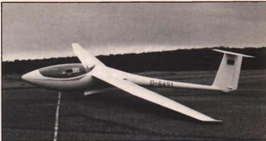
Inhoff Models International produces this impeccable, true-scale replica of the AS-W 24. The scale is 1/3.5, which results in a big 4.28-meter (14-foot) wingspan. Flying weight is 13 pounds. Very stable (Matt Inhoff reports one ship was lost O.O.S. when the airborne radio battery went dead) and easy to fly and yet very aerobatic.
