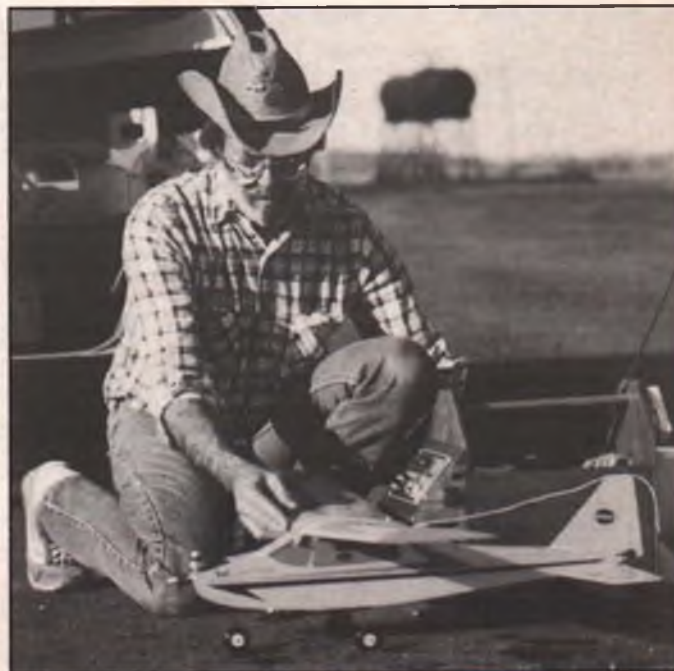
The author gets some run-in time on the Dragonfly .049 before the Katydid's maiden flight. As Bill relates, running a few tanks through a new engine before sending it aloft can save you some embarrassment and a possibly broken airplane.
