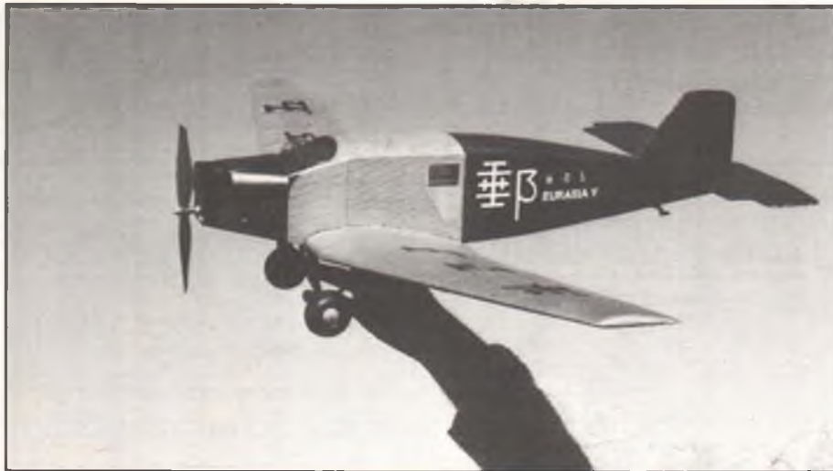
Tom Mallen II built this beautiful compressed-air powered Junkers W-33 "Eurasia" free flight scale model.
