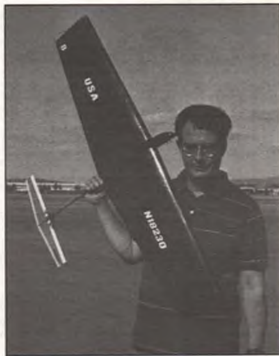
It's almost too beautiful to fly, and the designer/builder, Howard Rash (pictured), decided it was too much work, too! But this is the design Howard used in his last World Championships effort. It's made almost entirely of space-age materials, including lots of carbon fiber. Note the built-up elevator. Light, strong, and many hours of building time! It always draws a crowd at contests.
