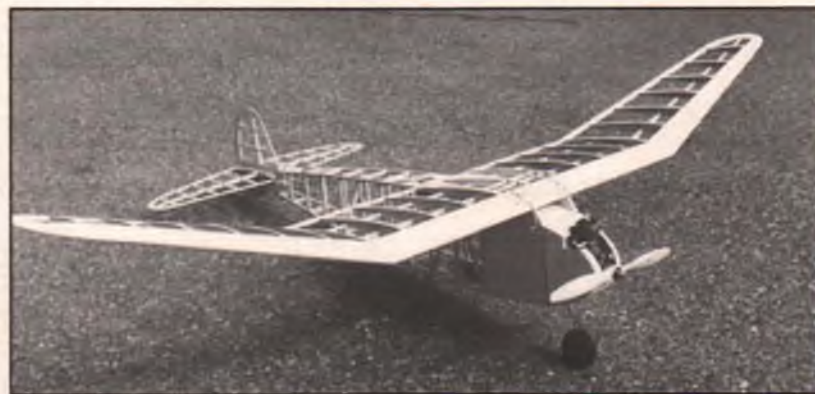
Framework of Bruce Augustus' structurally revamped (but still within SAM guidelines) 1938 Rambler, designed by Gil Sherman. One of the hot tickets in the Old Timer free flight game, the 72-inch span Rambler is being offered in a two-sheet plan set by Bruce, showing such niceties as aluminum engine mounts, screw-adjustable rudder tab, etc. Also included is an eight-page booklet of building and flying instructions. Going price of the complete package is $24.95 postpaid, direct from Bruce at P.O. Box 450, Sun Valley, ID 83353.
