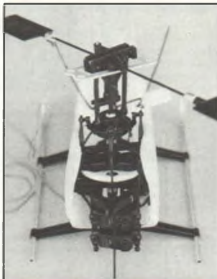
Aft view of the main rotor assembly installed in the fuselage pod, prior to installing the tail boom. Simple and light and amazingly tough—as Roger was soon to learn.
