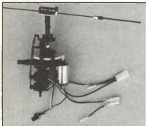
The completed main rotor assembly. Builder is in R with installing the motor, servos (Futaba S133 micros seen here) and pushrods; everything else on the rotor assembly is pre-assembled at the factory.
