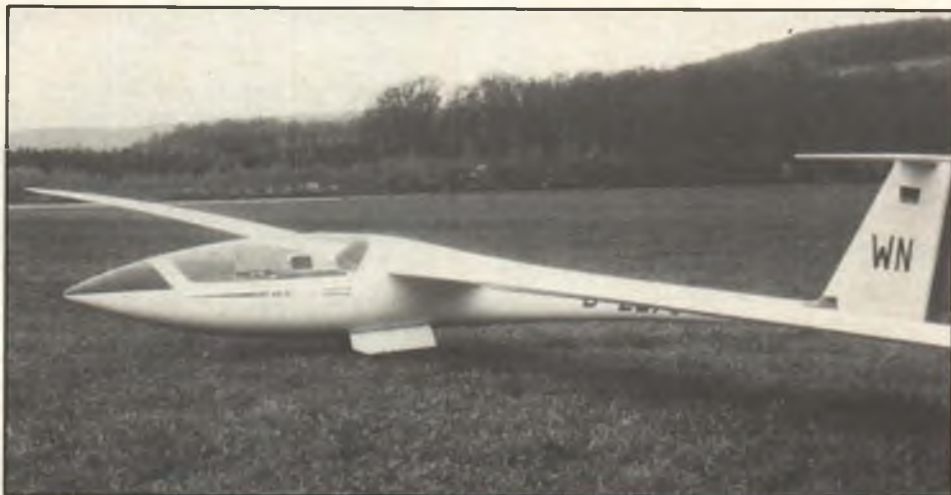
The 25-meter Schleicher AS-W 22 is a modern supership capable of truly phenomenal performance, and Inhoff's 1/3-scale model (27.3 feet!) has performance to match. Built-in water ballast tanks in the wings can boost the flying weight from 44 to 55 pounds. The water can be jettisoned by radio if lift is weak.
