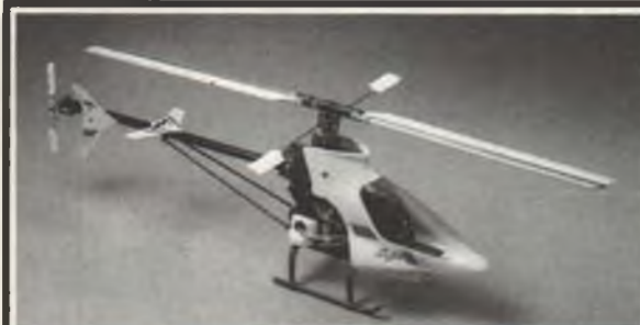
The completed main rotor assembly. Builder is in R with installing the motor, servos (Futaba S133 micros seen here) and pushrods; everything else on the rotor assembly is pre-assembled at the factory.
