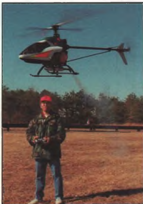
James checks out his flying buddy Alan D'Elena's XL-Pro. It's powered by an O.S. .61 FX with Hainl 666 muffler underneath.
