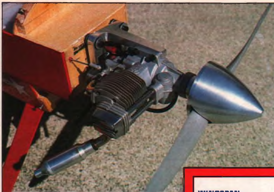
Power for the Laser comes courtesy of a pump-equipped O.S. 1.20 Surpass II four-stroke mounted on a very effective J'Tec Sauf-Vibe soft motor mount. Tre-Turn spinner adds a real touch of class.
