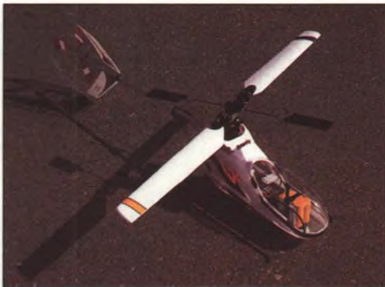
RC helicopters don't get any simpler than this, folks. The HyperFly requires only two channels, for left/right and right/left cyclic; a large clear plastic hub takes the place of the normal ball rotor; and there is no motor control, flight duration being limited by the battery pack. Flights typically average 3-1/2 to 4 minutes.
