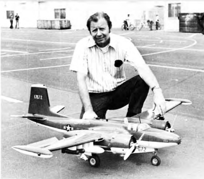
Ray Smith, Lawndale, Cal., and his A-26A. Span is 72", weight 15lbs. Uses two Fox .60 Eagle engines and is flown on seven (7) lines!
