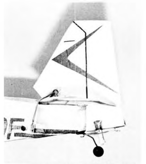
Close-up of the DT rig. Note also lifting stab airfoil. All photos by author.
