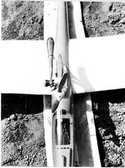
Cox .09 with tuned pipe powers this glider by T. Hirasawa, Japan. Flood-off stop by R/C.
