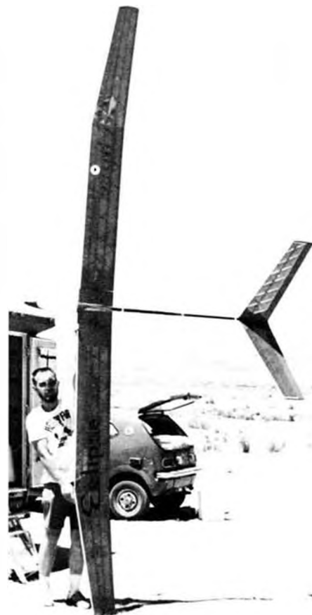
Hal Cover and his monstrous but graceful "Eclipse", well named for what it does to the sun when aloft! Span 15 ft., fish pole boom.
