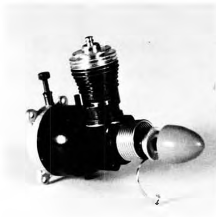
Latest Cox .049 is the "Black Widow," an updated version of the Golden Bee. Twin ported.
