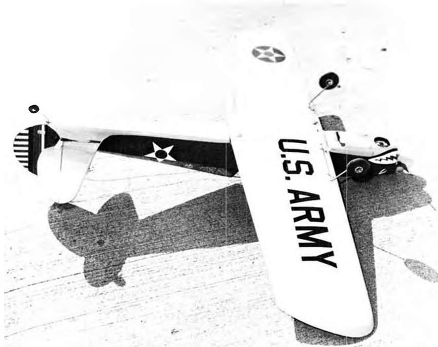
We're surprised that more pylon racers don't adopt the one-aileron system shown here on the P-40. Uneven drag should work in the pilot's favor during those knife-edge pylon turns.
