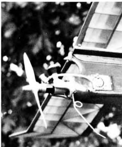
Business end of the FAIMan 7. Engine plate is drilled to take landing skid and set screw.
