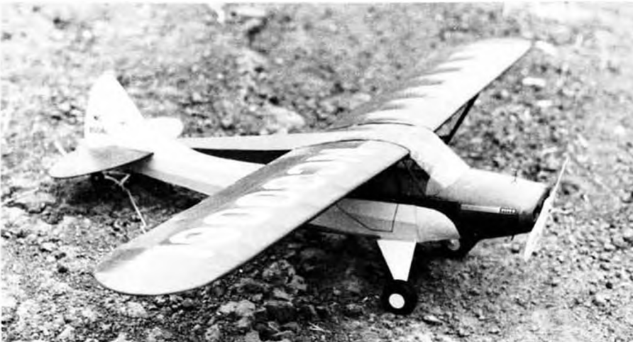
Sterling's Piper Super Cruiser as built by our Scale F/F editor. Ship was entirely trimmed by second flight, and performs superbly. Power is the Cox .020 Pee Wee.
