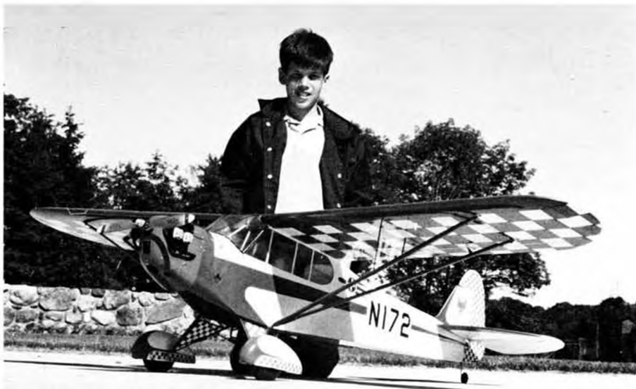
Span Aero's 8 foot Cub kit has been modified so that any one of three different versions may be built. Cowl and cabin area are of molded fiberglass. Wing spars are aluminum.
