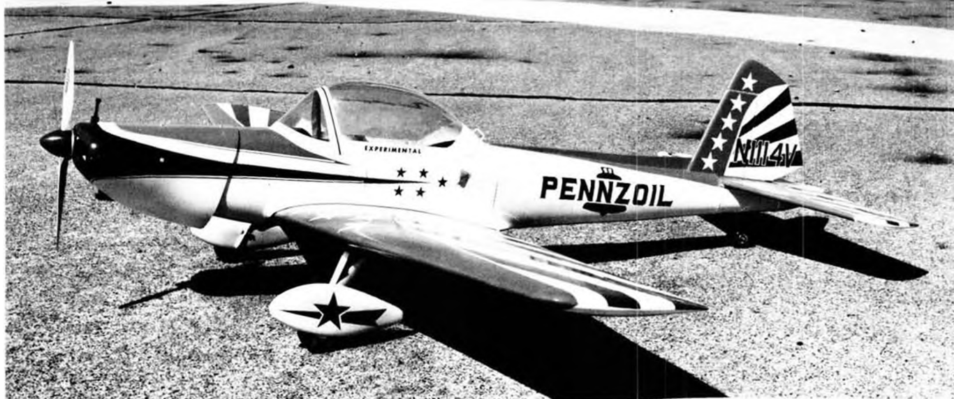
Sig's R/C Stand-Off Scale Chipmunk features the new "Kwik-Bilt" method of fuselage construction, which provides the detail of molded plastic combined with the strength of a 1/2" balsa crutch. Ship has foam wings and sheet tail surfaces, making for fast building. $39.95
