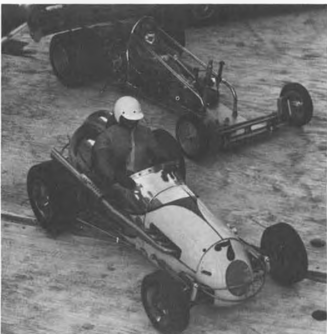
Ray Bell's winning concours car. Hand-formed aluminum body, front suspension with shocks, .15 powered. Looked great on track too.
