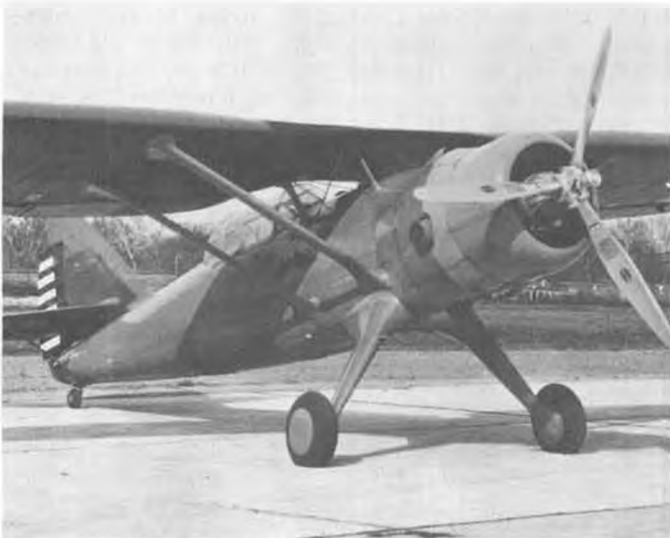
The last O-43A was redesigned to take a 725 hp "Twin Wasp" and had struts instead of wire cabane. Called the XO-46, it was good enough to earn a contract for 90 O-46A's.
