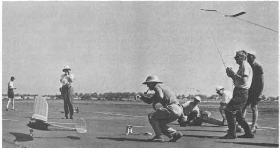
Cliff Schaible's Cleveland Playboy Senior R/C gets off with the pull of a Super Tigre .29 with 9-4 prop. A good action shot by Jack Humphreys.
