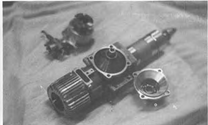
Specially built engine to fit in the turboprop cowl of the An-14M. The spare was not needed, as the two in the plane ran perfectly.
