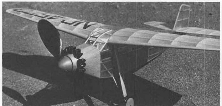
You can put a winding eye on the prop shaft if you prefer, but Bob chose to wind from an "S" hook. Thrust offset is put in for flying only in order not to mess up appearance when sitting.
