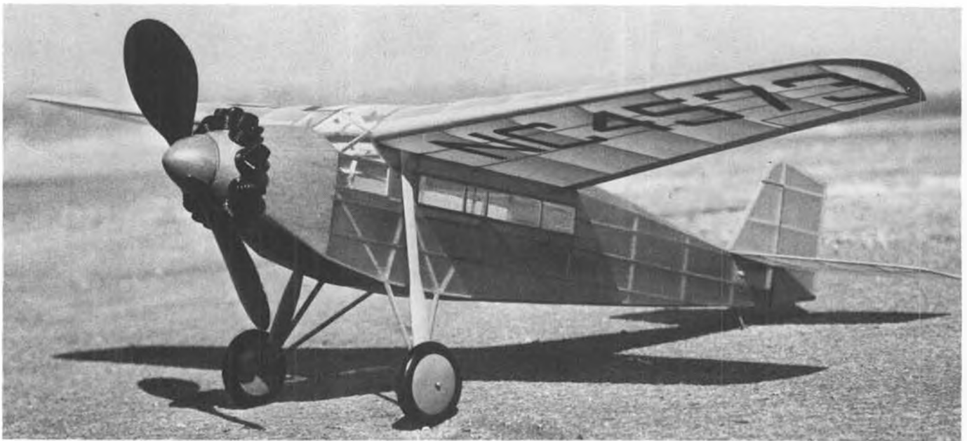
Thick wing section allows excessive strength without paying a weight penalty. Scale works out to .85 inch to the foot, so you'll have to carve engine cylinders or fudge something from Williams Bros. 3/4 or 1 inch scale plastics.
