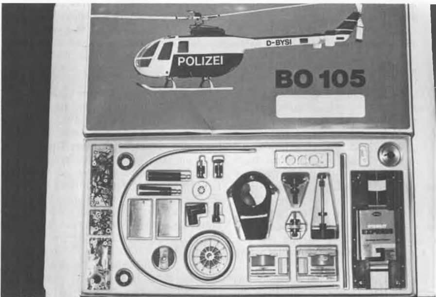
Neat packaging of the mechanicals for the Bolkow is a great help during assembly. Rotor head features adjustable pitch.
