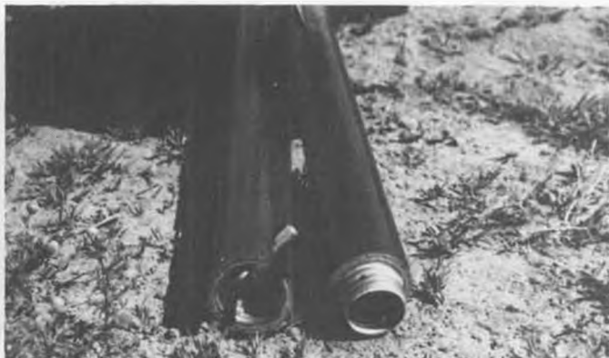
No, it's not a double-barrel shotgun. Glenn Coronel uses this light bulb base and receptacle detach system on his Unlimited. See text.
