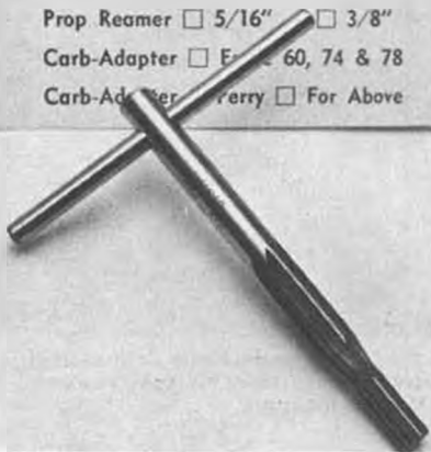
Special prop reamer cuts holes with parallel sides. By Rosie's R/C.
