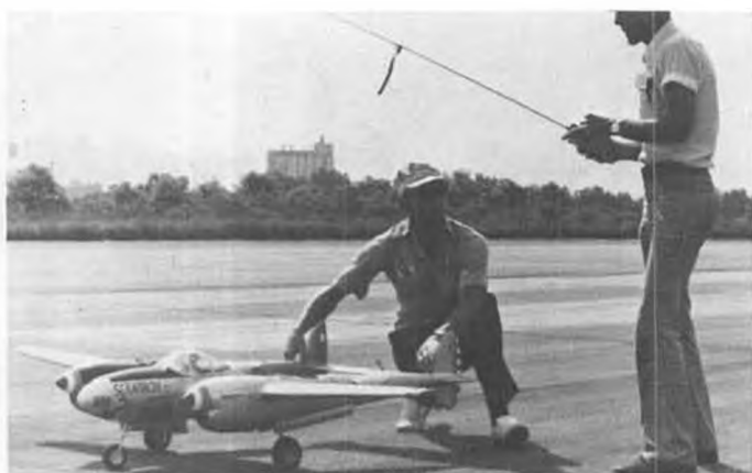
John made his own molds for the pod and booms. Additional heat sinks on the engines allowed them to run cool though enclosed.
