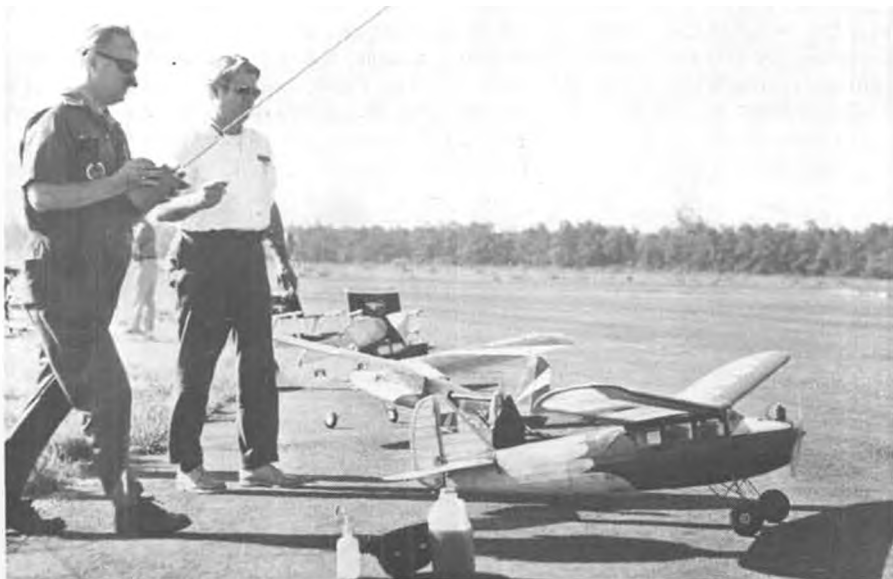
Fred Collins, Pittsburg, Pa., complete with cardboard mustache, flying his Forster .99 powered Super Buccaneer with radio. Engine swings a 17-6 prop. Note ailerons.
