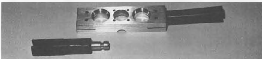
"See-Saw" and blade attachment for the Bolkow helicopter kitted by WIK and imported to the USA by Midwest Model Supply.
