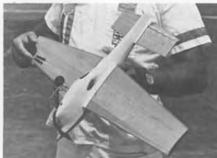
Underneath exhaust outlet created turbulence making control squirrely, OK in glide.
