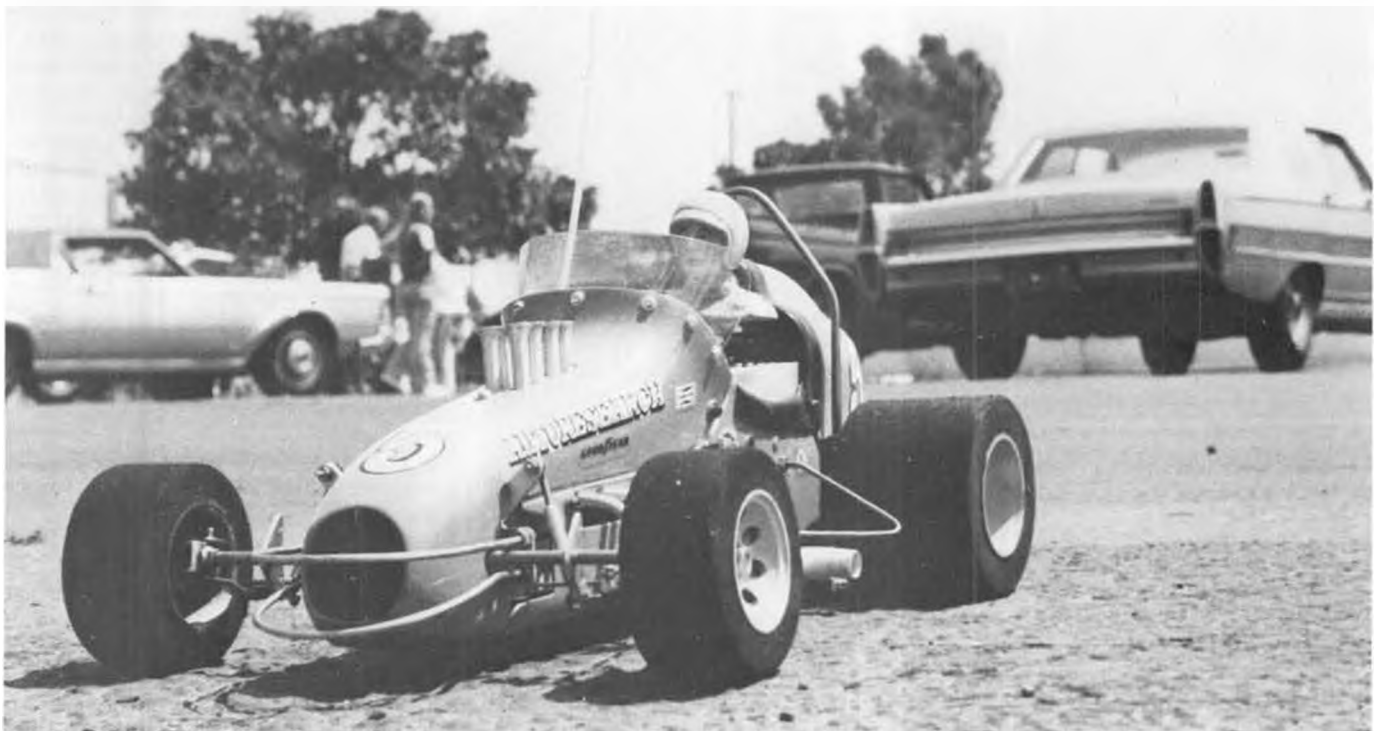
Sprint car by Jim Aubrey. Shocks, Pitman arm (movable) and stacks for appearance. Exhaust goes out bottom.
