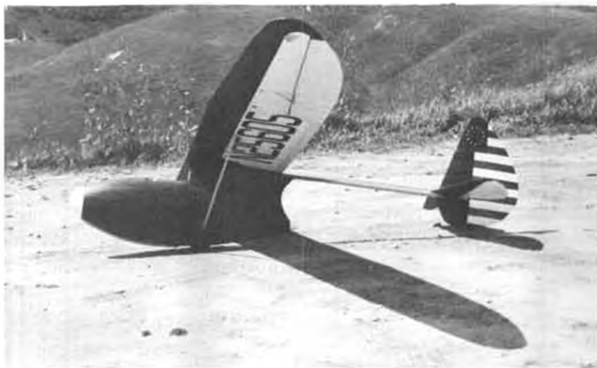
One of the most famous profiles in aviation, the epitome of pod-and-boom construction. Note the huge aileron area.
