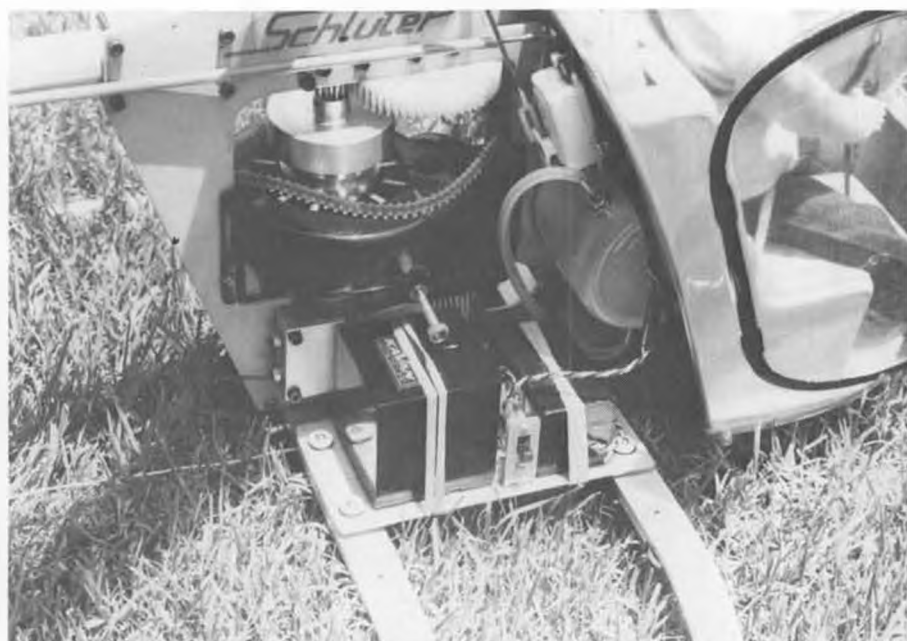
The Kavan Gyro installation on the Schluter "Heli-Baby." Note that a mounting plate has been installed, using vibration absorbing rubber grommets, directly onto the landing skid struts.
