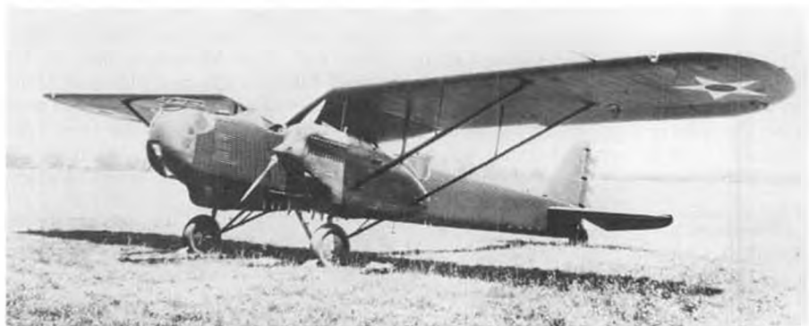
The XB-7 at Wright Field, fitted with Scarff rings on the barrel cockpits, and bomb racks for up to 1200 pounds of bombs. Useless little mudguards had been removed.
