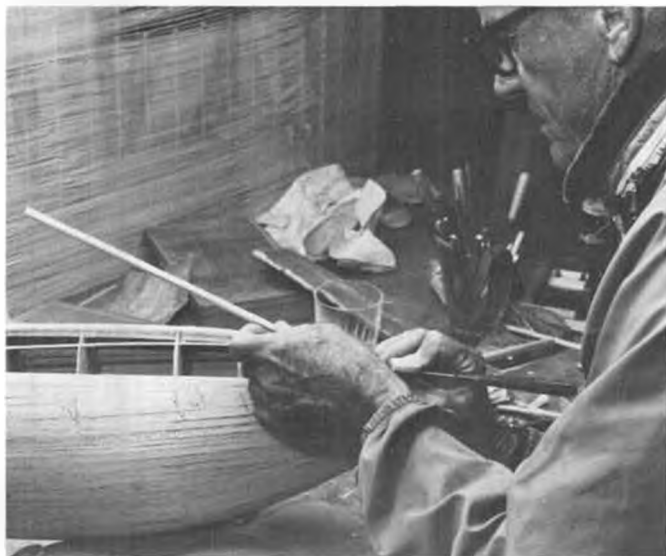
Fuselage planking is applied in small strips due to the compound curves involved. Note familiar modeler's equipment . . . a Band-Aid!
