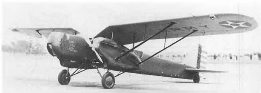
Two Conqueror engines flew the XB-7, with its wing area of 600 sq. ft., and maximum gross weight of 11,287, at a speed of 169 mph! Wheels retracted, but stuck out enough for landing.
