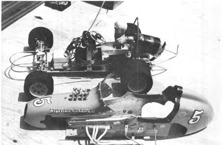
Body for Jim Aubrey sprint car was made by full scale midget car builder, Don Edmunds, of Autoresearch. Servos actuate through cables.
