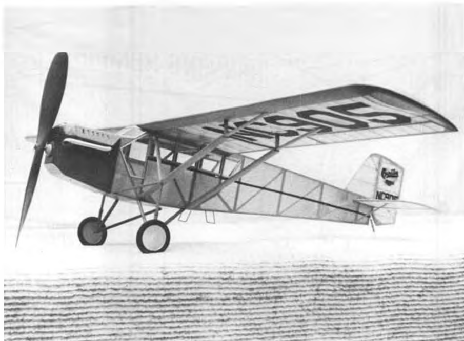
This Curtiss O-X5 Robin was built from Cleveland 3/4 inch scale plans by Phil Cox, Highland, Indiana. Span is 30-5/8 inches, and weight, without rubber, is 2-1/2 oz. Glen Goubeaux photo.
