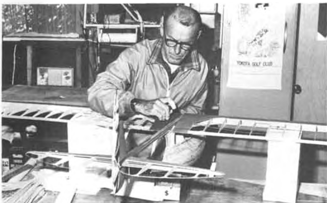
Test fitting the basic structure. The tail boom is made from a one inch diameter aluminum tube towel rack.
