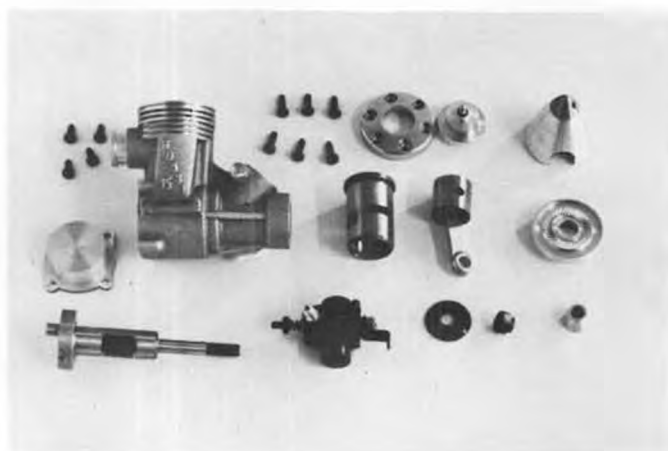
The disassembled Rossi .15 R/C, showing all of the basic parts. Bob Reuther had 9 perfect heats (landed with engine running) at '75 Nats.
