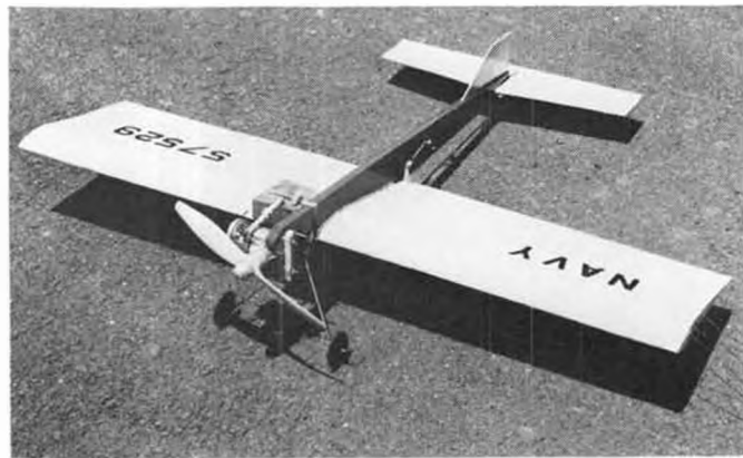
Modified "Carrier Pidgeon" from M.A.N. plans, by Joe Koch. It weighs 26 ounces and is powered by a Super Tigre .35.
