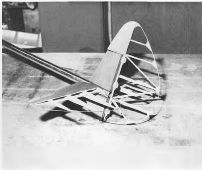
Gussets are realistic, and also help to keep the outline wire epoxied to the stab and rudder ribs. Structure is rugged yet not too heavy.
