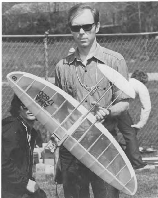
Steve Sacco, from Boston, Mass., and his Bosta. This model features a molded fiberglass leading edge.
