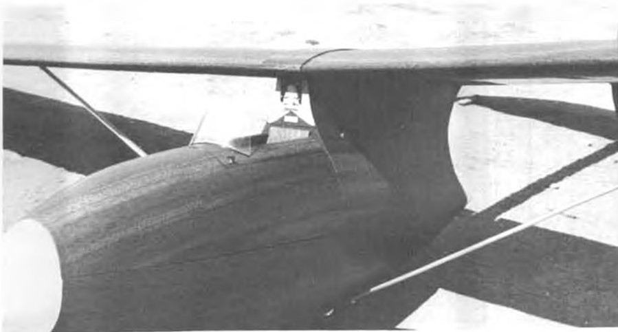
All of the mahogany planking on the original Bowlus was duplicated by using mahogany-finished Contact paper. Struts are K&S streamline tubing, reinforced with music wire.
