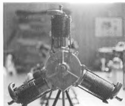
Real Anzani three-cylinder engine from which model at right was copied.
