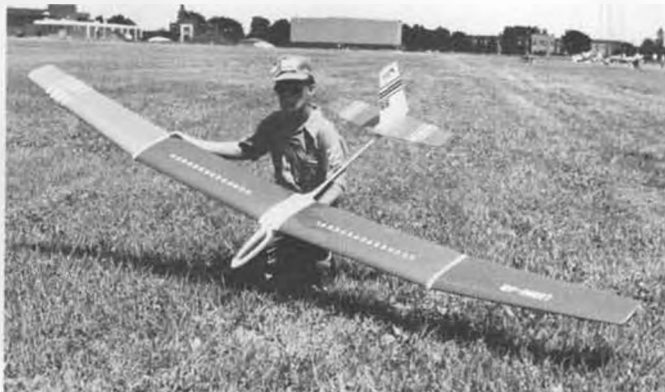
Cecil Haga, with the 12 foot span Legion-Air, which he designed. Note large spoilers, aluminum tube tail boom.
