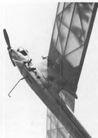
Ron Young's Cox .049 powered 1/2A ship, showing timer, plumbing, and DT.
