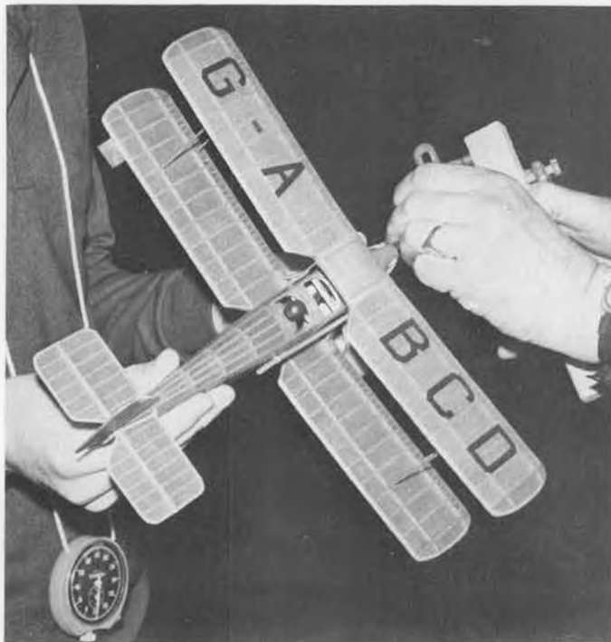
A beautiful little Gipsy Moth-like biplane, an Avro Avian, built by Keith Miller. Note profusion of false ribs.
