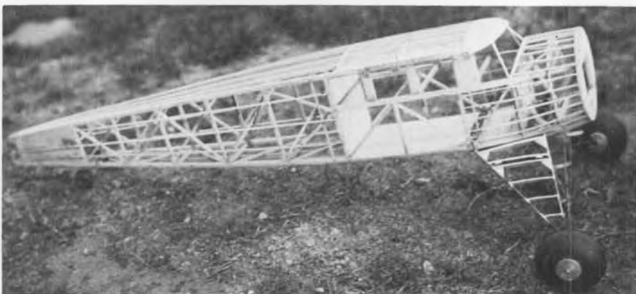
Fuselage framework of 1937 model. Most gas models of the time were rather box-like in appearance. Note built-up fairings between front and rear landing gear struts.
