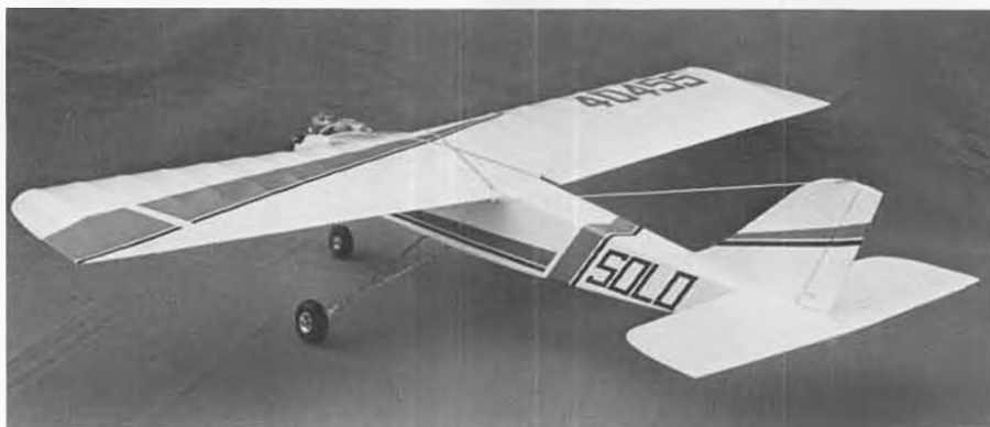
Three-quarter rear view accents wide landing gear tread. Lack of surface spars permits smooth airfoil along full span of wing. Sheet tail surfaces add to ease of construction.
