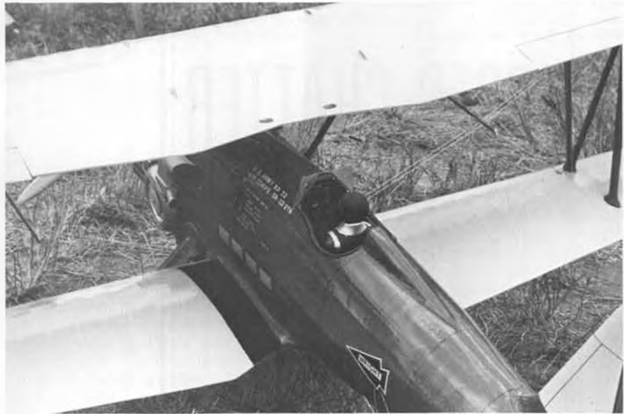
Close-up of Charlie Smith's XP-23. This was the last of the famous Hawk series, and one of the most beautiful. Featured metal clad fuselage, fabric surfaces.
