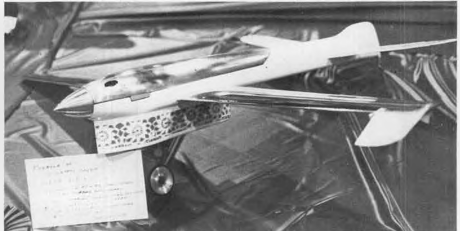
Max Snyder's trick Formula 40. Aluminum wing, half-pan, "V" stab, stainless gear, ball bearing wheel. Flies clockwise to eliminate torque problems on takeoff. Set record at '76 NW Regionals.
