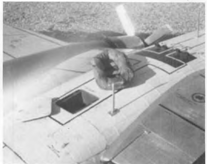
Foam stuffed life raft seems to inflate when it is released from compartment. Skin is actual aluminum plates over balsa sheet.
