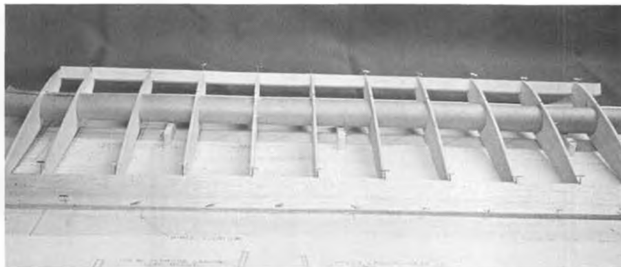
Right wing panel on construction board. Leading edge and top trailing edge sheeting have been added. Might be fun to put cork in tip and carry odds and ends to flying field!
