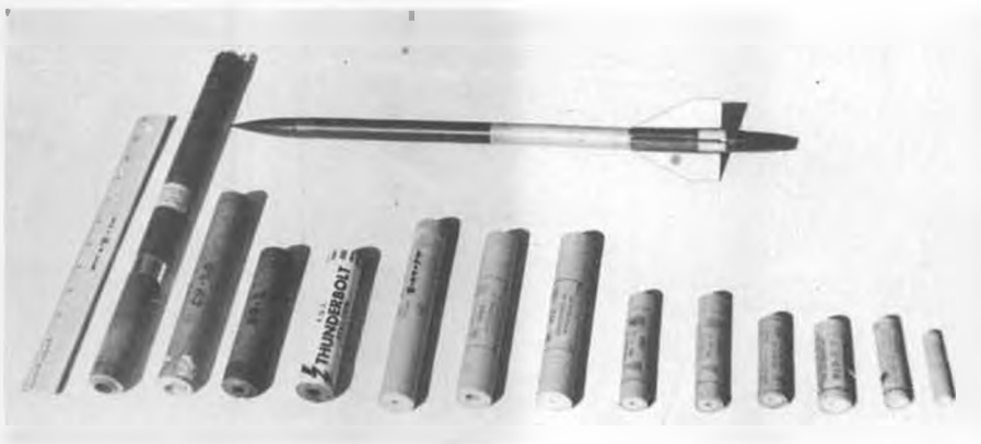
(l to r): Three professional sounding missile engines by FSI; FSI 'Thunderbolt'; another commercial motor; five FSI model rocket engines; an Estes D12-5; Estes C6-5; and AVI 'mini' B3-5m.
