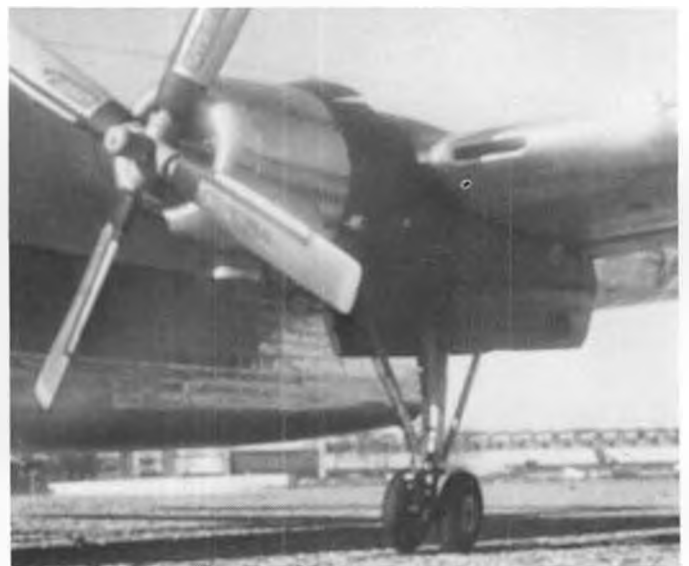
At last, a give-away! You can spot the engine cylinder head in this photo. Tires filled with silicon rubber to hold shape under weight.
