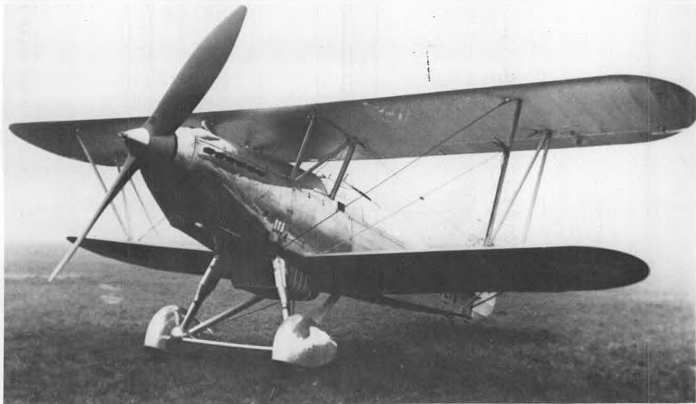
A pristine, ex-factory Mark II Fury. Most obvious difference was the addition of wheel spats, but the engine was a 640 hp Kestrel, in place of the 525 hp engine in the Mark I.
