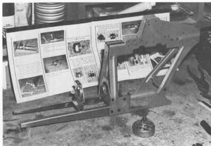
Stamped aluminum frames and formers bolted together. Clutch bell housing is in the foreground.
