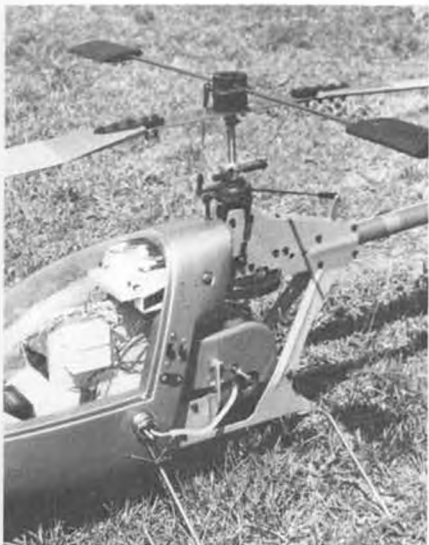
Flexibility of main rotor plate shows here. Also canopy attachment. Nice fit.
