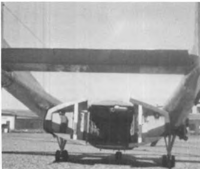
Most typical view of C-119. Complete interior work is described in text. Monorail delivery system is operational.
