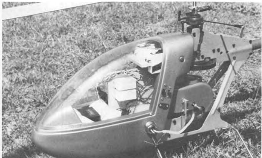
Not a scale-like interior, but then, the radio gear has to go someplace, and this is primarily intended to be a small, compact helicopter. Note that John installed Kavan gyro.
