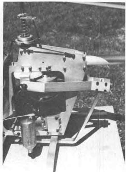
Close-up of yoke on Schluter trainer. Chopper can be mounted or demounted in minutes.
