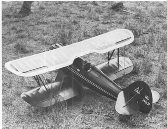
Another fine Waco. This one by Dean Copeland, who placed 2nd in Sport Scale at Mile High. Note corrugated ailerons, wheel pants.
