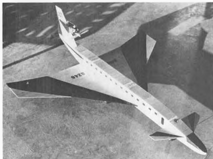
All-sheet balsa model from Competition Models. Two-channel radio on rudder and Medallion .049 throttle. A fun sport aircraft.
