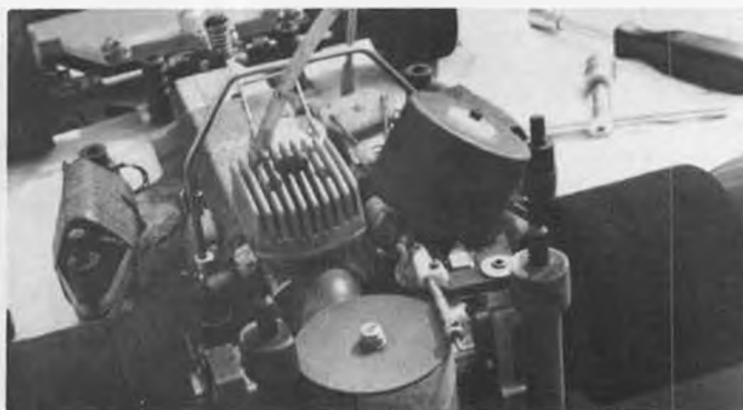
Another PB car, this one with a wet weather air cleaner, simply a spray can top put over the stock air cleaner.
