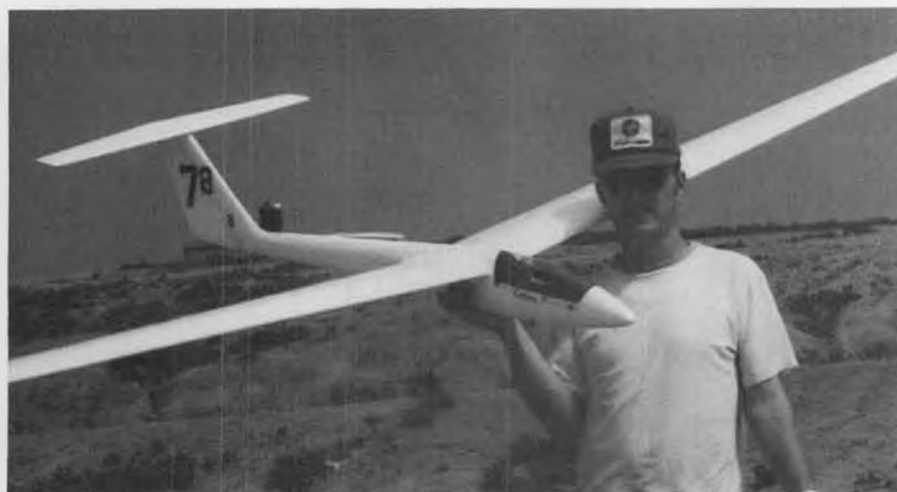
Mike Foreman did a beautiful job on this 1/5-scale Cobra 17, built from a Veron kit. Wing span stretched to 136 inches, weighs 6-1/4 lbs.
