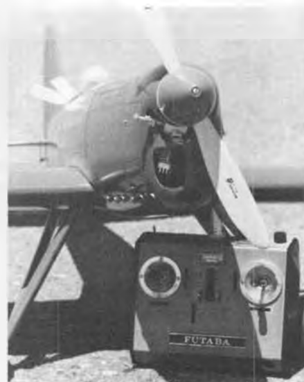
Engine tilted to line up with cowl opening. Top Flite 11x7-1/2 for flying.
