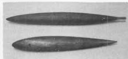
Note the difference in streamlining between the BONE bulb plug (top) and EPIC bulb.
