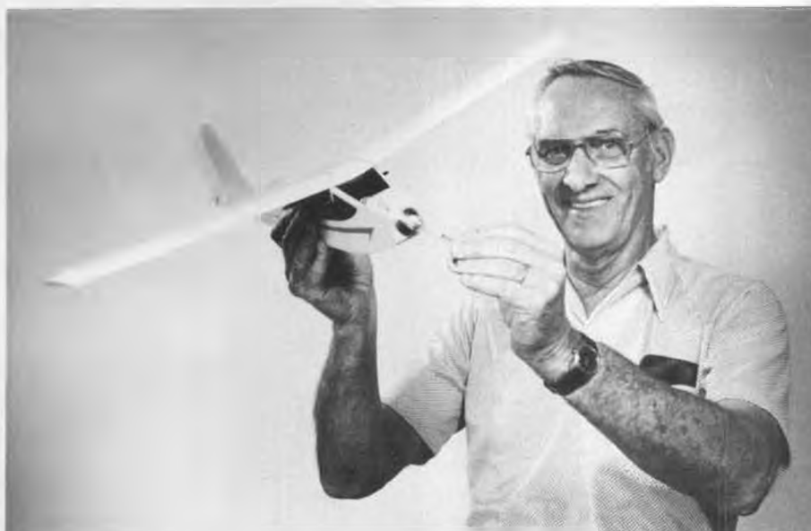
Dick Henderson, author of the "Hendertoons" that appear in Model Aviation , with his Poling-designed Electro Flea. Has 115 sq. in., Astro 020 motor, Ace R/O unit.
