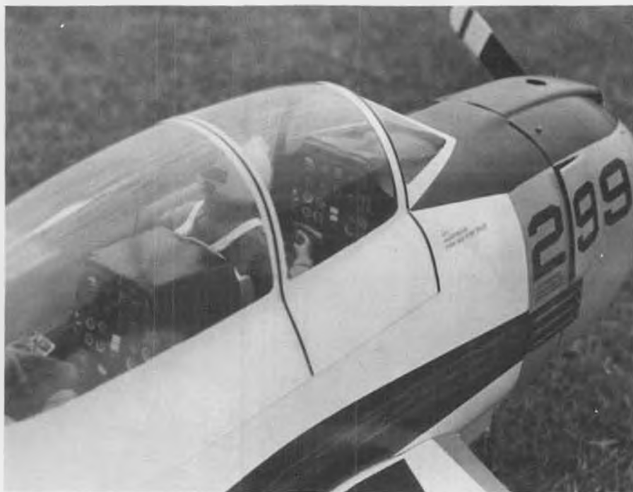
Over-the-pilot's-shoulder view of the cockpit in Jerry's T-28 shows very impressive workmanship. Model is powered by a Webra .61, has Kraft radio and Rhom retracts. Fitz photo.
