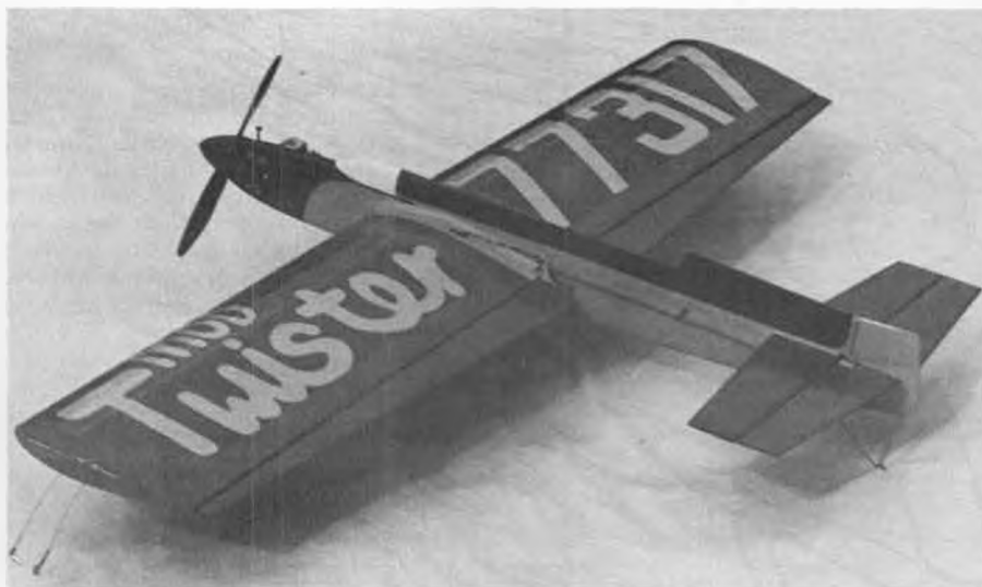
The "Mod Twister" built by Jim Thomerson. Basically a stock Sig kit, but changes to rudder, fin, and canopy give it a new look. Photo by Don Taphorn.
