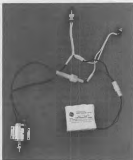
Modified motor wiring circuit includes a push-push switch and charge jack.
