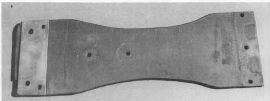
An experimental graphite-epoxy chassis by Bill Steele. Saves weight but is brittle.
