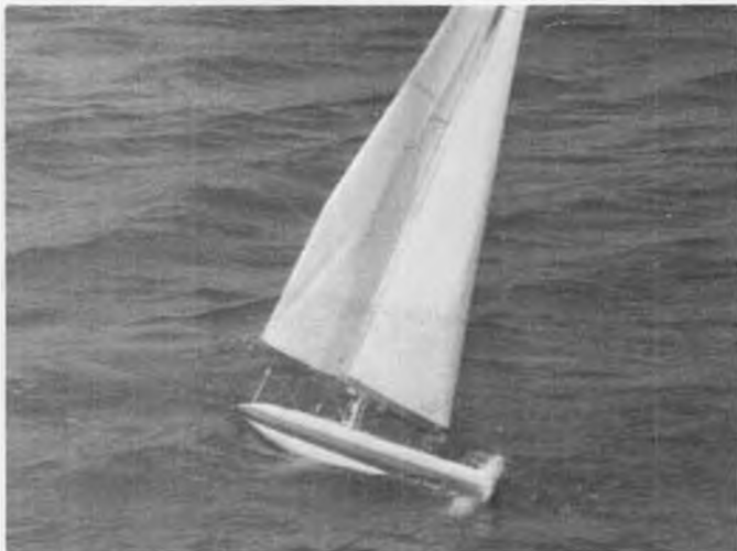
Low freeboard of BONE and BONE II shows on this run in which a bow roostertail is being thrown. BONE III has added freeboard.
