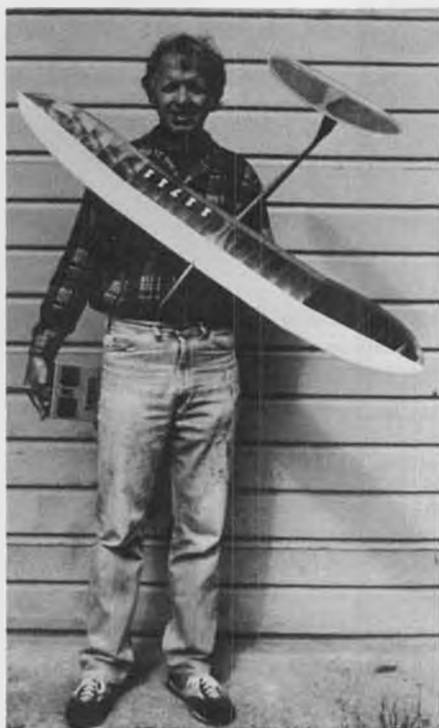
Smallest ship was Thornburg's T-tail. Spans 54 inches, weighs 11-1/2 ounces.
