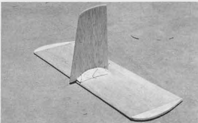
Stab assembly is a cinch. Triangular fin gusset is on left side only. Rudder is attached with figure-8 thread hinges.
