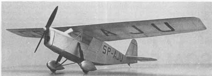
A rare Polish RWD-5 rubber model by Alan Callaghan of England. Spans 19-1/2 inches, weighs 18 grams. With that wing area and simple lines, it would be a good choice for a Peanut.
