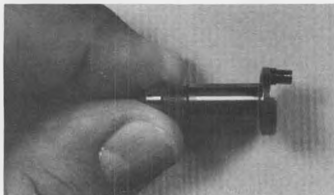
Flooded engines and electric starters don't mix. Note the bent crankpin. More info in text.
