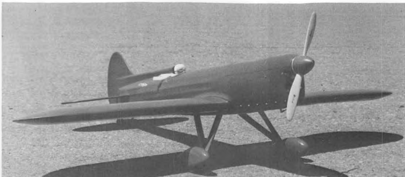
Brown B-2 Racer "Miss Los Angeles" built and flown by MB's graphic art man, Chuck Blackburn. Bridi kit includes glass fuselage, foam wings. Finish is red K&B Super Pox. Fast stable flier, with Enya 60 Schneurle and Futaba 6-Ch. radio.
