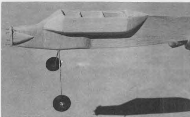
Fuselage with the nose doublers, firewall, firewall fairings, and front and rear radio box fairing blocks added.
