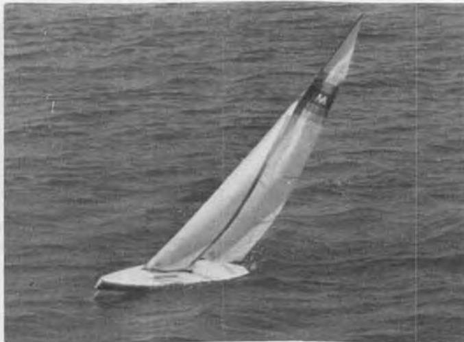
The aft placement of the keel on the prototype BONE has proven excellent at keeping the bow out of the water.
