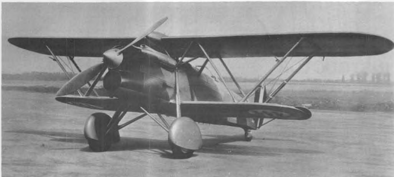
Public relations photo of the CR-32 shows the fighter in pre-1938 aluminum finish. An agile fighter, the Fiat had a top speed of 205 mph. Note use of struts instead of wires to brace wings.
