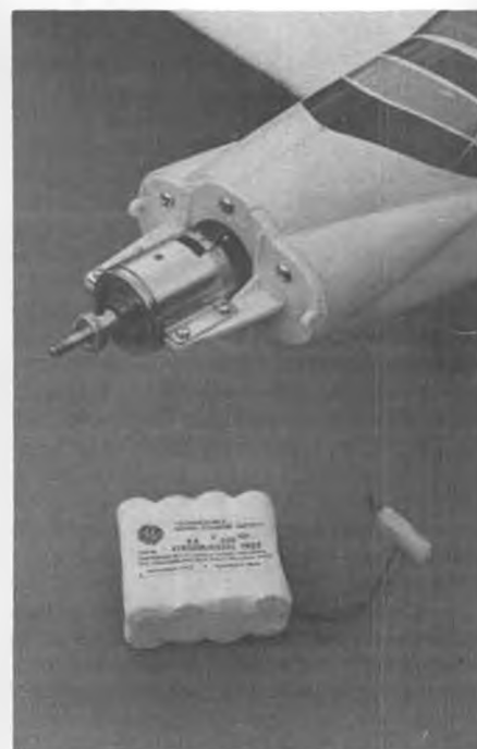
Closeup of the motor installation and motor battery for the Sportavia. Motor turns 6X3 prop at 14,000 rpm.
