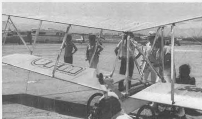
The Solar Riser, world's first man-carrying solar plane, is based on the popular Easy Riser tailless biplane hang glider. Has 168 solar cells in top wing. Photo by Jerry Litwak.
