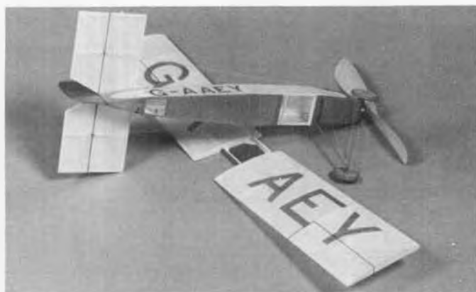
Gillespie's Gadfly comes apart for storage and transportation. Wings are a friction fit in the fuselage.
