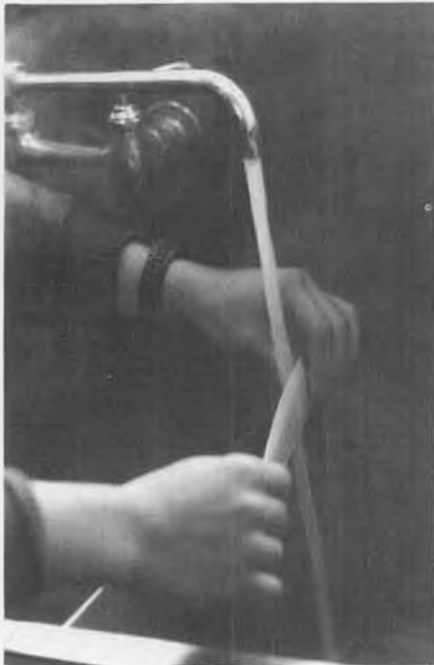
Bruce Kimball shows how to make prop blades from a twisted sheet of balsa (a la George Perryman), instead of carving them from a block. After soaking thoroughly with hot water (left), the blade is held over a hot stove and twisted to the shape desired. More details in text.
