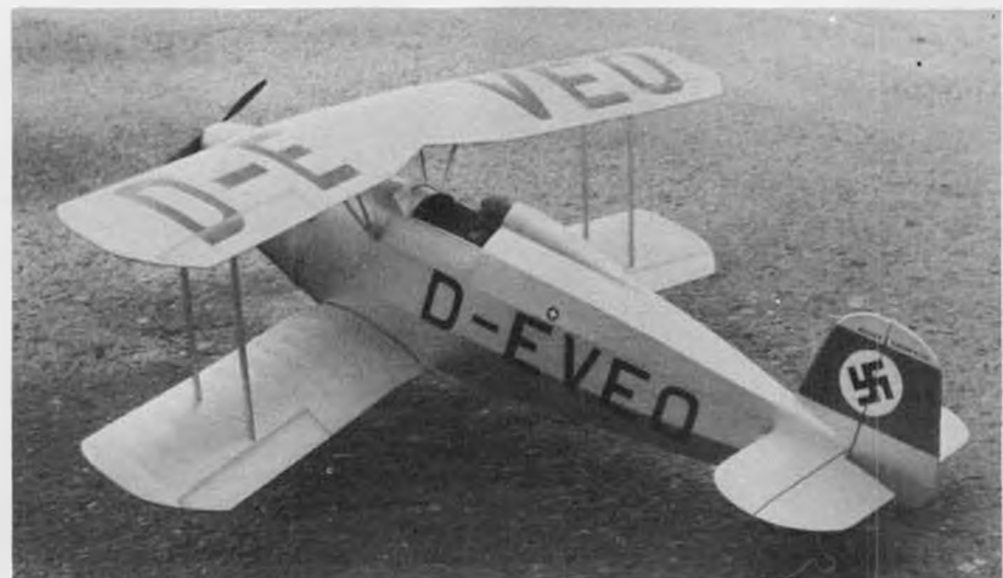
Another of Fernando's Flyline kit models is this Bucker Jungmeister with Cox .049. Wings and tail are tissue covered, fuselage is tissue over silkspan. It's R/C... WHA T!!!
