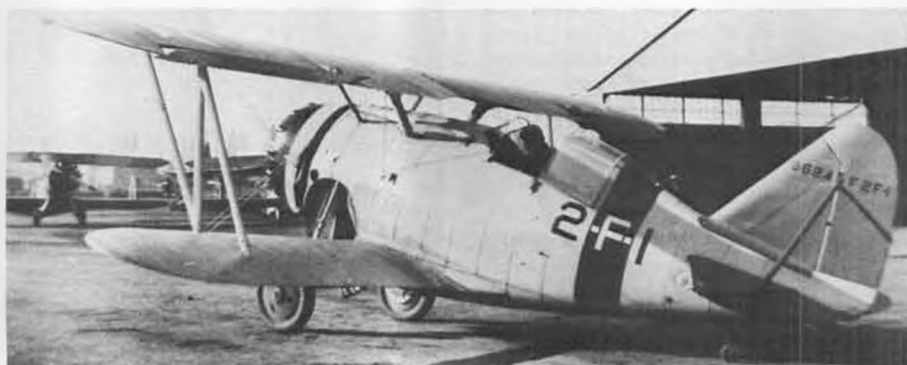
Second production F2F-1 went to squadron leader of VF-2B on USS Lexington . Joints of wrapped fuselage skins are evident. Photo courtesy Fred Dickey, Jr.
