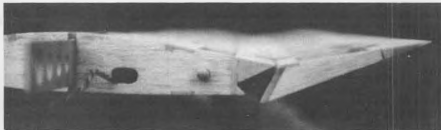
Up aileron is where the Frieze type aileron is unique. Note that the lower leading edge of the aileron protrudes down into the slipstream, causing drag on that one side only and offsetting the adverse yaw (tendency for the airplane to yaw opposite to the intended direction of the turn) present when using conventional ailerons.
