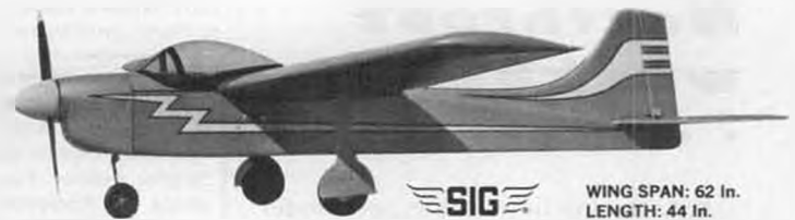
LARGER SIZED MODEL - FOAM CORE WING WITH BUILT-IN WASHOUT
