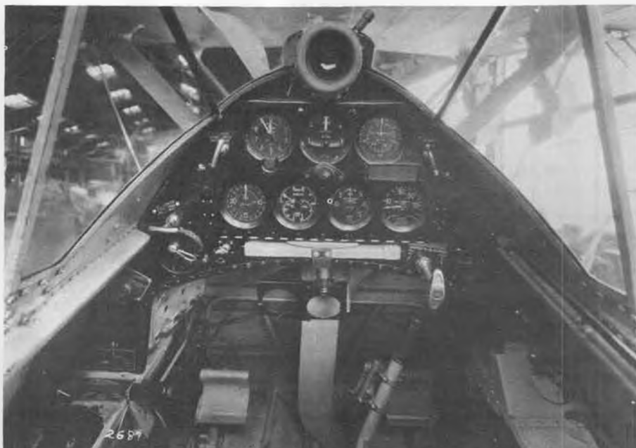
Cockpit of the F2F-1 was roomy with a well-designed instrument panel. Knob on telescope gunsight was pulled down to rotate dust cap off forward lens. Clendennen photo.
