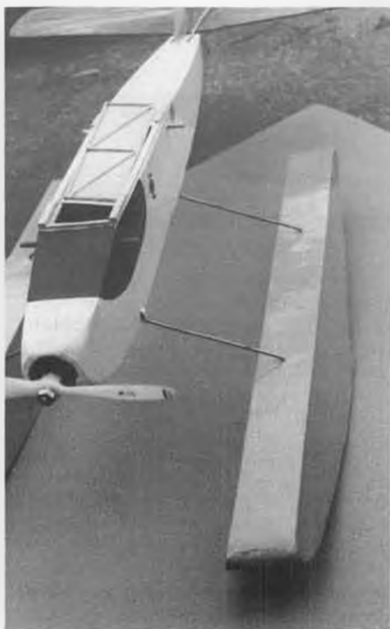
Float mounting on the Astro Sport 15 is super simple. No water rudders used.
