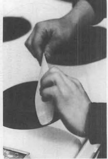
Bruce Kimball shows how to make prop blades from a twisted sheet of balsa (a la George Perryman), instead of carving them from a block. After soaking thoroughly with hot water (left), the blade is held over a hot stove and twisted to the shape desired. More details in text.
