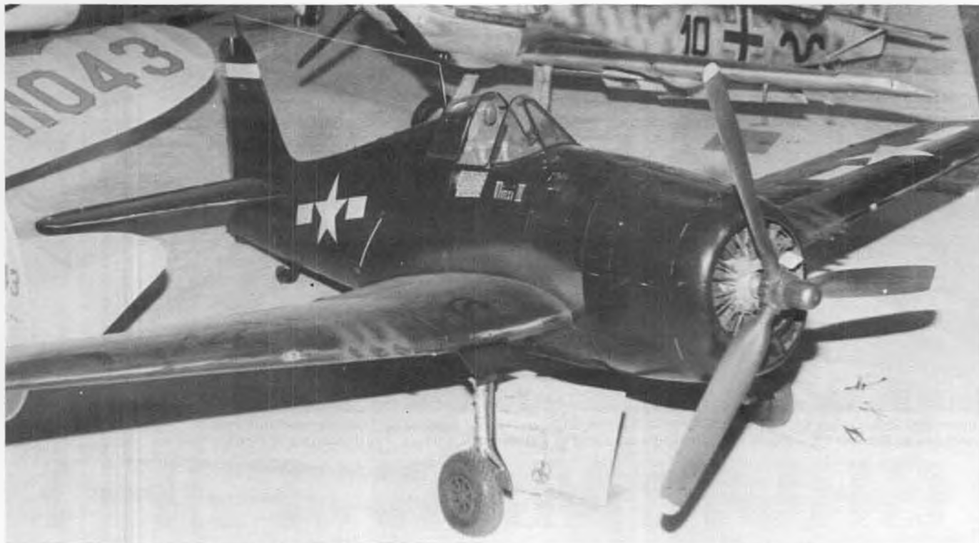
An excellent example of a realistically weathered finish is that on Bill Mikesell's F6F-5 Hellcat, 2nd place winner in Precision Scale at Toledo. Bill built the ship from Bob Holman plans, at 1-1/2 inch scale (64-1/4 inch span).
