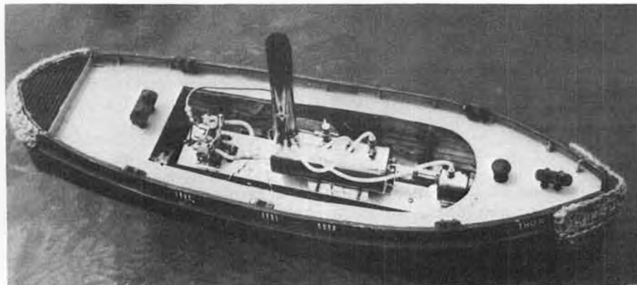
Interior shot of Mike Deleeuw's tugboat shows the Saito B2F boiler and 4-cylinder V4PR steam engine. Boat measures 37 inches overall, took Mike about 3 years to build.
