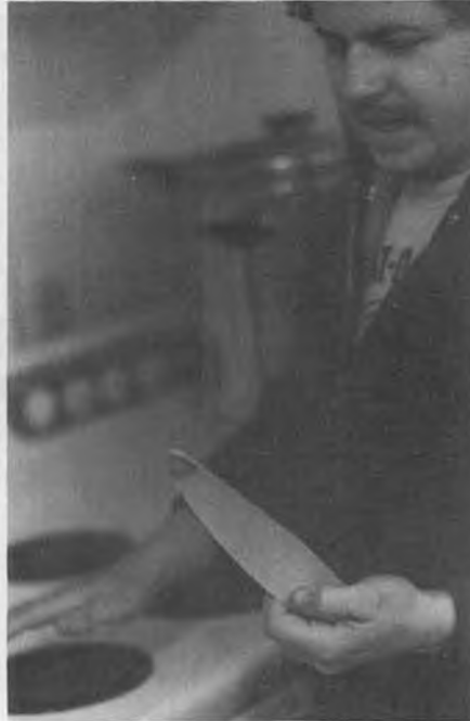
Bruce Kimball shows how to make prop blades from a twisted sheet of balsa (a la George Perryman), instead of carving them from a block. After soaking thoroughly with hot water (left), the blade is held over a hot stove and twisted to the shape desired. More details in text.
