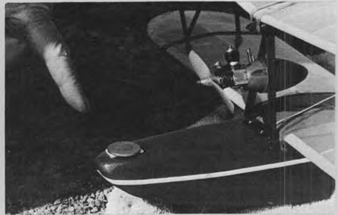
Two-bit nose weight gets the balance point forward, makes flight stability better and takeoffs longer.
