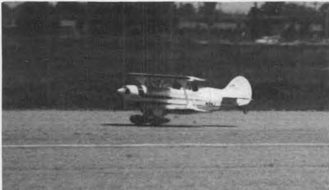
Bob Seigelkoff's 2-holer Pitts is powered by a Kawasaki engine. Muffler added for flying at Mile Square caused some problems.
