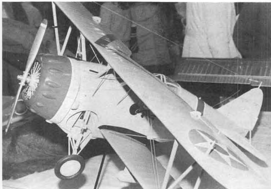
Bob Godfrey's Grumman F3F-1 was a favorite among the spectators, has almost all the colors of the rainbow. Landing gear was scratch built, retracts as per the original. Note the radio switch mounted in the wheel well. Placed 5th in Precision Scale.
