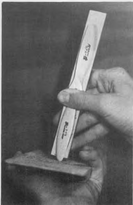
Hardwood jig being used to trim prop blades to desired length prior to rework.
