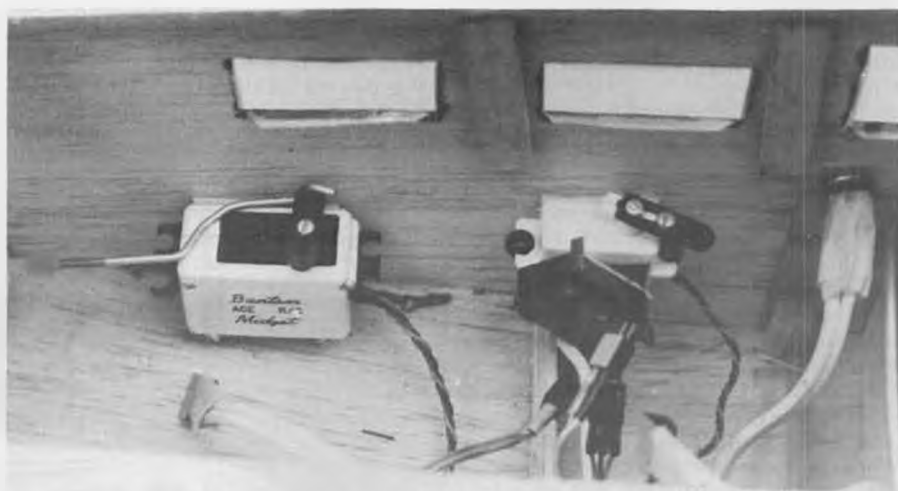
The Bantam Midget and Cannon Super-Mini servos mounted in Mitch's twin 020 Widgeon flying boat. Mini servos makes the Midget look huge!
