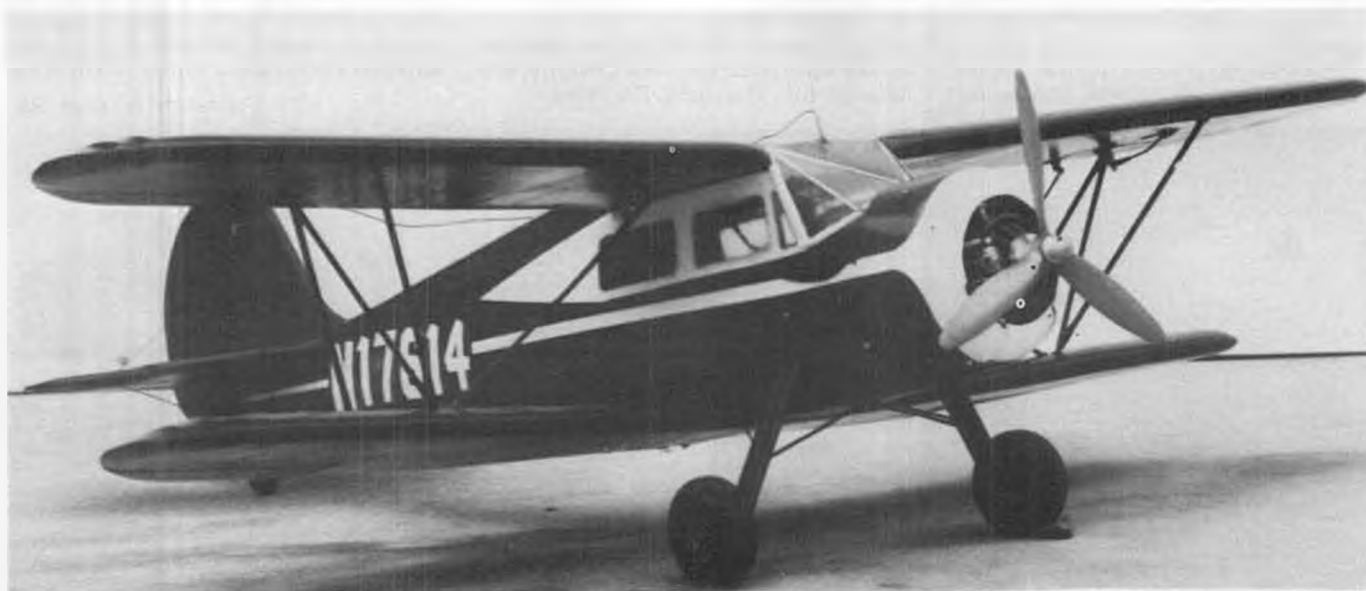
A possible future construction article may appear on this fine Waco YKS-6, designed and built by Jack Burns, El Cajon, California. The ship is extremely stable, and is powered by the O.S. Wankel engine. Construction is traditional balsa and plywood.
