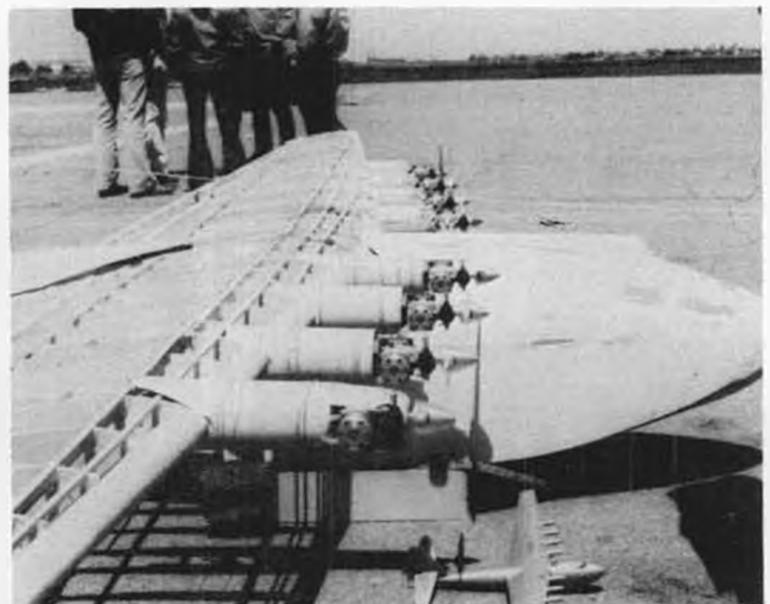
Look closely at left and you'll see Kraft receiver, battery pack, and two servos in the tail of giant Howard Hughes "Spruce Goose" being built by Ray Baker, of Norwalk, California. That's 3.2 cu. in. worth of K&B 40's up front. Ray's planning to switch to 60's. Whatta project!
