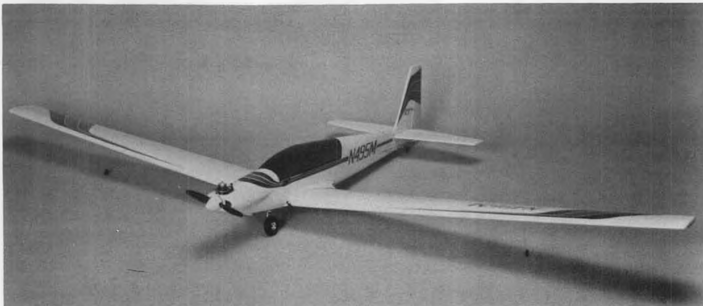
The Cox Sportavia has been around for a couple of years now, is just as popular as ever, especially with beginners. Available with gas or electric power. All-foam construction with a few hard plastic parts and hardwood wing spars for extra strength.
