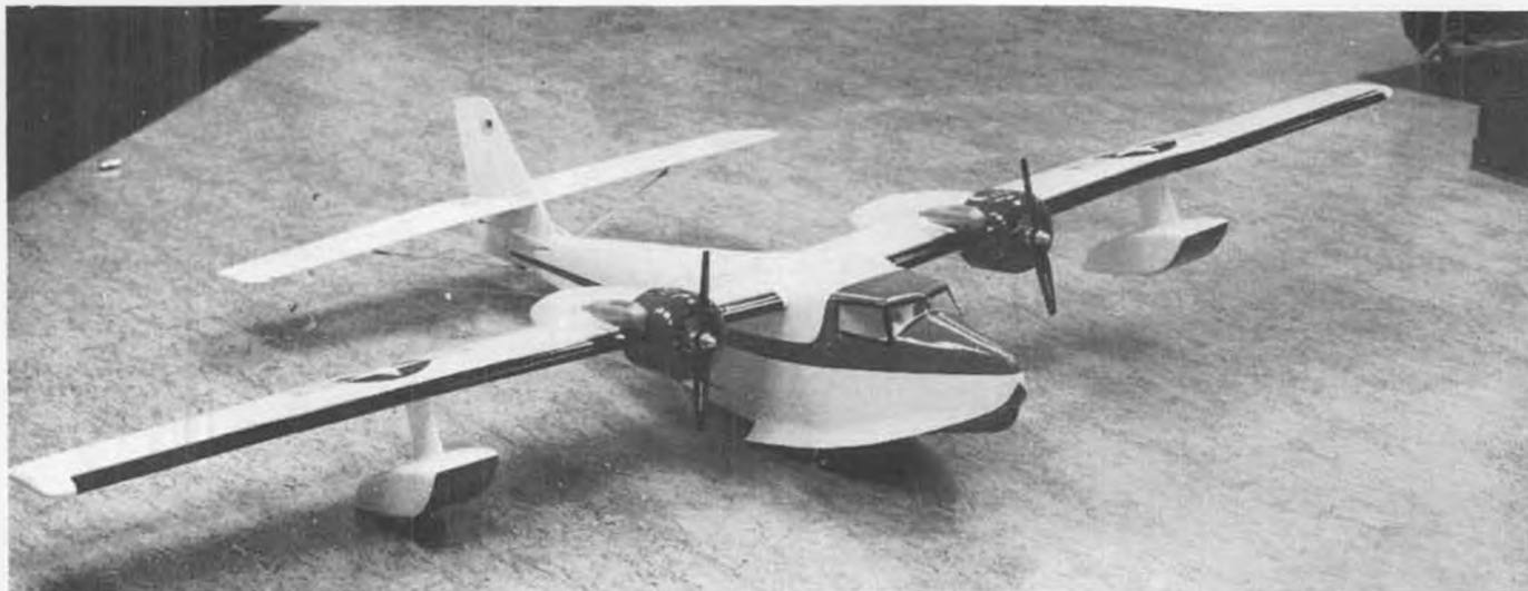
Kurt Olsson, Stockholm, Sweden, built this version of Pavel Bozak's "Cleopatra" design, from the article published in our August '77 issue, plans available. Powered by two OS .45 engines, Kurt plans to fly it over the Baltics, between Sweden and Atland, about 40 miles, following by boat.
