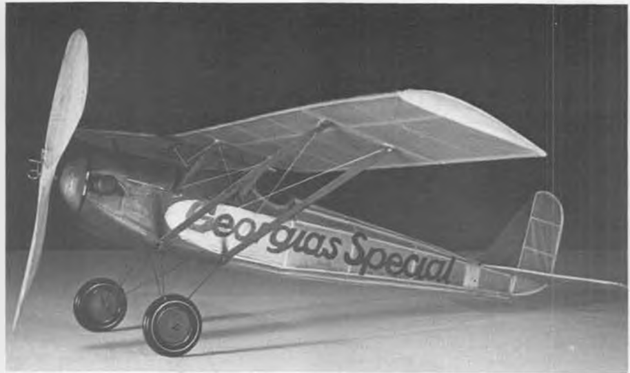
Maj. Ed Heyn built this 20-inch Georgias Special from drawings in the 1931 Flying and Glider Manual , an EAA reprint. Built for indoor scale, it has dyed condenser paper covering, molded acetate cowlings, and pre-war celluloid wheels.
