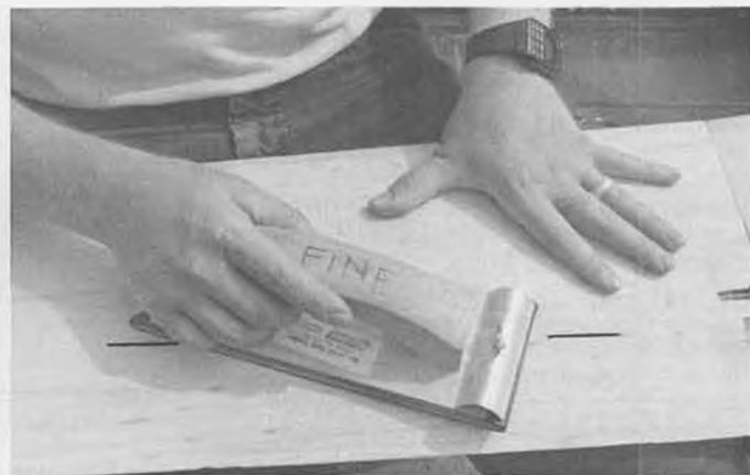
Even though it appears that I am not sanding at an angle, I am. The black lines indicate contact area of sanding block. Comfortable grip.
