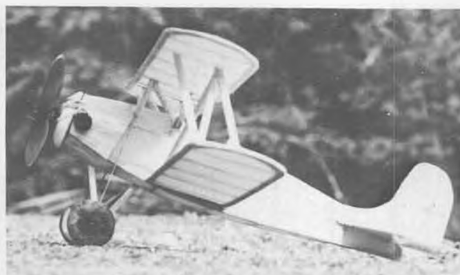
The Rose Parrakeet is one of the easier biplane Peanuts to construct as there are no flying wires to hassle with, and the tail is sheet wood.
