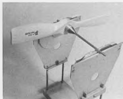
After rounding the cut-off edges, the prop requires balancing. This is very important!
