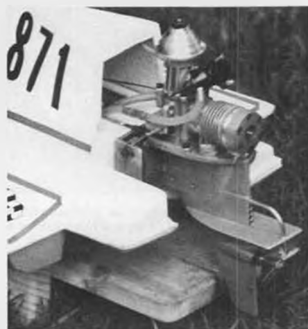
K&B 3.5 Outboard with Teague mount (see text). Octura X-442 prop does the pushing.
