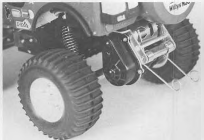
The rear end, showing the electric motor before protective heat shrink tubing was applied. Wire "feelers" are wheelie bars.
