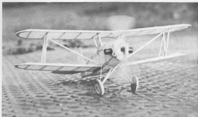
The Rose Parrakeet is one of the easier biplane Peanuts to construct as there are no flying wires to hassle with, and the tail is sheet wood.
