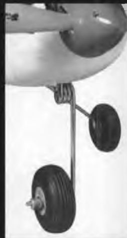
Steerable nose gear for taxi, takeoff and landing.
