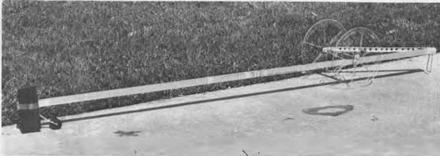
As Bill Gaines linearly stretched his rubber band for power, a long car was necessary. Note wire loop at rear of vehicle for the guide wire.
