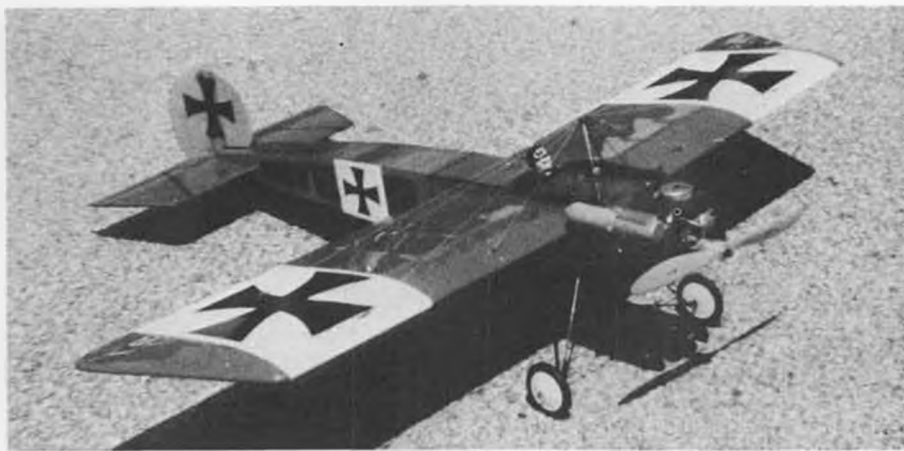
Joe Averitt, of Miami Beach, Florida, sent in this photograph of his recently completed Eindecker E-III which he converted to control line from a Nick Zirola R/C kit. Joe says it's a "fun flying plane". Specs: span, 55 in.; power, ST .60. Easy conversion.
