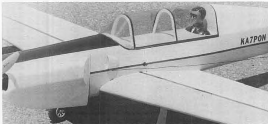
Looking for a quick and easy airscoop for your next project? Try the rear half of a wheel pant on for size. This one cools off the receiver! Hey Dick, better get a new receiver!
