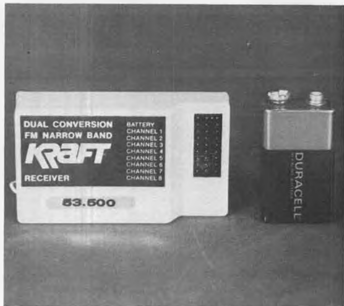
Kraft Systems new "Dual Conversion FM Narrow Band Receiver" and a nine-volt transistor radio battery for size comparison.
