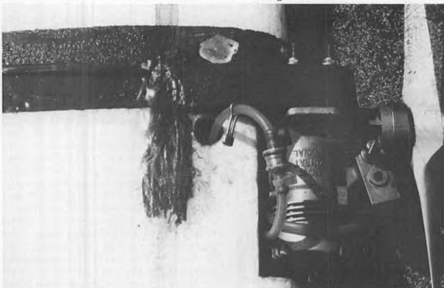
What you are looking at is a foam wing combat job with one heck of a strong repair . . . that black blob is actually carbon fiber and epoxy over a fractured spruce spar cap. Quick & dirty!
