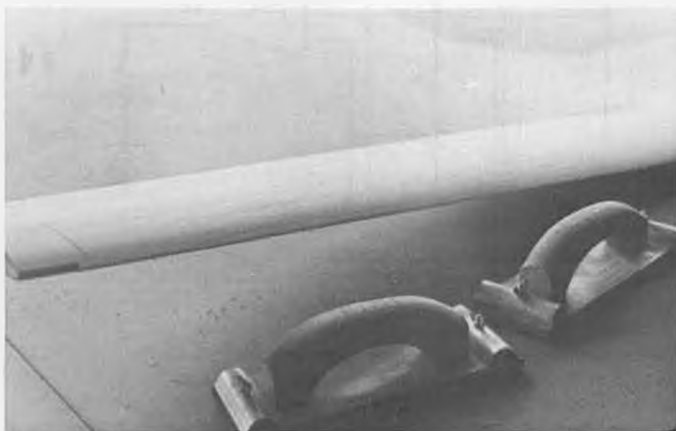
You really can see any high spots when using the shadow method. If you sand at a 45 degree angle, they will disappear like magic.
