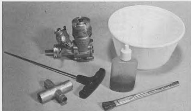
Here's what you'll need to clean that engine of yours: a cleaning solvent (kerosene), small brush, disassembly tools.
