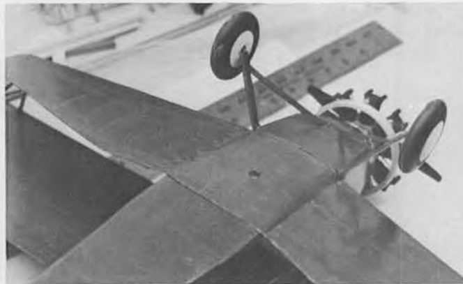
Bottom view of the 1/2A Airsedan reveals the landing gear setup, and the method of mounting the lower half-wing.
