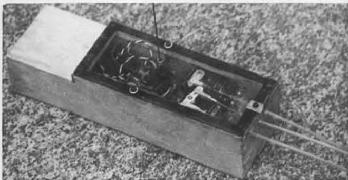
The radio box kit from International Hobbies. Futaba radio system shown. Braided wire and tubing used for throttle and steering.
