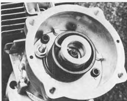
PK Products Super Starter installed on the backside of a Quadra. Works very well!
