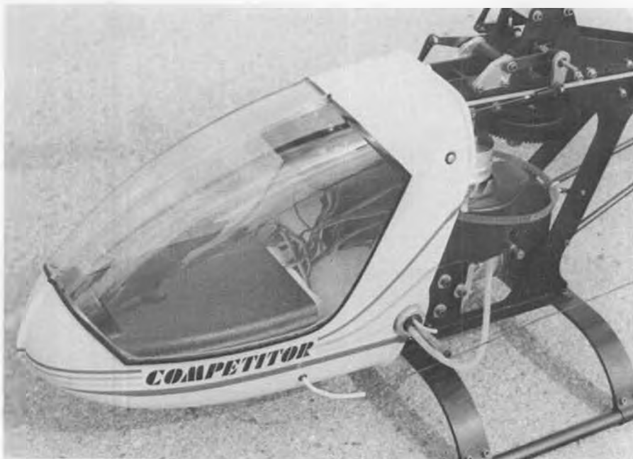
The Competitor's canopy is joined by first tack gluing it together with Hot Stuff, then by applying acetone with a Q-Tip along the seam. This method dries clearly and neatly.
