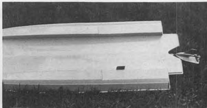
The view from the bottom. AMPS 3.5 Tunnel needed a turnfin according to author. Note sponson break.
