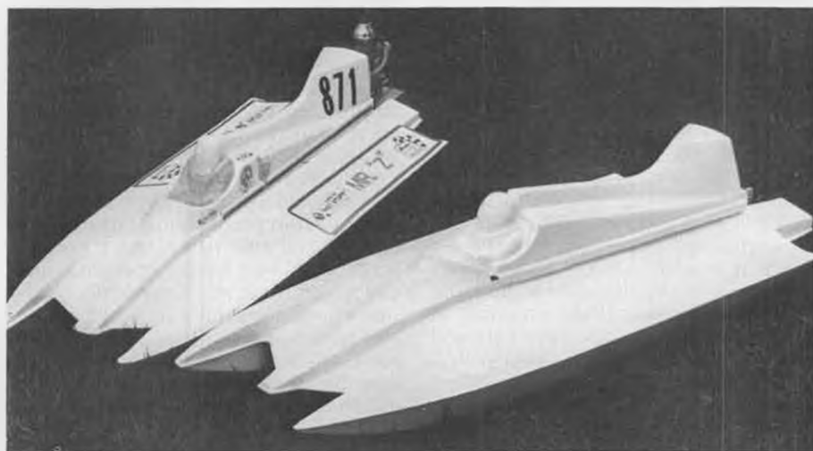
The AMPS 3.5 Tunnel (left) and the 7.5 Tunnel (right) are distributed by International Hobbies, Ft. Collins, CO. Fiberglass construction, drivers are molded into cowls.
