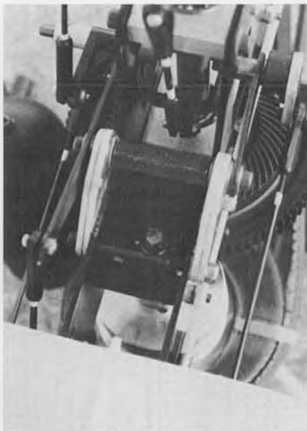
Additional aluminum pieces (No. 478) are shown on each side of frame for collective arm support. Author's modifications.
