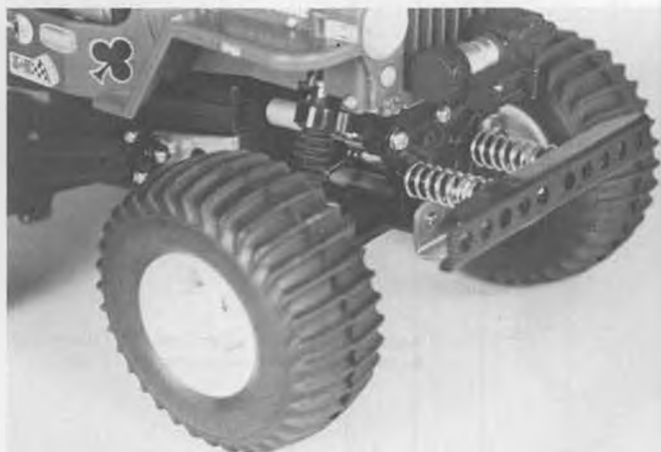
The front end, showing the massive bumper springs, entire front end is rugged enough to withstand shock with little damage.
