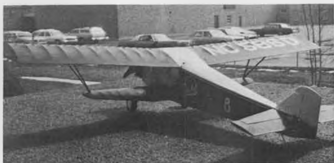
This 3/4 rear view graphically depicts the long tail moment of the Airsedan which aids stability in a 1/2A-size model.
