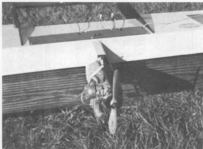
Close-up photo of the Razorblade showing inexpensive .15-size C/L engine, pushrod linkages, fuel tank mounting details, etc.
