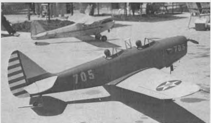
PT-19 built from Pilot kit by John Eaton, Redondo Beach, Calif. Power is an Enya 1.20 4-stroke w/ Bernhardt ignition conversion.
