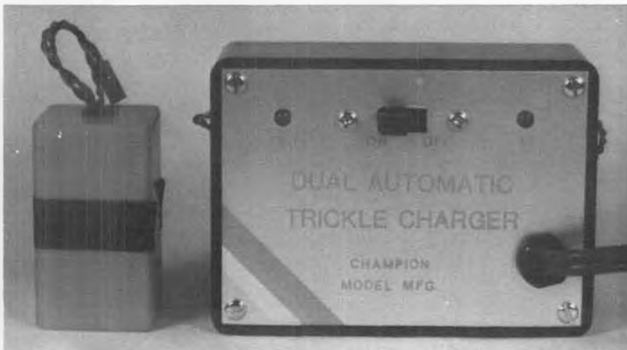
Champion Model Manufacturing's Dual Automatic Trickle Charger will charge your 8-cell TX battery and 4-cell receiver battery to max, then trickle charge them indefinitely.
