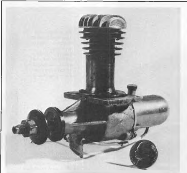
The stately French Micron 5cc diesel engine started the 40-plus year lineage of that country's most noted model engine manufacturer . . . a company which produces engines to this day. The Micron 5cc has no compression adjustment. Fuel's OIL CONTENT was varied to control ignition of ether/kerosene mixture.
