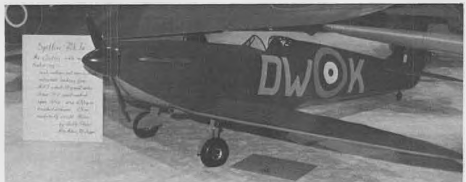
An electric powered (!) model entered in Military Standoff Scale by Keith Shaw of Ann Arbor, Mich. It is a Spitfire Mk 1-A, and it features four-channel control, Jomar SC-2 speed controller, Astro Flight cobalt 25 with gear reduction. Weighs 5 lb, has 670 sq. in. of wing, scratch-built!
