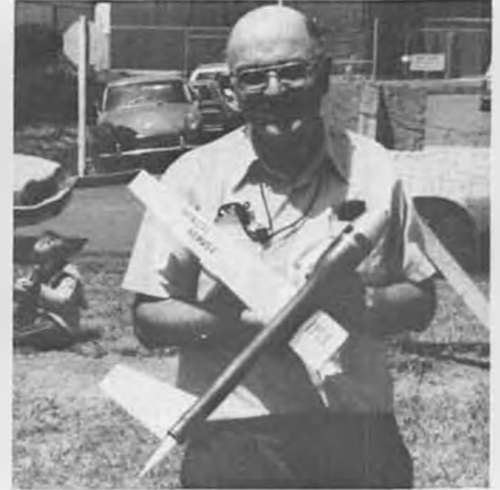
Jerry Thomas' latest asymmetrical wing Jet Speed design, Ironside Hummer, features aluminum wing, tail, and fuselage.
