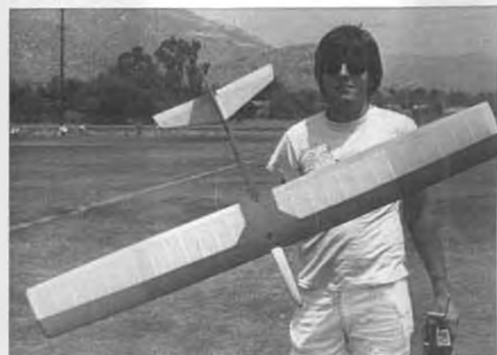
Dieter Lamprecht, Huntington Beach, Calif., made up three wings for his Gnome : stock (seen here), stock w/ E-182 airfoil, and constant taper/polyhedral w/ E-205. He liked the latter for its handling, but flew stock anyway.
