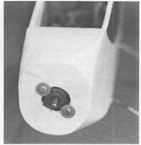
Here is a very simple method of mounting an electric motor to an airplane: simply place the motor behind a 1/16 (or thicker) plywood firewall and drill 3 holes. The two small ones are for the actual mounting screws, washers.
