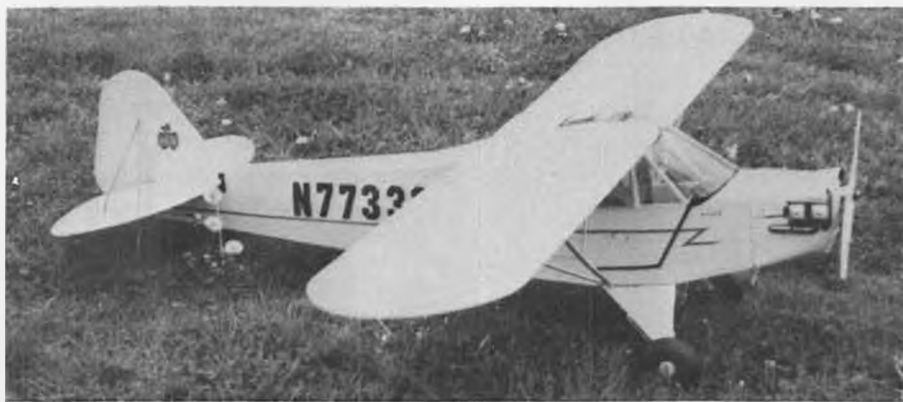
The BIG Sig Cub powered by a .90 or 1.20 four-stroker is becoming a very popular combination. This one belongs to Tony Della Vecchia, Newtown Square, Pennsylvania, who flies with the Mt. Holly, New Jersey, club, the High Rollers. The model weighs 13 lbs., uses Enya .90 4-cycle, 15-6 prop, Ace battery backup system, Permagloss yellow paint. Great flier!!!
