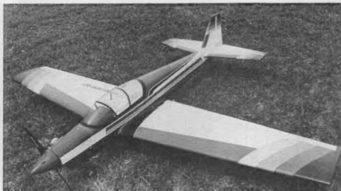
The completed Cavalier 40 , ready to fly, weighs 6-1/2 pounds, and is powered by a K&B .40. Stripe on cowl applied by author.
