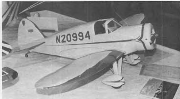
John Hodgson of Massillon, Ohio, likes to scratch build. He entered this Culver Dart GK built from RCM plans in Non-military Standoff. Span is 59 inches. Covering is Super Coverite and Chevron paints.
