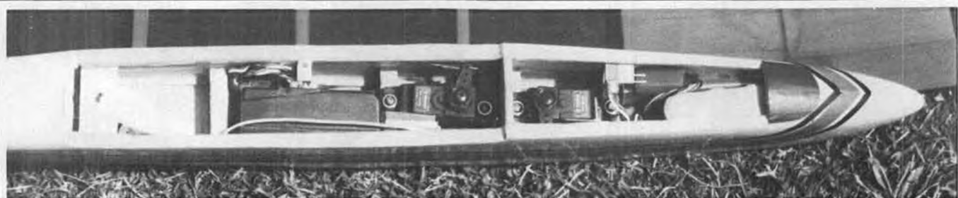
Radio equipment layout inside the Flinger fuselage. Fuselage is designed to accommodate various receiver/servo combinations.
