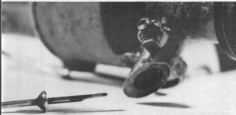
The original, preproduction engines probably copied their "tapered-sliced" needle valve from the American Brown Jr. which was so successful. The first true production versions had a magnificently designed and manufactured, five-piece needle and valve assembly . . . which is STILL USED on today's modern Micron Moteurs.
