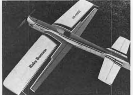
ABOVE: This Stunt model belongs to Randy Schultz, Seattle, Wash. Design is a composite of Fancher's Imitation and Excitation planforms. Powered by O.S. .45 FSR.
