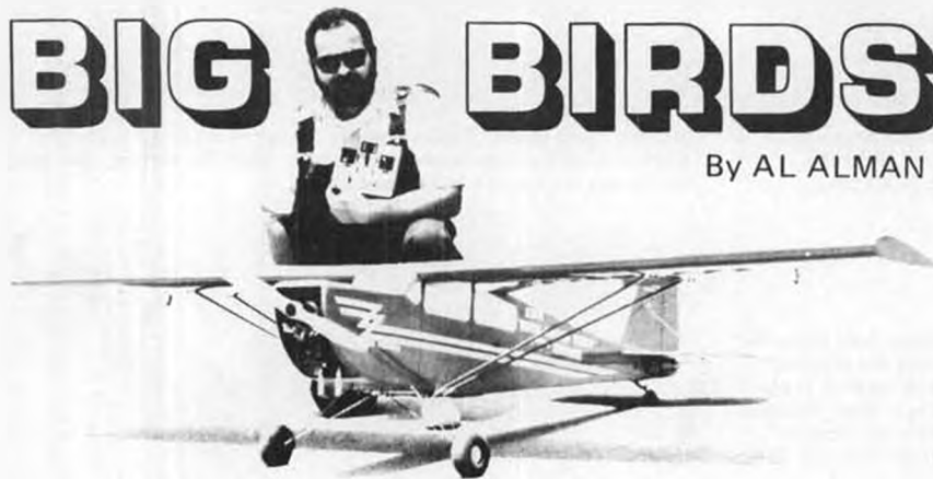
The BIG Sig Cub powered by a .90 or 1.20 four-stroker is becoming a very popular combination. This one belongs to Tony Della Vecchia, Newtown Square, Pennsylvania, who flies with the Mt. Holly, New Jersey, club, the High Rollers. The model weighs 13 lbs., uses Enya .90 4-cycle, 15-6 prop, Ace battery backup system, Permagloss yellow paint. Great flier!!!
