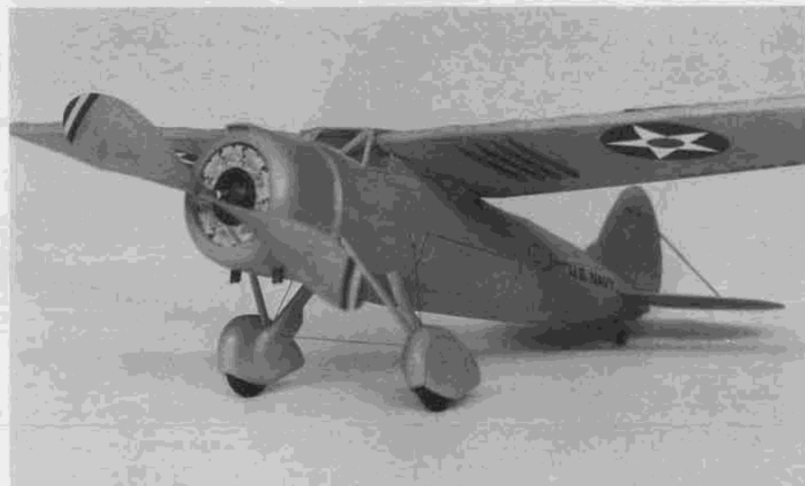
The radial engine is a paper cut-out. Note the elastic thread used to simulate wire.
