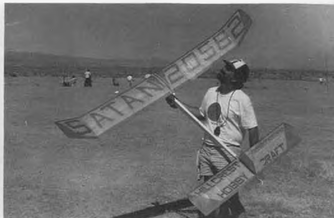
Phoenix's Randy Archer cleaned up in FAI Power with seven max flights. All aluminum-clad surfaces, graphite boom, Nelson .15.
