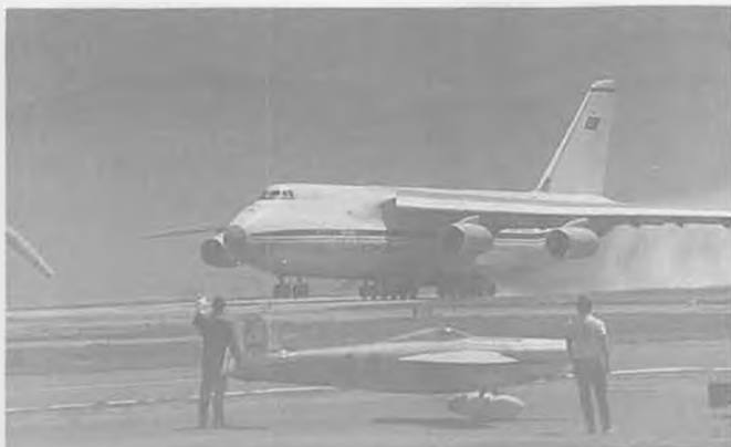
In spite of its size, the An-124 accelerates rapidly. The four nose wheels have already left the ground in this view.
