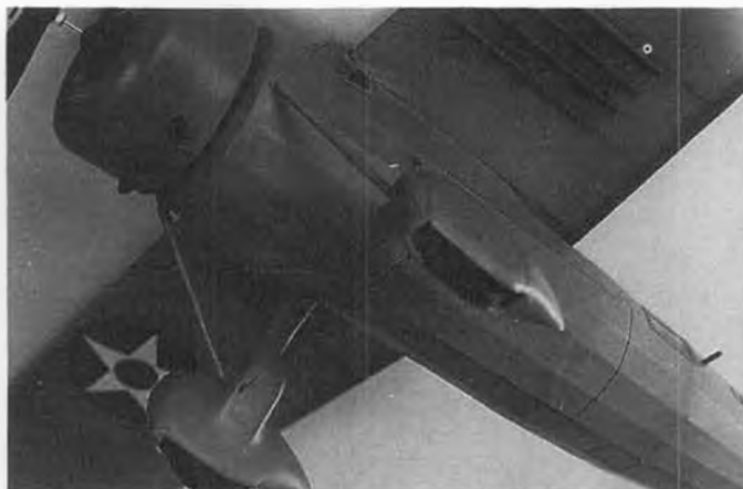
Bottom details: ribbed flotation gear is glued to a 1/20 balsa plate in the wing of the craft.
