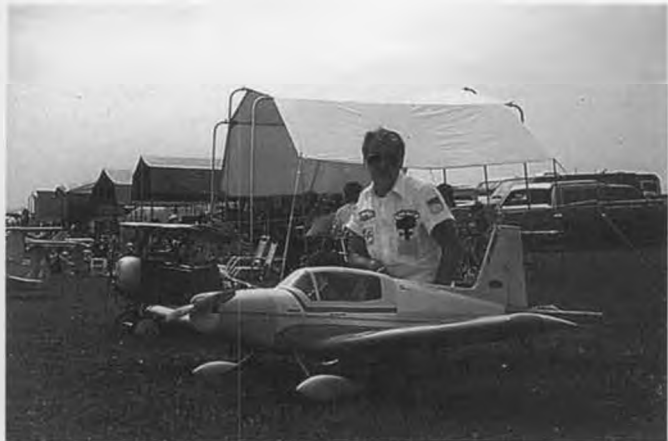
A nice-looking Morrisey Bravo from the Sig kit by Bob Burich. This one came in at 17.5 pounds with a Zenoah G-38 for power.
