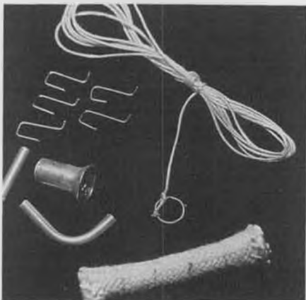
Parts for a front-mounted D.T.: fishline with stop ring, fuse, flared snuffer tube, bent guide tube, stop tube, .015" music wire hooks.
