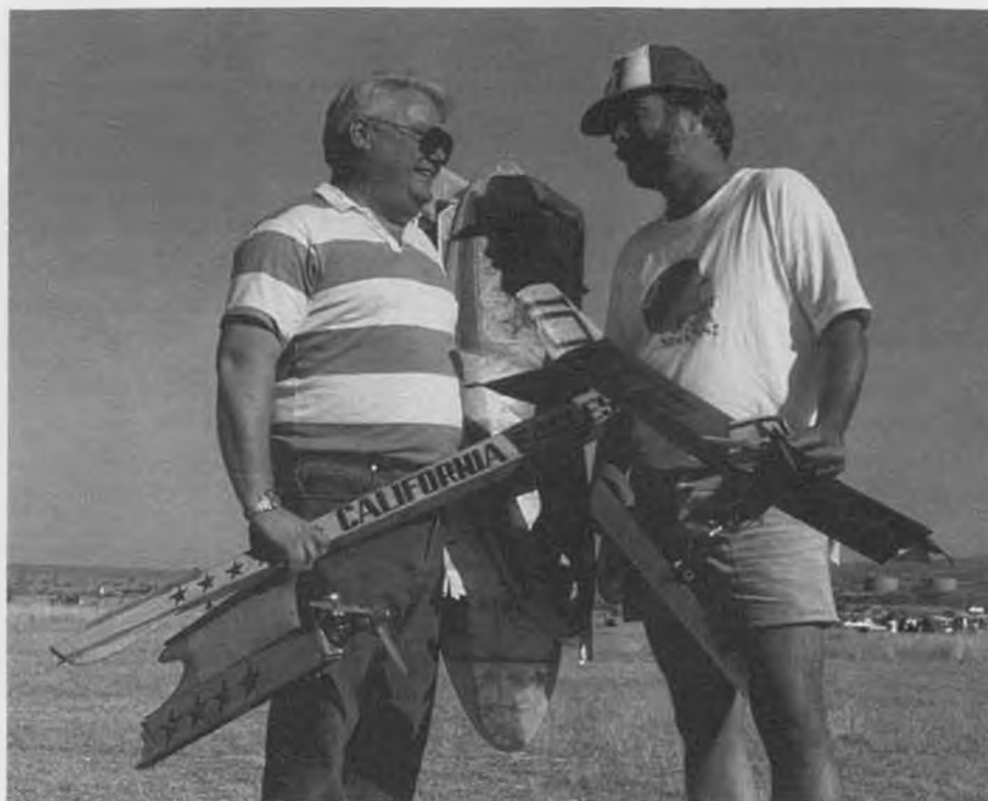
Fresno's Dallas Porter with humongous D Gas Satellite 1300 with O.S. .60 glow engine. Not a kit, it took a carload of balsa, Hot Stuff, and MonoKote.
