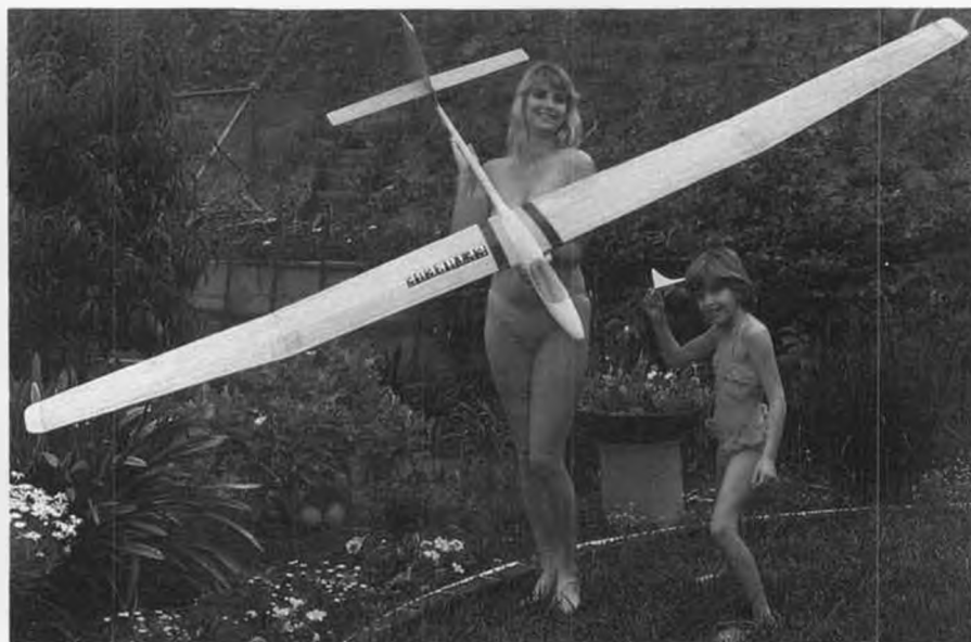
The Eftbrebe, a ready-to-fly sailplane from Ed Cutler Plastics, shown here in its floating stabilizer configuration.
