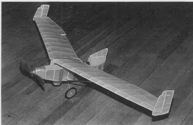
Al Backstrom's Coconut scale Lippisch Storch is rubber powered, spans 36 inches and has exceeded 30 seconds indoors.
