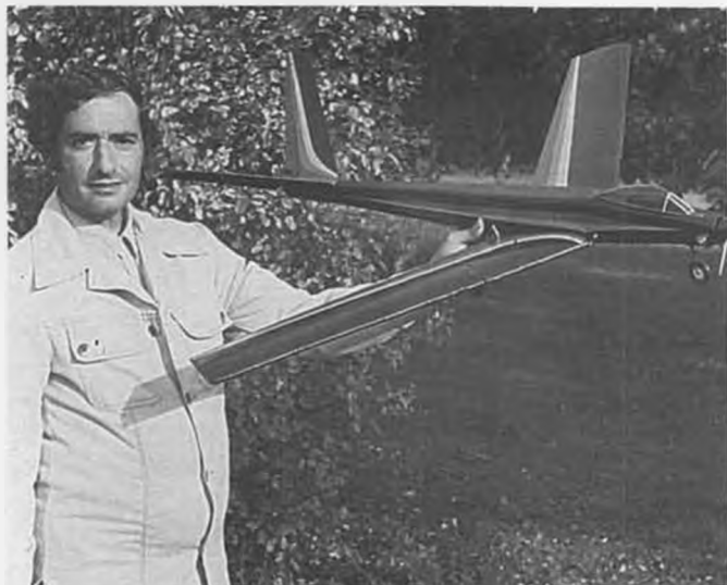
Author/builder with his sleek black beauty. The use of ready-made foam wings from Ace R/C makes construction easy.
