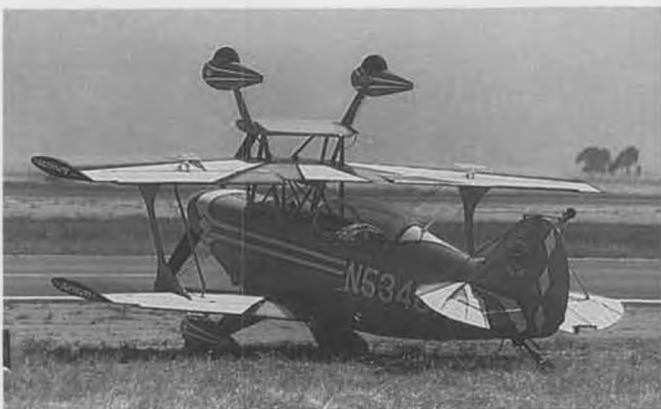
Craig Hosking's Double Take Pitts made upside-down touch-and-gos as well as landings. For takeoff from inverted position, pilot must be hoisted into cockpit with internal winch.
