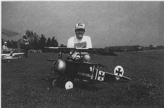
Ed Andrews turned out this six-foot version of a Fokker DR-1. A G-38 hauls this 20-pound tripe around.
