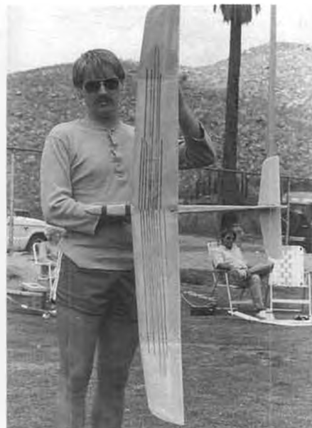
Top view of Wurt's no-name model. Wing is foam core and fiberglass, covered with carbon fiber tow stringers as reinforcement.
