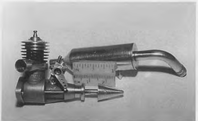
Exhaust system is shaped like Magic Muffler which boosts power over a very broad speed range. Stu didn't use pressure nipple for test running.
