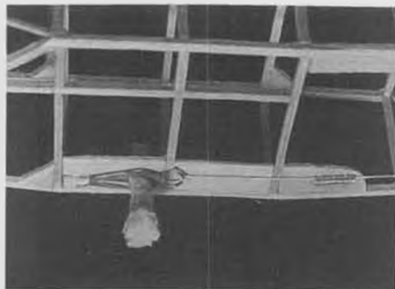
The most sensible location for a D.T. is near the center of gravity, though it involves running the limiting line forward.
