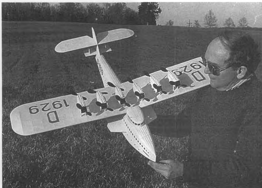
Don Srull with his remarkable free flight Dornier DO-X, featuring 12 electric-motor driven propellers. A good flyer. Photo: Tom Schmitt.
