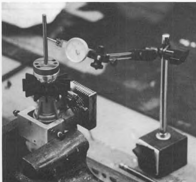
Always use a dial indicator to center the clutch shaft on the engine. Shaft runout should be no more than .003" for minimal vibration and wear.
