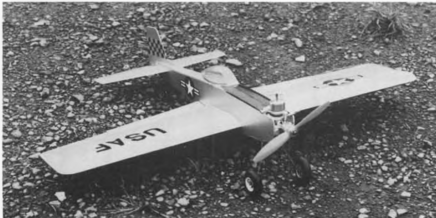
Nathan's 38-inch semi-scale Mustang is powered by a P.A.W. .19 diesel turning a Grish nylon prop.
