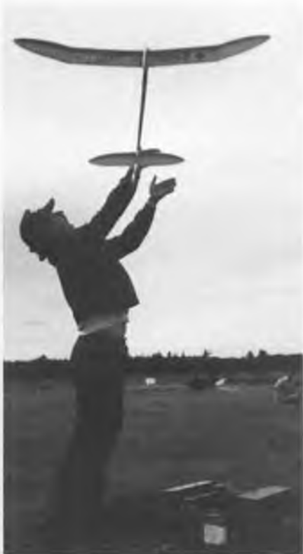
"Deluxe" is the name of this original 1/2A design by Nigel Tarvin, of British Columbia. The ship was inspired by this month's mystery model and features VIT and autorudder. Weight is 6 ounces, wing area 250 square inches. A hot Tee Dee .049 takes it up very quickly. Photo by Barbara Stalick.
