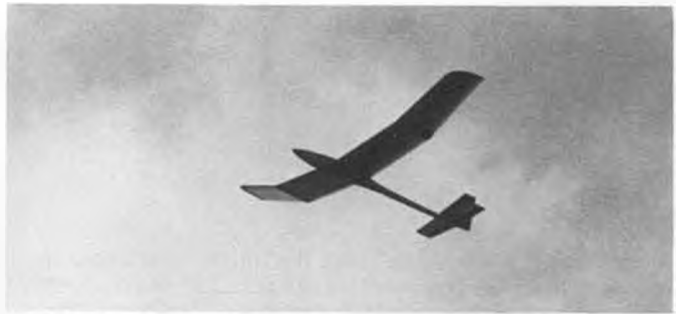
Tony Martin (left) flew this foam-and-glass winged Flinger to 8th place. Model is very clean and fast, but at 16 ounces is too heavy to be really competitive. Tony says his next one will be lighter and will have a Selig 3021 airfoil. Photo above shows the model's semi-translucent trailing edge—a common sight on foam/glass wings.
