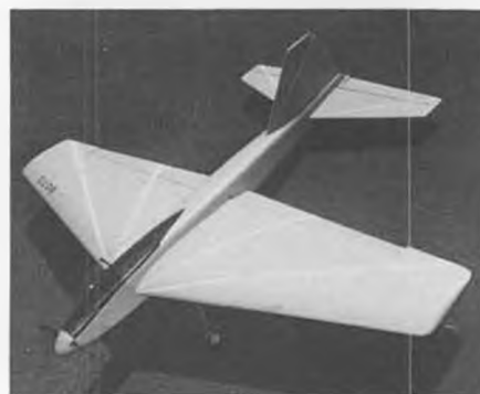
Electric pattern ship by Woody Blanchard uses a Graupner Ultra 1600 motor on 14 cells.
