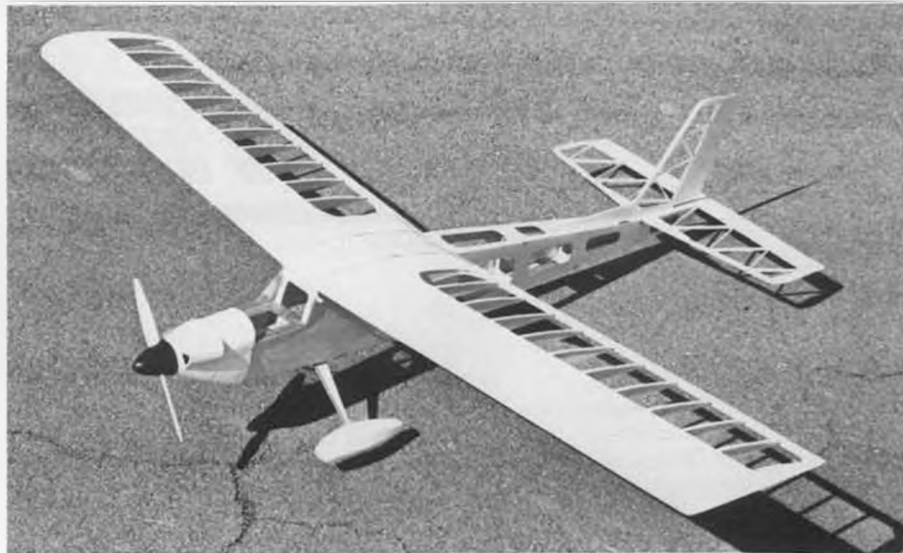
Construction of the Mirage 550 is entirely conventional, with a capstripped D-tube wing and sheet balsa fuselage—note cutouts in fuselage parts for lightness. Span is 54 inches, weighs 50 ounces.
