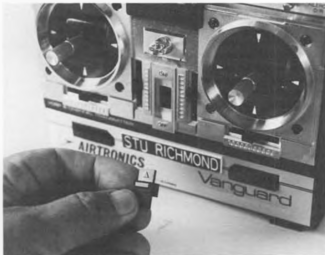
Stu chose to remove the on-off switch actuator on the transmitter; text tells why. Actual switch is recessed into the transmitter case.
