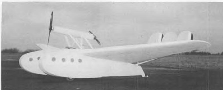
Also from Woody Blanchard comes this photo of his Savoia Marchetti S35X flying boat, a very unusual and successful six-footer powered by two Mabuchi 550 ferrite motors.
