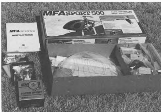
Kit contents are well packed. The Sport 500 is designed for .40 to .45 size engines; this one is powered by an Enya .45.
