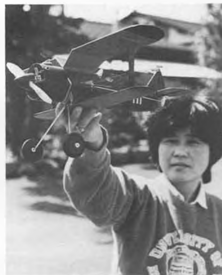
Interesting sheet-balsa Polikarpov I-15, displayed here by Masako Sturman, Nathan's wife, is powered by an Enya .06 diesel.
