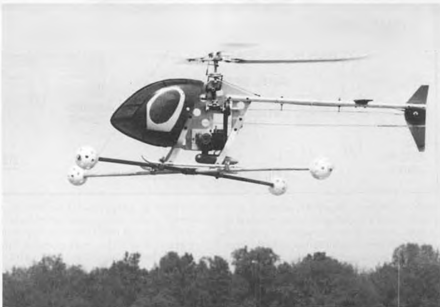
The MFA Sport 500 in a stable hover with the recommended beginner's training skid. This is a simple, inexpensive machine produced in England by Model Flight Accessories and imported into the U.S. by Hobby Lobby International.
