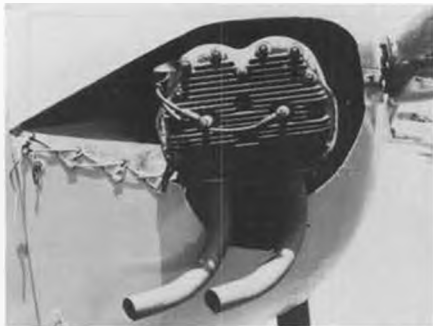
Continental A-40 cylinder head detail as seen on a Cub. Note the sheet metal baffle plate held in place with leather lacing cord.
