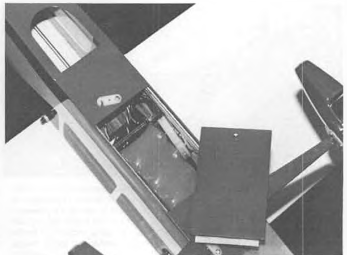
Access to the motor batteries is through a hatch in the fuselage bottom. Opening just aft of the hatch is an exit for battery cooling air.
