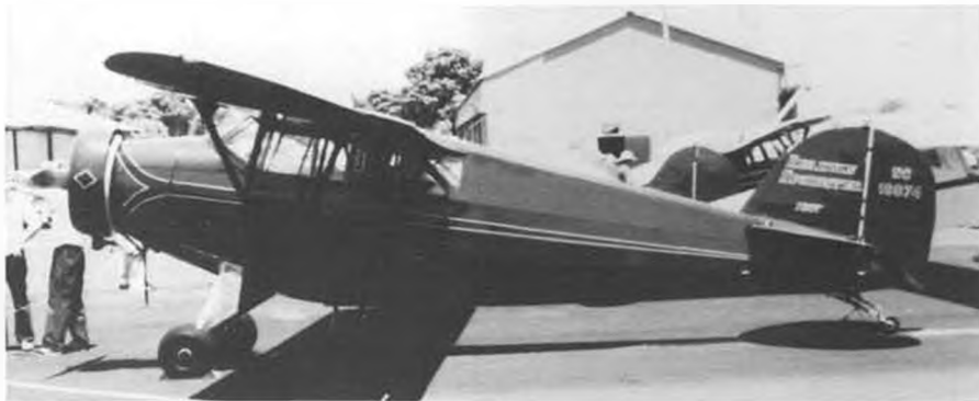
Rearwin Sportster is one of the rarer antiques seen these days. They were built in Kansas from 1935 to 1941 and were usually equipped with LeBlond engines of 70 to 90 hp, with an occasional 90-hp Warner. Fernando says he had a chance to buy one of these planes, in excellent condition, at a Rockford fly-in several years ago for only $2500, and passed it up!
