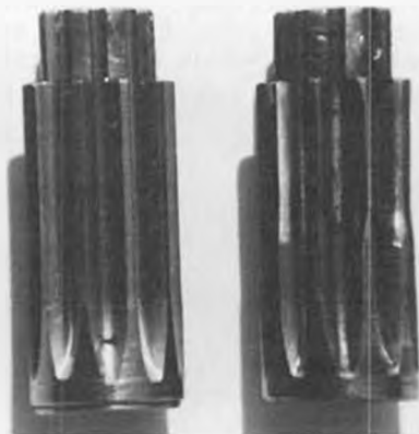
A comparison of new (left) and well-used clutch bell gears. These steel gears will eventually wear out just from routine use.
