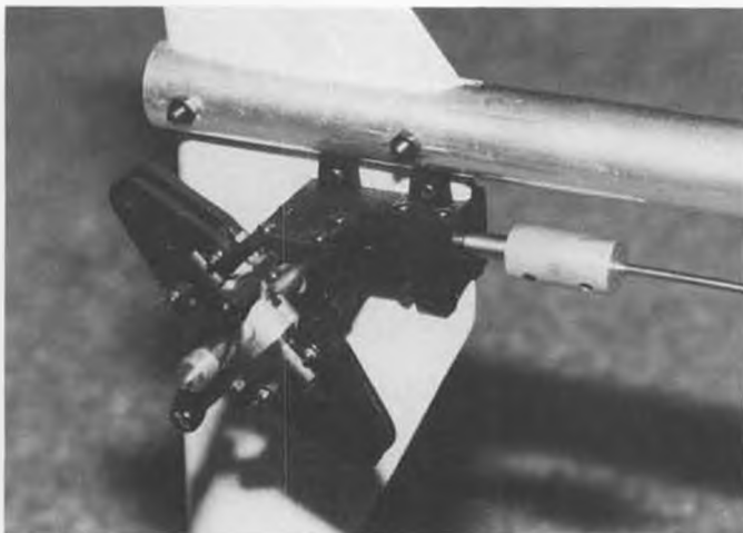
The tail rotor gearbox is mounted on the wooden tail fin to keep the tail rotor drive shaft straight. The instructions show the tail rotor facing to the left, but our author mounted it on the right because it's more efficient to have the rear-most tail rotor blade rotating downward.
