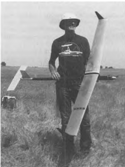
Ken Oliver's V-wing FAI model is a state-of-the-art design featuring an aluminum covered wing, tiplets, and shallow dihedral. See the March/April '89 F/F column for more details on this design concept. Wil Nakashima photo.
