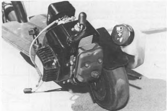
A close-up of the 1.4 hp Zenoah engine on the Go-Ped. Tires are solid rubber, not pneumatic, and should last a lifetime.
