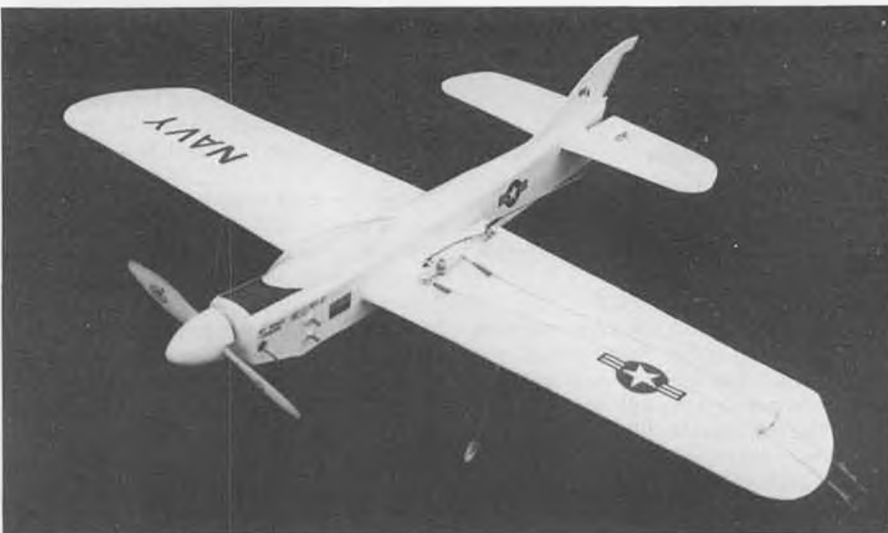
The "Novi" is one of Nathan Sturman's smaller C/L models, spans 32 inches and flies up a storm with a P.A.W. .09 diesel and 8x5 MK prop. Covering is tissue and dope.
