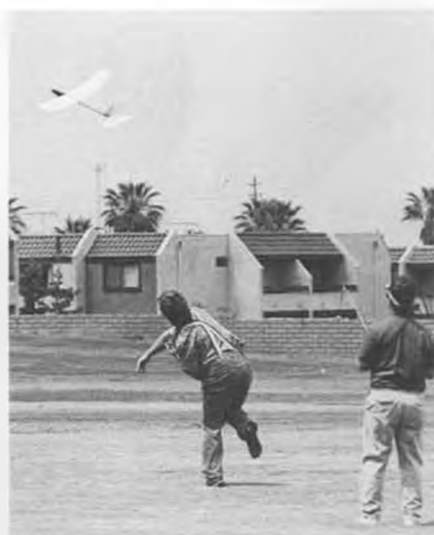
Charlie Morey's "Greg Oakert Vader Plane" gets a strong toss from Gary Anderson. Model spans 50 inches, weighs a mere 12 ounces, and has a Jack Chambers #18 airfoil.
