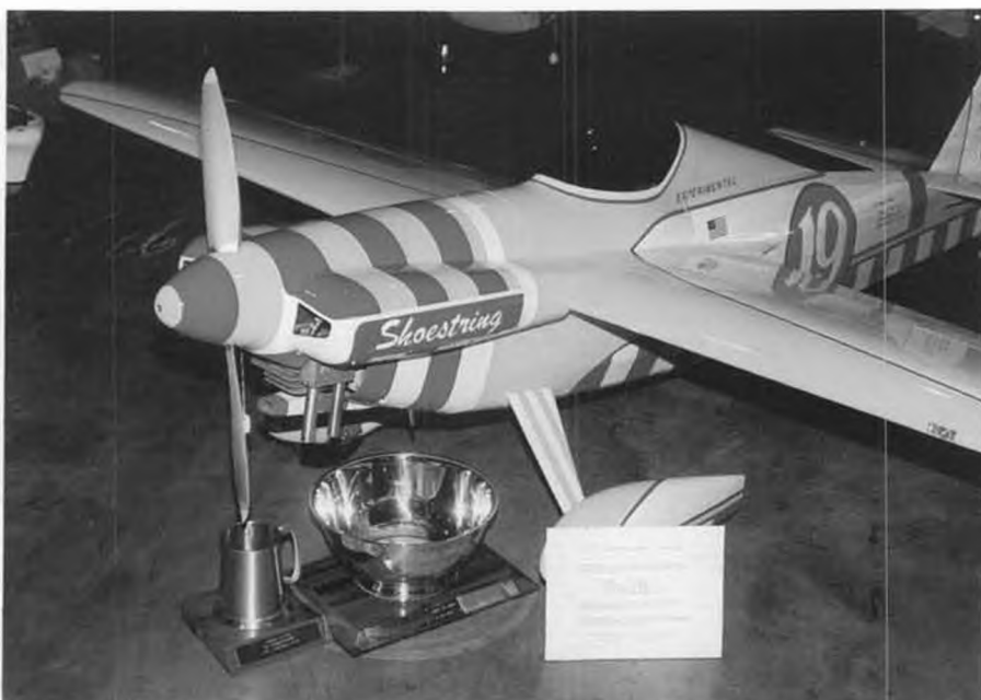
Winner of "Best of Show," and of course, first in its category, Giant Scale, is this K-10 Shoestring by Greg Waits. He used Bob Morse plans (now from Bob Holman Scale Plans), Dan Parsons cloth and Micafilm, K&B satin epoxy base under DuPont 580s clearcoat. Power is a Sachs Dolmar 4.2 cu. in. on C.H. throttle coupled ignition, with 6-volt, 900 mA battery. Zinger 22x14 prop. Radio is JR PCM9, with Futaba 9201 and 31s coreless servos. SR 6-volt 2000 mA battery through JMP 5.2-volt power supply.
