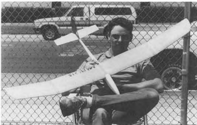
Tony Martin (left) flew this foam-and-glass winged Flinger to 8th place. Model is very clean and fast, but at 16 ounces is too heavy to be really competitive. Tony says his next one will be lighter and will have a Selig 3021 airfoil. Photo above shows the model's semi-translucent trailing edge—a common sight on foam/glass wings.
