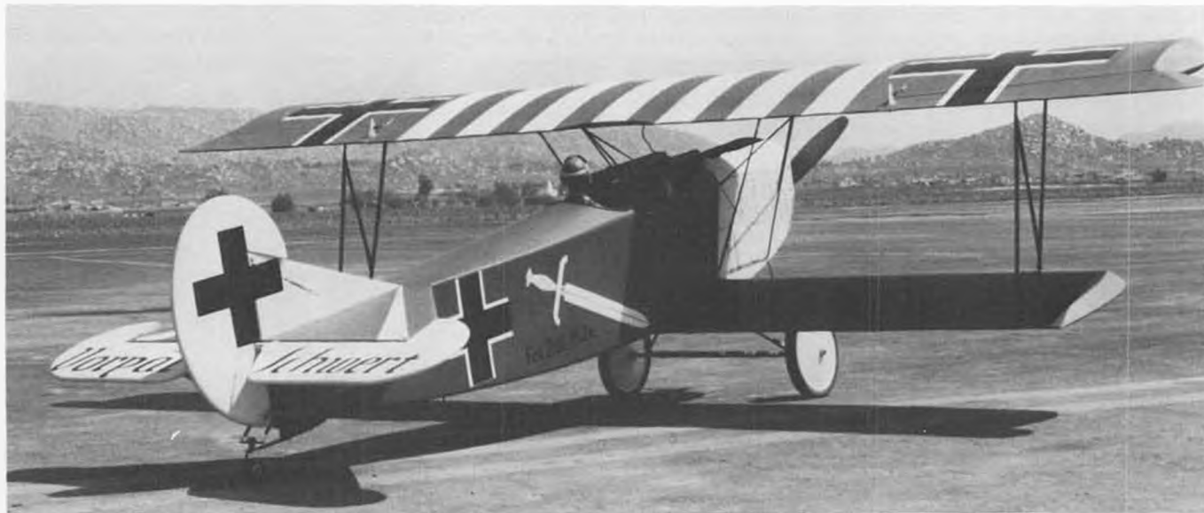
Pretty shot of a colorful Fokker D-VII by an unidentified builder. It's Quarter Scale, but a little smaller, being a 3" = 1' model of a 7/8-size replica that was built specifically for film work. Model weighs in at 15-1/2 pounds, is powered by an ST-2500.
