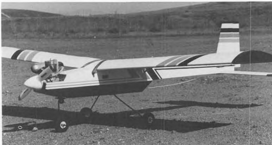
This month's featured ARF is the "Golden Wind II," imported from Taiwan and sold here in the U.S. by the Ten Plus Company in Santa Fe Springs, California. It's a four-channel ship for .25 size engines.
