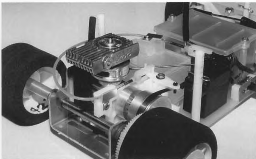
Cox Hobbies showed the prototype of its new, under-$100, R/C gas engine powered car. Real fine engineering, and it has a muffled .049 over the rear axle.
