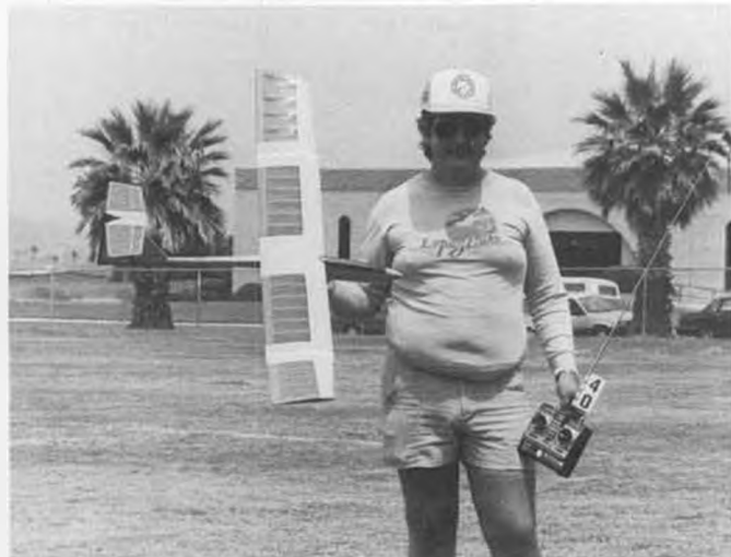
T-tail RO-8 look-alike is the work of Mike Petten. Features a Sellg 3010 airfoil, 59-inch span, 7-inch root chord, 6.5-inch tip chord. Needs "a couple of refinements" before it will be fully competitive.
