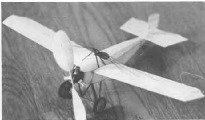
Two of Stan Fink's indoor Peanuts are the Caudron 11 (above) from Larry Kruse plans, and a French Bebe Jodel homebuilt (right). The Caudron weighs in at only 4.5 grams; the Jodel goes 6 grams and is good for over 40 second flights.
