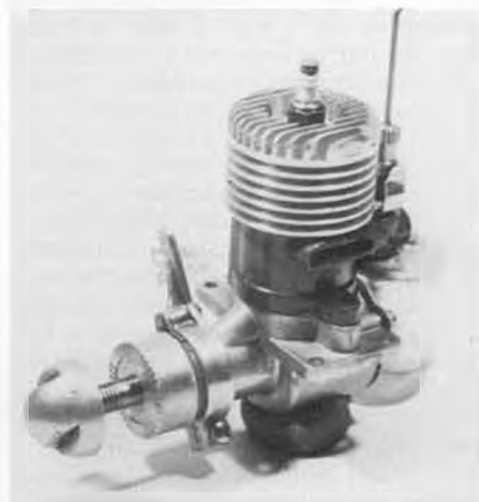
3. Karl Spielmaker did a nice job reworking this "Thor" slag engine. Modifications include a new, larger cylinder fin assembly. Turns a 10x4 prop at 8000 rpm.
