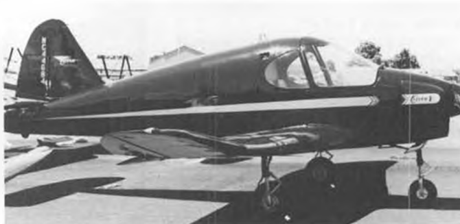
Culver V of 1946 carried 85 hp, featured retractable tricycle gear and dihedralled tips. This one is red overall with silver trim.
