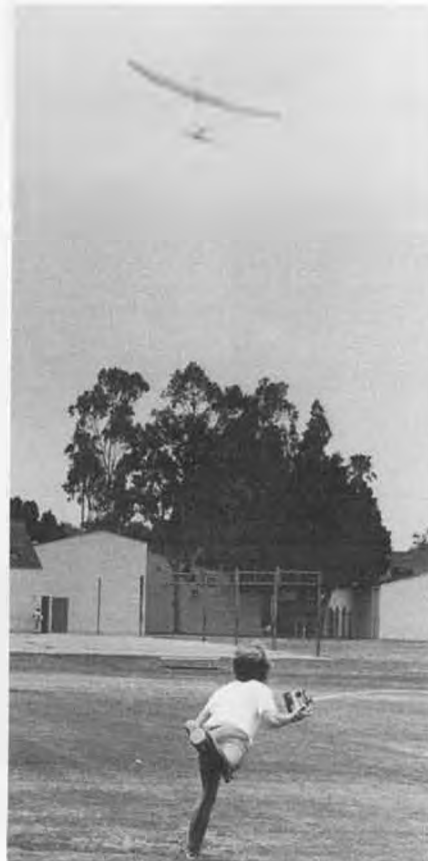
Our columnist's “3 a.m. special” modified Flinger finished the night before the meet. Schuemann wing tips with extra dihedral bring the span to a full 59 inches. Tips will stall if the plane is yawed sharply and will be removed pronto! Tail surface chords have also been increased by 1/2 inch.
