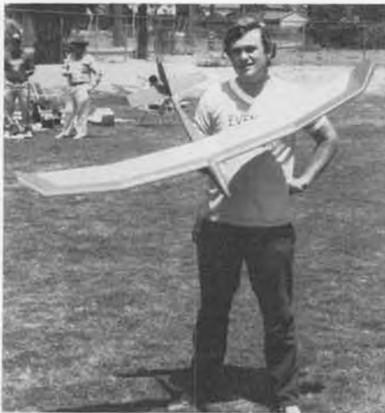
Our columnist's “3 a.m. special” modified Flinger finished the night before the meet. Schuemann wing tips with extra dihedral bring the span to a full 59 inches. Tips will stall if the plane is yawed sharply and will be removed pronto! Tail surface chords have also been increased by 1/2 inch.
