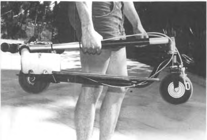
The Go-Ped's steering column folds down for easy transport and storage. All-up weight is only 21 pounds. can do up to 18 mph.
