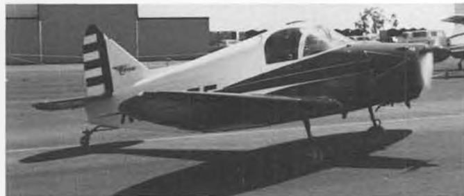
One of the four 1940 Al Mooney designed Culver Cadets that showed up at Merced. With its cantilever wing, retractable gear and 140 mph top speed on only 75 hp, the Cadet was way ahead of its time and is considered a sprightly performer even by today's standards.
