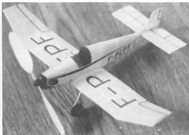
Two of Stan Fink's indoor Peanuts are the Caudron 11 (above) from Larry Kruse plans, and a French Bebe Jodel homebuilt (right). The Caudron weighs in at only 4.5 grams; the Jodel goes 6 grams and is good for over 40 second flights.
