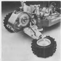
Sealed gearbox VariLok differential
