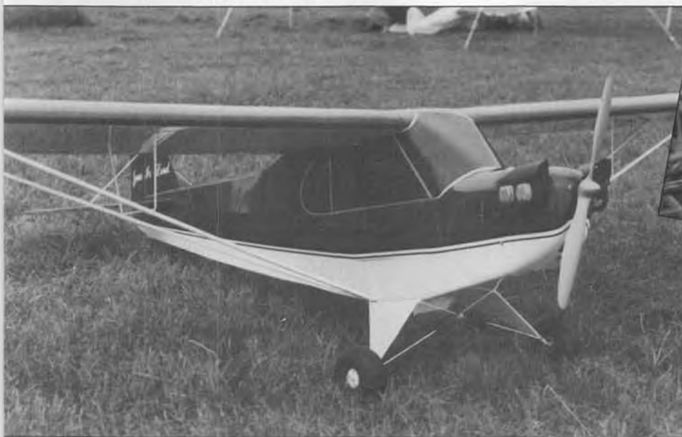
(Above) Bare bones close-up of Kirk Massey's Cub shows the battery installation and the extensive use of lightening holes in the cabin area. (Right) A lightened Bud Nosen kit was the basis for this very nice 1/4-scale clipped-wing Cub built by Kirk Massey in 1985 and flown regularly by him ever since. Weighs only 11 pounds with an Astro 60 and 27 cells.
