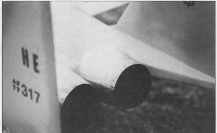
Plastic tailpipe cones were painted silver and then dry-brushed with a little red and blue paint to make them look hot.
