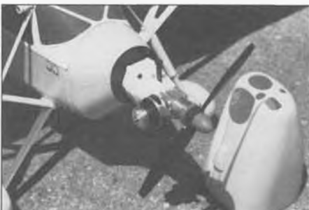
The Cox .049 Ranger engine, with cowl removed. Skip found it better to turn the muffler exhaust exit downward to keep residue away from the decals.
