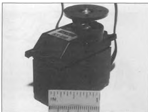
Stu crash-tested four of these standard servos from 400 feet at full throttle vertically into hard ground. All survived due to clever engineering as test tells and this picture shows.
