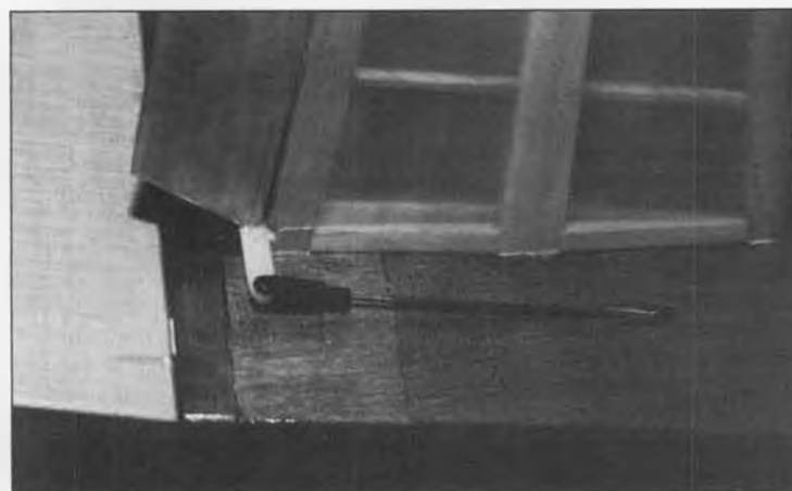
Elevator linkage detail. Tail surfaces are glued permanently to the fuselage. The prototype Quietus was covered entirely in good ol' silk and dope, but any of the lighter iron-on films could also be used.
