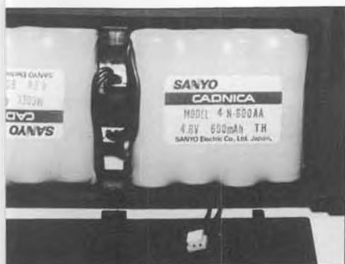
The Advance PCM5 system uses three identical high quality NiCd battery packs. These two power the transmitter.
