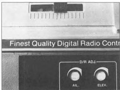
When the smoked gray door on the front of the transmitter is lowered you have access to the adjustable controls. Trim levers have positive clicking detents.
