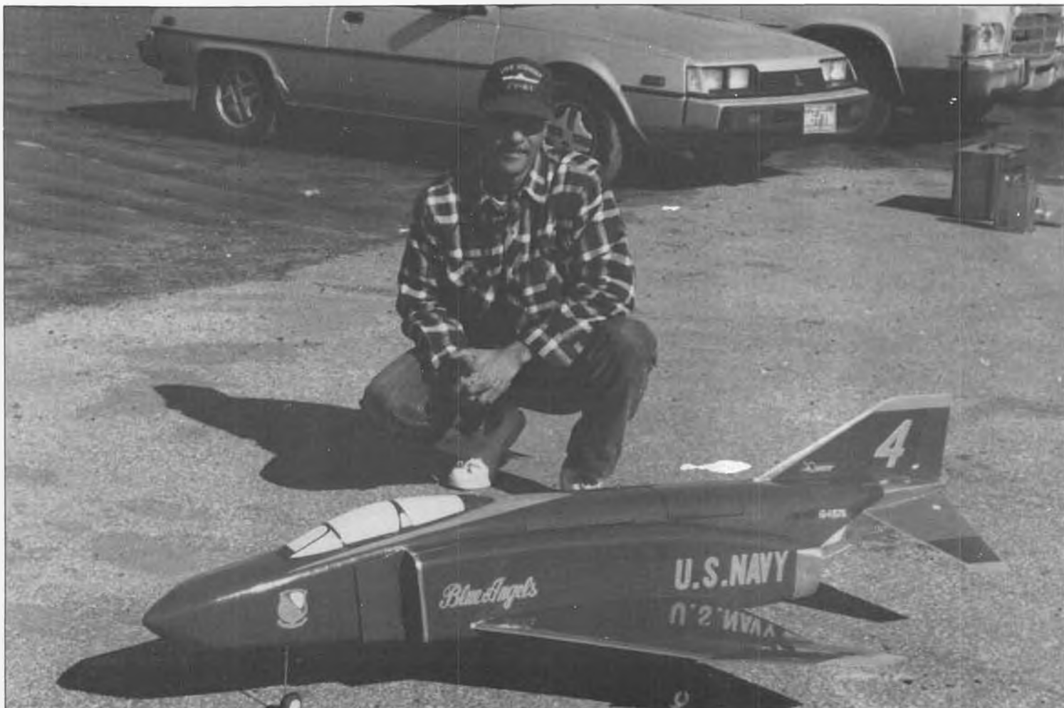
John Whitmore couldn't be more pleased with his scratch-built F-4 Phantom ducted fan, which is all the more unusual in that it is powered by a diesel converted Rossi .65—see text for details. The airplane performs well in spite of the fixed landing gear.
