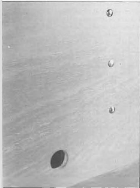
The lower back and shelf are attached to the legs with standard hardware store carriage bolts, nuts and washers. The large holes in the back pieces are there for the passage of wires for electrical items that might be placed permanently on the bench.
