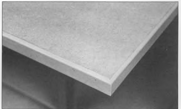
The workbench top, which is made from a common flush door, and all the plywood pieces are given a more professional look with wooden edging available from any building supplier. The molding is attached with white glue and finishing nails.
