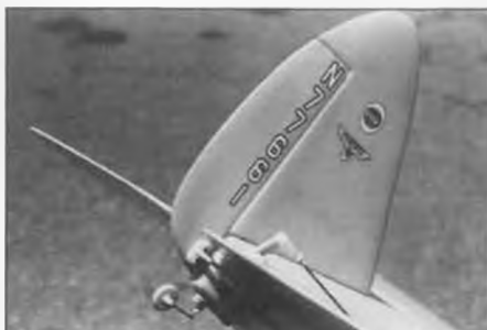
Close-up of pushrod attachment to tail surface control horns.
