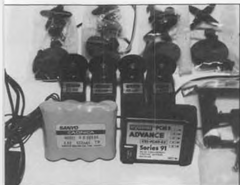
These components receive the transmitter's "uplink" information. Murphy's Law of Radio Testing took effect when our test crew overflew the capacity of the airborne battery during their enthusiasm for this totally terrific performing system... see text.
