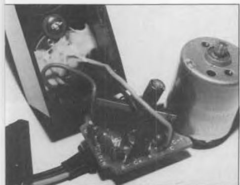
These servos closely parallel the final generation Kraft servos. The suggestion has been made that the three wires to the circuit board lettered "A", "B", and "C" also receive a dab of the mastic for vibration protection.
