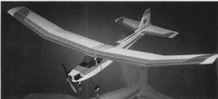
ELECTRIC SUNDANCE 55" Wingspan 31" Length Electric Motor Powered
