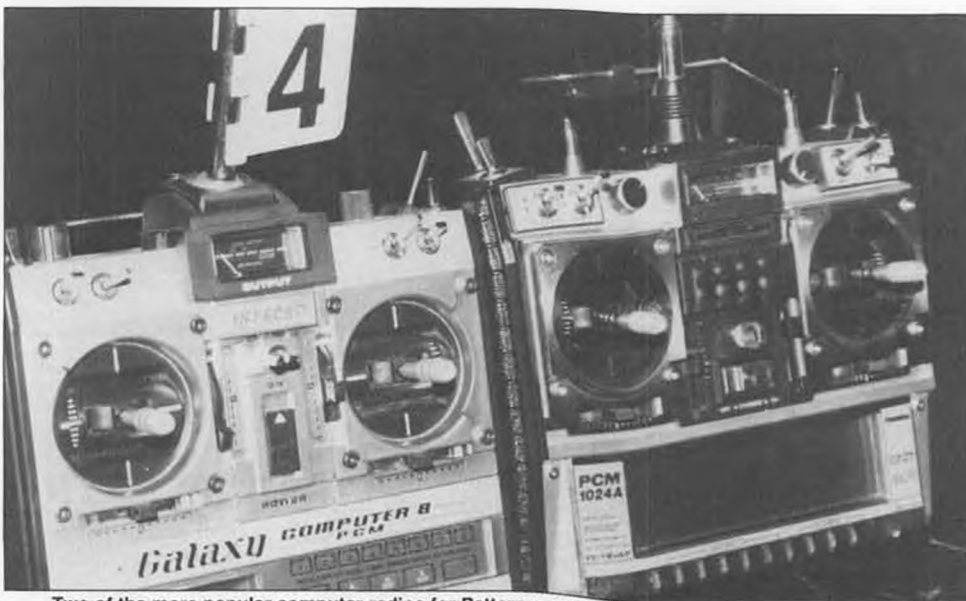
Two of the more popular computer radios for Pattern are the JR Galaxy Computer 8 PCM (left) and the Futaba 1024A PCM.
