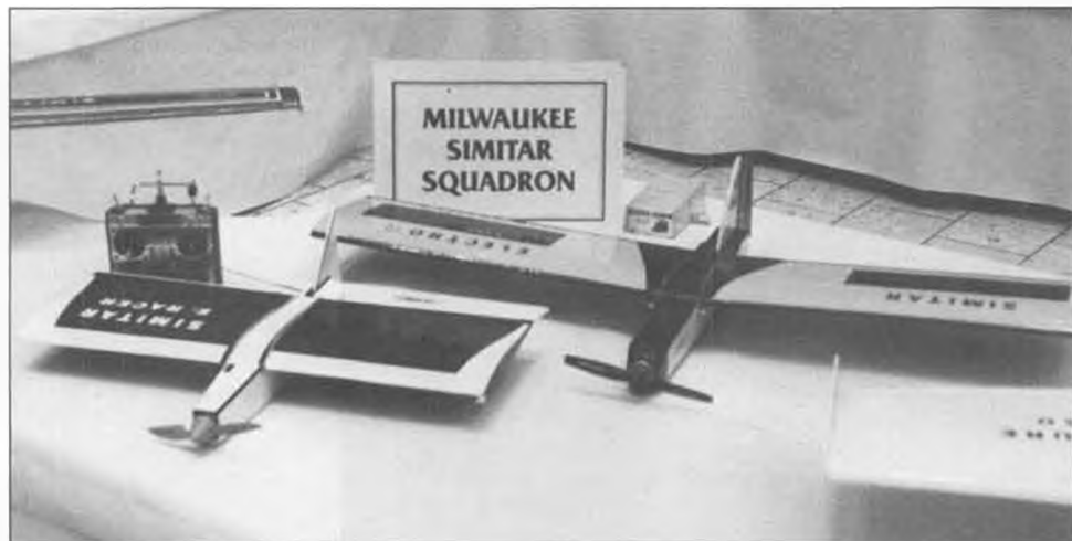
Two more of Gordy Stahl's variations on the Simitar theme are the "Simitar E-Racer" (left) with Graupner Speed 600 motor, and the "Simitar Electro-Q" with Astro 25. Gordy is the Commander of the Milwaukee Simitar Squadron.
