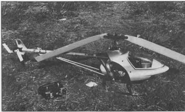
Oh no! James' banged-up Excalibur is the result of pilot error—an improperly executed low-altitude roll. Doesn't look too bad, but the broken canopy and fins, cracked main rotor hub, bent main shaft and flybar, and
