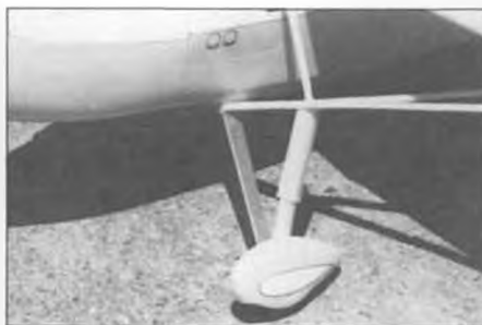
Close-up of landing gear and wing strut combination, a trademark of the Fairchild 24. Main landing gear strut of pre-bent and drilled aluminum actually takes landing loads.
