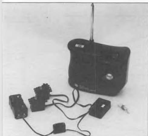
The complete Cobra radio system, with sensible single stick control for rudder and elevator. Odd transmitter shape is more comfortable in the hand than the usual square box.
