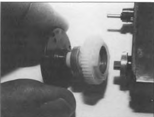
Unlike other servos seen so far, these K-100s with the Advance systems have dual bearings on the output shaft for maximum mechanical support. The R/C Think Tank feels this system beats a single ball bearing at the top of the shaft... as some upscale servos use.
