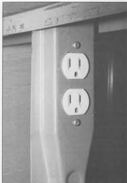
The recommended pre-formed metal bench legs come with knockout mountings for electrical sockets on both the front and rear legs. Wiring the front sockets is definitely recommended, as they are in an extremely handy location. Rear ones are optional.
