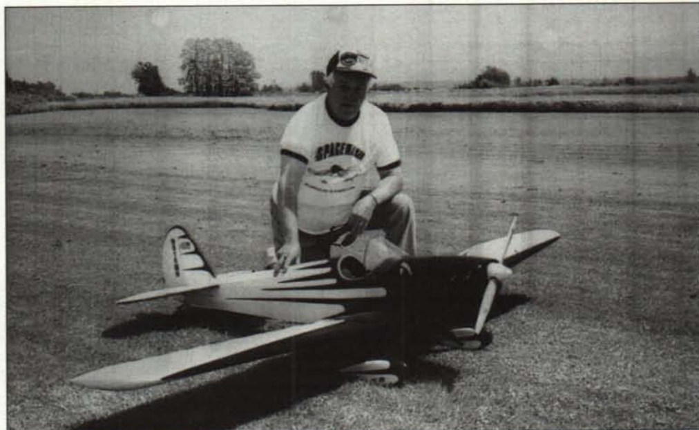
Ralph Graham enjoys flying his Sig Spacewalker. It has flaps and is powered by a Kawasaki 3.3 cu.in. engine with CH spark ignition.
