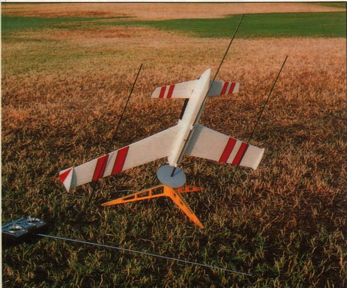
All set to go! Note the two guide wires out at the wing tips, which stabilize the model while on the launch pad.
