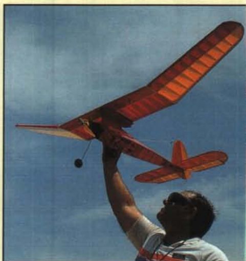
Contest Director Jo Lupberger measures Skinner's landing for bonus points. Jim won Seven-Cell Sailplane with this ship, which boasts a built-up balsa sheeted wing with flaps deployed by rubber band power—once per flight!
