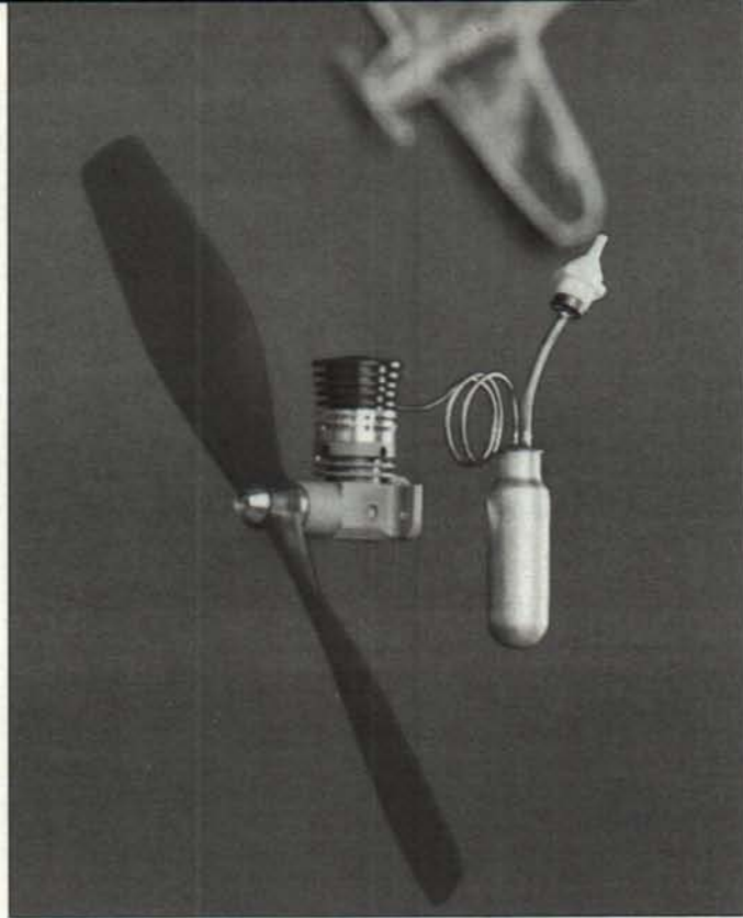
The Swiss Heibi CO 2 motor, 0.08cc displacement. An excellent example of Swiss craftsmanship!
