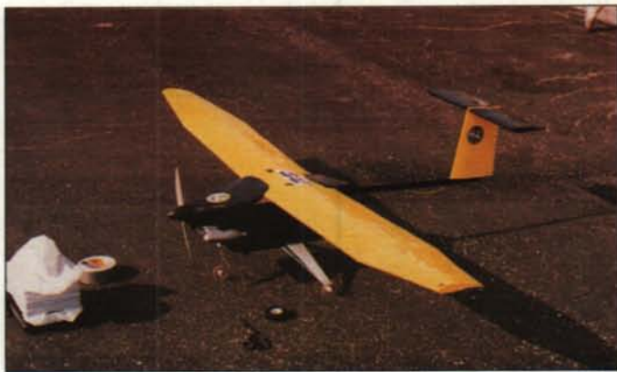
Highly tapered wing tips and clear acrylic wheels characterize the 87-inch span, T-tail entry from the University of Waterloo, Ontario, Canada.
