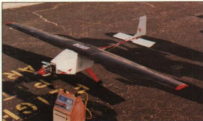
The University of Cincinnati's entry lifted 10 lbs., 8 oz., appears to have a fairly thick wing skinned with carbon fiber. Note the canard foreplane just behind the firewall.
