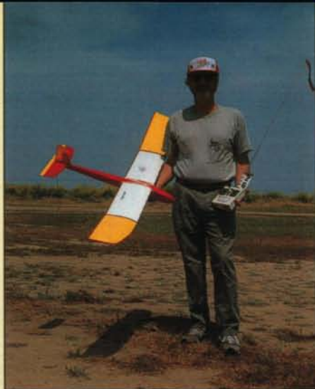
Chuck Grim's Astro Mini Challenger was the only sub-05 model entered in the Champs. All things considered, he did very well with the little direct drive 035 Astro Cobalt on six cells and a Graupner 7x3 folder.
