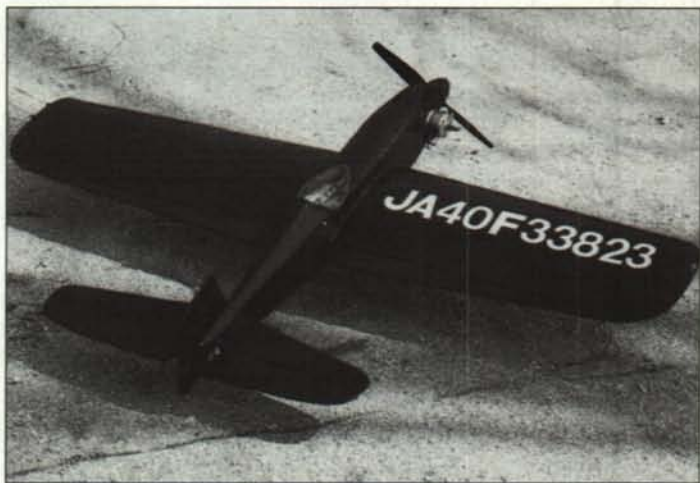
Nathan Sturman, an occasional correspondent from Shibukawa, Japan, was proud of this P.A.W. diesel-powered Kimura Skylark .15...until it met its untimely demise as the result of failure of an aluminum retainer spring on the pushrod at the flap horn. Nathan recommends solder!
