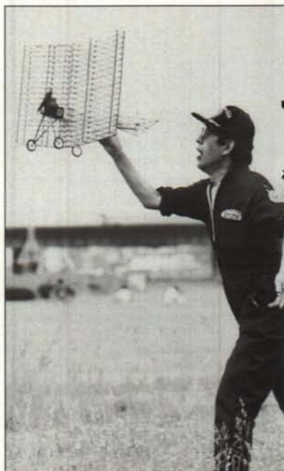
How would you like to cut out the wing ribs for this one? Akira Igami, of Japan, launches his 20-winged Phillips multiplane. And, yes, it does fly!
