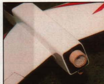
The D-11P motors are an easy slip fit inside the motor mounting tube. It's not readily visible here, but there's a small metal clip that holds the motor in place and keeps it from falling out when the model is on the launch pad.
