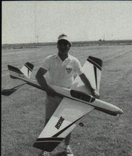
FAI pilot Bob Crump with his brand new Chidgey Typhoon. All balsa, 1000 sq. in. wing, YS 120 powered, JR PCM-10, 9.75 pounds. It flew very well.
