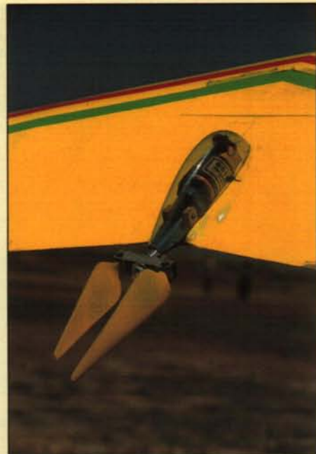
Left: All eyes were on Kris Larson's Klingberg Wing every time he flew. Addition of electric power brought the flying weight up to 42 ounces, for a wing loading of 14 ounces per square foot. Above: The Klingberg Wing's power system—Astro 05 FAI, Leisure Electronics long gearbox, and Sonic-Tronics 11x6 prop, all enclosed in a standard clear plastic canopy.
