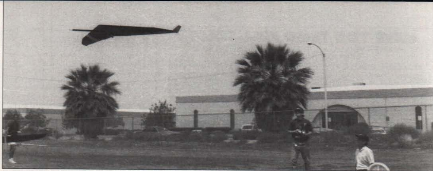
Launch! First-ever electric winch launch for this particular Klingberg Wing 100, Bill Forrey on the sticks. He was impressed by the model's "on rails" stability during tow. Launch height, while only average compared to conventional (tailed) models, is good for a wing.
