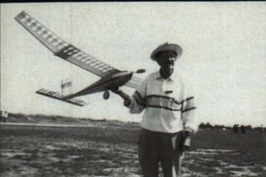
Our vote for the most unusual electric went to Frank Wetherill's "Quasimodo" seven-cell entry. Foam core wings and wheels, carbon fiber reinforced spars, homemade folding prop and gearbox, wire wing bracing, and pull-pull control cables were just a few of its many unusual features.
