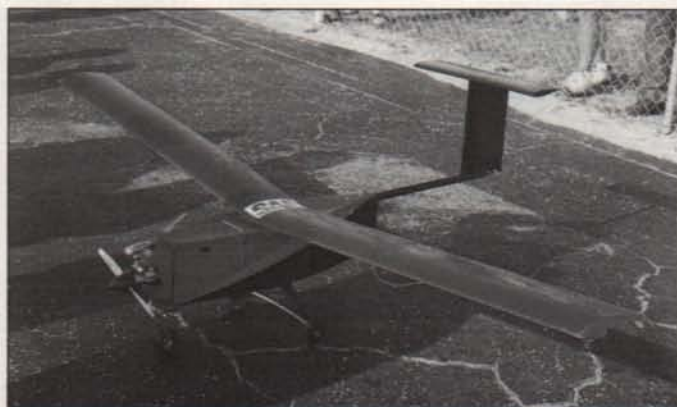
This basic, straightforward design from the Milwaukee School of Engineering lifted just over 13 lbs. Note the full-span flapersons.
