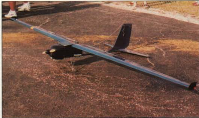
The two teams from Cedarville College entered identical ships based on this 12-foot, high aspect ratio design. Best lift was 14 lbs. plus. Like most others, this entry uses a tubular aft fuselage for minimal planform area (see text for rules).
