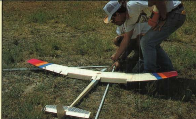
Contest Director Jo Lupberger measures Skinner's landing for bonus points. Jim won Seven-Cell Sailplane with this ship, which boasts a built-up balsa sheeted wing with flaps deployed by rubber band power—once per flight!
