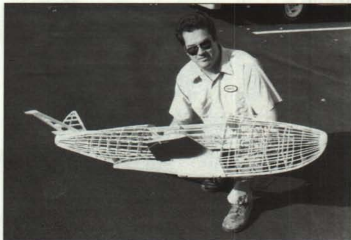
Grant Heistand with the fuselage framework of his electric-powered scale Boeing 314 flying boat. We'll publish a report on the finished product when it's available. See text for details.
