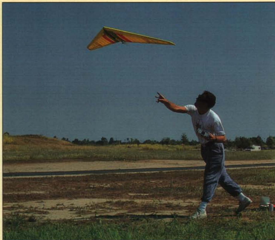
Chuck Grim's Astro Mini Challenger was the only sub-05 model entered in the Champs. All things considered, he did very well with the little direct drive 035 Astro Cobalt on six cells and a Graupner 7x3 folder.
