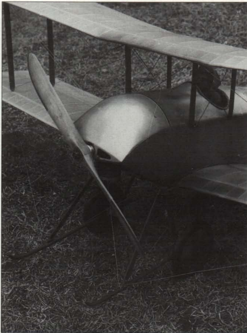
Unusual cowl shape originally housed a LeRhone 80-hp rotary engine.
