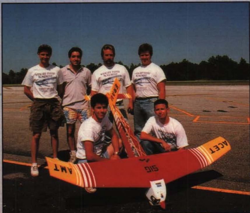
"Eagle III" was flown by one of the four Embry-Riddle Aeronautical University teams. Best lift was 15 lbs., 7 oz. Note how they minimized the alt fuselage's planform area—by leaving the top and bottom uncovered!
