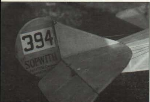
The sum total of the decoration on the Tabloid is right here. Controls are operated by stranded steel cables. Curved outlines are laminated 1/32 balsa strips.
