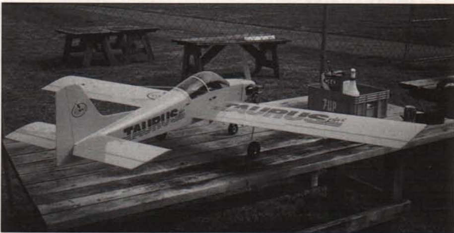
Fred Pierce says his "Taurus Plus" is a good sport flier. It is kitted in Germany and imported into the U.S. by Hobby Lobby. The big ship weighs eleven pounds, has an 82-inch wingspan, and the flaps make landing a breeze. An O.S. 1.20 four-stroke provides the thrust.
