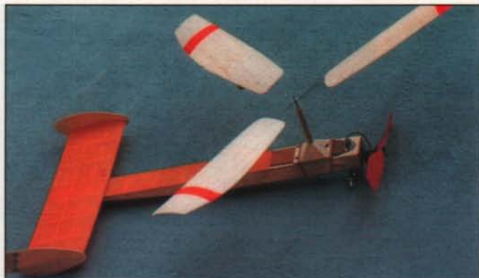
Another of Fritz Mueller's creations is this CO 2 powered autogyro, with exceptionally slow-turning rotor blades.
