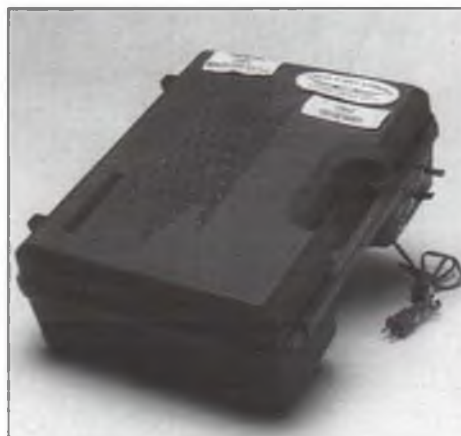
■ LEFT: The author's completed charger case holds two Astro Flight chargers, a digital voltmeter for manual peak charging, and an assortment of adapter cords. The AC power cord from the AFI Model 115 AC/DC charger allows you to charge packs of up to seven cells from house current before leaving for the field. ■ CENTER: The chargers and digital voltmeter as mounted in the pistol case. Adapter cords are stored in an open space in the other half of the case. ■ RIGHT: Close-up of the installed switches. The foam is cut out, the switches are installed and wired, then the foam is stuffed back into the hole to conceal the works.
