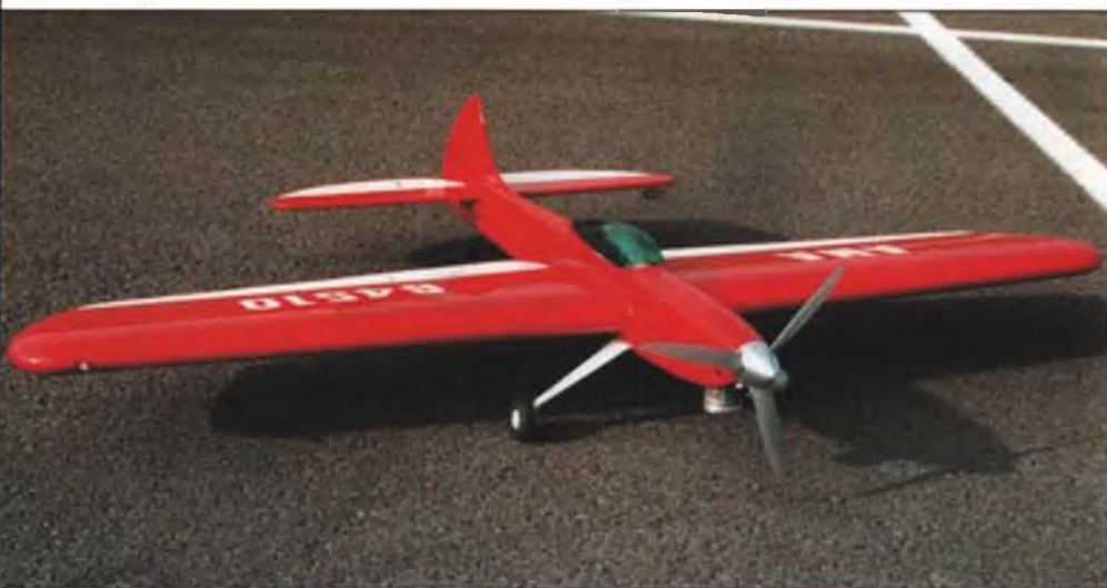
Gerald Schamp's Big Oriental is based on Ted Fancher's Imitation design, adding a full fuselage in the Oriental shape. It has 640 square inches and uses a Tom Lay Super Tigre .60 and a Bolly 11-1/4x6-1/2 three-blade prop. Gerald Schamp photo.
