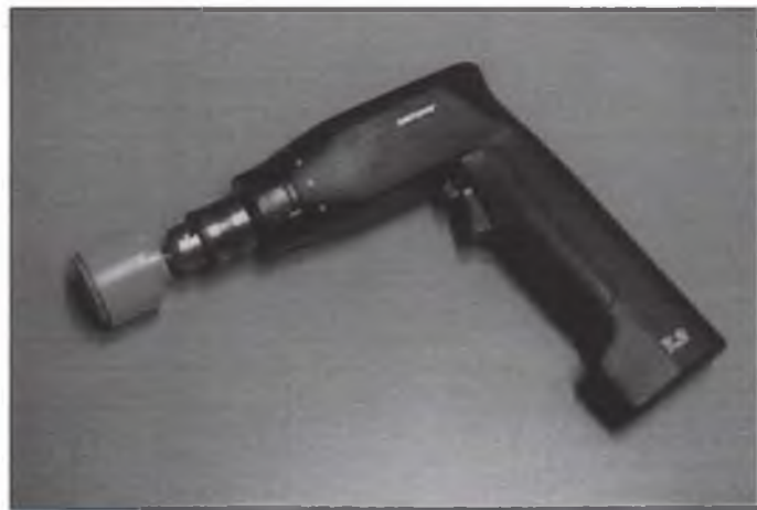
As an experiment, Francis tried using a Craftsman cordless drill/driver as an engine starter. No good—plenty of torque, but not near enough rpm (about 500).
