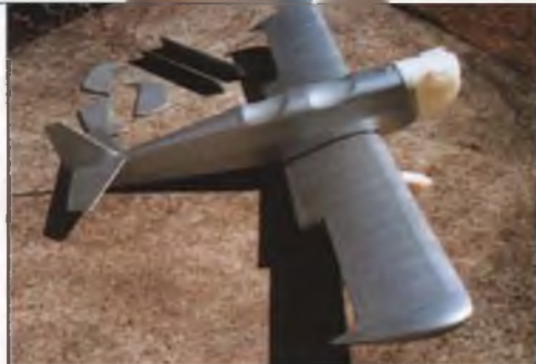
■ LEFT: Here the basic framework has been framed up and covered with Sig Koverall, a heat-shrink polyester material popular with the Giant Scale crowd because of its easy handling and extreme puncture resistance. Covering is adhered with "Stix-It," a heat-activated adhesive also produced by Sig. ■ RIGHT: To provide an opaque base for the color coats, the model was first given two brushed coats of Sig clear nitrate dope, followed by three sprayed coats of Sig butyrate dope with aluminum paste added. Bruce described the Spacewalker's finishing process in considerable detail in his March '93 "Big Birds" column.
