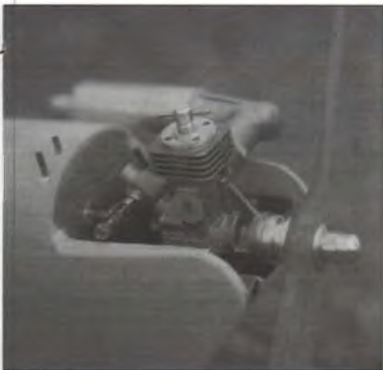
■ LEFT: Photo No. 7. Beautifully made ABC square-fin .21 diesel by that Australian master of the engine building art, Gordon Burford. It's a rear-intake design that appears to use an O.S. RC carb assembly. Gordon has this engine mounted in a V-K Challenger and another in a Kanga Cab. ■ RIGHT: Photo No. 8. Here's one you don't see every day: a Hal DeBolt "Blitzkrieg," this colorful example built by Albert Fisher of Australia. The 53-inch model weighs in at a very light 24 ounces and is hauled aloft by a Super Tigre X-11.
