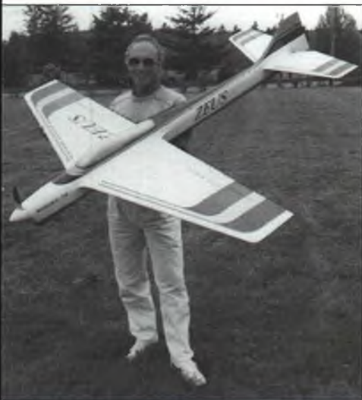
NSRCA District 8 VP John Noster of Eugene, Oregon, and his new Zeus design for FAI. About 925 square inches, 10 pounds, YS 1.20AC and Futaba 92AP radio. A fine flier, and John isn't bad either.
