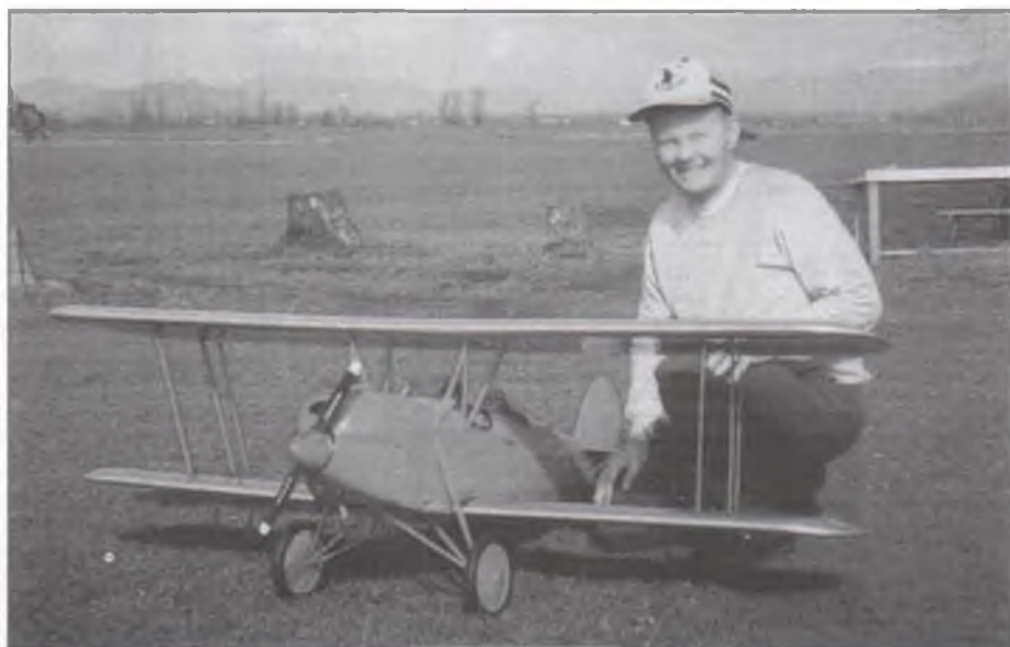
Bill Pottage built this gorgeous Waco 10 from an Ikon N'wst kit. It's powered by an O.S. .91 four-stroke. Bill says it's a great flying model, something you can shoot touch-and-go's with all day long and never get bored.
