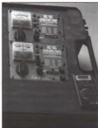
■ LEFT: The author's completed charger case holds two Astro Flight chargers, a digital voltmeter for manual peak charging, and an assortment of adapter cords. The AC power cord from the AFI Model 115 AC/DC charger allows you to charge packs of up to seven cells from house current before leaving for the field. ■ CENTER: The chargers and digital voltmeter as mounted in the pistol case. Adapter cords are stored in an open space in the other half of the case. ■ RIGHT: Close-up of the installed switches. The foam is cut out, the switches are installed and wired, then the foam is stuffed back into the hole to conceal the works.
