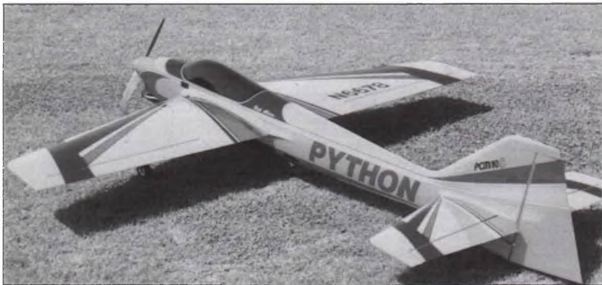
The author's new Python from Pioron Models on its maiden voyage to the field. The 950 square inch, 10.5-pound bird is a super flying machine. Rick is using a JR PCM-10S rig. Plug-in wings, stab, and two-piece fuselage fit in a 43x28x14-inch carrying case!
