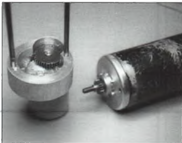
■ FAR LEFT: Dissatisfied with the performance he was getting out of his commercial direct-drive electric starter, our columnist made up this all-metal 2:1 gearbox to double the available torque. Output shaft appears to be riding in an oilite bushing, with possibly some sort of thrust bearing setup directly behind the starter cap. Works great! ■ LEFT: Gearbox is held in place by means of the two long bolts that hold the front and rear starter covers in place. No-load output rpm is 2,800, which is close to the idle speed on most common .60s.
