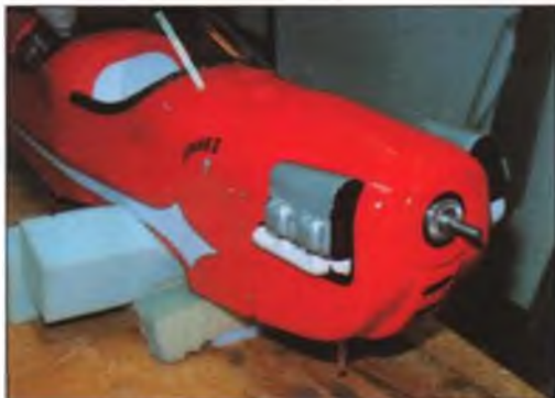
■ LEFT: The dummy Continental engine is molded from ABS plastic and is included in the Spacewalker II kit. Bruce spent some extra time getting the cylinder cooling shrouds to look just right—time well spent, as the finished product adds greatly to the model's appearance. Bruce recommends painting the engine parts before gluing them to the cowl, which would have saved him a lot of masking work. ■ RIGHT: Du-Bro rigging pins and clevises make excellent rudder controls and tail guy wire attachments. Tail wheel assembly is part of the large hardware package that comes with the kit. It's also available separately for scratch builders; see "Over The Counter," July '93 MB.
