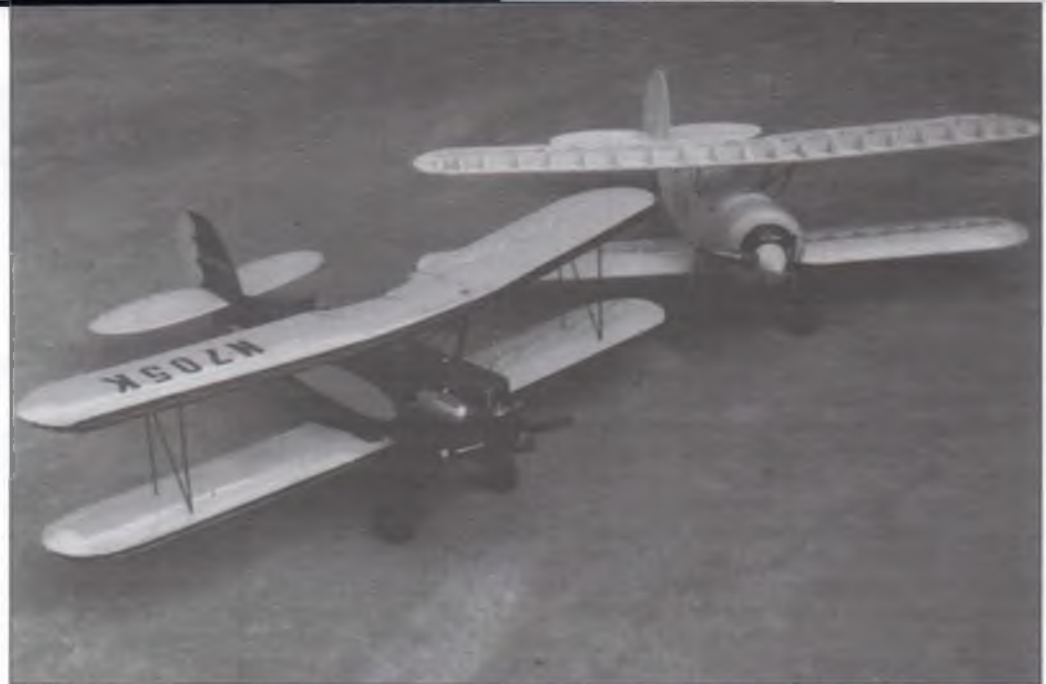
The plans show both the in-line (90-horsepower Cirrus) fuselage and a latter "round engine" fuselage typical of the higher-powered radial engine aircraft. The rest of the airplane is the same.
