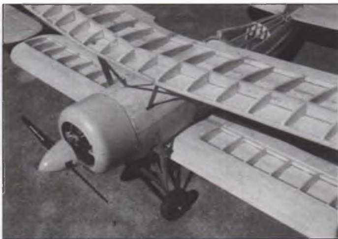
■ LEFT: Here the powerful Great Lakes is almost ready to cover. Note the wing construction—fully sheeted on the bottom, sheeted from the spar forward on the top. This is typical of all of AJ's EEE-Z-FLJ efforts. ■ RIGHT: Three EEE-Z-FLJ oldies but goodies: the two versions of the Great Lakes being followed in close formation by AJ's Staggerwing Beech (MB plan #2921, $14). AJ has still more semi-scale projects coming—watch for 'em!
