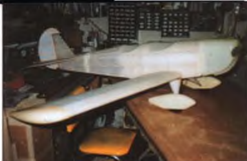
■ LEFT: Here the basic framework has been framed up and covered with Sig Koverall, a heat-shrink polyester material popular with the Giant Scale crowd because of its easy handling and extreme puncture resistance. Covering is adhered with "Stix-It," a heat-activated adhesive also produced by Sig. ■ RIGHT: To provide an opaque base for the color coats, the model was first given two brushed coats of Sig clear nitrate dope, followed by three sprayed coats of Sig butyrate dope with aluminum paste added. Bruce described the Spacewalker's finishing process in considerable detail in his March '93 "Big Birds" column.
