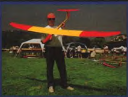
■ LEFT: Keven Anderson had a colorful sailplane that was a real eye-catcher—a Fox Models "Scorpion 100," available from Northeast Sailplane Products. You could probably guess the features: molded fiberglass fuselage with slip-on nosecone, lightweight foam core wings, SD7037 airfoil, and 100-inch wingspan. According to Keven, "It signals lift really well, practically jumping up once inside a thermal. It's pretty stable and docile." ■ RIGHT: PSS had three of these winches (paired with retrievers) with chargers set up to do the launching chores. Very few winch-related problems or slowdowns were encountered throughout the meet.
