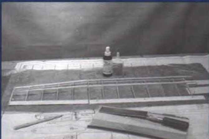
Standard balsa rib-and-spar construction is used for the Merlin's Selig 3010 airfoil wing. Rick built the inboard and outboard panels side by side to help insure good alignment.
