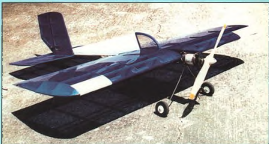
The two versions of the Electric Blues as developed by the author; the one with the yellow wingtip plates features a flat-bottom airfoil, the other has a semi-symmetrical section. Construction is so simple that it shouldn't take more than a few evenings to get one framed up and covered.
