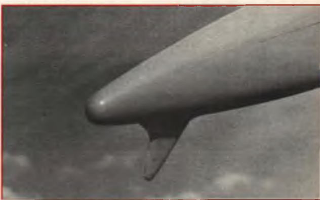
The "skullsplitter" landing skog on the author's Dove II. Does an effective job of bringing the model to a quick halt for those 100-point landing scores. After getting it sorted out, Sherman flew his Dove II in a local Seattle Area Soaring Society contest, walked away with 1st place its first time out!
