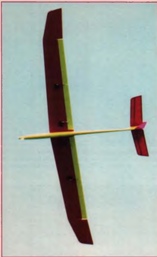
The Dove II maneuvering close to the ground. Sherman found he could pull some extremely tight maneuvers at low altitudes without fear of tip stalling.
