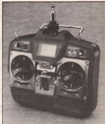
Our columnist's first experience with a computer radio (JR's six-channel XF622) was a happy one—see text for comments.
