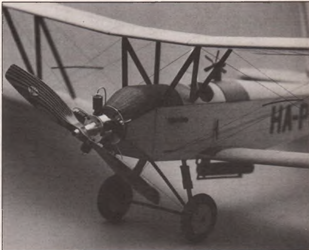
Splendid Polikarpov PO-2 "Mule" by Vladimir Vavok, is powered by a Gasparin radial CO 2 engine. Photo by Otakar Saffek, via Fritz Mueller.
