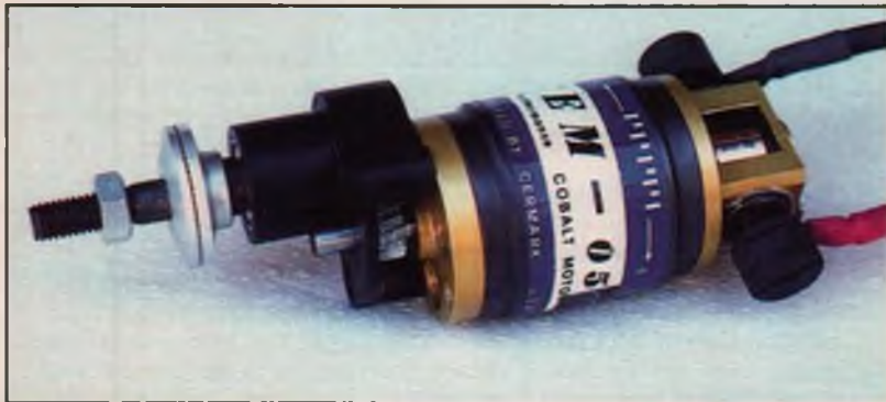
"The other cobalt motor." Cermark's powerful CEM 05 motor has been on the market for the past couple of years in a direct drive version but is now also being offered with a 2.33:1 gearbox, which is the setup Roger used in his Porterfield. The gearbox features a combined, black anodized aluminum body and helical gears. Note the cooling air openings in the motor's front end bell and the way the rear end bell is cut away to expose the brushes and commutator.
