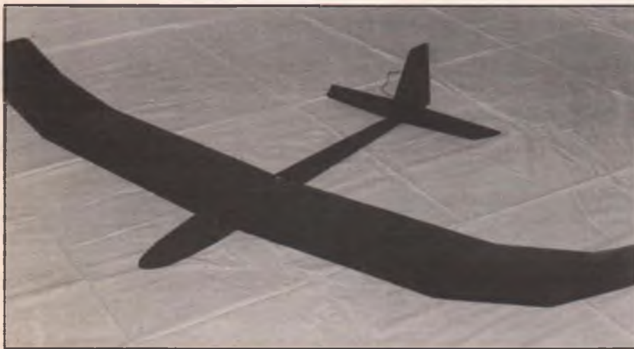
Two views of Bill Erwin's (P.O. Box 40-16, Azmarillo, TX 79118) HLG design based on columnist Bill Forrey's S4043 wing plan published in the December 1995 Model Builder . The wing was built pretty much stock except Bill also kicked up the outboard panels (last two rib bays), making a triple-dihedral wing. Standard sheet balsa fuselage and built-up tail construction. Covering is Goldberg's Ultracote Lite, which Bill really likes; interestingly, the wing was covered in just four pieces, with no splices at the dihedral breaks. Radio is Hitec's 535 FM micro receiver and HS-30 micro servos, with a 270-mAH battery. Bill says the model weighs 12 ounces and flies very well, reports several other fliers are building similar models after seeing his fly.
