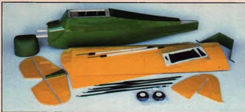
The kit contains right out of the box; not shown are the instruction manual and a small hardware bag with all of the necessary screws, clevises, hinges, horns, motor mount, etc. The fiberglass cowling is painted, but everything else comes pre-covered with Goldberg's Ultracote. Model is available in different colors—see text.
