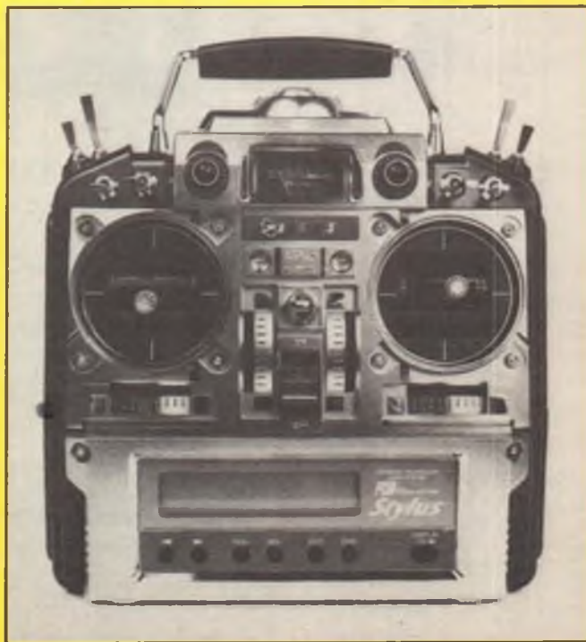
An impressive looking piece of equipment, no? There are eight toggle switches, two rotary knobs, and two trim levers, and they can be assigned by the user for any function. The only difference between the Stylus heli and airplane systems is the airborne package—transmitters are identical.
