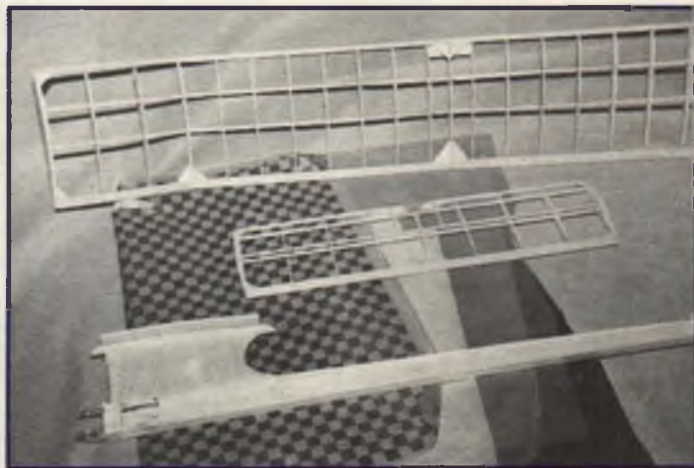
■ LEFT: The finished wing, stab and fuselage of the author's Dixie Pearl 1/2A free flight. The solid and checkered tissue on the wing and stab were adhered with gluestick and gluepen respectively; the fuselage was also covered with Japanese tissue but using Superseam and thinner. The aft section of the fuselage is covered with white tissue, the front with yellow. Trim strips and lettering are cut from black tissue, glued in place. ■ RIGHT: The sanded, ready-to-cover Dixie Pearl framework lying on top of the various colors of Japanese tissue to be used for the covering. Shown are checkerboard, white, yellow and black tissues.
