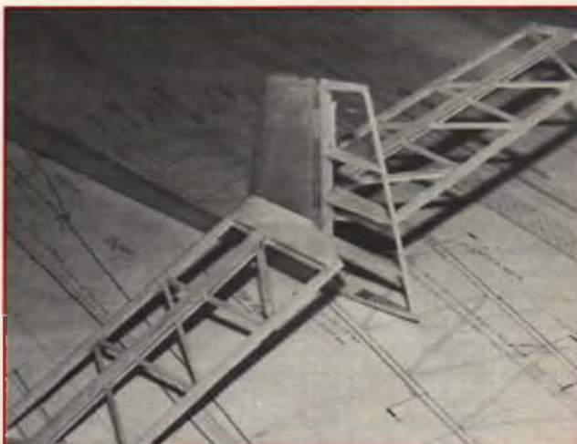
Tail surfaces look pretty lightly built, but Sherman built them according to plan and has yet to damage one in the air despite some lead-footed "gorilla" launches.
