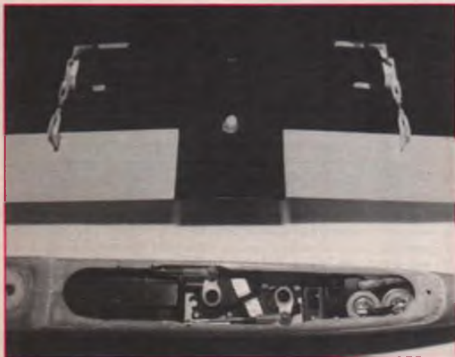
LEFT: Radio compartment is tight, but the receiver, two servos, switch, charging jack and 600-mAH NiCd pack all fit in front of the wing. The author ultimately had to remove the case from the receiver to get the CG right on. RIGHT: Close-up of the gear setups on the JR 341 (left) and new 351 metal-gear micro servos. On his Dove II, Sherman is using the 351s for the flaps and 341s for everything else. See text for his comments.
