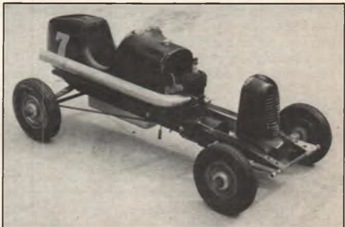
Model race cars were extremely popular during the 1935-40 era. Several companies produced both engines and bodies. Irwin Ohlsson and his early partner, Frank Bertelli, built this one-of-a-kind racer; balsa body was carved and finished in high-gloss enamel. Ohlsson made the engine, frame and running gear. Engine was an early "step fin" Ohlsson Miniature.
