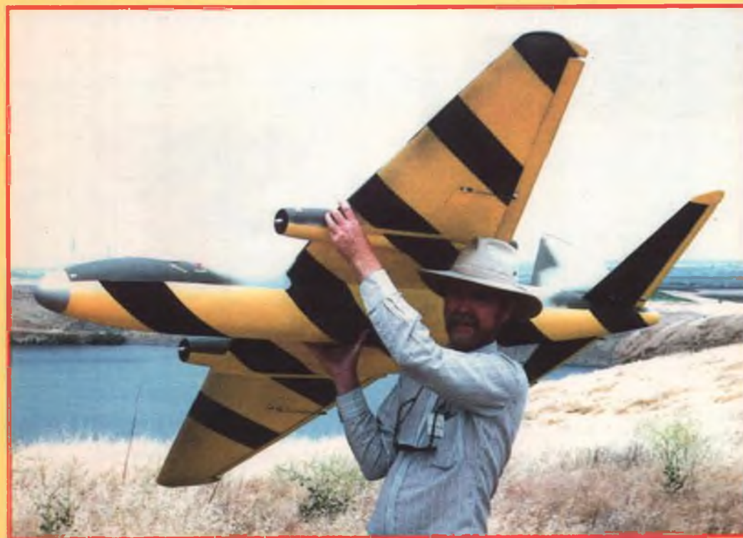
Most of the Los Banos regulars favor large PSS models; here's Lynsel Miller with his 1/10-scale Canberra bomber. Model was scratch built from foam and fiberglass, while the hardwood engine nacelles were turned on a lathe.
