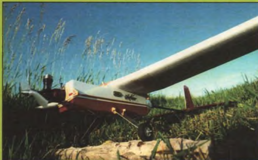
This ground-level close-up clearly shows the Grasshopper's rubber-band-together assembly. Dave used MonoKote on the fuselage pod and tail surfaces. Pod could also be painted with K&B Super Pozzy for a durable, totally fuelproof finish.
