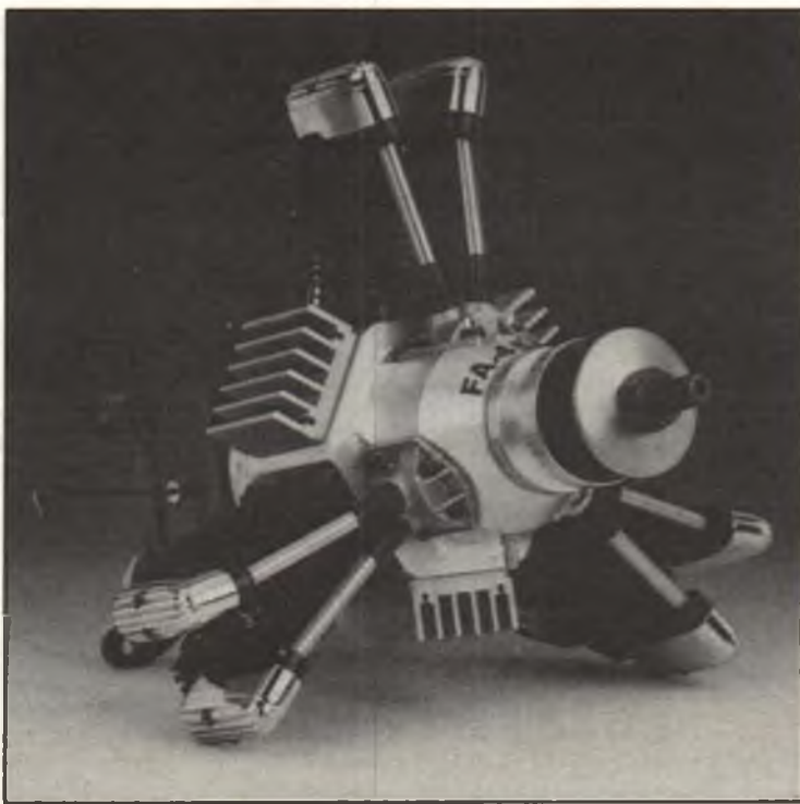
Horizon Hobby Distributors has Saito's latest and biggest four-stroke engine available for the Big Bird enthusiast. The new FA-450 three-cylinder radial displaces a whopping 4.5 cubic inches and will turn a Boly 22x18 propeller at 8,000 rpm using 15 percent nitro PowerMaster two-stroke fuel.
