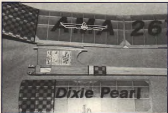
■ LEFT: The finished wing, stab and fuselage of the author's Dixie Pearl 1/2A free flight. The solid and checkered tissue on the wing and stab were adhered with gluestick and gluepen respectively; the fuselage was also covered with Japanese tissue but using Superseam and thinner. The aft section of the fuselage is covered with white tissue, the front with yellow. Trim strips and lettering are cut from black tissue, glued in place. ■ RIGHT: The sanded, ready-to-cover Dixie Pearl framework lying on top of the various colors of Japanese tissue to be used for the covering. Shown are checkerboard, white, yellow and black tissues.
