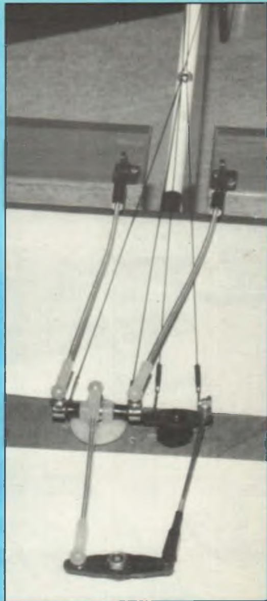
View of the bottom of the wing reveals the ingenious linkage setup that provides coupled ailerons and rudder and coupled elevator and flapons, using only two mini servos. Pull-pull cables are used for the rudder and elevator. The elevator/flapone coupling can be deleted by omitting the turnaround ballcrank and the De-Bro mechanical mixer. Both control systems are detailed on the plans.
