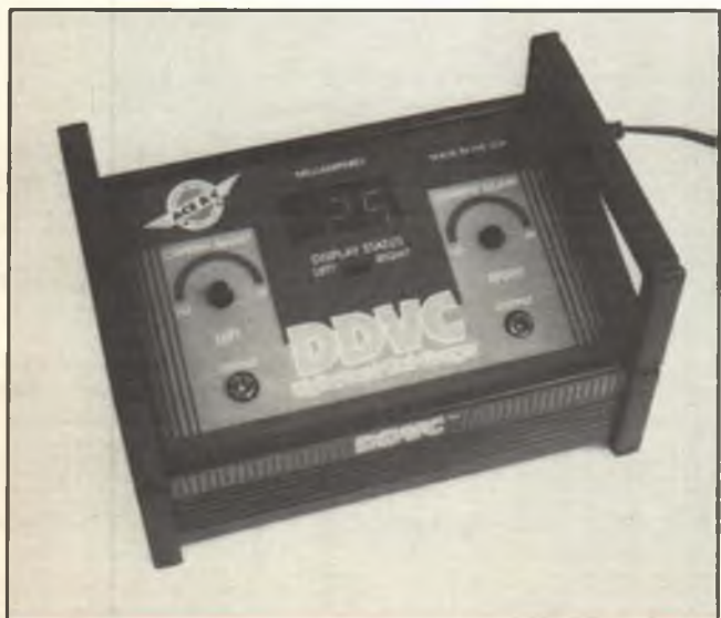
■ LEFT: Ace's DDVC (Digital Dual Vari-Charger), either AC or 12VDC powered, can be used to charge two one- to ten-cell batteries at up to 500 mA; charge rate is displayed digitally. ■ RIGHT: The insides of the DDVC are significant in that they show how well designed and constructed this new equipment is—all modern components and circuitry are used throughout.
