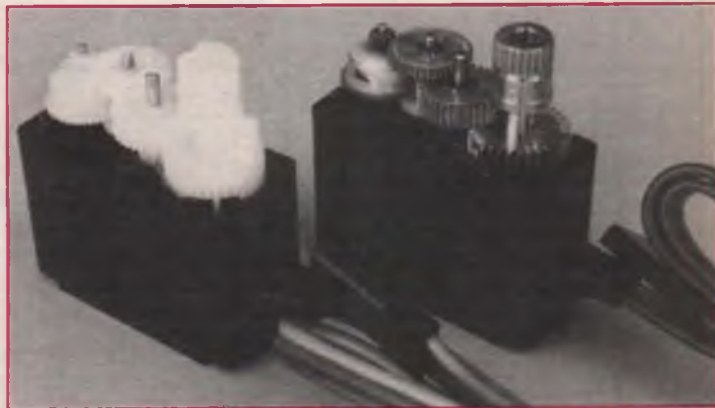
LEFT: Radio compartment is tight, but the receiver, two servos, switch, charging jack and 600-mAH NiCd pack all fit in front of the wing. The author ultimately had to remove the case from the receiver to get the CG right on. RIGHT: Close-up of the gear setups on the JR 341 (left) and new 351 metal-gear micro servos. On his Dove II, Sherman is using the 351s for the flaps and 341s for everything else. See text for his comments.
