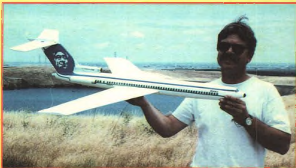
Here's something neat and interesting for a PSS subject: Brian Just built this Boeing 727 with Alaska Airlines fleet markings. The fuselage was built with formers and stringers, then wrapped with 1/84 plywood sheeting. No problems with tailheaviness on this bird!
