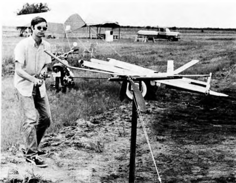
Charlie Learoyd with stooge. Note winding tube in body to protect it from possible breaking motor. Canopies give away windy condition.
