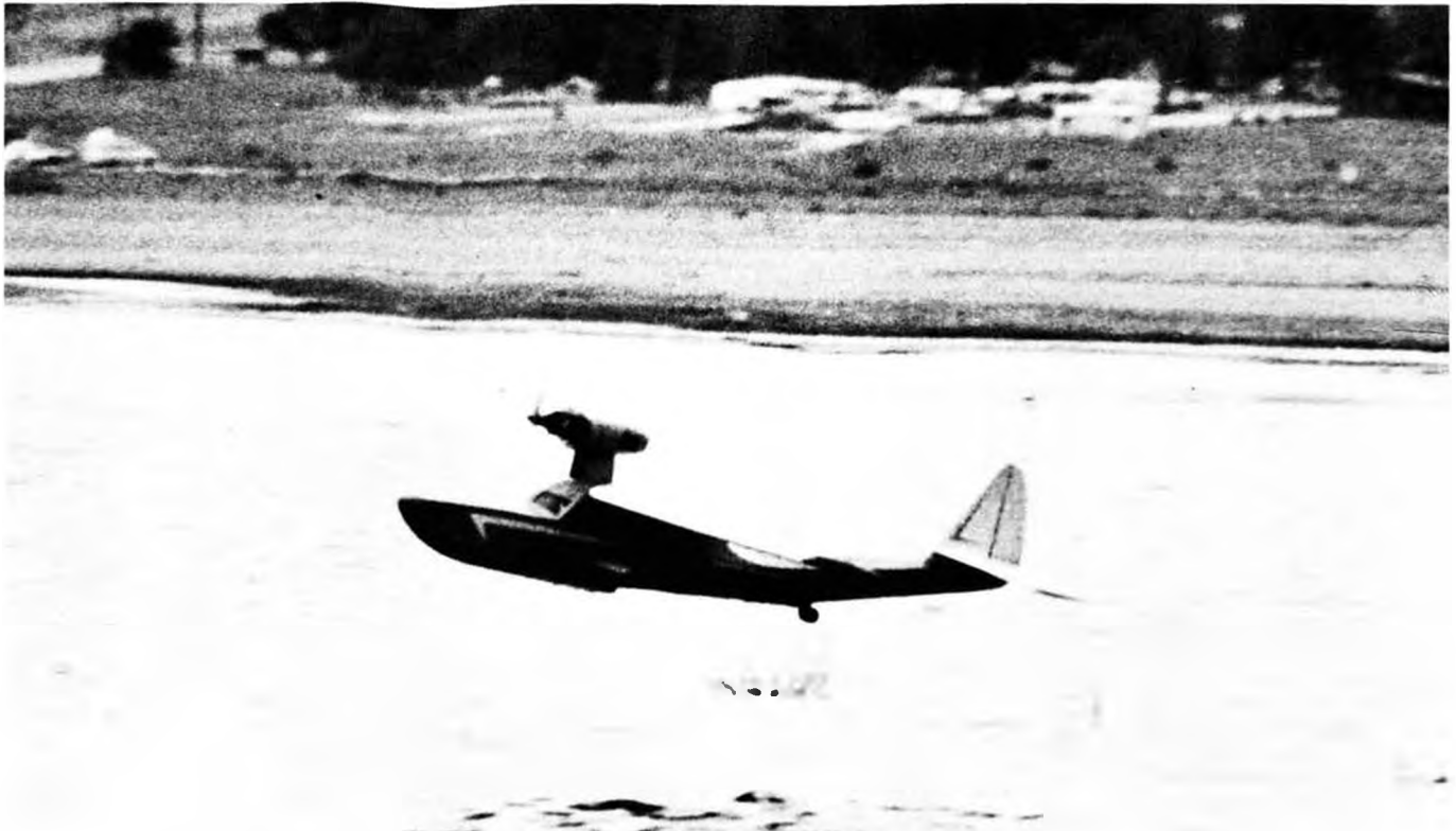
The "Elsinore Garbage Scow" is really a pretty flying boat, and it convincingly refutes the popular belief that in order to get off the water, a model must be overpowered. The ship weighs 12 pounds, has a seven foot span, and the engine is an Enya 60!
