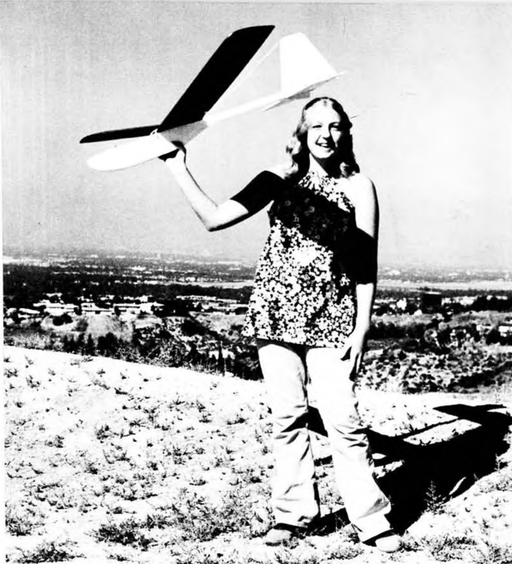
This glider has a dark green wing and bright white fuselage. When viewed through an amber polarized filter, the fuselage is much brighter than the darkened sky and the wing looks black. It's a highly visible combination. The author's daughter, Julie Ann, holding.
