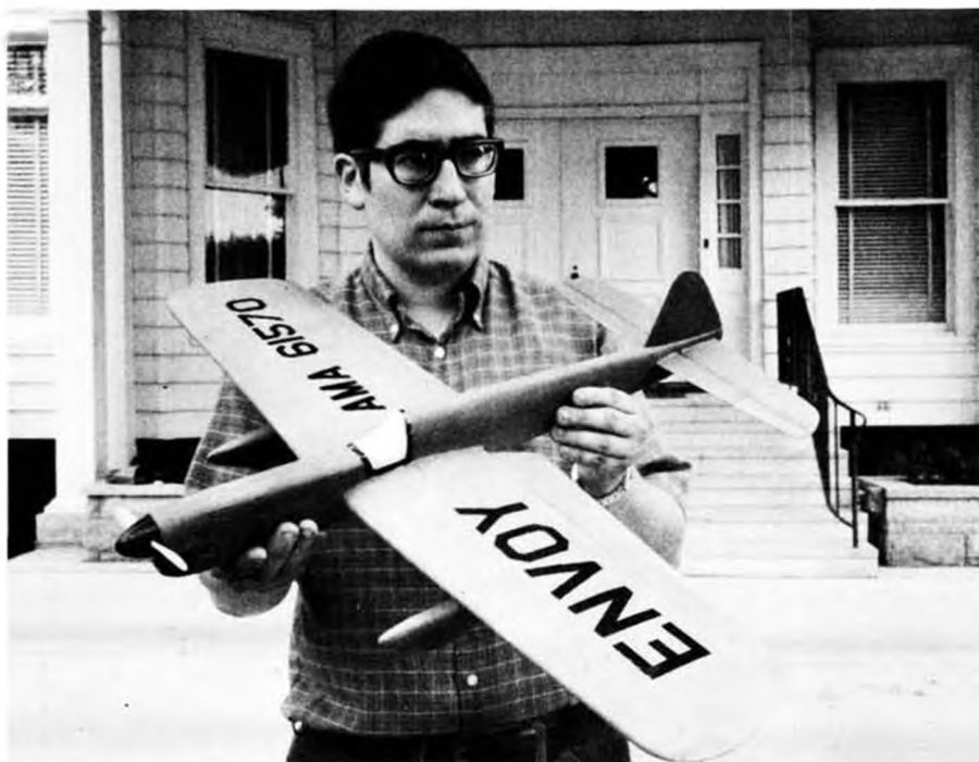
Steve Stumpf, Pana, Ill., and his 1/2A stunter flown on 45 foot lines. Cox Tee-Dee power, 6-3 prop, Tenny tank. Design is reduced Envoy from MAN plans. Next he'll do Sirotkin's stunter.
