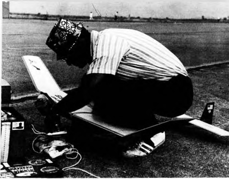
Roger Simpson's power ship shows German FAI influence. Sheeted wing built on full-span jig, with dihedral and warps all included.
