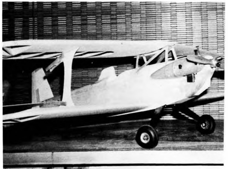
This view shows some of the construction and assembly techniques employed in creating the Toot. Note simple top wing attachment.
