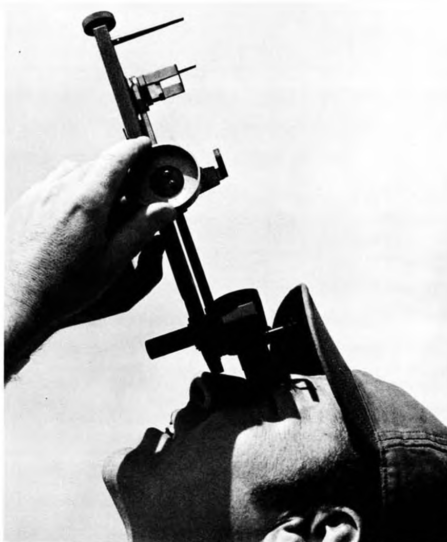
John Ferrer demonstrates the way to use a stadiometer. It provides a fairly accurate measurement of your plane's altitude. R/C soarers, please note! Read all about it in this free flight column.
