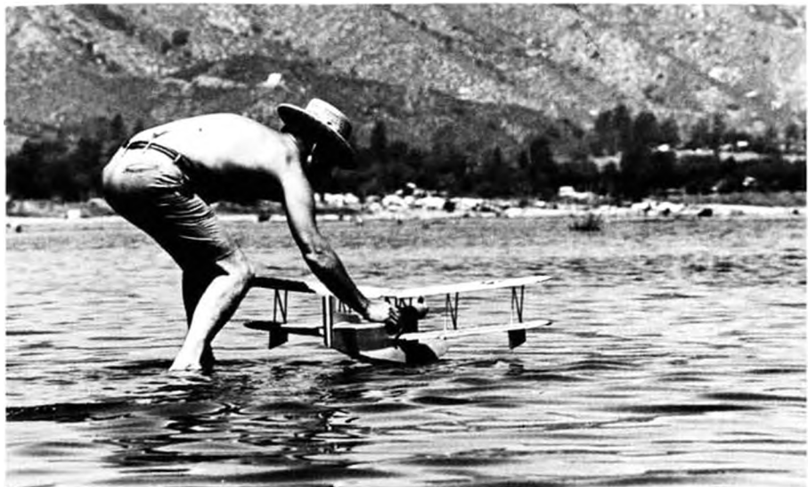
Jim Adams, Santa Ana, California, launches his free flight Loening OL-9, built from Aeromodeller plans. Span is 48 inches, and power is a 1cc (.06 cu. in.) Taifun diesel.
