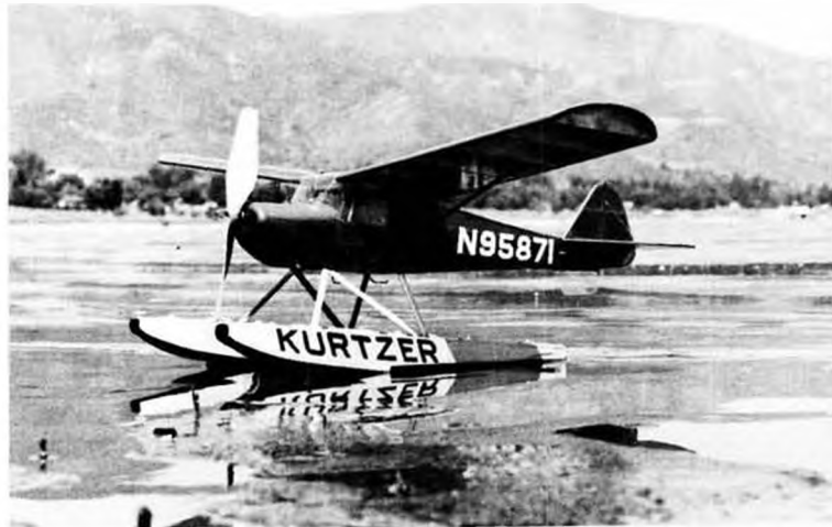
Walt Mooney's 24 inch Taylorcraft featured in last month's center-spread. Note clear plastic sub-fin required for stability.
