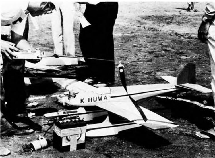
Eventual winning plane in this particular contest is fairly conventional set-up. Note water rudder connected to air rudder. Like Seahorse.
