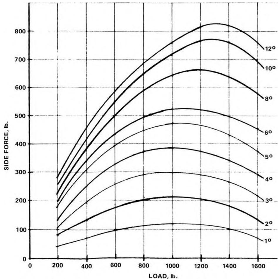
Fig. 3. For a given slip angle, a tire's cornering ability increases with the weight on it, but not in direct proportion; it peaks and falls off with further loading.
