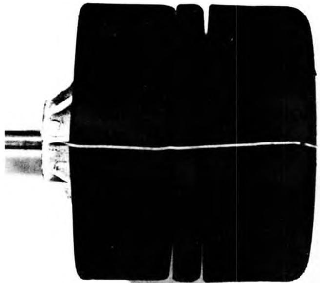
Fig. 7. Slip angle of a rear tire is pretty large, but some lightly loaded parts of the tire are sliding.
