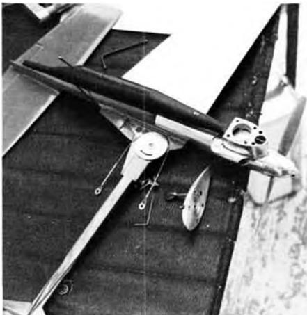
Dick Hall's engine with head removed. Note neat bellcrank system. Fine workmanship.
