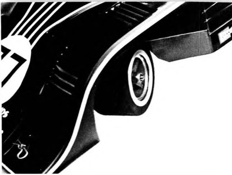
Fig. 4. Wide front tires can be used on sports cars because of the fantastic rear tire bite.
