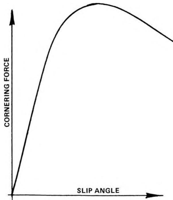
Fig. 2. Cornering capability of a tire increases with slip angle, reaches a peak and drops off . . . breaks away.
