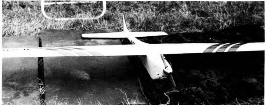
Vern Smith's FAI ship with homemade engine. It was fastest plane next to Violett's Bobcat. It crashed during qualifications when rain water got in the transmitter.
