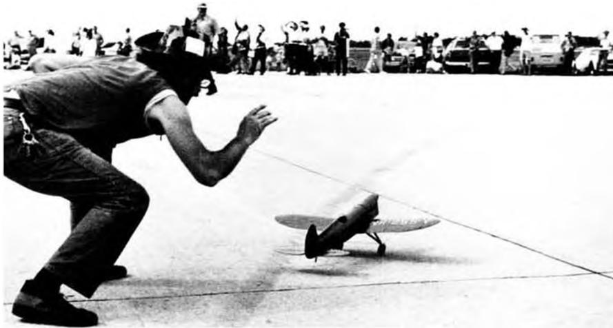
Engine running at last, Bill Warner's Brown Racer begins takeoff. For added stability in flight, Bill rigged the wings so that they pivot into extra dihedral under flight loads. Cleverrrr!
