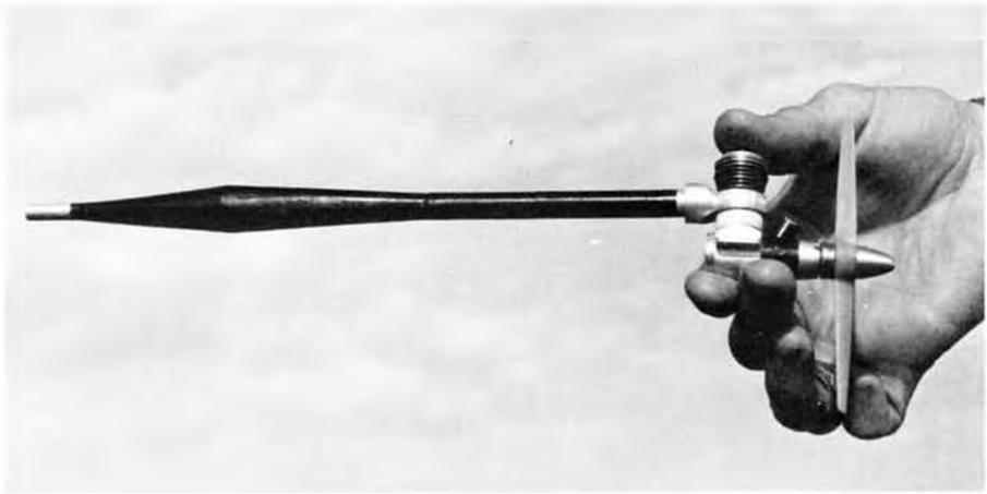
John Shannon's modified Tee Dee .049 with tuned exhaust. Homemade prop is 4-1/8 Dia. by 6 inch pitch.
