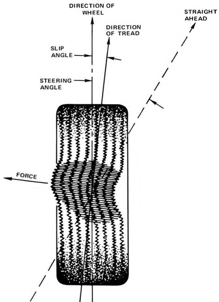
Fig. 1. Defining the concept of slip angle; the departure of a tire's direction of travel from the way it is pointing.
