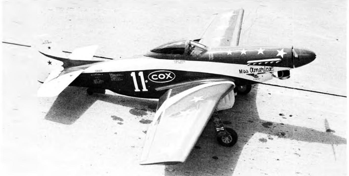
Beautiful scratch-built model of Howie Keefe's Cox sponsored P-51 unlimited racer, by Ron Norgard, Davenport, Iowa. Has operating flaps and canopy, retractible landing gear, and throttle control. Max .80 powered ship placed 4th in Open Scale.
