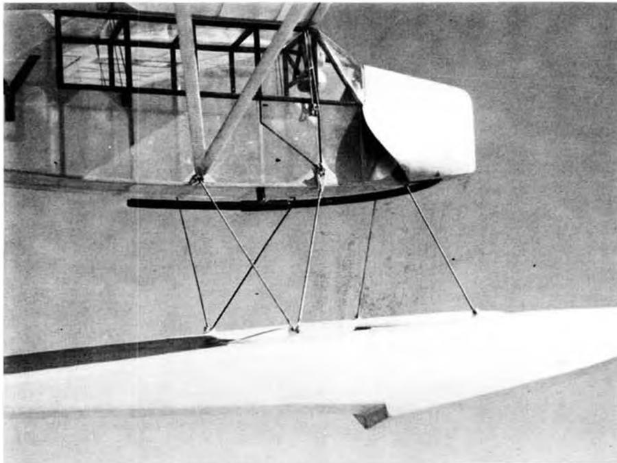
Plug-in landing gear struts makes it a simple task to switch from R.O.G. to R.O.W. Ship lifts off water in about 5 to 7 feet. Floats are 1/32 sheet balsa covered, very light.
