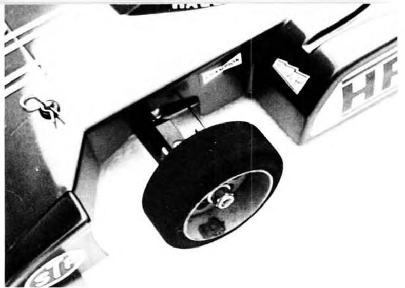
Fig. 5. The rear tire bite of Formula cars is less than the sports cars, so front bite is decreased by using narrower tires.
