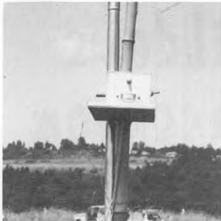
Photos of Jon Fink's thermal detector at top of pole, and meter box at the bottom.
