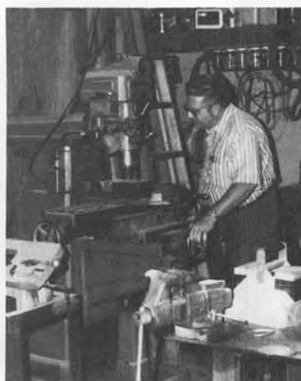
Charley operates his vertical milling machine. Power hacksaw barely visible at left.
