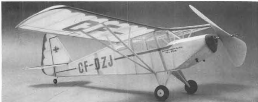
Fred Hall's Fleet Canuck, 16 inch span indoor model, does over 80 seconds R.O.G. Placed second in M.I.T. contest.
