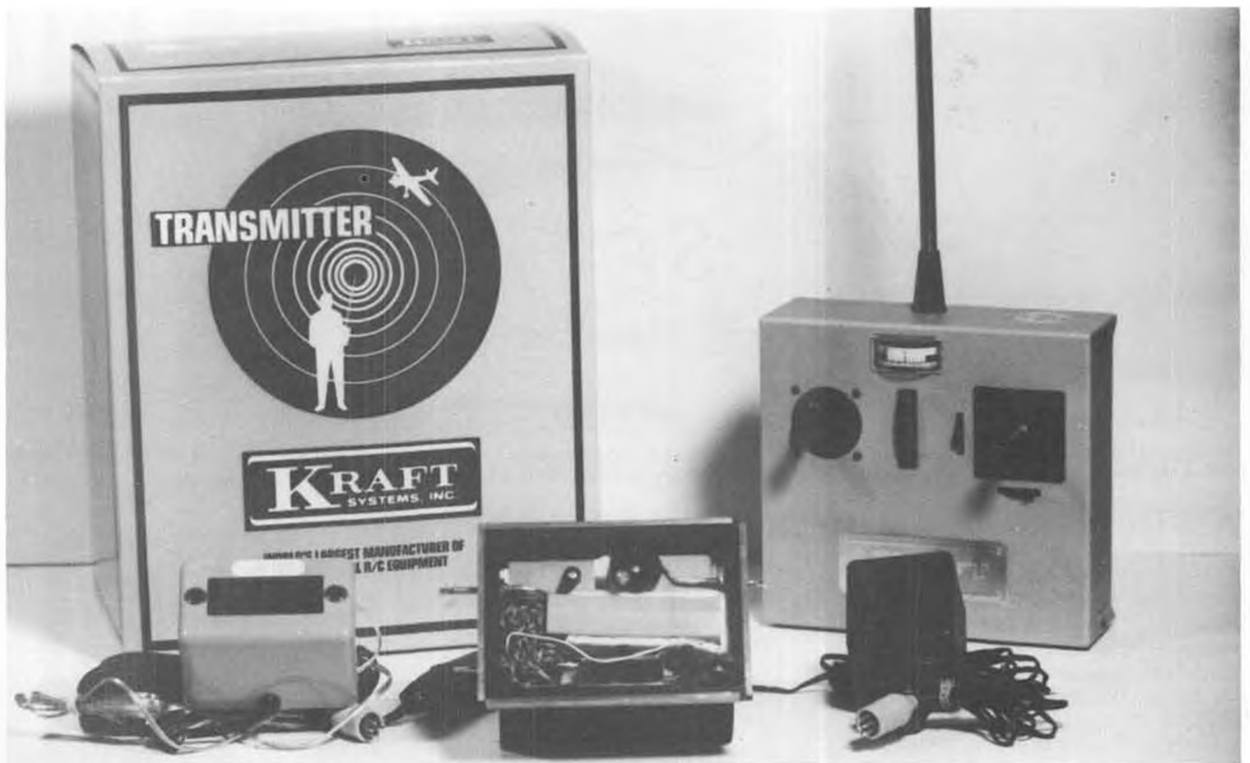
Kraft KP-3C transmitter, with 120V. charger in front, the G&M waterproof radio box with Kraft receiver, servos, and battery pack inside, and the Kraft KBC-A charger, for use with a 12-volt car system through the cigarette lighter socket.
