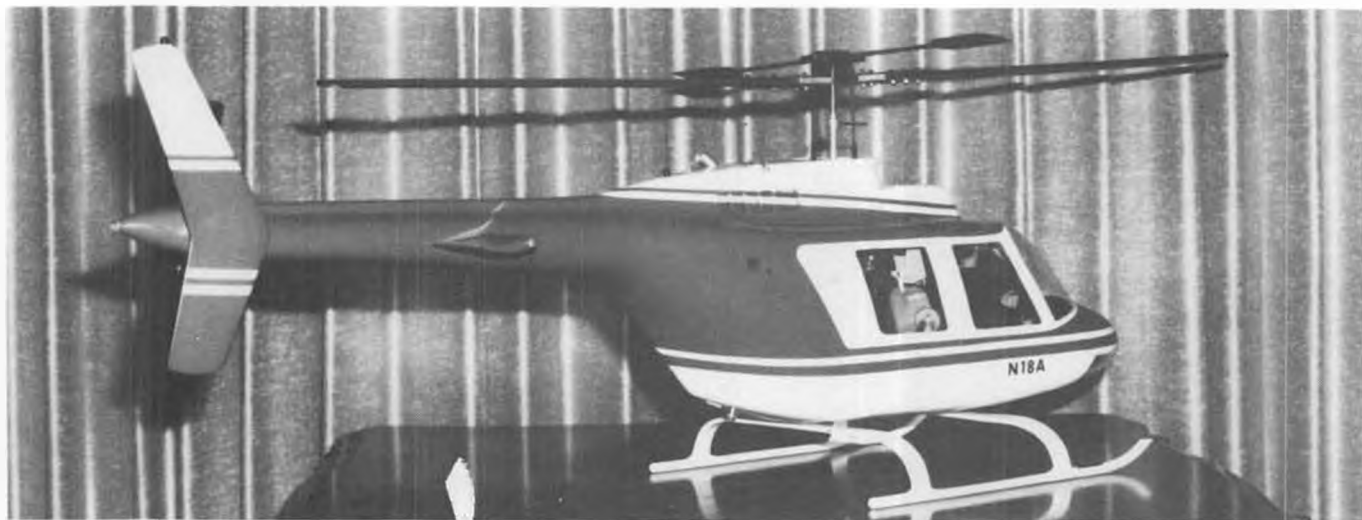
Charley Gilbert's "Baby Ranger". Glass body, vacuum-formed windows. Adapts to Heli-Baby, Revolution, or Alouette mechanics.
