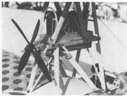
Close-up of the engine mounting in Tschirgi's (say "Shirgi") plane. That's the flying prop!
