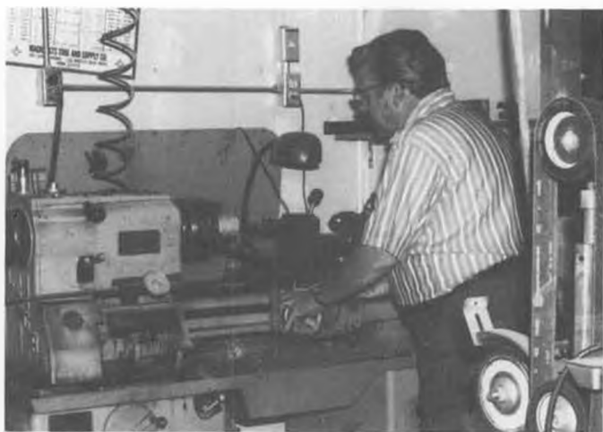
Charlie at the console of his Logan lathe. Belt sander/grinder is the latest thing for sharpening tools, etc., better than grinding wheel.
