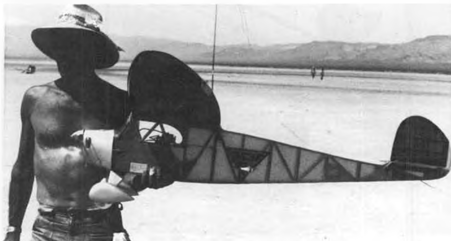
Slick SCIF builder, Phil McCary, and his "gussied" up Comet Clipper. Note gravity trim tab on left wing trailing edge. Streamlines during power burst, then drags wing in glide.
