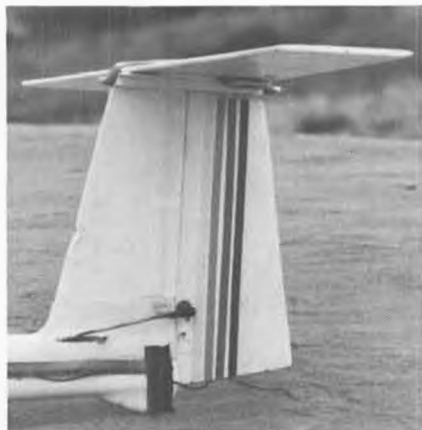
The tail on this Keil Kraft Ivory Gull, built by Ben Watson, has a horizontal pivot for pitch control . . . the whole thing moves as a unit . . . fin, rudder, stab, and all. The rudder is turned by a ball-joint, and there is no interaction between the two. Just one question . . . What's the advantage?
