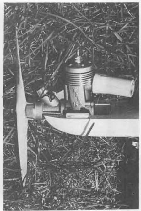
Front end of Howard Rush's long-nosed plane. Pipe gets exhaust clear of wing. Bartels prop.
