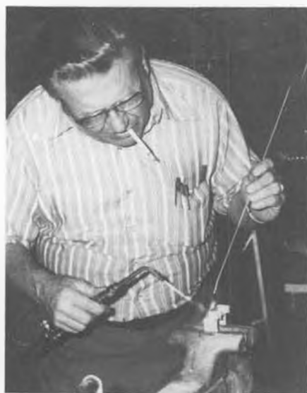
Demonstrating new aluminum brazing rod, for home shop use. Low heat required. See text.
