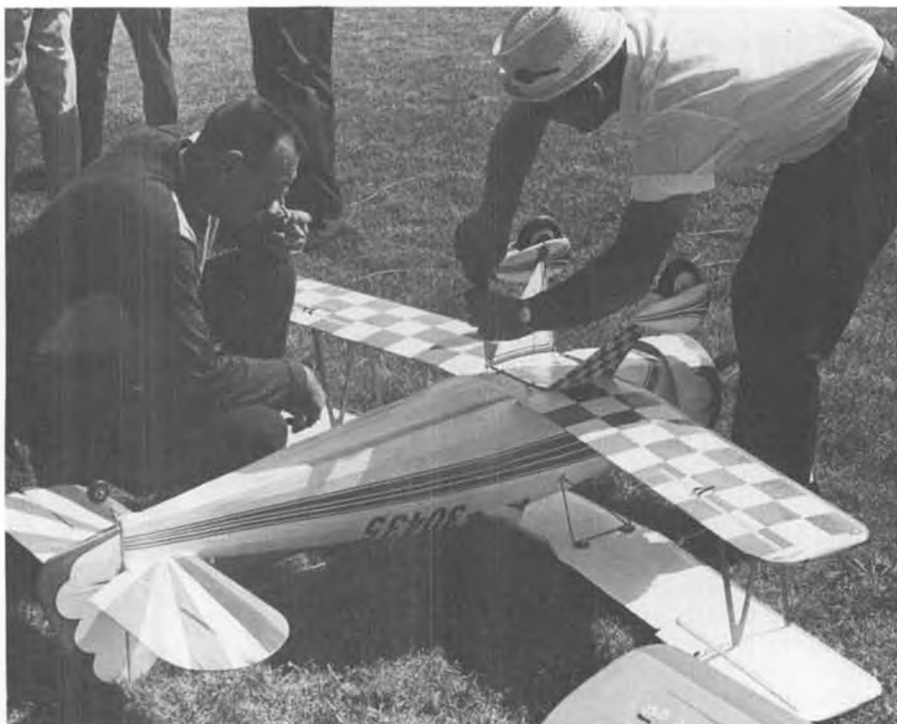
Ray Nugen snugs down the nylon wing bolts. Photo gives an idea of the size of this biggie. If you don't fly from a grass field, you better make a rack to hold fuselage during assembly.
