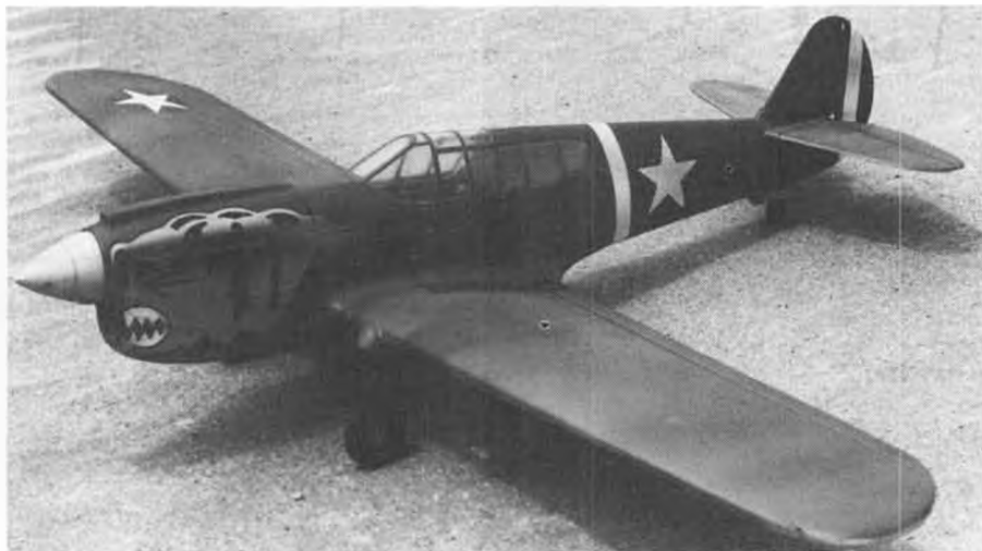
Model Merchant's newest, the P-40. Construction is similar to the Rickey Rat, and also features retract, which fold and rotate, just like the real ones.
