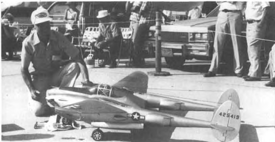
Art Johnson and his remarkable P-38. Built entirely of balsa and hardwoods, it is scheduled to be a future Model Builder construction article. Very realistic in the air; scale speed and sound.
