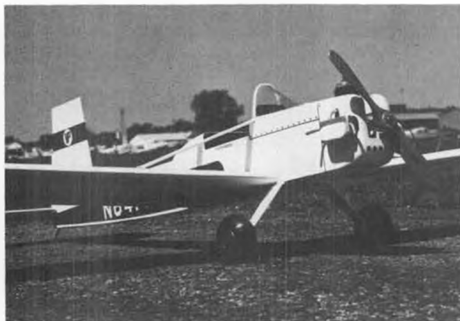
Ancient Cub .14 was used in original model. Though a modern .09 or .10 would do, a .15 would give livelier performance.
