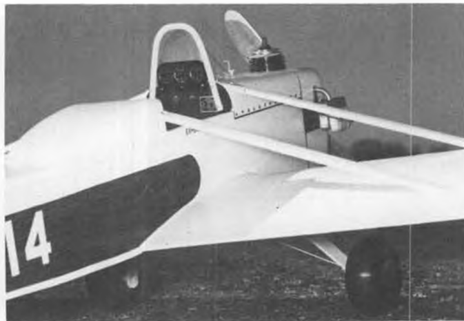
Contact shelf paper simulates natural finished plywood sides. Seal edges with epoxy. Plans could be used for R/C version, as is or larger.
