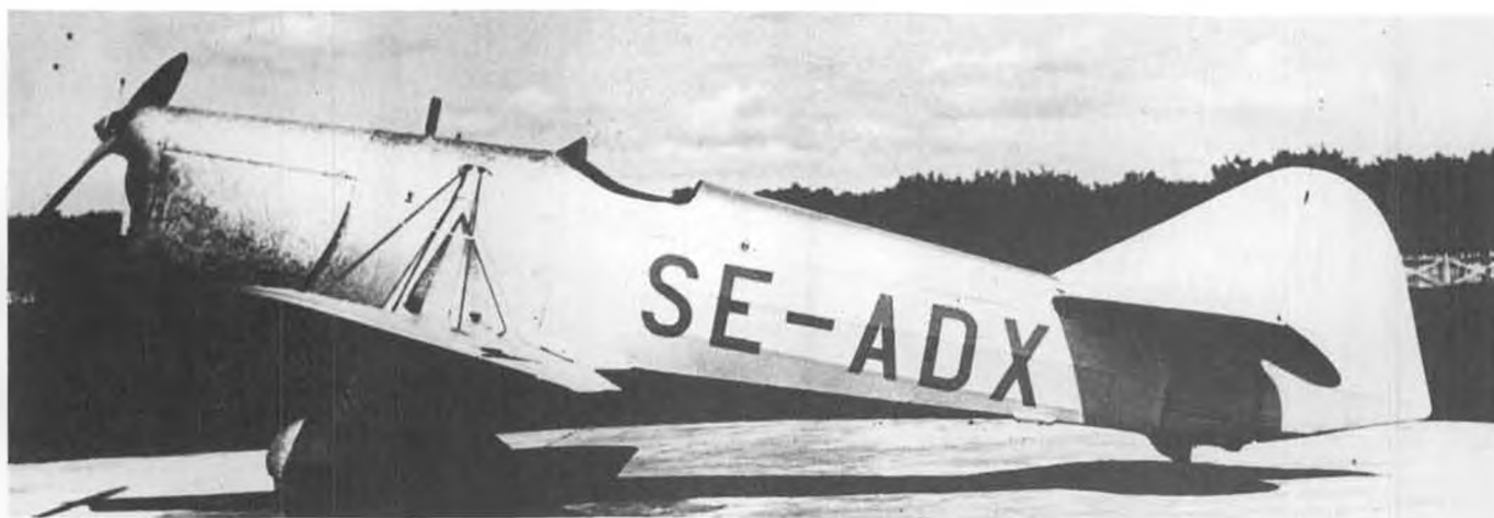
The original P-1 had a civil registration and was called the S1. It had rounded wingtips, and no headrest. Before this photo was taken, the rudder outline had been changed from a lozenge shape (rounded). Finish on aluminum work was damscened to hide hammer marks.
