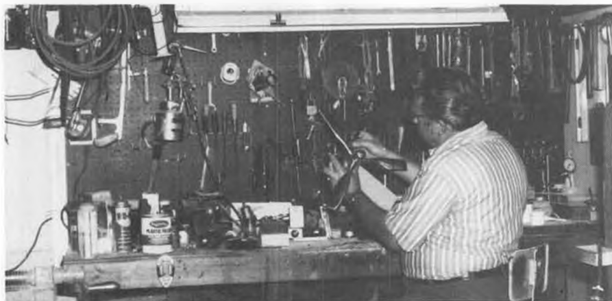
Charley, at his main workbench, working on his adjustable pitch, three-bladed aluminum prop.
