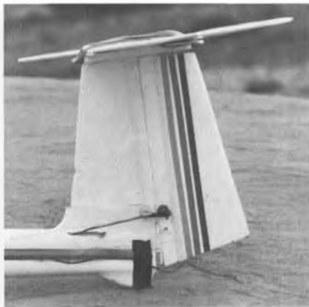
The tail on this Keil Kraft Ivory Gull, built by Ben Watson, has a horizontal pivot for pitch control . . . the whole thing moves as a unit . . . fin, rudder, stab, and all. The rudder is turned by a ball-joint, and there is no interaction between the two. Just one question . . . What's the advantage?
