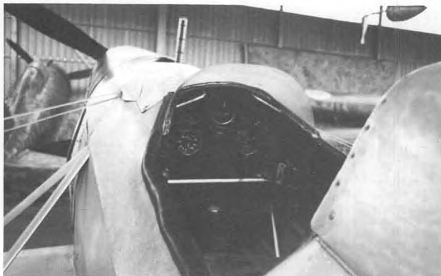
Cockpit shot reveals two handholds below windshield, slides for map board just below instrument panel, standard instruments. Cylindrical object ahead of windshield is fuel gauge.
