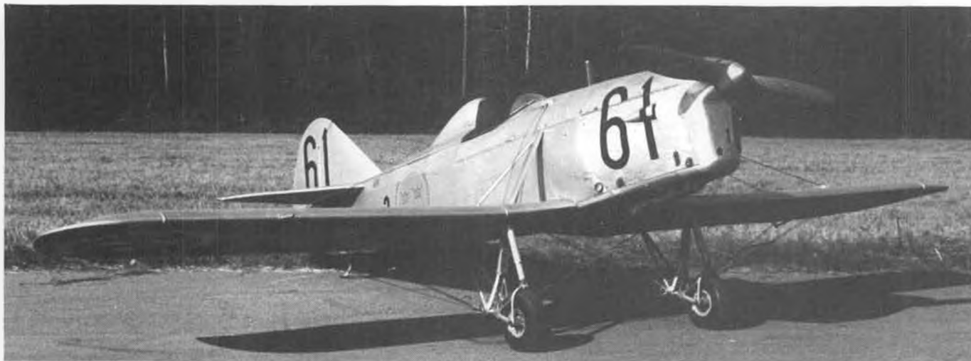
Photo of the only still-existing P-1, which, unfortunately, has no wheel pants. Original fairing consisted of a sprung portion which telescoped into the fixed upper streamlines.
