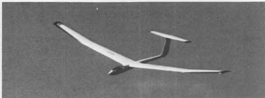
In addition to his "Nonstop," Bob Groves also flies this nicely finished Sea Breeze from Bob Smith R/C Aircraft. Ship is of all-fiberglass construction, spans 99-3/4 in.
