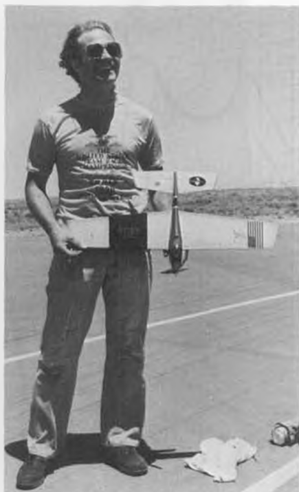
Dave Elledge of Glasswerks fame, with Team Racer at U.S. T/R Champs. Plane is Dave's design with multi-piece epoxyglass shell, Nelson AAC power, John Gray prop. Pic by Whipper (Flipper's husband).
