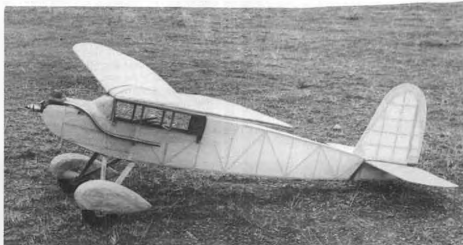
Photo No. 10. Gordon Coddling is at it again! One of his most recent customized O.T.'s is this Miss America, complete with wheel pants molded from brown paper tape!
