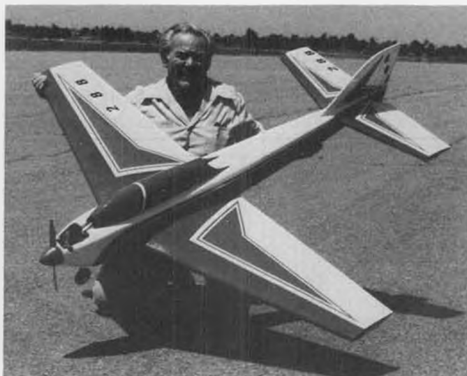
Joe Bridi's latest pattern ship is this biggie which spans 65 inches with 975 sq. in. wing area. It's 70-1/2 inches long, weighs 11 - 2.
