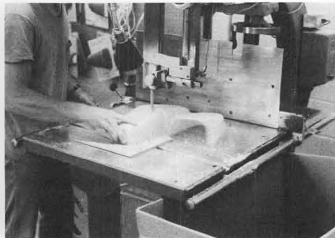
Here's a mold guide in use, cutting two halves of the Bonanza cowl. Many types of clever gimmicks like this speed up production.
