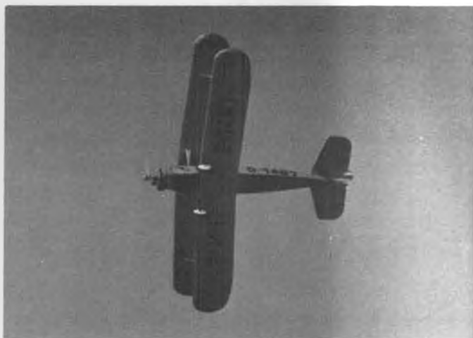
In flight the Flamingo handles as easy as anything. Total wing area of 900 sq. in. and 5-1/2 lb. flying weight put it almost into the trainer class. K&B .40 has more than enough power . . . proportionately more than the real ship with its 100 horsepower.
