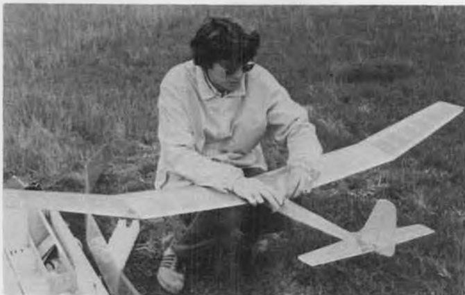
A potent handlaunch machine is this modified Drifter II by Peter Esherick. Mods include narrowing the fuselage and putting the wing hold-down dowels inside. Drag reduction important!
