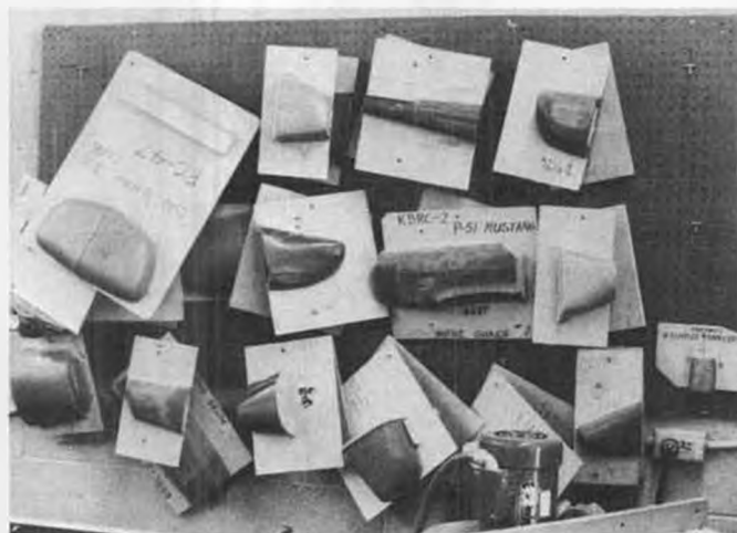
These heavy molds serve as saw-guides when the plastic molded parts are trimmed to size. Sig kits don't leave this job to you!
