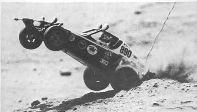
Excellent body painting and detailing work was done by Frank Killam. Body shell is molded from styrene plastic, same as a plastic display model. Decals are pressure-sensitive.
