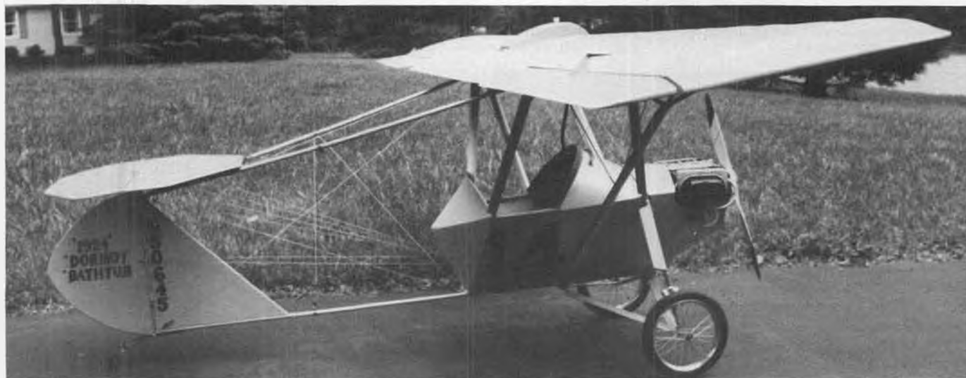
Hank Iltzsch, Seekonk, Mass., designed and built this 4" = 1' scale 1924 Dormoy Bathtub, based on Mike Kimbrel's plane which appeared in the Sept. '77 Sport Aviation . Span 8 ft., 12 lbs.
