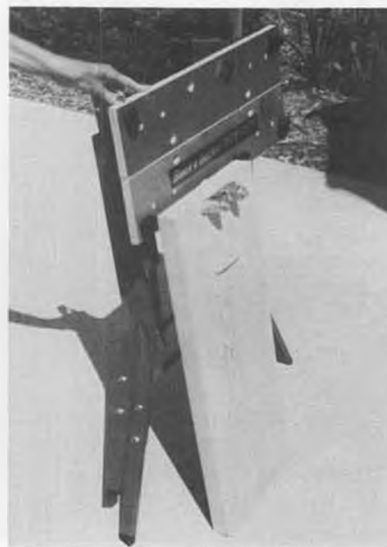
Workmate folds up for easy, convenient storage and transportation.
