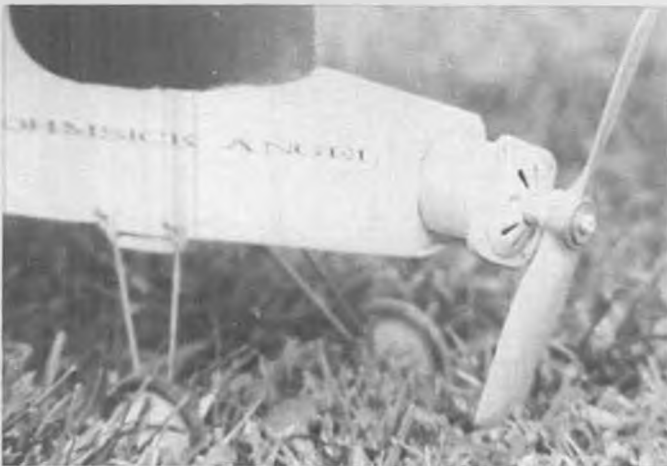
Astro 020 motor is a tight fit in a 1/64 ply tube, held in place by four screws. Quickly removed if necessary.
