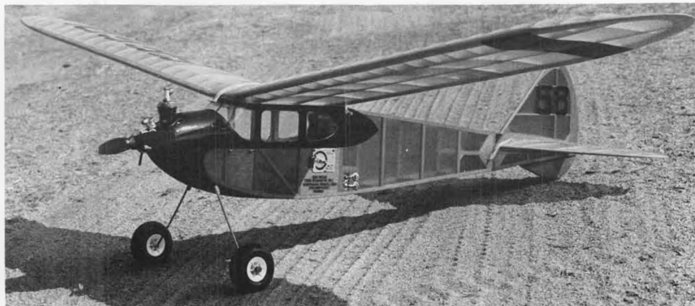
Photo No. 3. Bob Oslan did one of his usual superb building jobs on this Pete Bowers "Fly Baby," which held the 1941 Hydro record. Covered in silk and dope, of course, and equipped with a Cox Tee Dee .09 with 77 Products ignition conversion.
