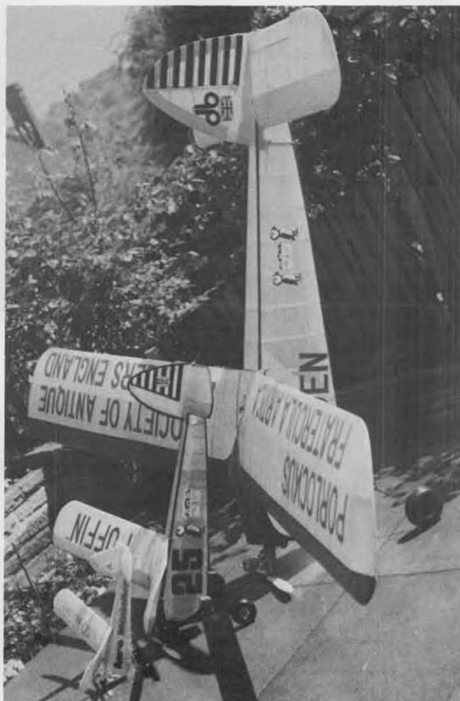
Photo No. 7. Not content with one Porlock Puffin, England's Dave Baker built three! Little one is F/F, middle one is single-channel R/C, and the biggie has three channels.
