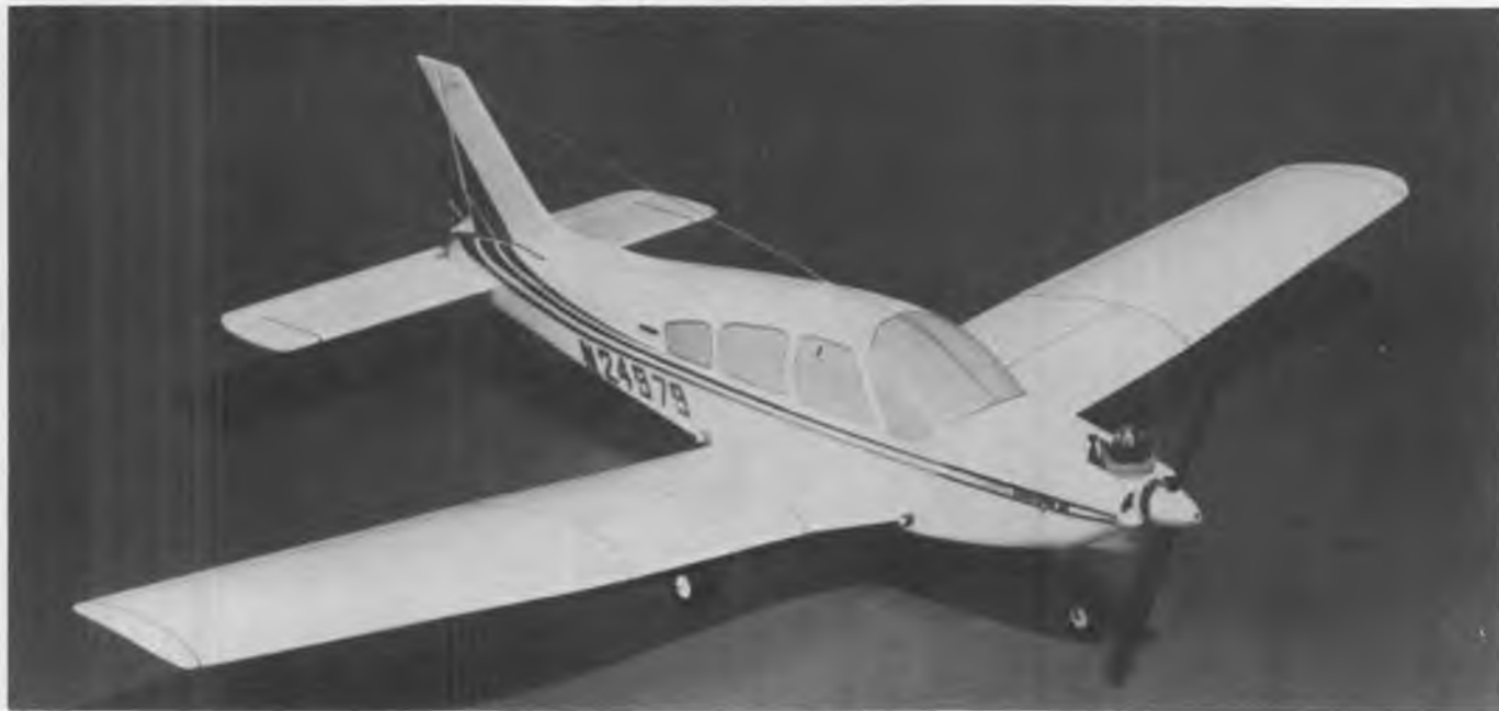
Cox has two new ARF 1/2A low-wingers, one of which is this Piper Arrow with rudder/elevator/throttle controls. Construction is foam and plastic. Engine is the relatively new R/C Bee .049, with oversize fuel tank and clunk pick-up for positive fuel flow when doing aerobatics.
