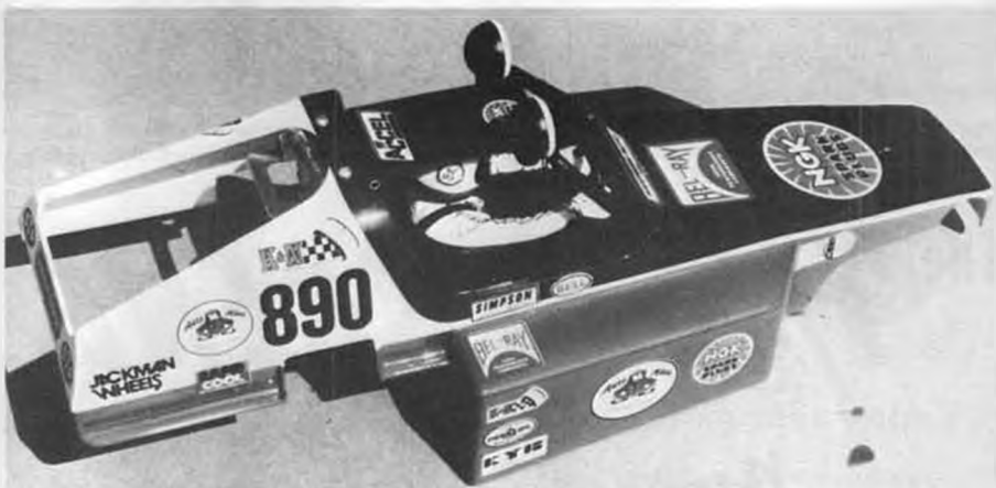
Excellent body painting and detailing work was done by Frank Killam. Body shell is molded from styrene plastic, same as a plastic display model. Decals are pressure-sensitive.
