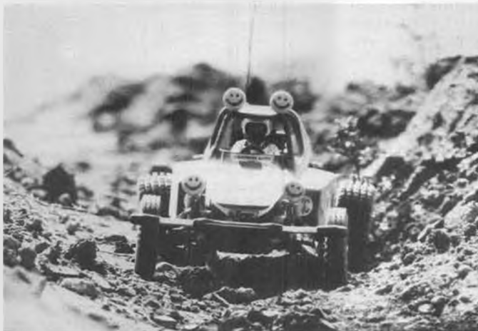
Excellent body painting and detailing work was done by Frank Killam. Body shell is molded from styrene plastic, same as a plastic display model. Decals are pressure-sensitive.
