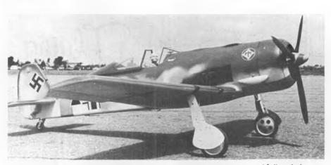
Ted Hyde's quarter-scale FW-190A features sliding canopy, original pilot, and full cockpit. Landing gear is non-retracting. Span 8-1/2 ft., weight 31 pounds. Needs more than Quadra.
