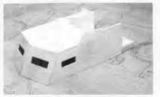
Front cabin top and front pieces glued in place. Windows cut parallel to roof line.
