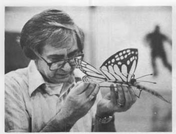
Our Indoor columnist attaching rubber to rear hook on Butterfly One (page 67). Motor length controls performance, Sunderland pic.
