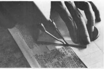
2. Cutting part of filler tube opening. Piece of wood holds pattern and also guides movement of soldering gun.
