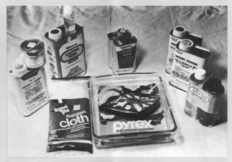
Pyrex potting dish, fiberglass cloth, and various epoxy/casting resins that can be used to construct this easily-made transmitter solar cell charger.
