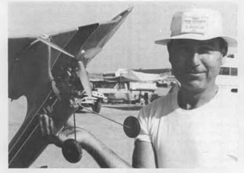
14. Don Rasmussen uses three 3-bladed prop to ensure adequate ground clearance. Thrust just as good as with two-blader.
