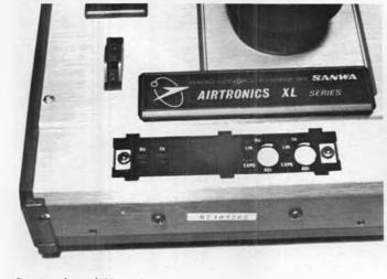
Panel on face of Airtronics transmitter conceals switches and adjustments. More information in text.
