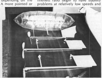
By using a detachable motor stick, various configurations can be tested using same bag.
