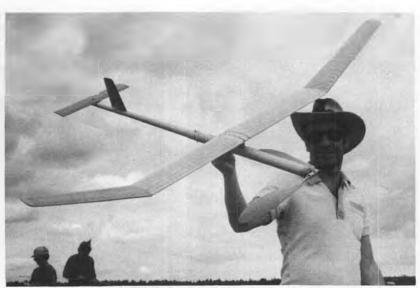
Norm Beattie's new Wakefield uses Kevlar motor tube constructed in manner described in text. Tube is light, and really bullet-proof.
