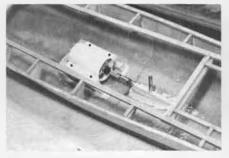
Astro 25 lined up with shaft before epoxying mount. Vertical extension for lubricating.
