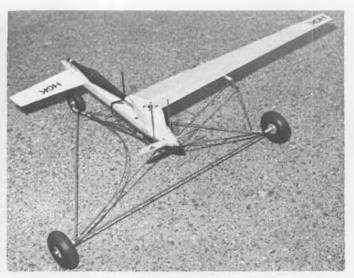
Another Steve DeBord model, flown in AMA "A" speed; 78% nitro, Newton metal wing, and Rumpel type body and tail. 'Case you hadn't noticed, power is HGK.
