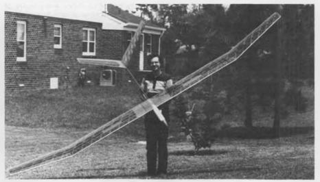
Tony also builds HTA (Heavier Than Air) models. The Eclipse was featured in Oct '74 American Modeler. Span 15 feet, weight 7 lbs, 2 oz. Red transparent MonoKote covering.
