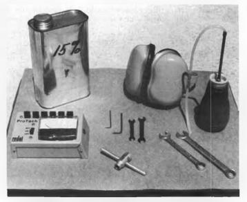
Tools of the trade for running in. Hearing protection most important. Hearing damage is accumulative. Have good tach, clean fuel, and tools.
