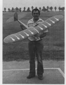
Roland Boucher with his 67-inch Playboy powered by Leisure 05 motor; speed reducer, six 600 mah Sanyo batteries, 32 oz. weight.
