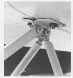
Holes were drilled in bolt ends to safety-wire wing mounting nuts. Strut-end bolts and nuts are fixed permanently to brackets.
