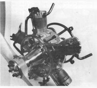
Engine is built from highly successful O.S. 4-cycle 60 units. Intake manifold collector ring design still being optimized.
