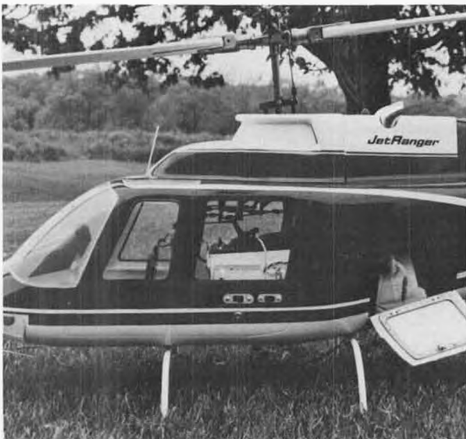
Another Dick Hausfeld project, this Kavan Jet Ranger, with modified scale landing gear, antennas, and baggage door.
