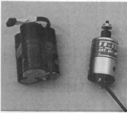
Astro 035 will give 12,500 on a 6x3, 14,500 on a 5-1/4x3. With six .550 cells, weighs 26 oz.
