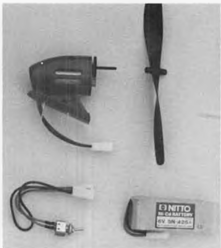
Power unit for Airtronics "Kitty". Geared Mabuchi, 7-1/4-inch prop, five NiCd cells.
