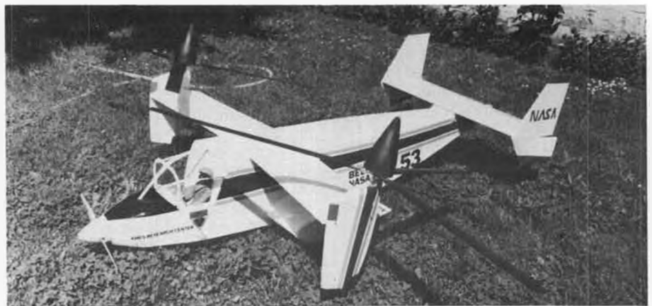
Semi-scale Bell Convertiplane R/C model by Georges Chaulet, of France. Powered by OS 90. Eight foot span model flown as autogyro (unpowered rotors).
