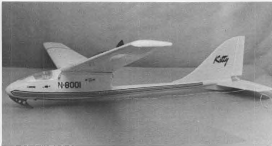
Airtronics "Kitty". Prop in safe location. Skid very helpful, allowing "no elevator" landings. Nice looking in the air.
