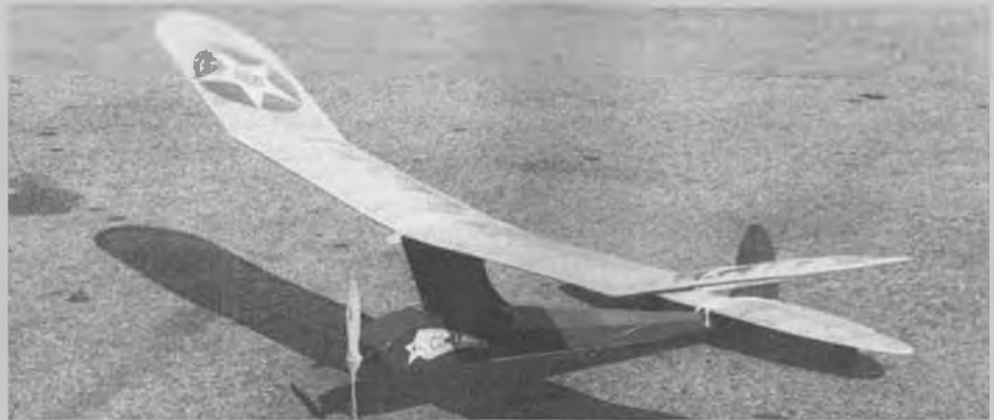
Full view of Jolly's 1-1/2 times Goldberg Interceptor. Span 74 inches, weight 38 ounces, 15-minute flights a snap.
