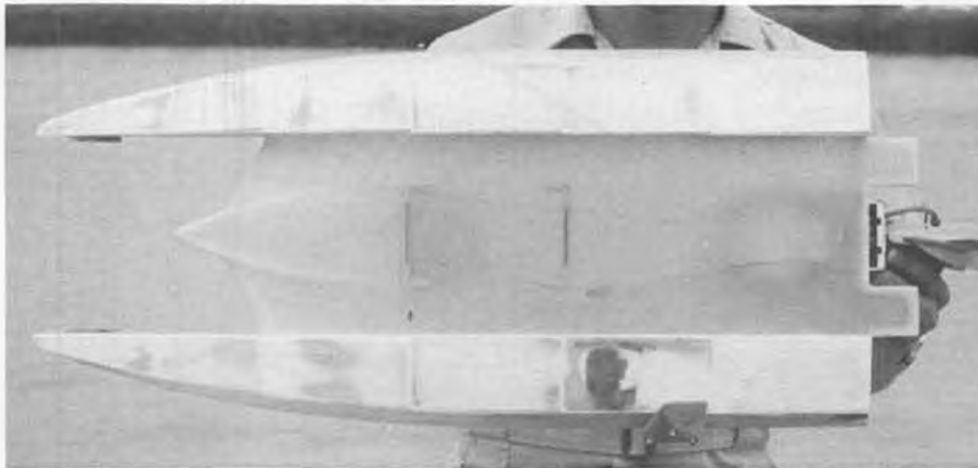
Bill Hornell shows the reworked sponson bottoms, with four steps along sponson runners.
