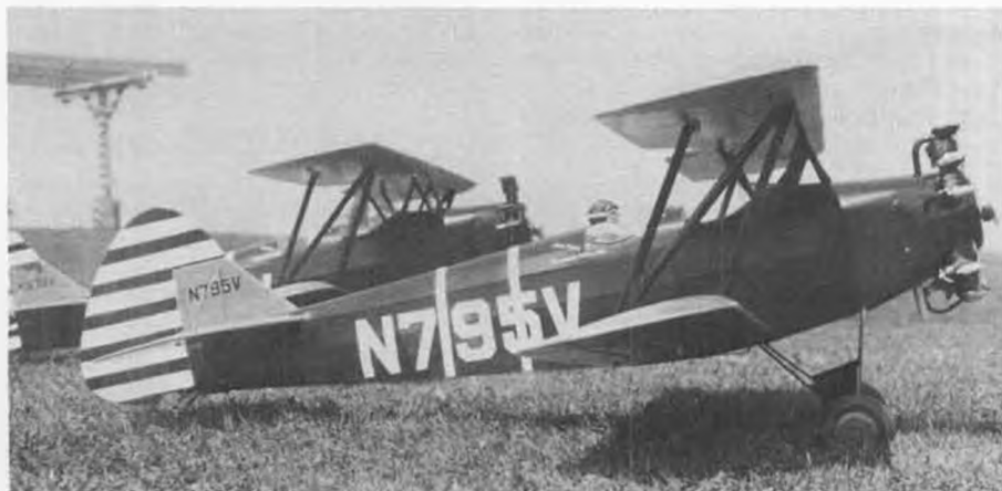
Two (his and hers) Concept Fleet Model 10's by Dick Igaz. Both Quadra powered and weighing 18 pounds. Hmmm, getting ready for formation flying?
