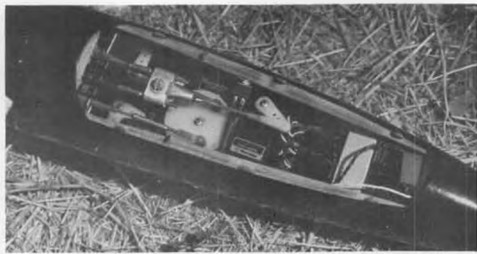
Control management department in Odle's RO-15. Rear servos for rudder and elevator. Big wheel servo for ailerons. Front servo with cable joiner for flaps. Rubicks cube easy after this!
