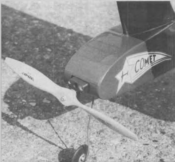
Larry Jolly's 1-1/2 times up Goldberg Interceptor, with L.J.'s 3 to 1 gear box and Leisure 05 motor.
