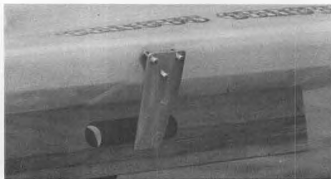
External turn fin on Ed Fisher's tunnel. Both boats finished in natural shades of epoxy glass.
