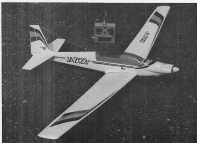
Cox Sportavia. Suggested modifications in text include reinforcing wing and streamlining nose.
