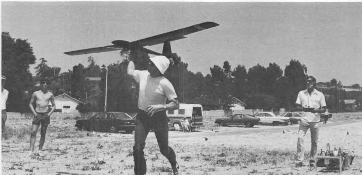
Mike Bame helps Dick Odle launch his RO-15 off "Gorilla" winch. Getting glider up to speed before letting go is a must . . . winch tends to jerk ship out of your hand otherwise.
